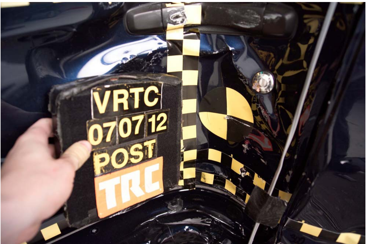
Figure A-20 Post-Test Impact Point View
