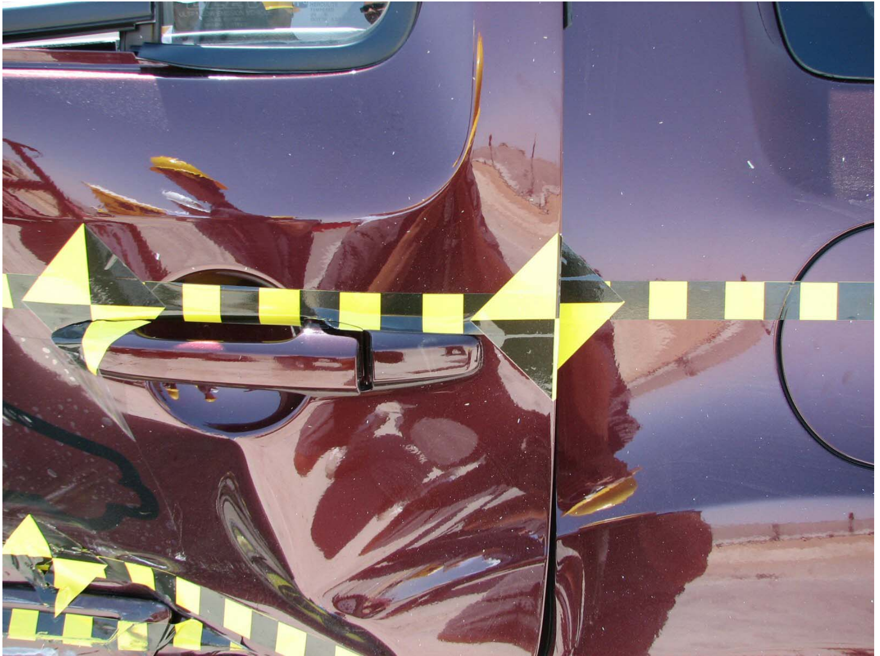
Figure A-34: Post-Test Left Rear Door
