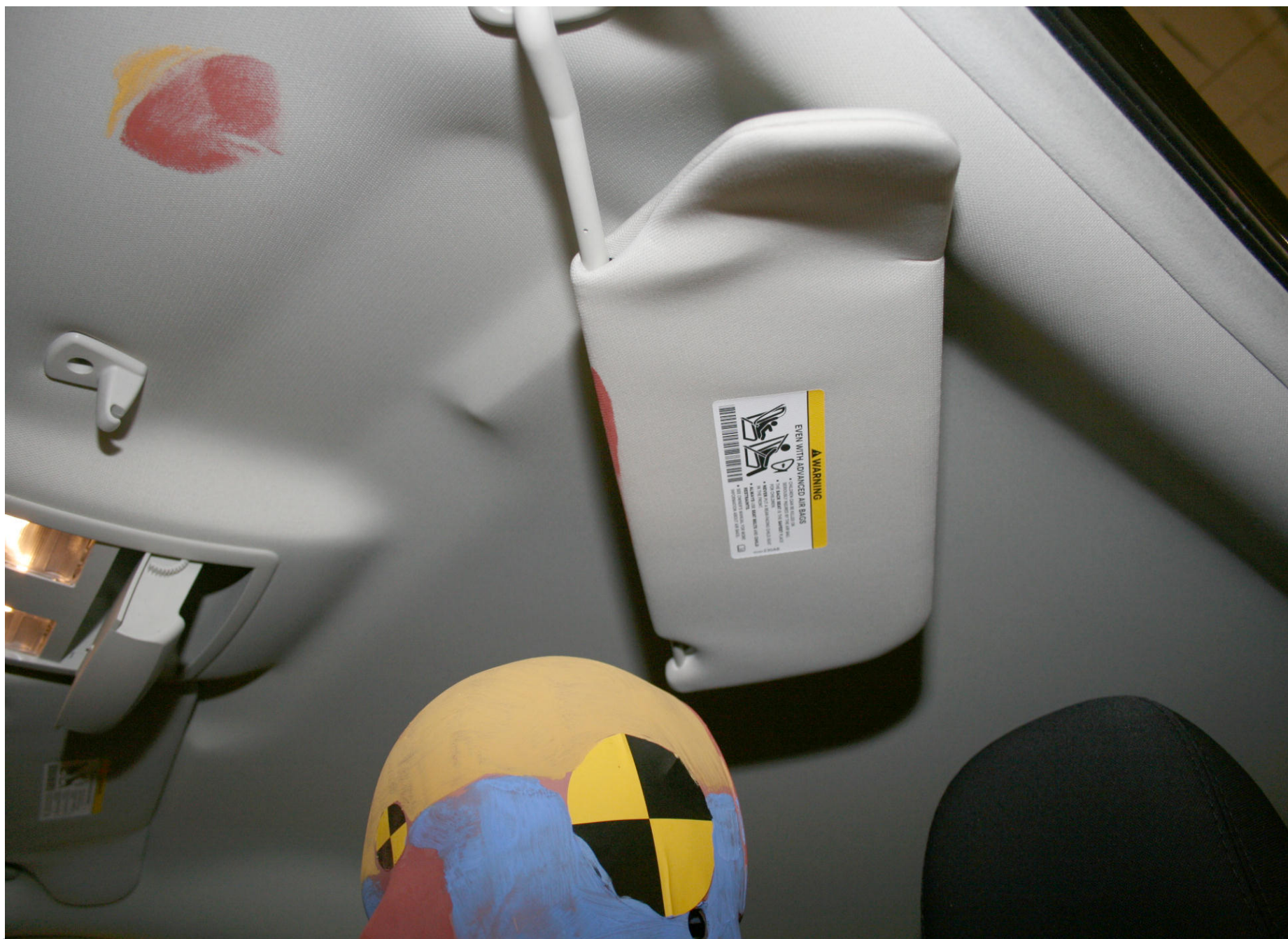
Post-Test Driver Dummy Head Contact (visor and header)
