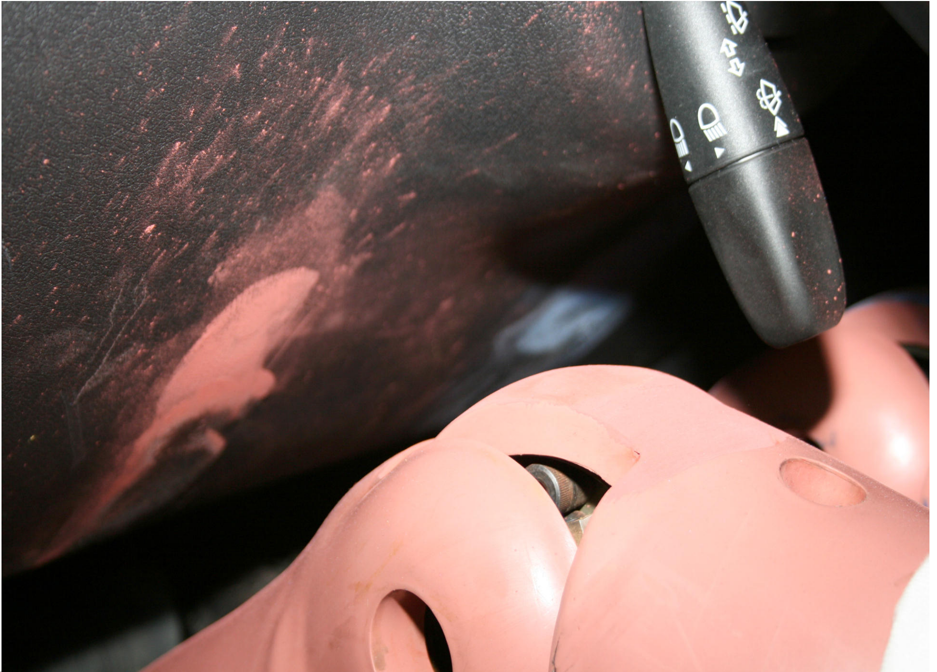
Post-Test Driver Dummy Knee Contact (left side)
