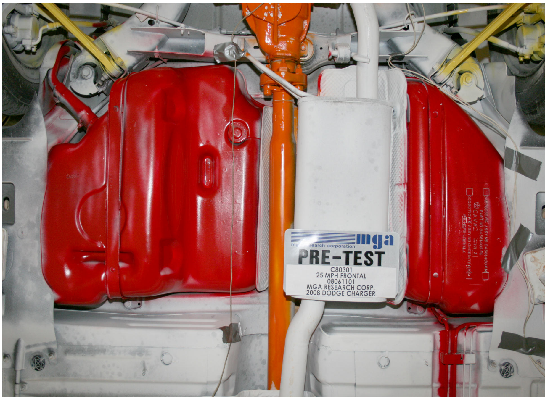
Pre-Test Fuel Tank View
