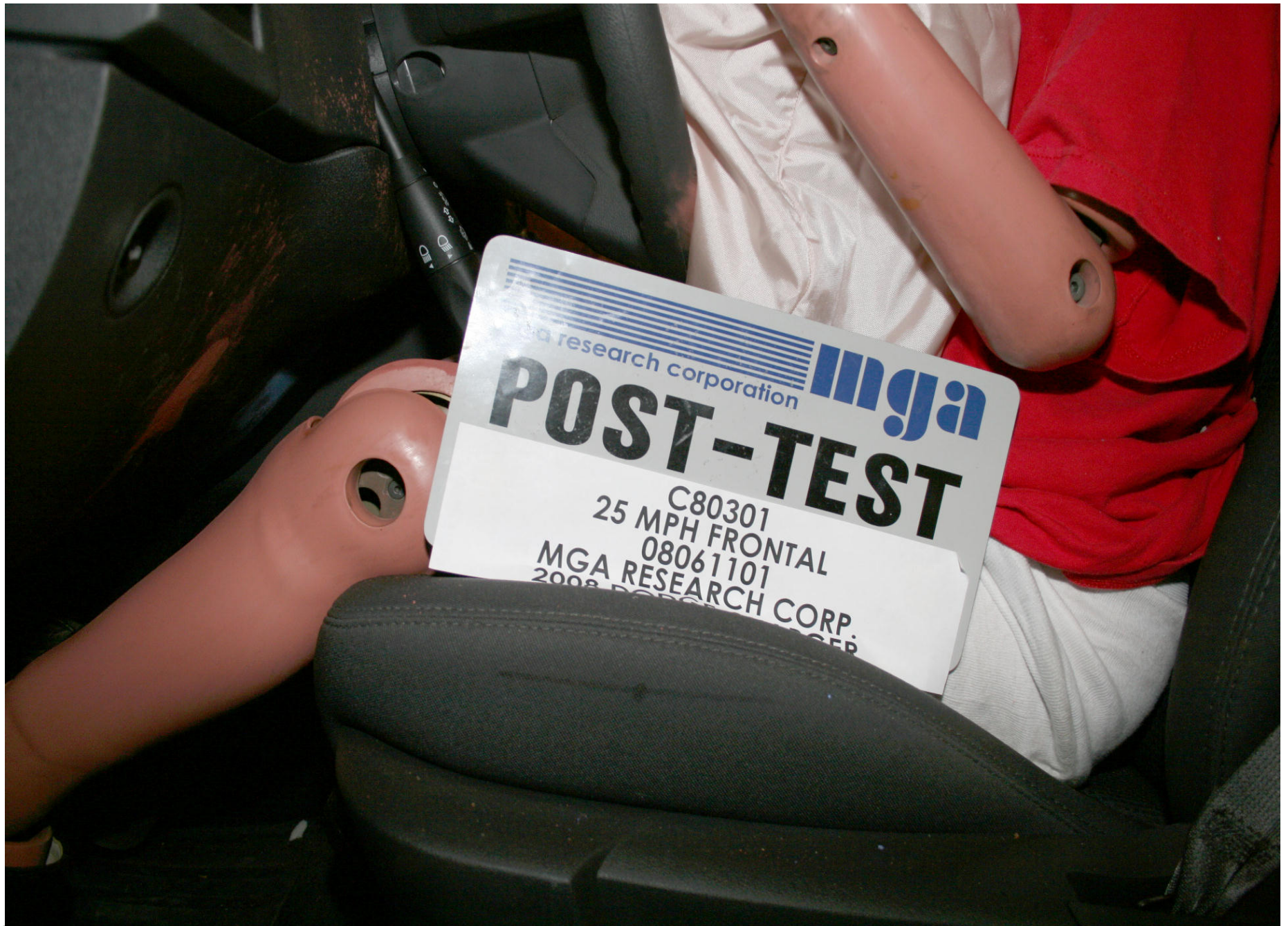
Post-Test Driver Side Knee Bolster View
