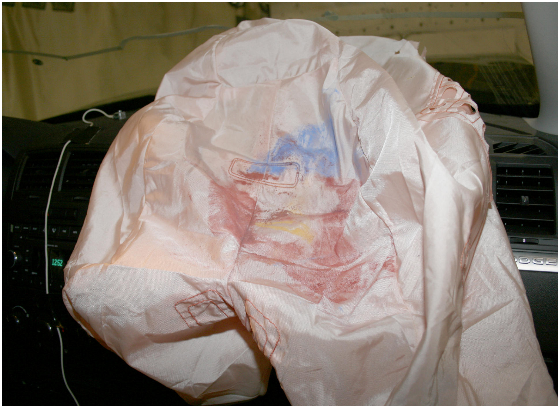
Post-Test Passenger Dummy Airbag Contact
