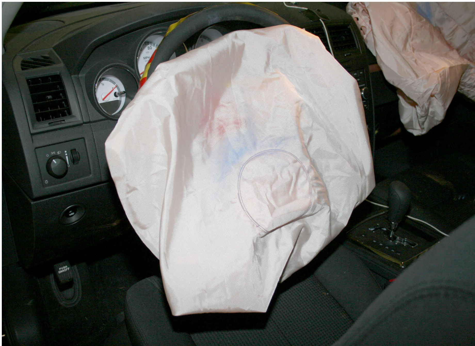
Post-Test Driver Dummy Airbag Contact
