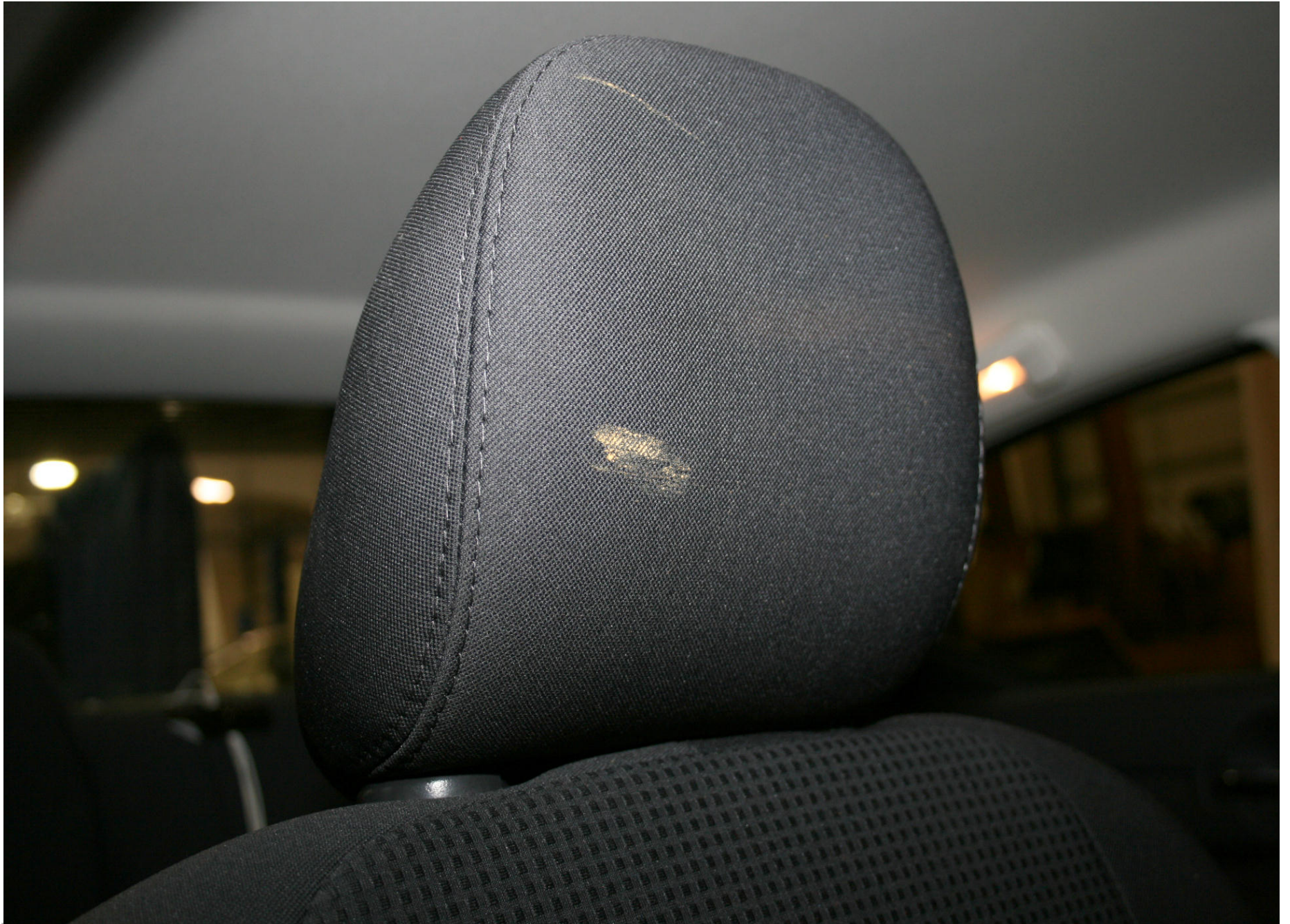
Post-Test Passenger Dummy Head Contact (headrest)
