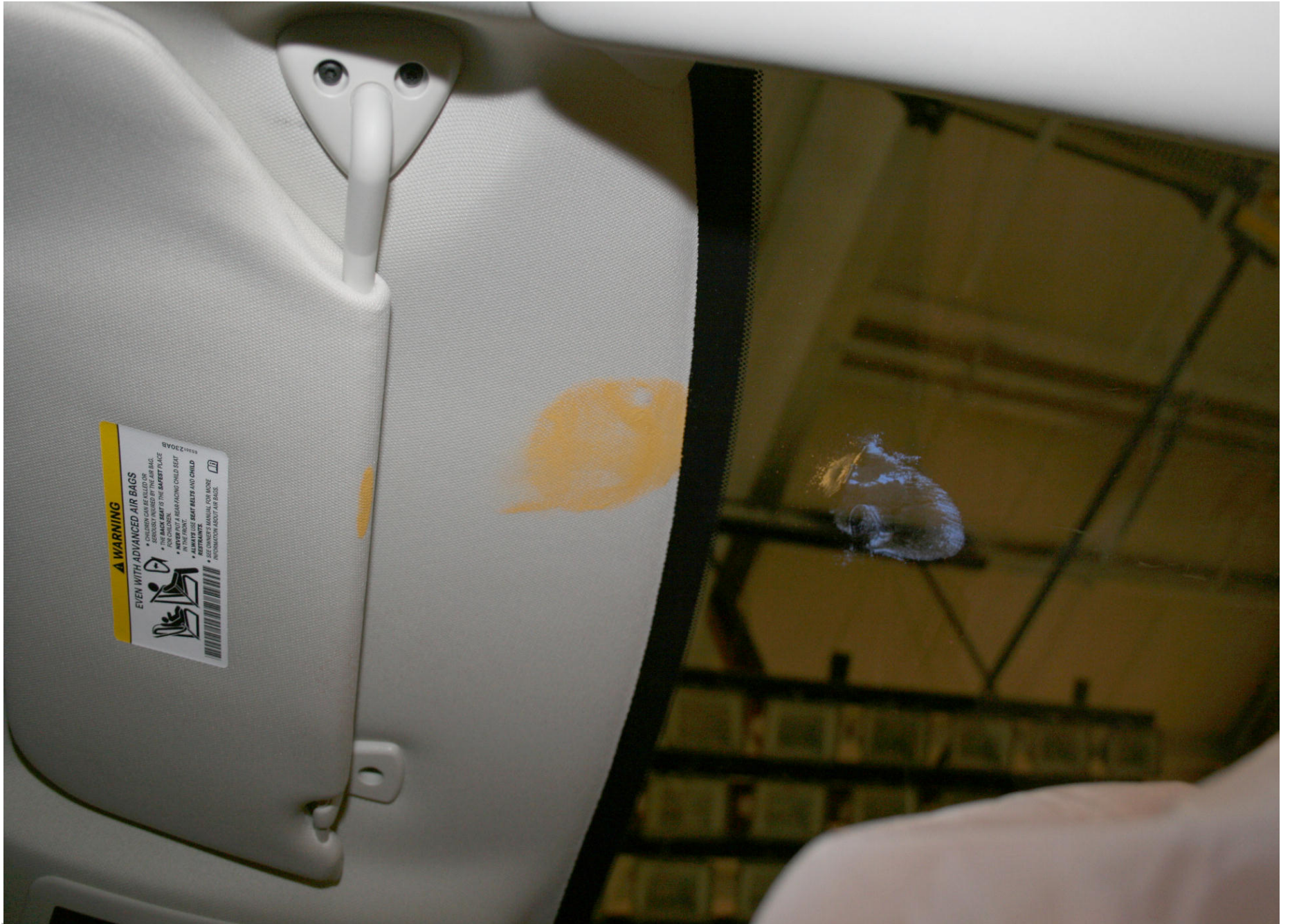
Post-Test Passenger Dummy Head Contact (visor, header & windshield)
