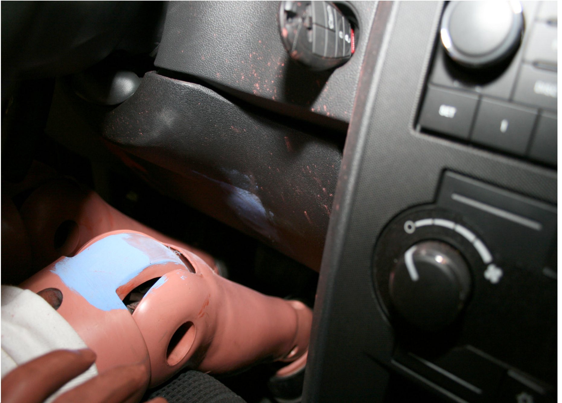
Post-Test Driver Dummy Knee Contact (right side)
