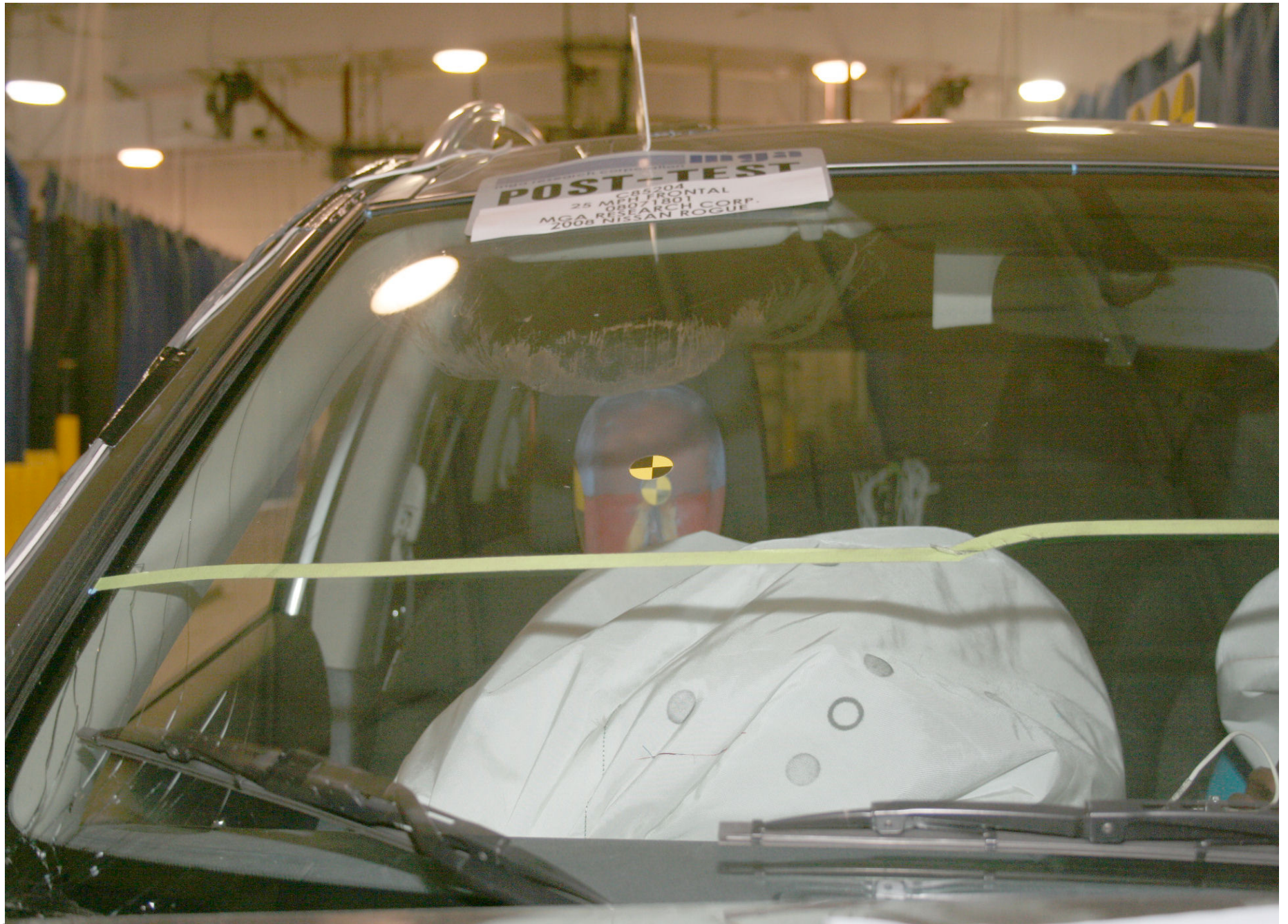
Post-Test Passenger Dummy Front View (head position)
