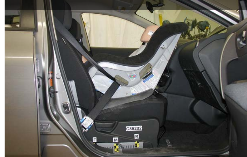
Century Encore Rear Facing Belted, Middle Seat Track
