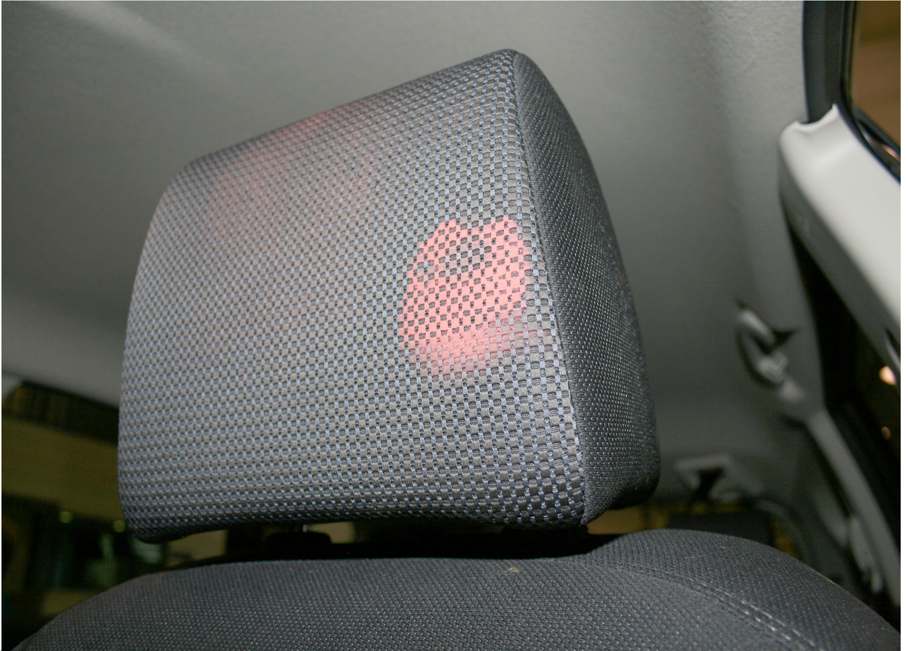
Post-Test Driver Dummy Head Contact (headrest)
