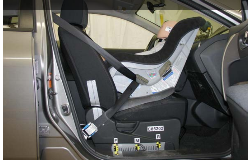
Century Encore Rear Facing Belted, Forward Seat Track
