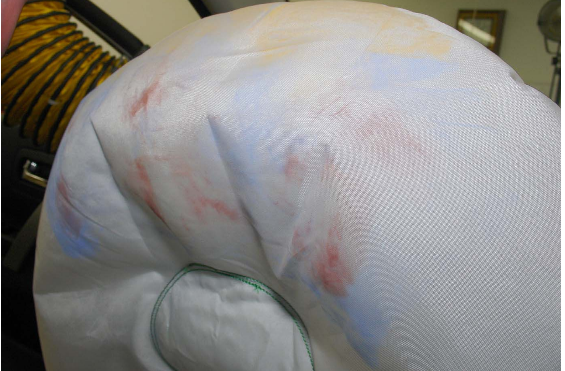
Post-Test 5th Fem. P1 Driver Dummy Airbag Right Side View
