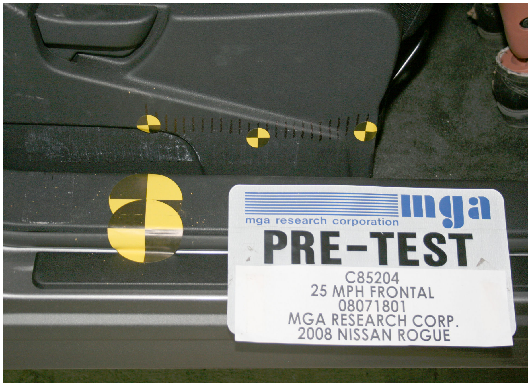
Pre-Test Passenger Dummy Seat Position
