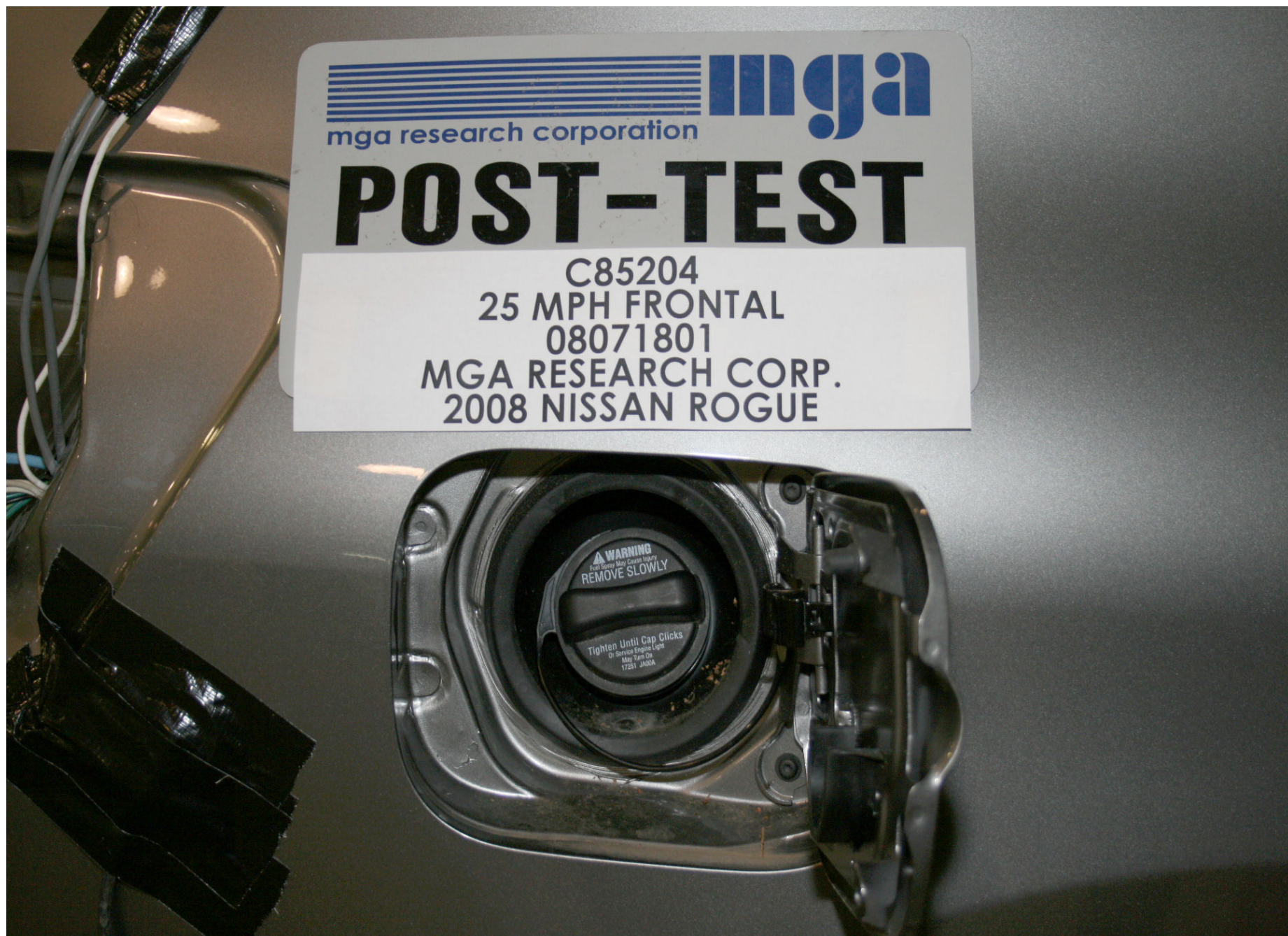
Post-Test Fuel Filler Cap View
