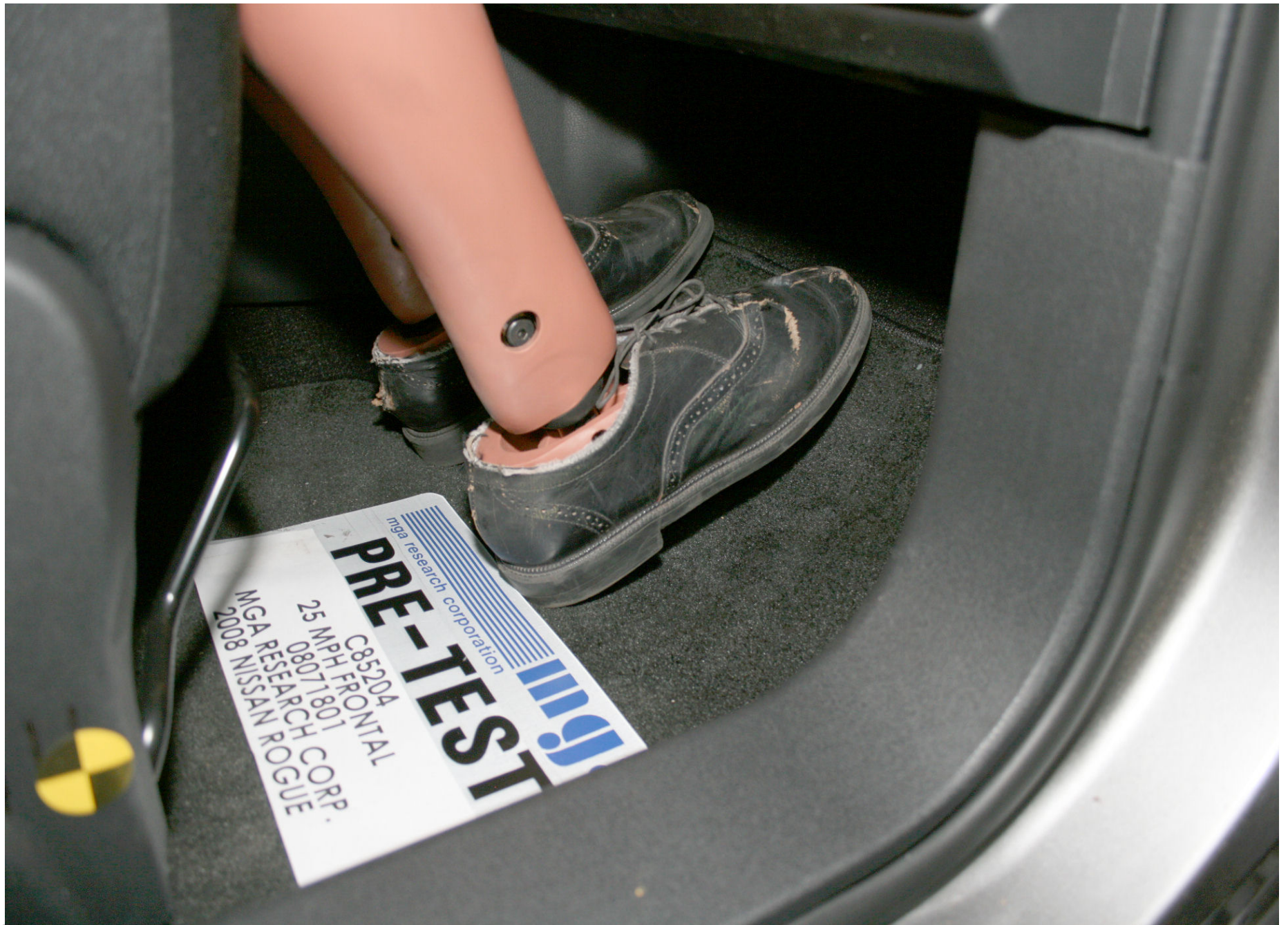
Pre-Test Passenger Dummy Feet Position
