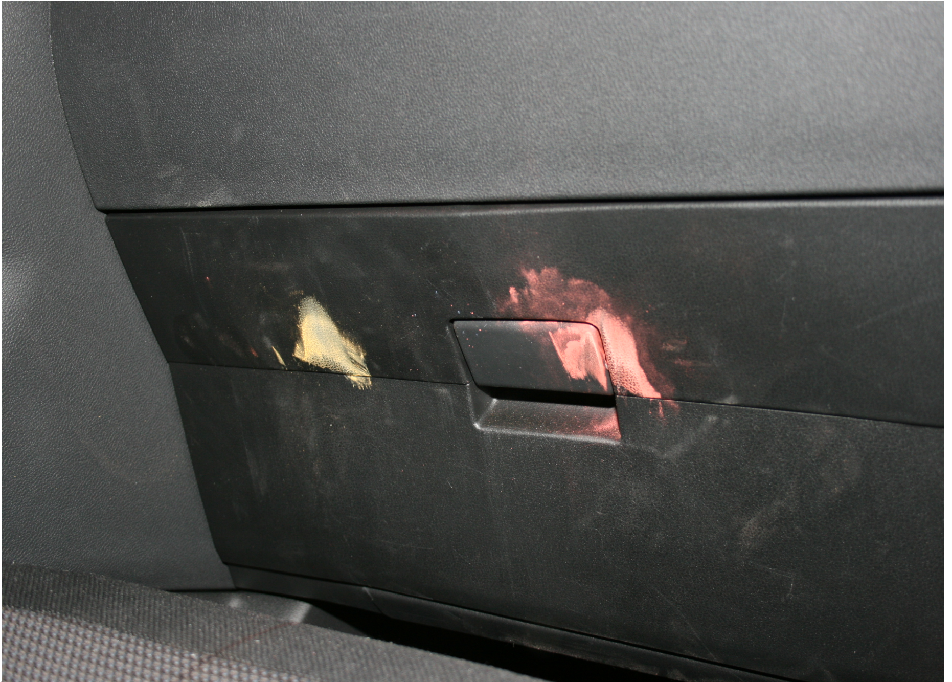
Post-Test Passenger Dummy Knee Contact
