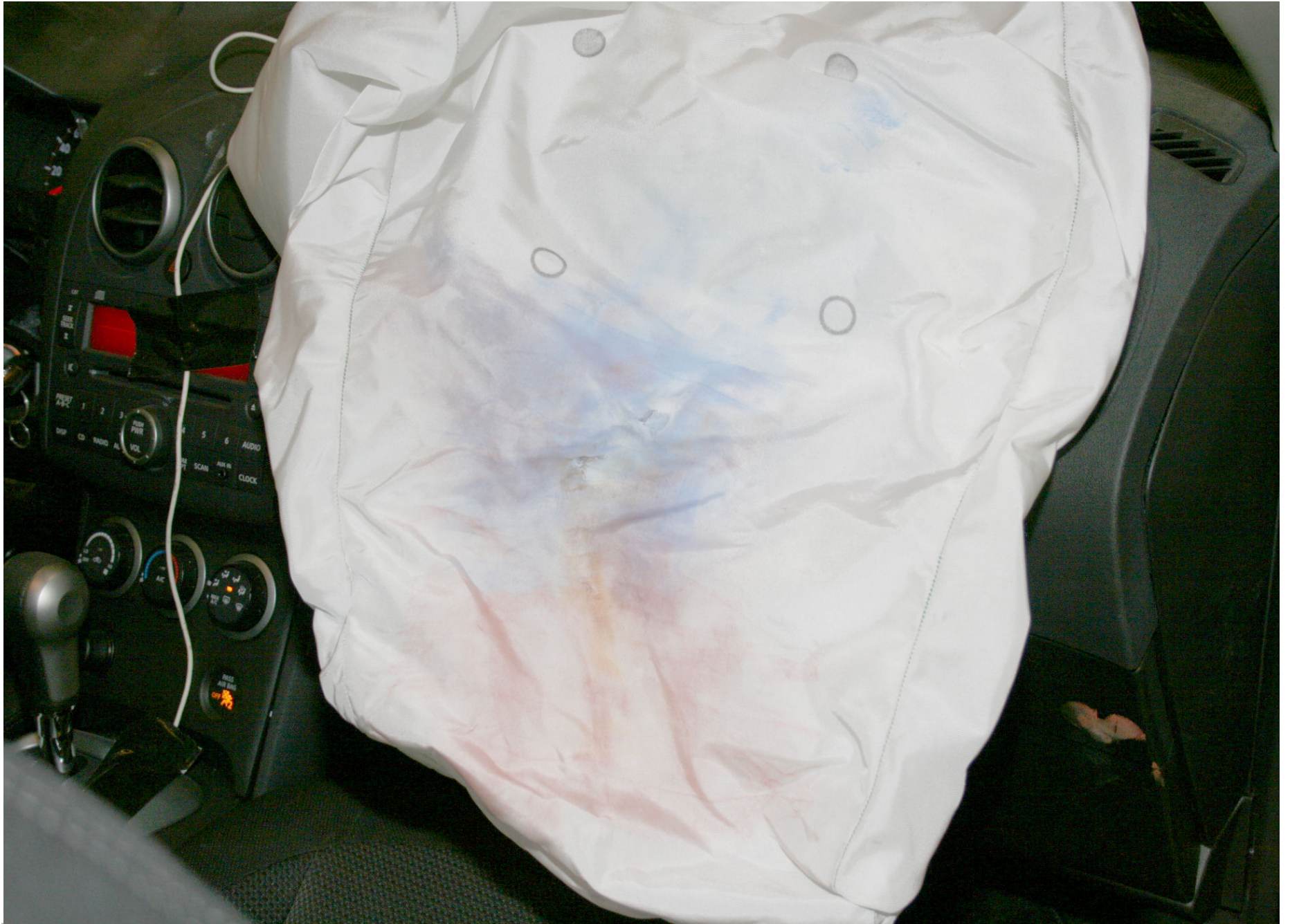
Post-Test Passenger Dummy Airbag Contact
