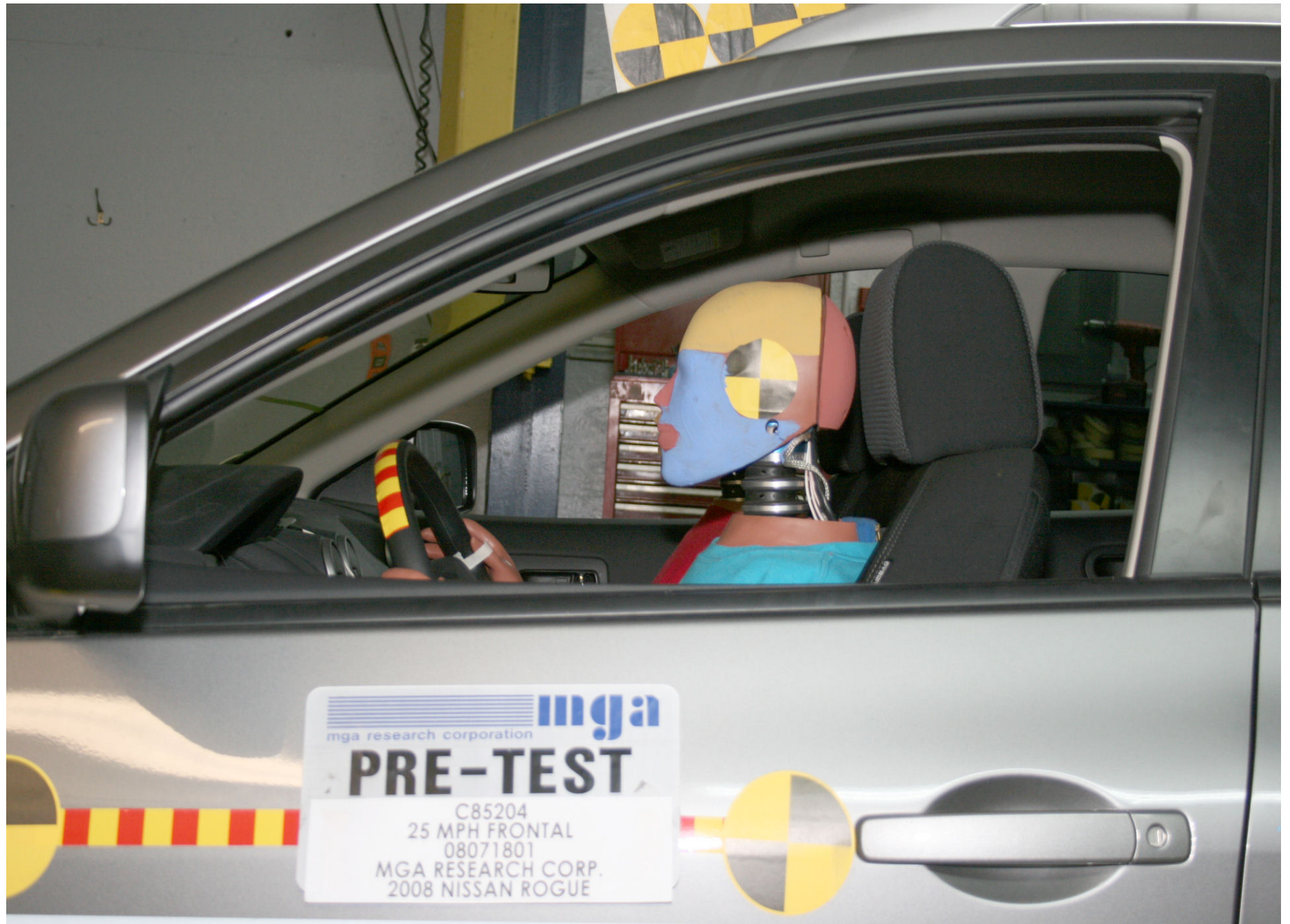
Pre-Test Driver Dummy Position Left Side View
