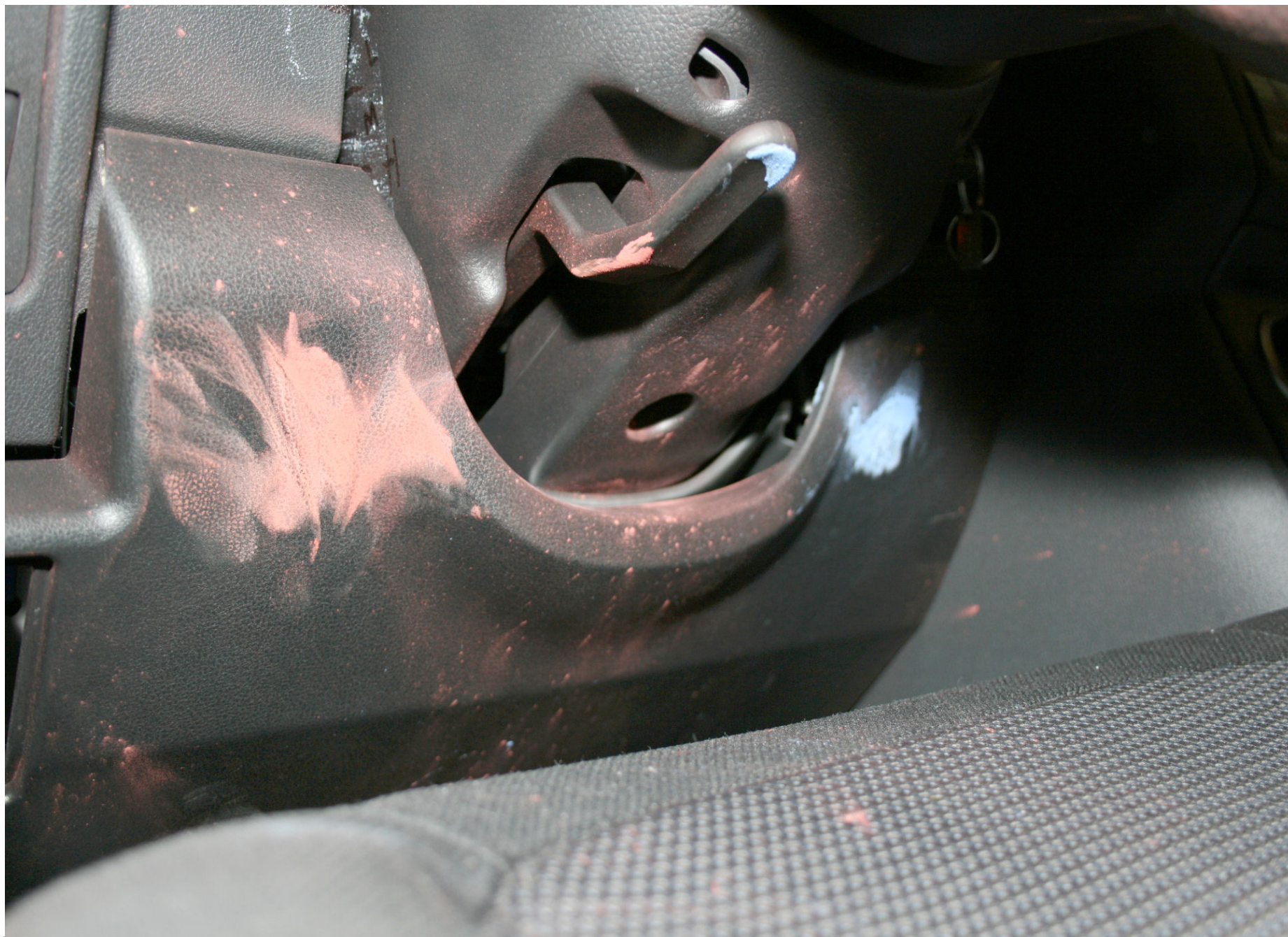
Post-Test Driver Dummy Knee Contact
