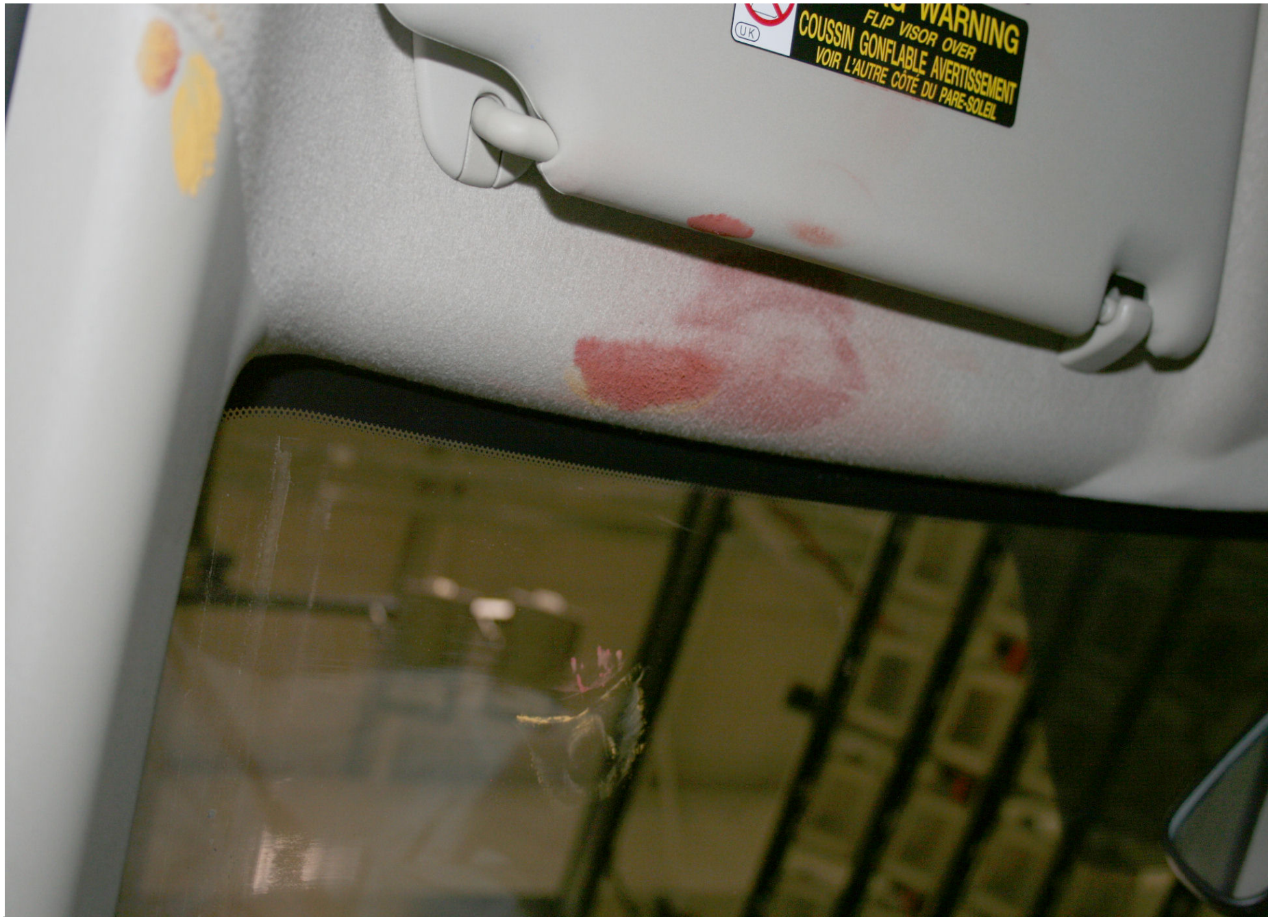
Post-Test Driver Dummy Head Contract (header and visor)
