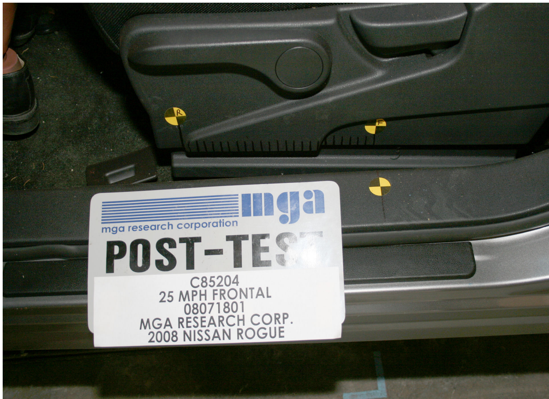
Post-Test Driver Dummy Seat Position
