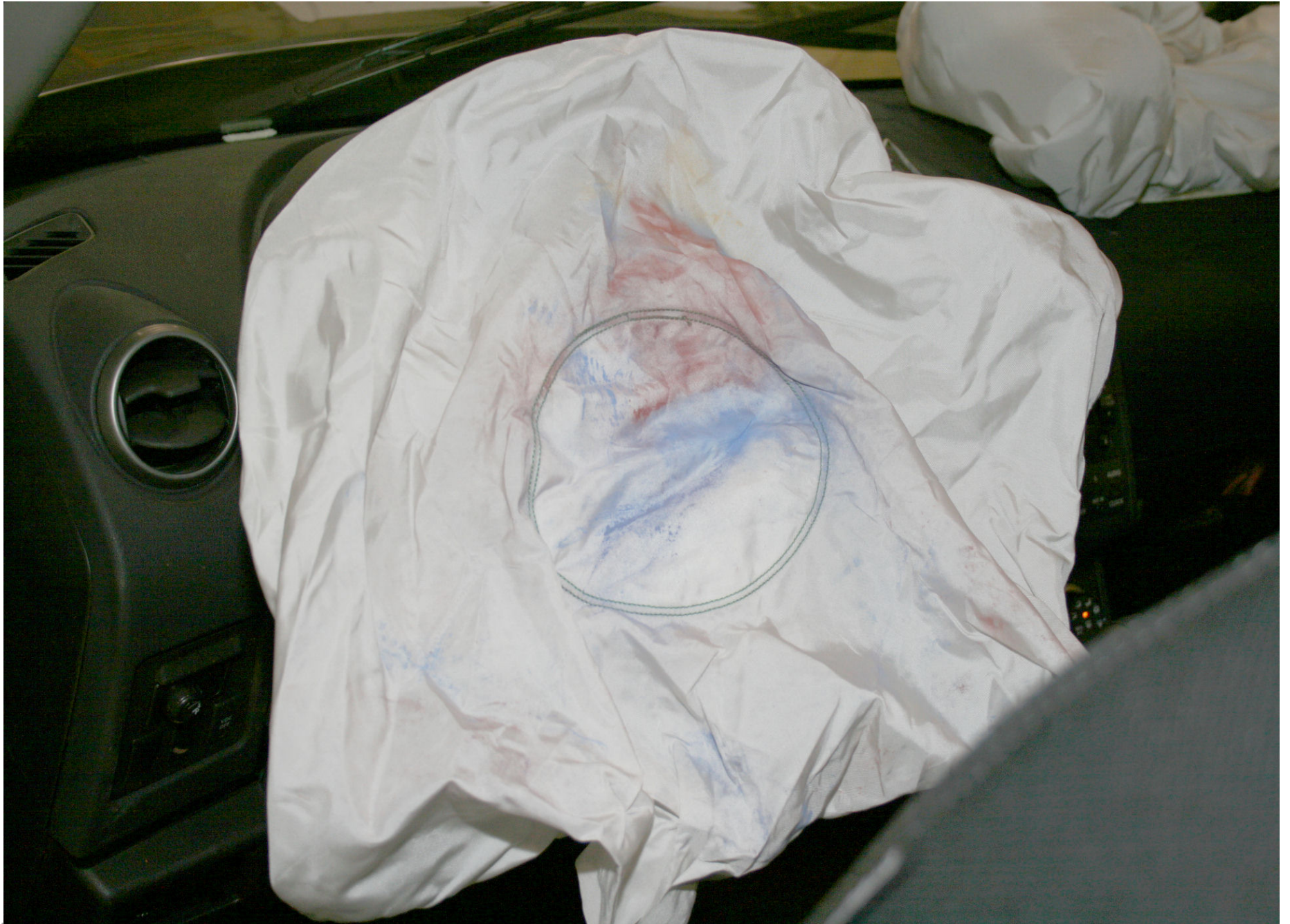
Post-Test Driver Dummy Airbag Contact
