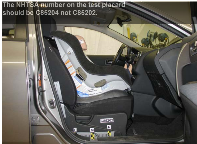
Century Encore Forward Facing Unbelted, Middle Seat Track The NHTSA number on the test placard should be C85204 not C85202.
