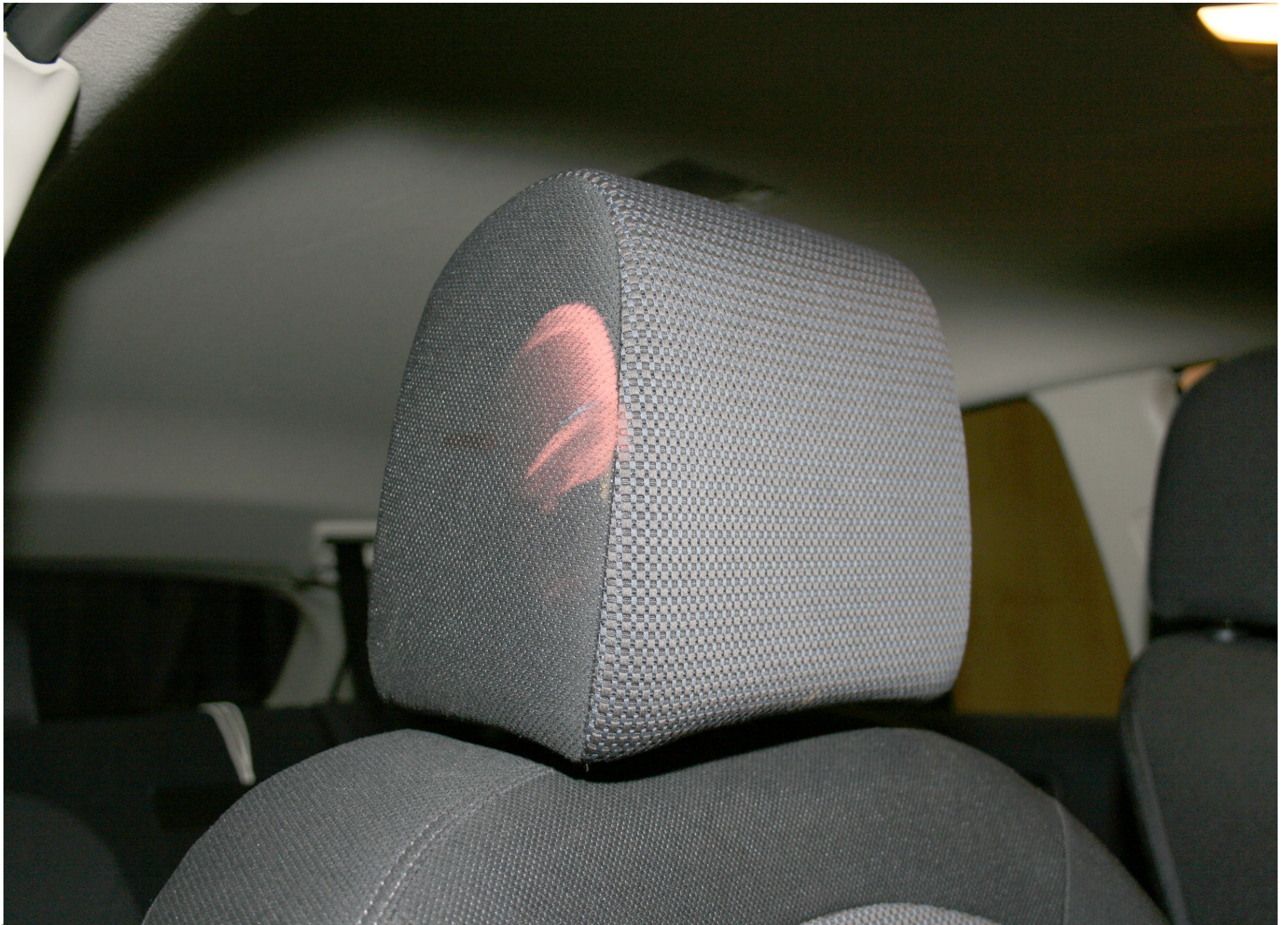
Post-Test Passenger Dummy Head Contact View (headrest)
