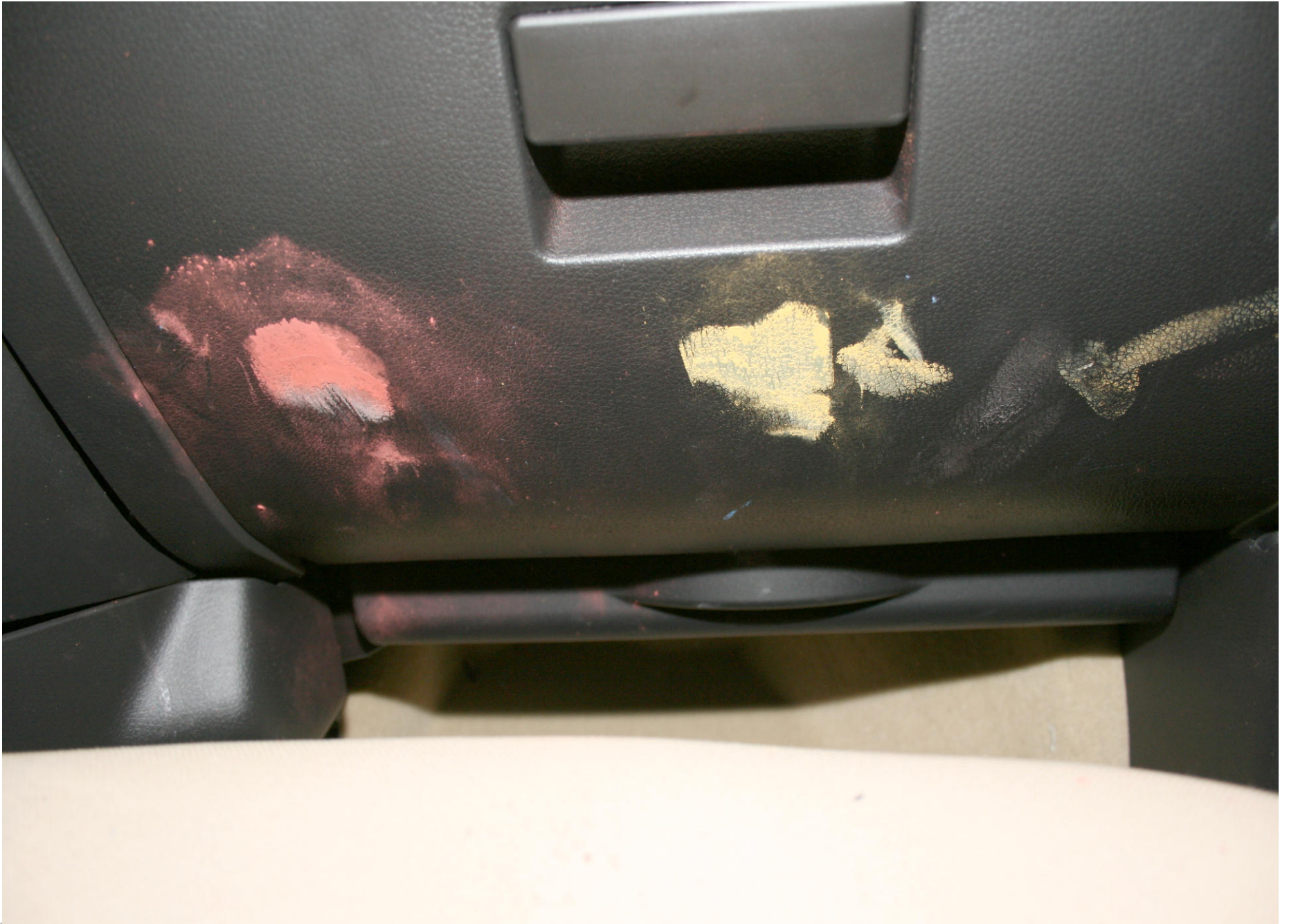
Post-Test Passenger Dummy Knee Contact
