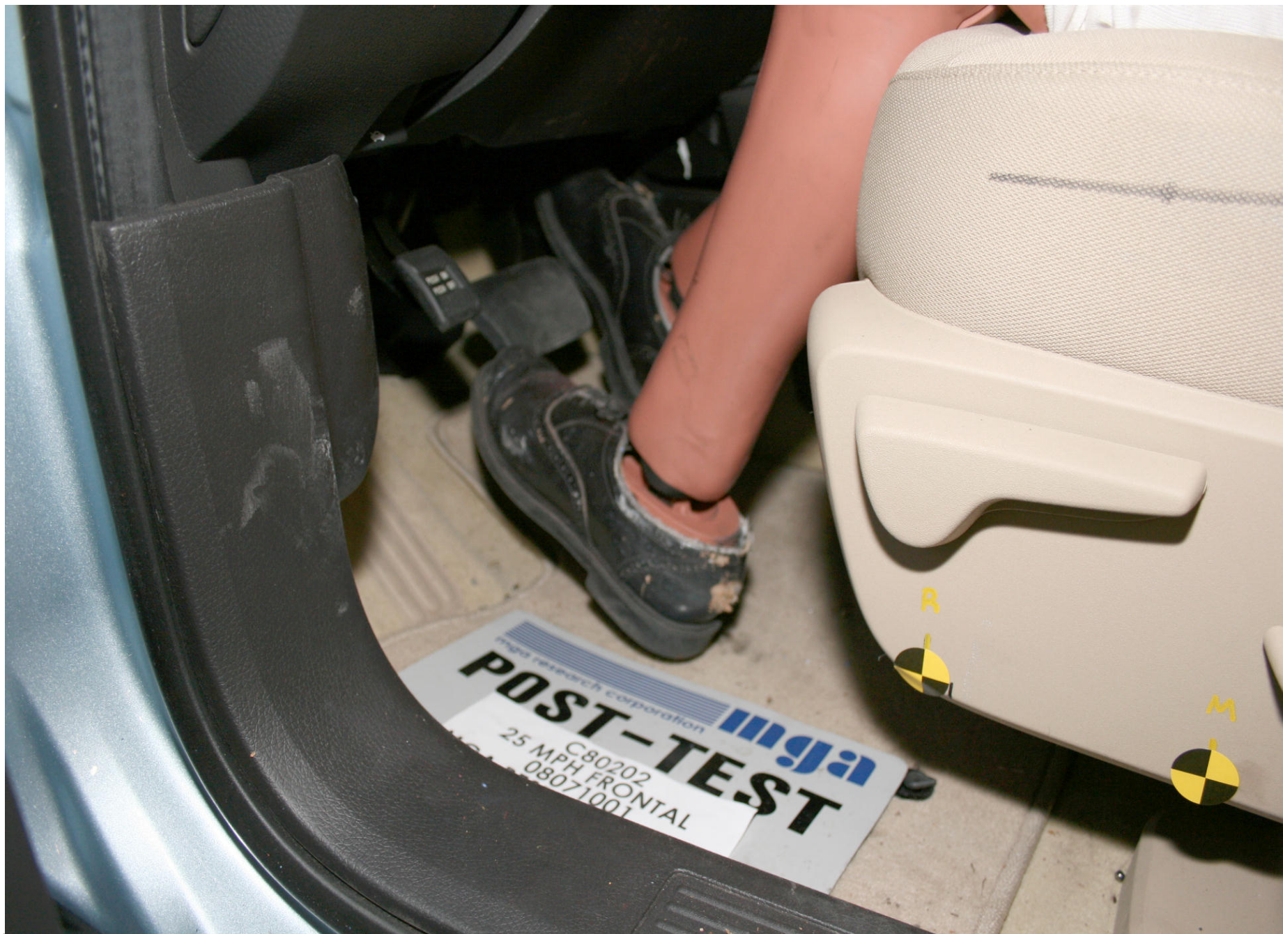
Post-Test Driver Dummy Feet Position
