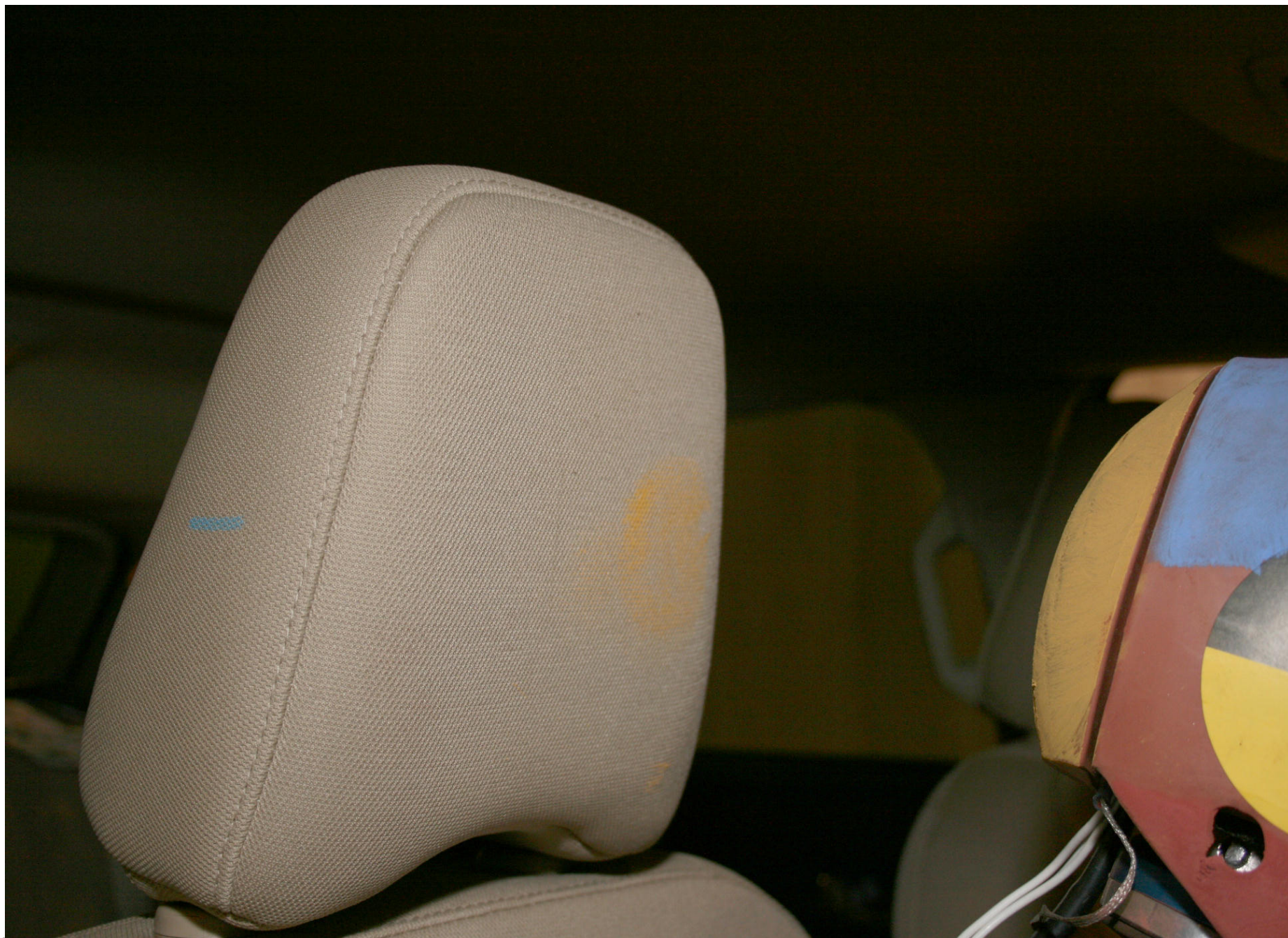
Post-Test Passenger Dummy Head Contact View (headrest)
