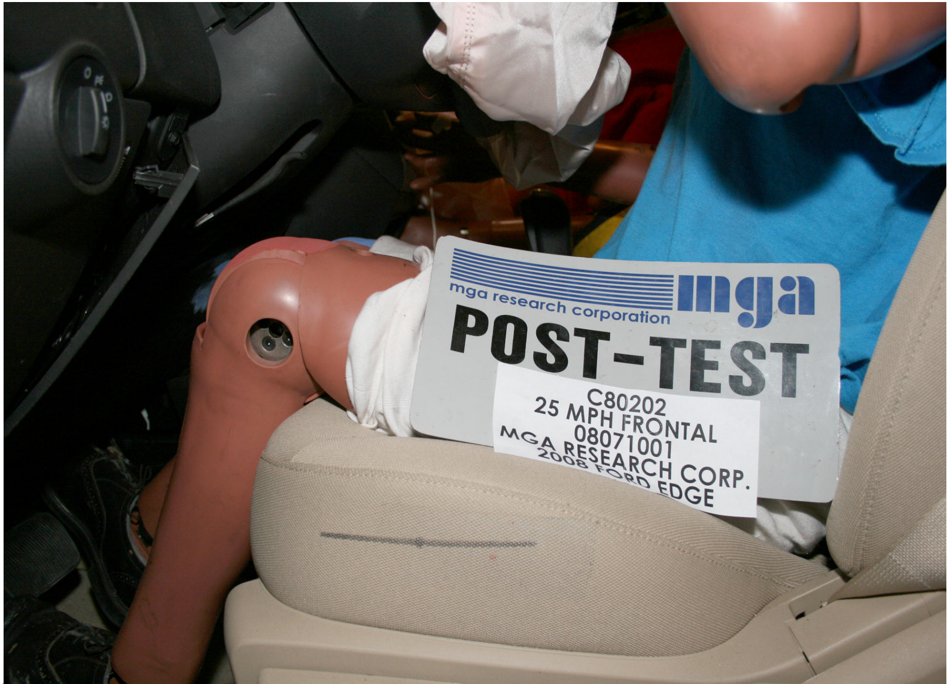
Post-Test Driver Side Knee Bolster View
