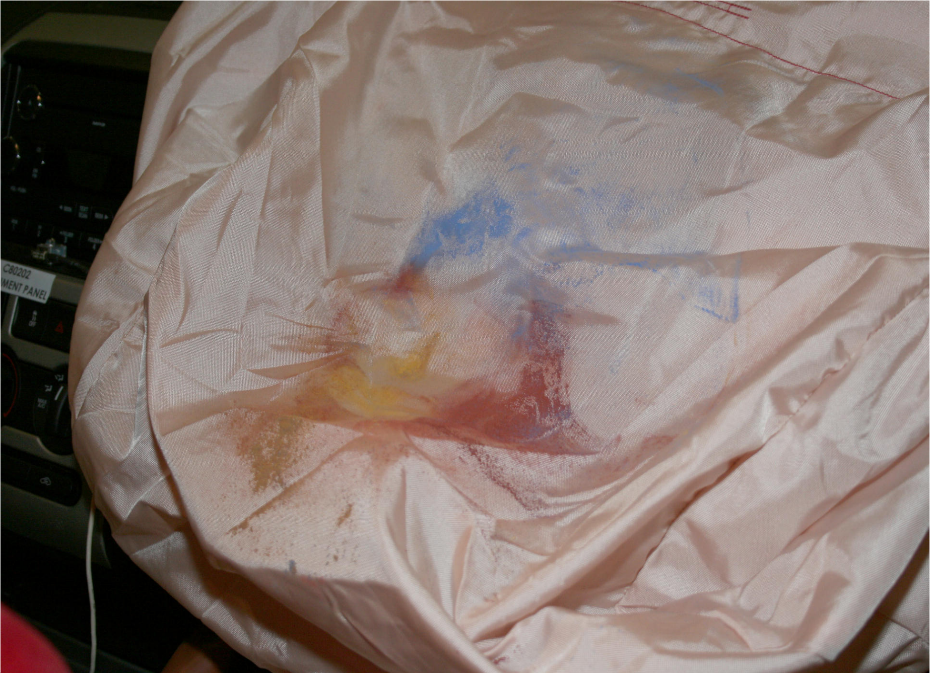
Post-Test Passenger Dummy Airbag Contact
