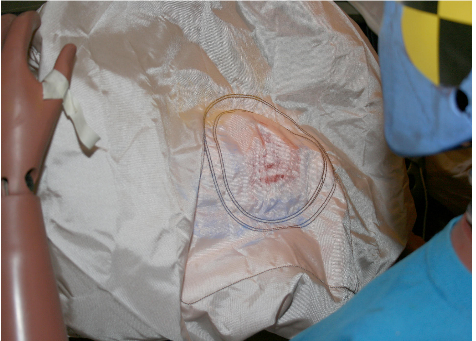
Post-Test Driver Dummy Airbag Contact
