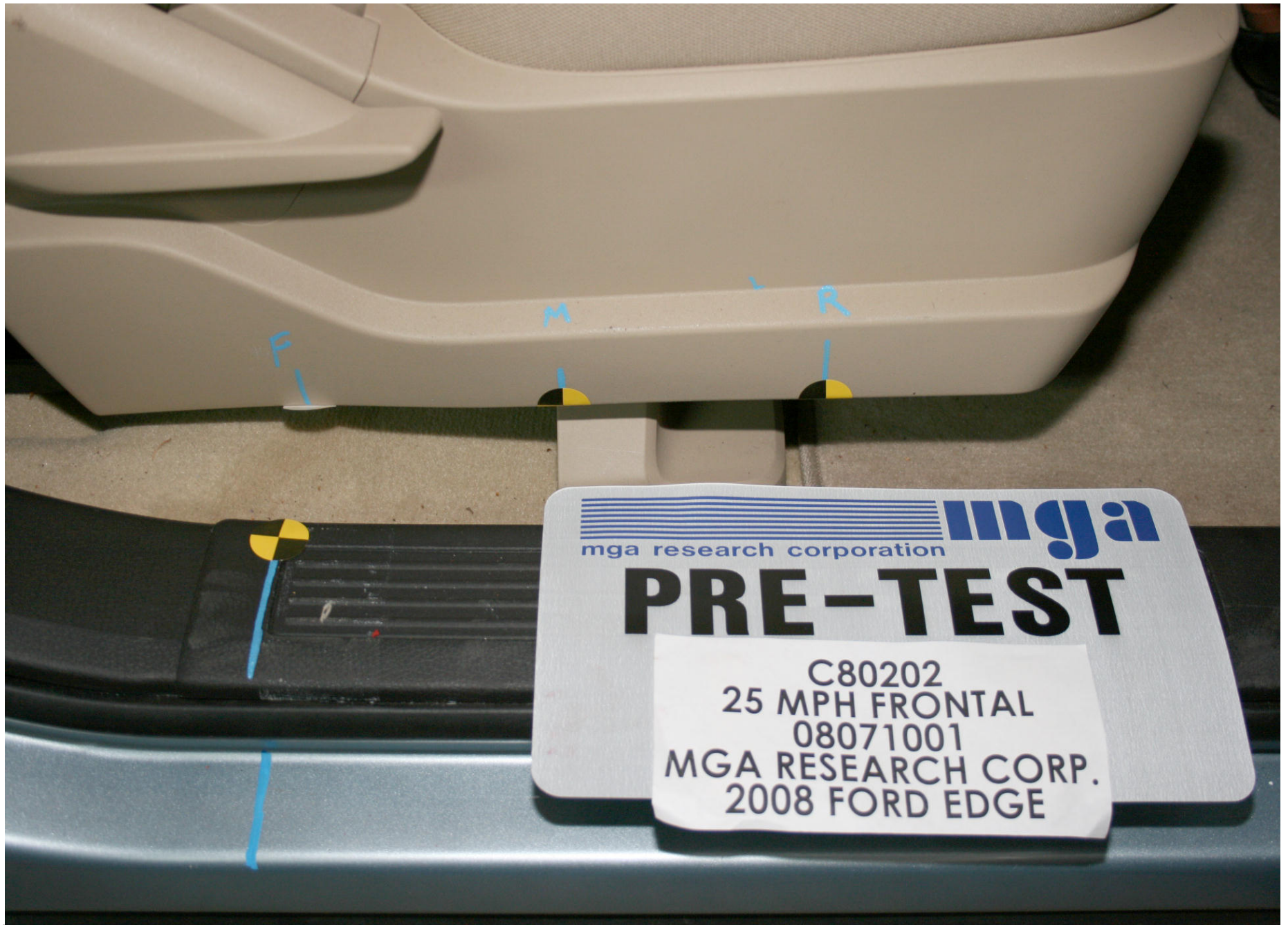
Pre-Test Passenger Dummy Seat Position
