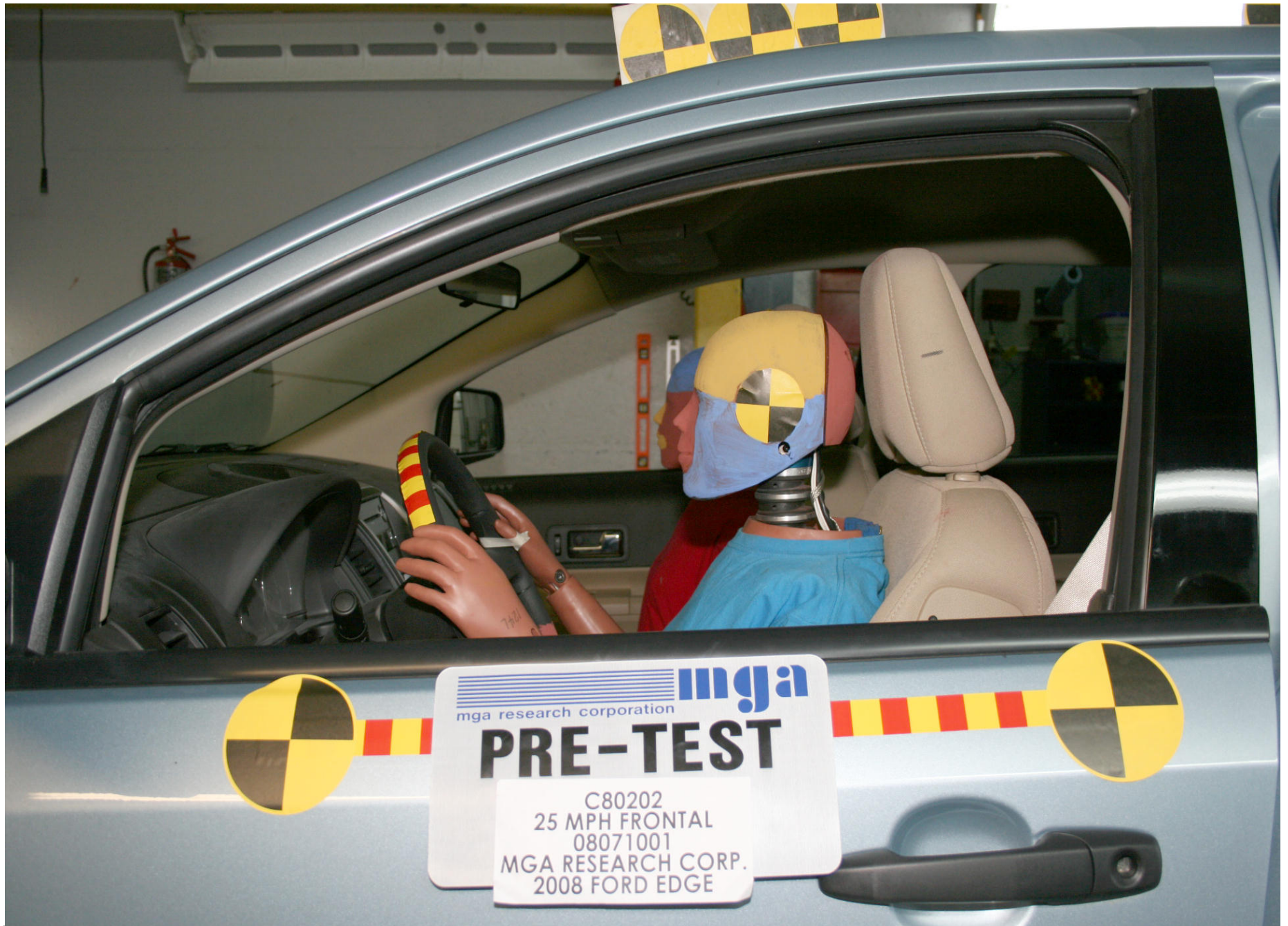
Pre-Test Driver Dummy Position Left Side View
