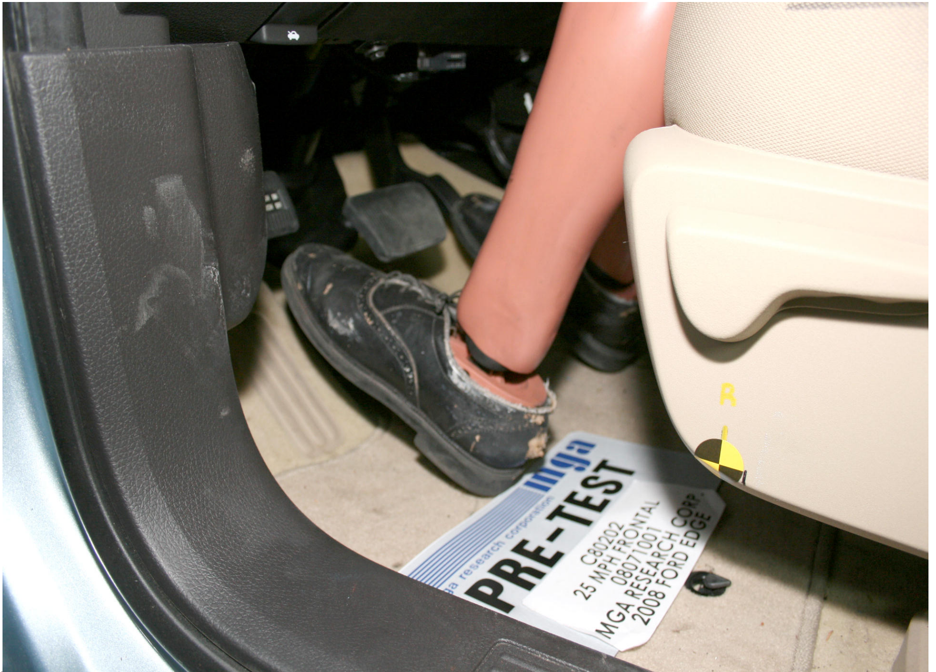
Pre-Test Driver Dummy Feet Position
