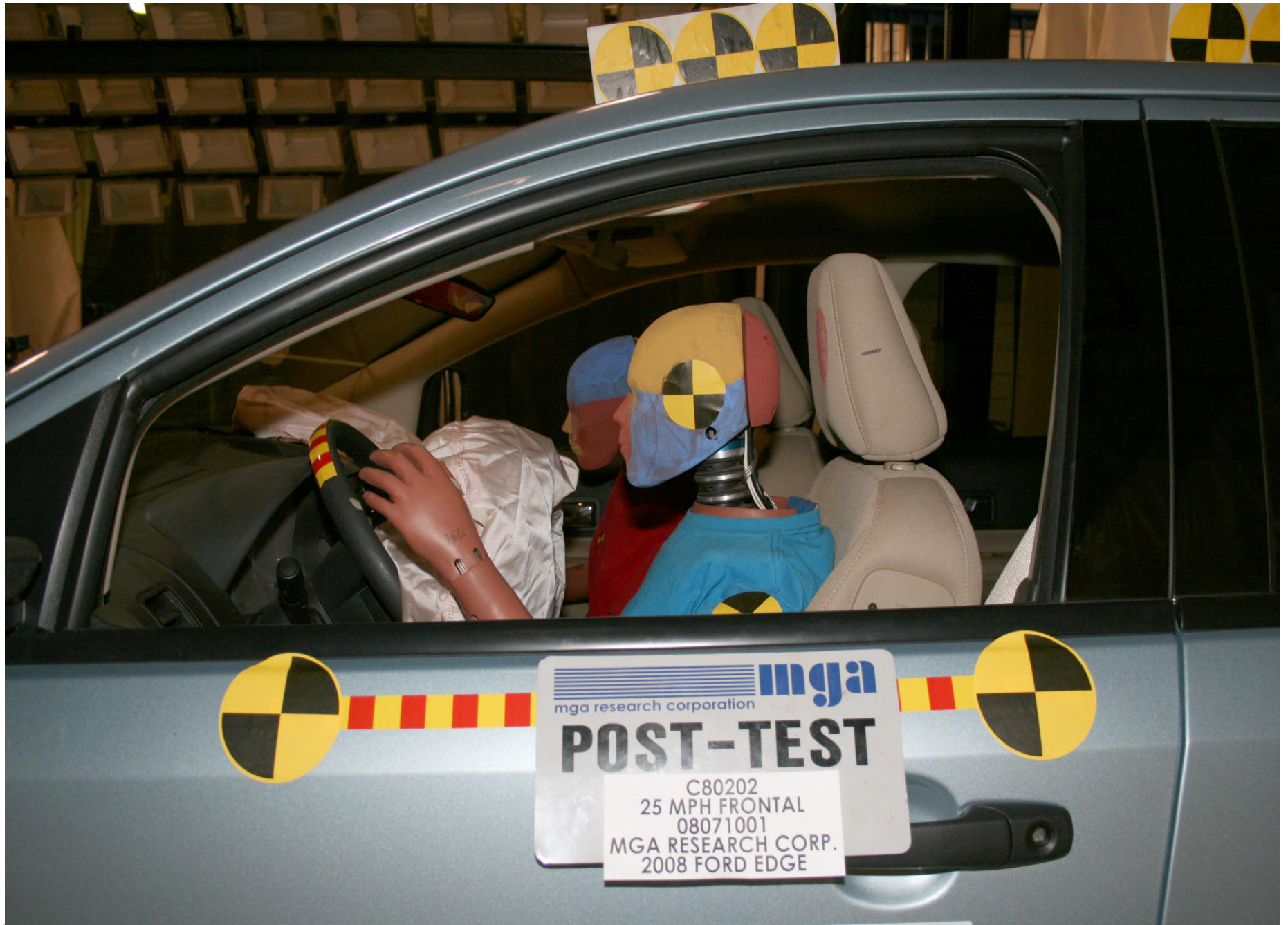
Post-Test Driver Dummy Position Left Side View
