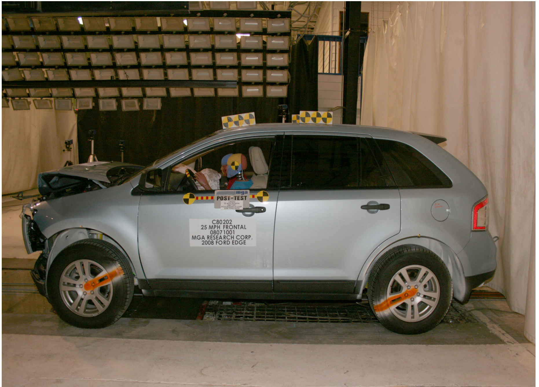
Post-Test Left Side View of Test Vehicle
