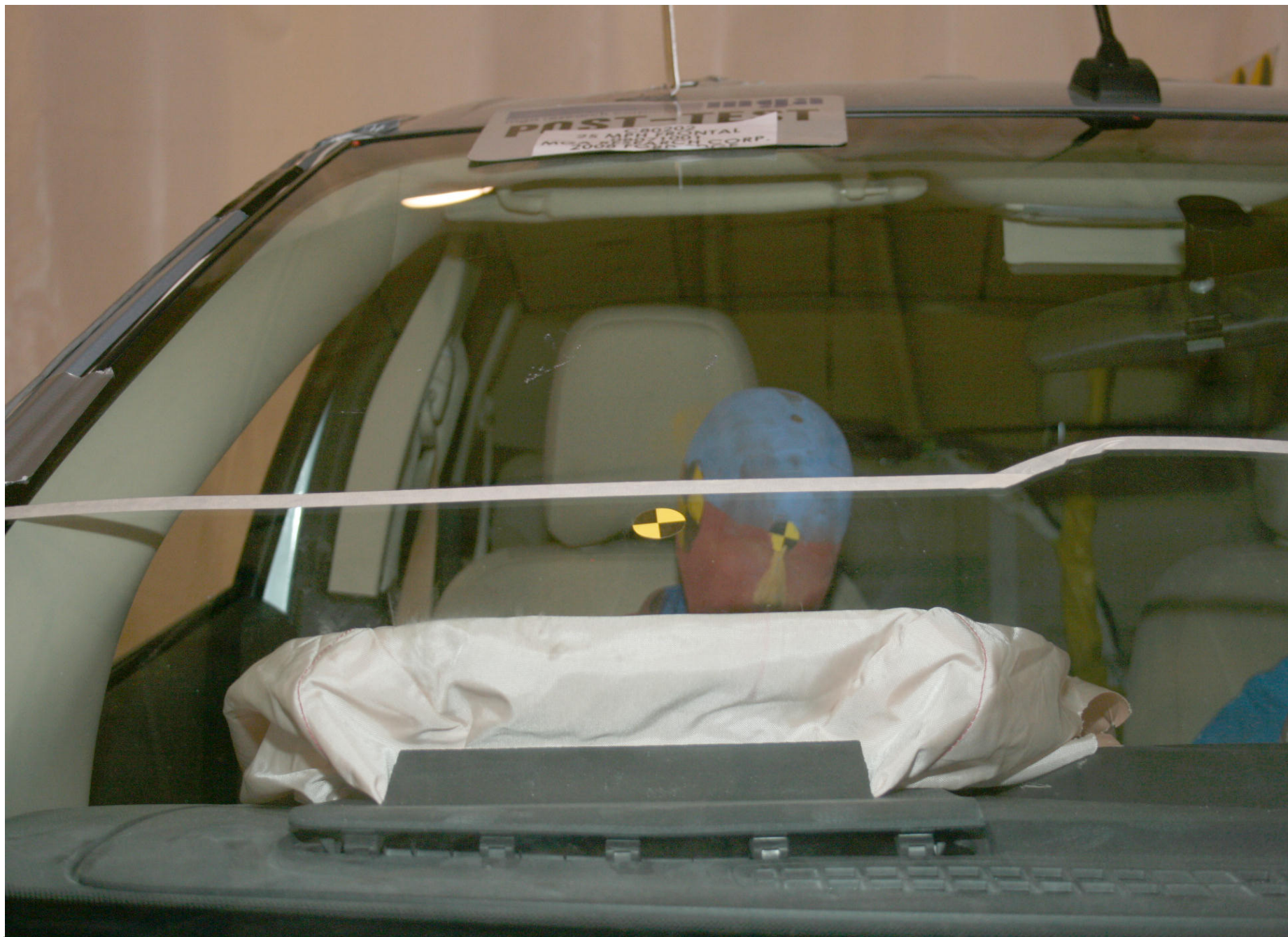
Post-Test Passenger Dummy Front View (head position)
