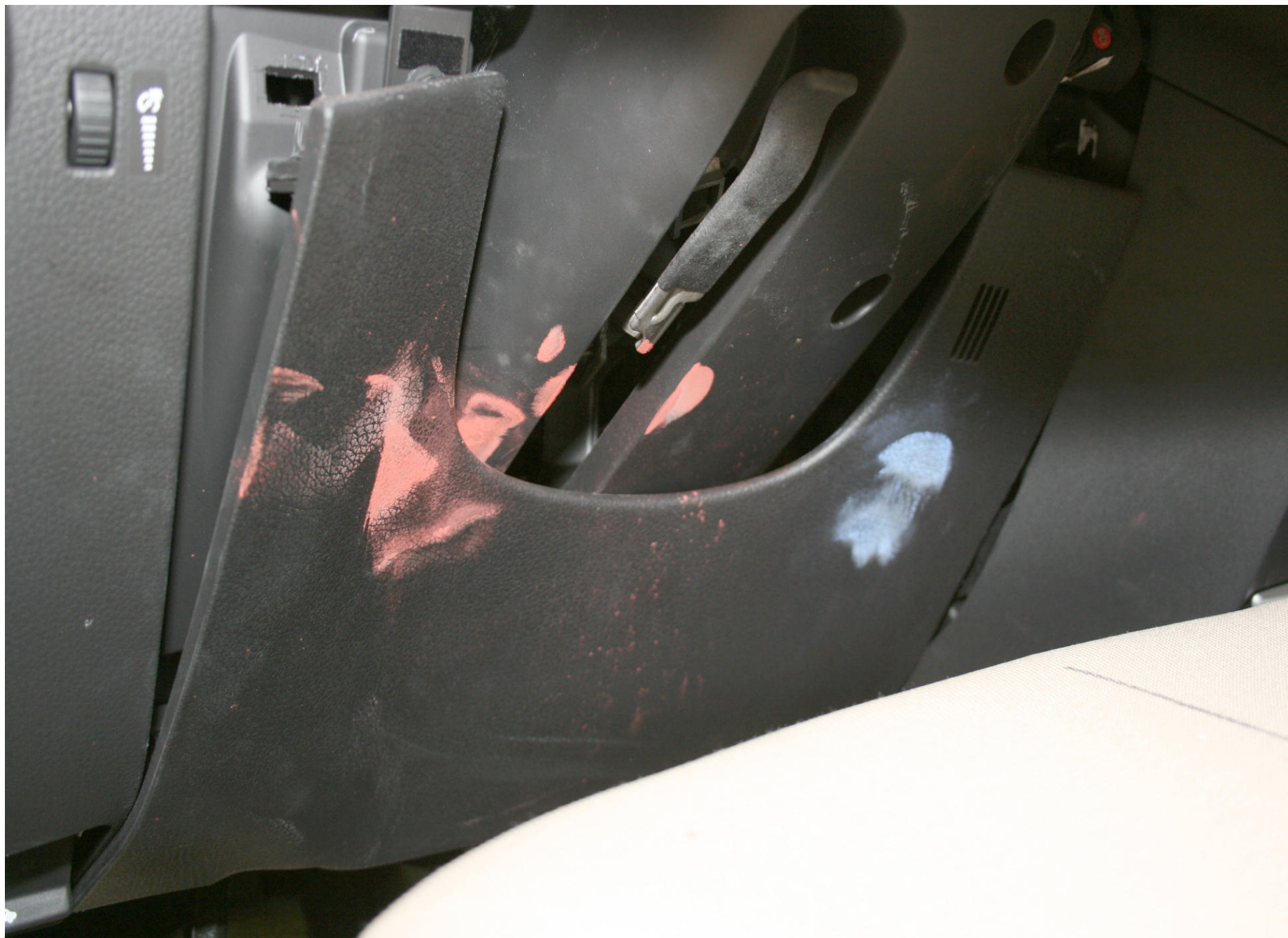
Post-Test Driver Dummy Knee Contact
