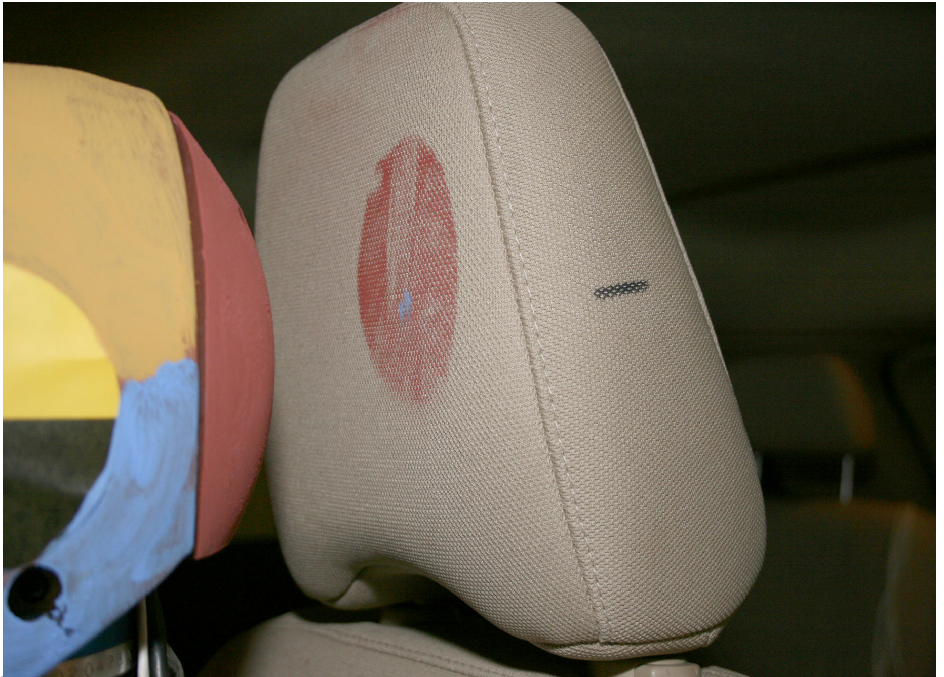
Post-Test Driver Dummy Head Contact (headrest)
