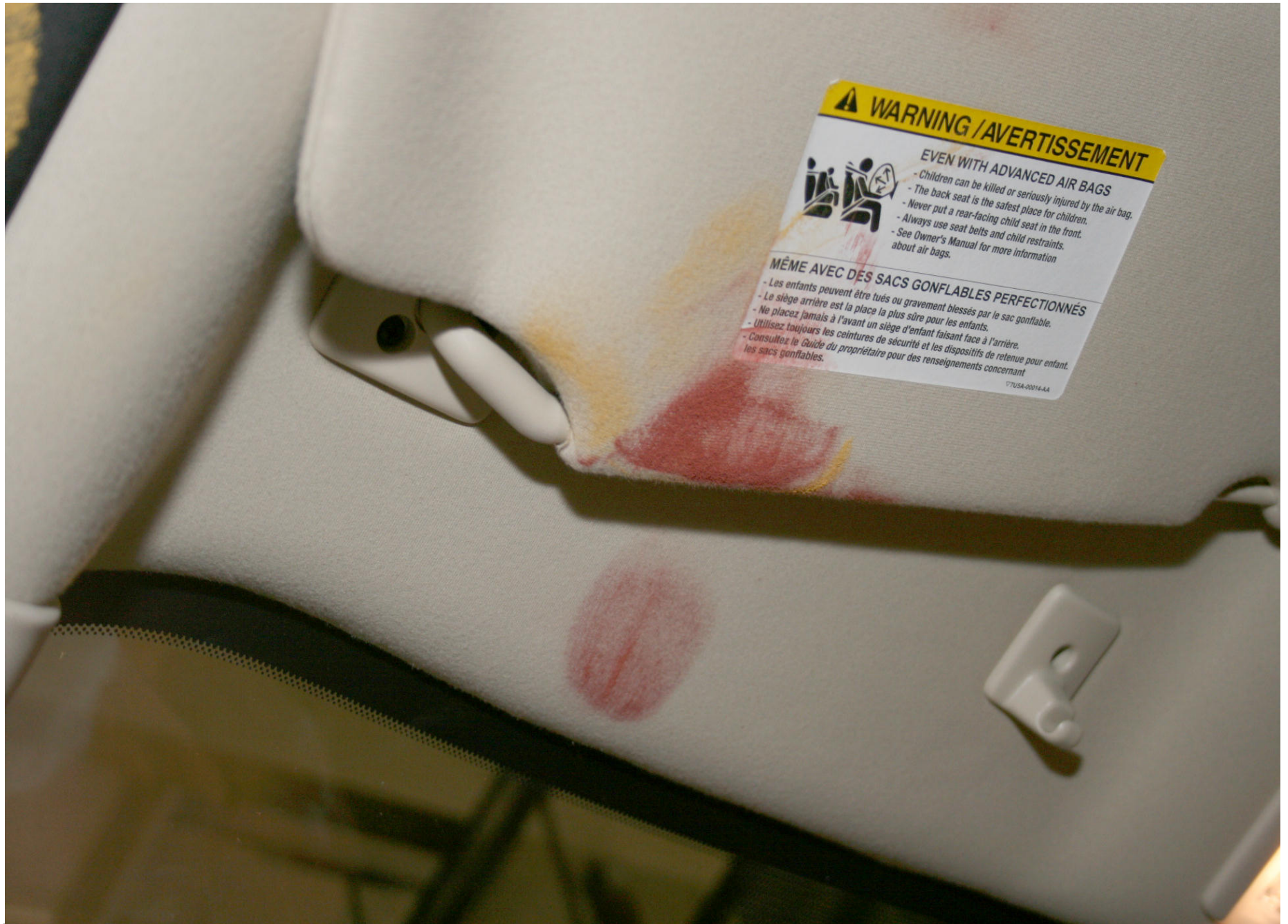
Post-Test Driver Dummy Head Contact (header and visor)
