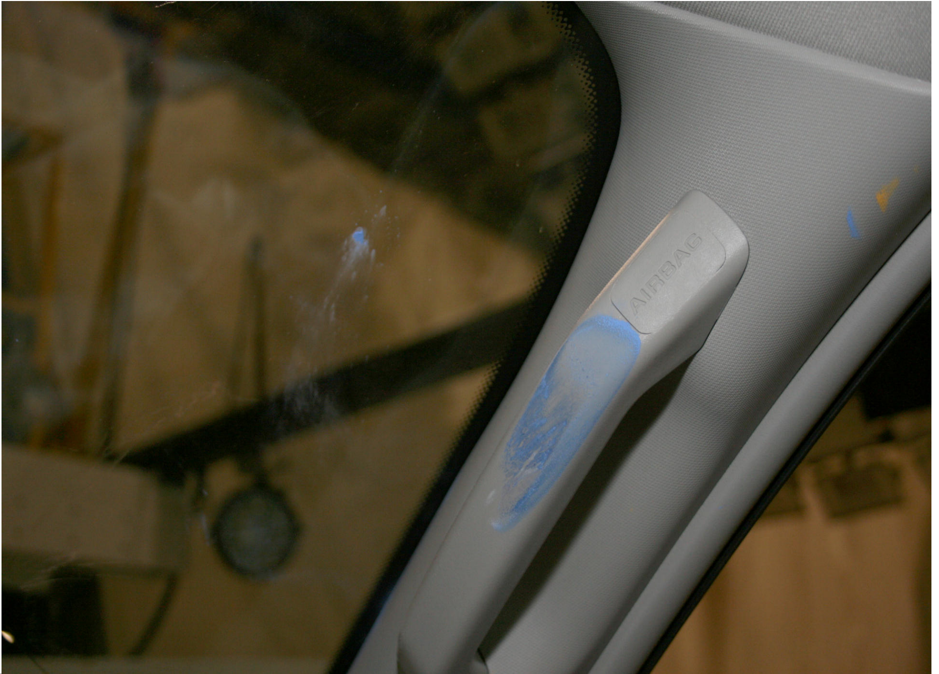
Post-Test Passenger Dummy Head Contact View (C-pillar)
