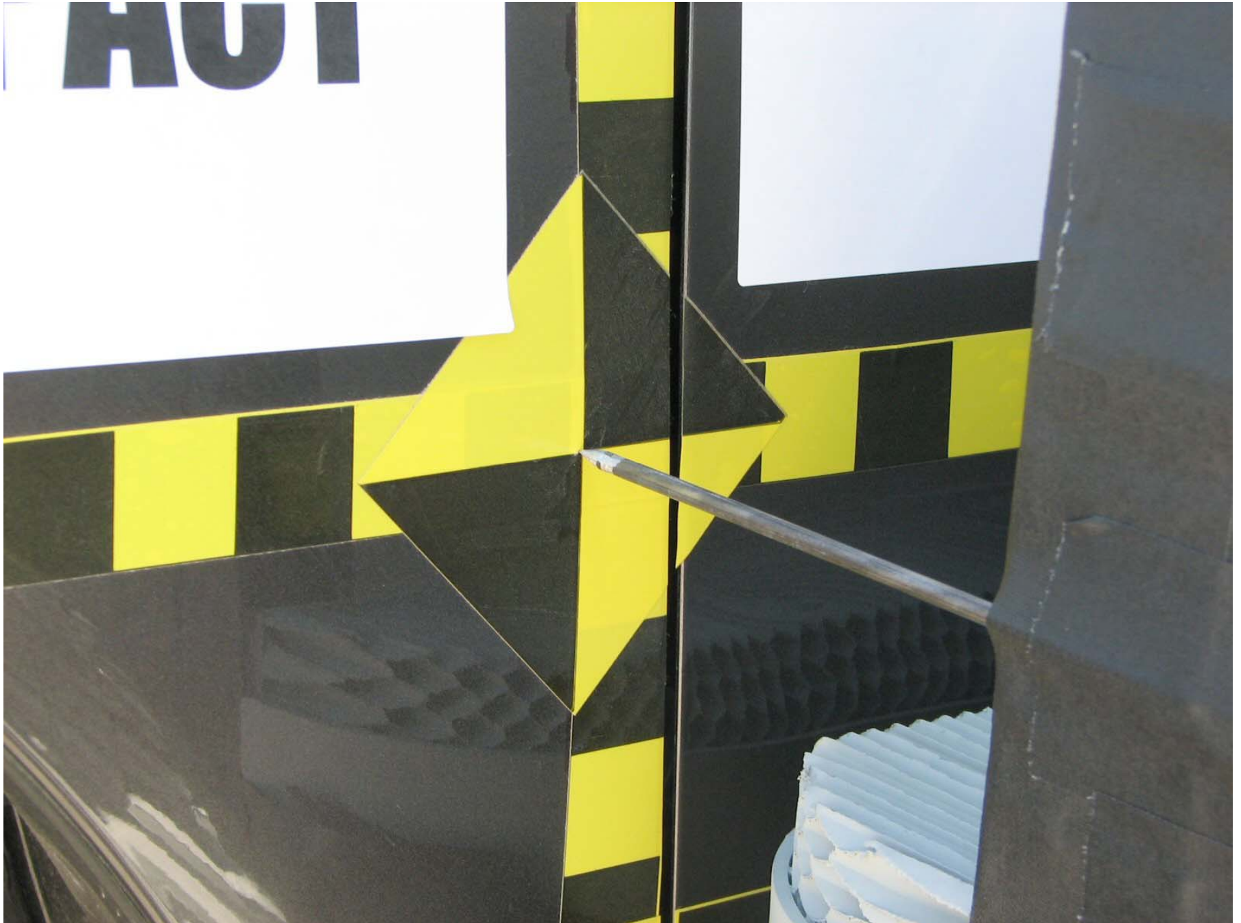
Figure A-25: Pre-Test Left Impact Point
