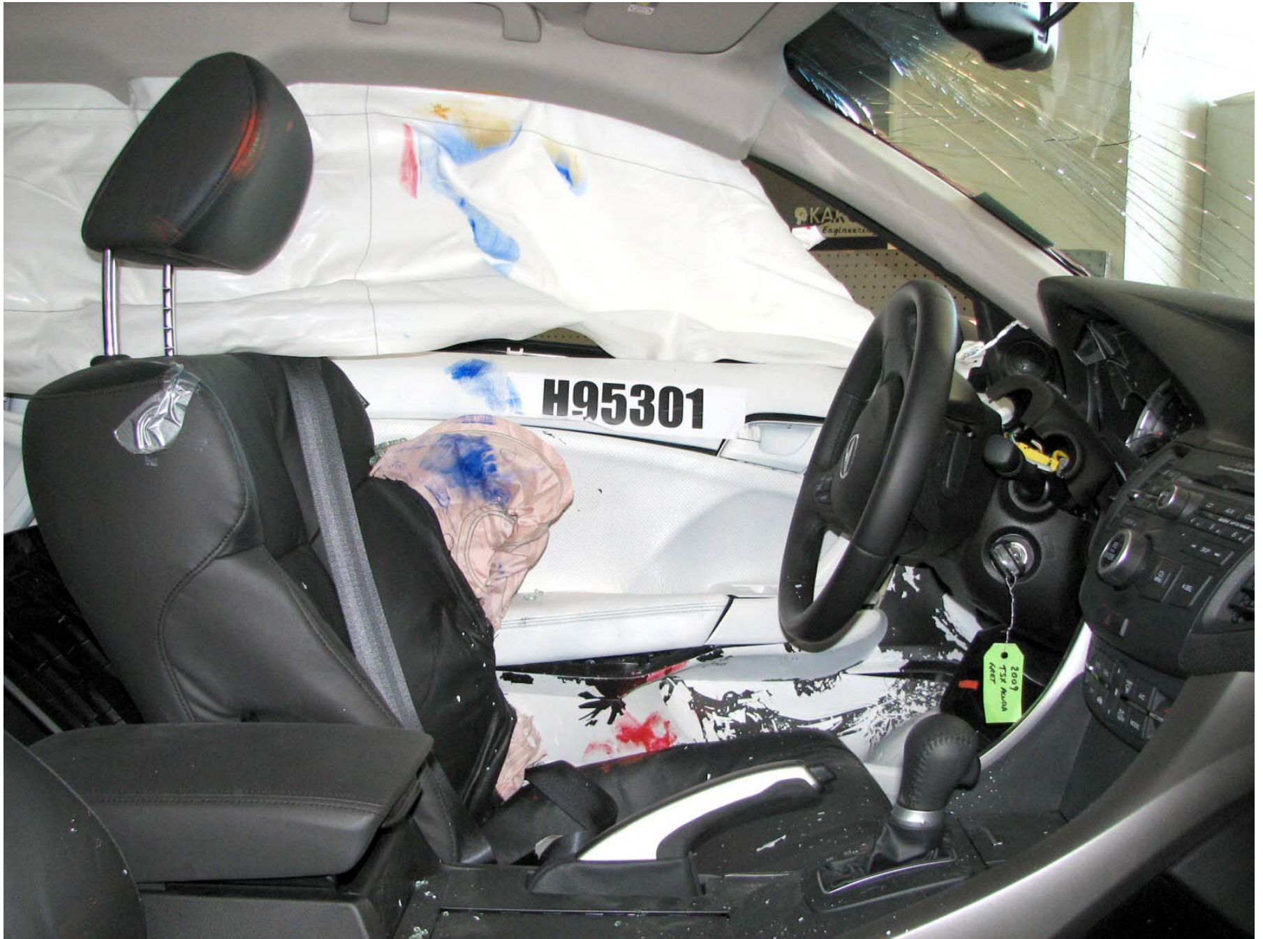
Figure A-43: Post-Test Front Door Panel (Interior)
