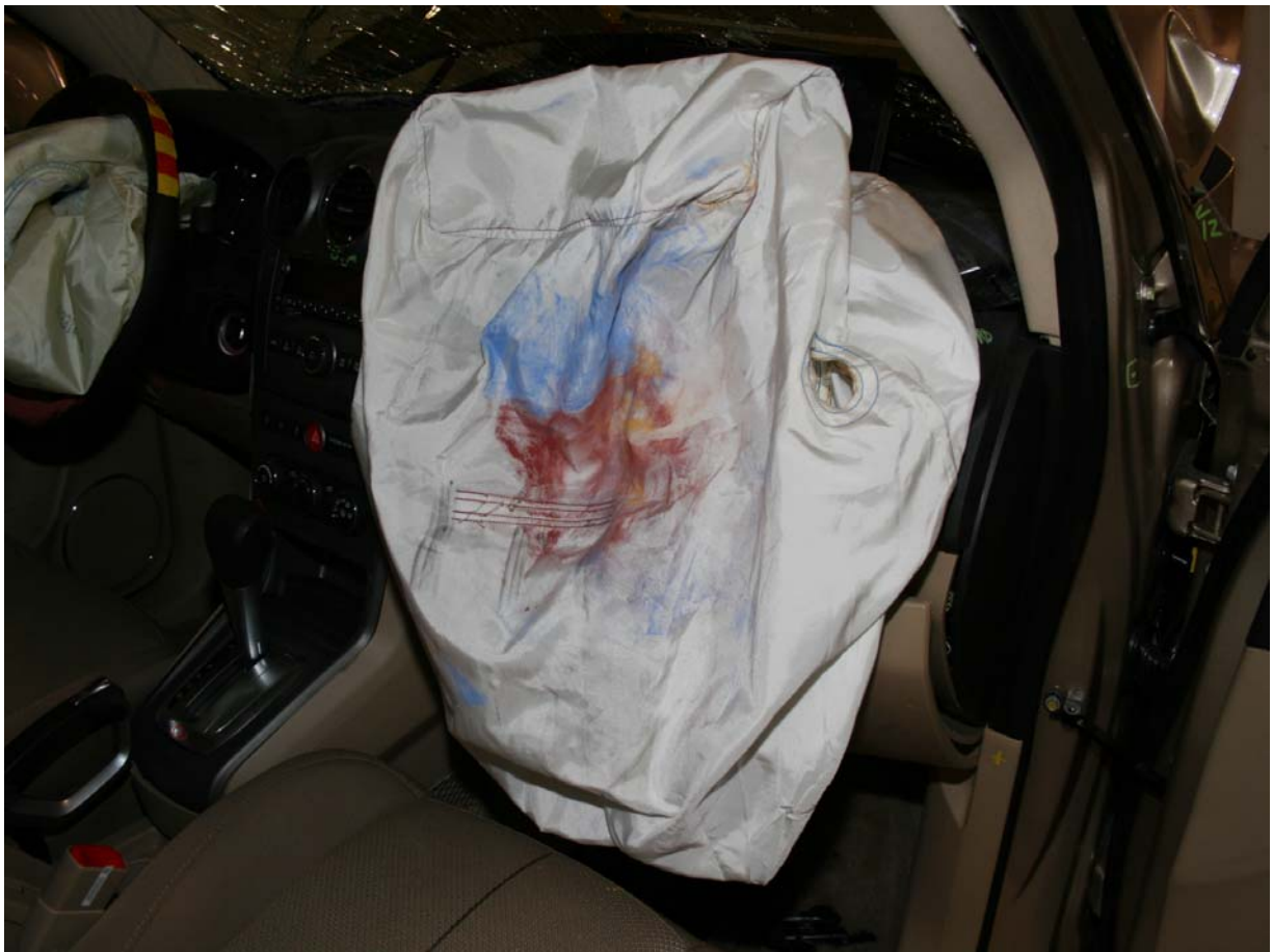
Post-Test Passenger Dummy Airbag Contact
