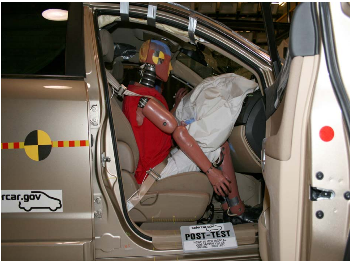
Post-Test Passenger Dummy (Door Open)
