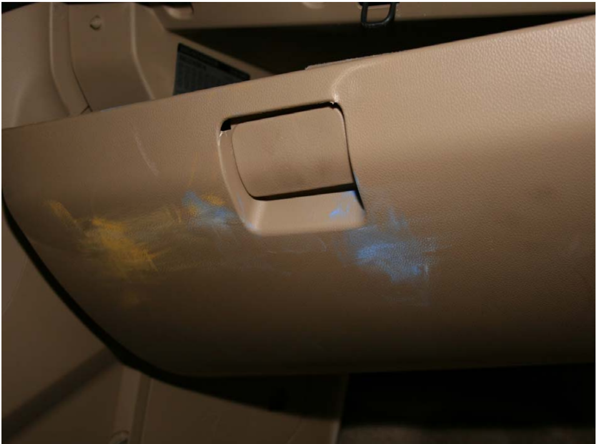
Post-Test Passenger Dummy Knee Contact
