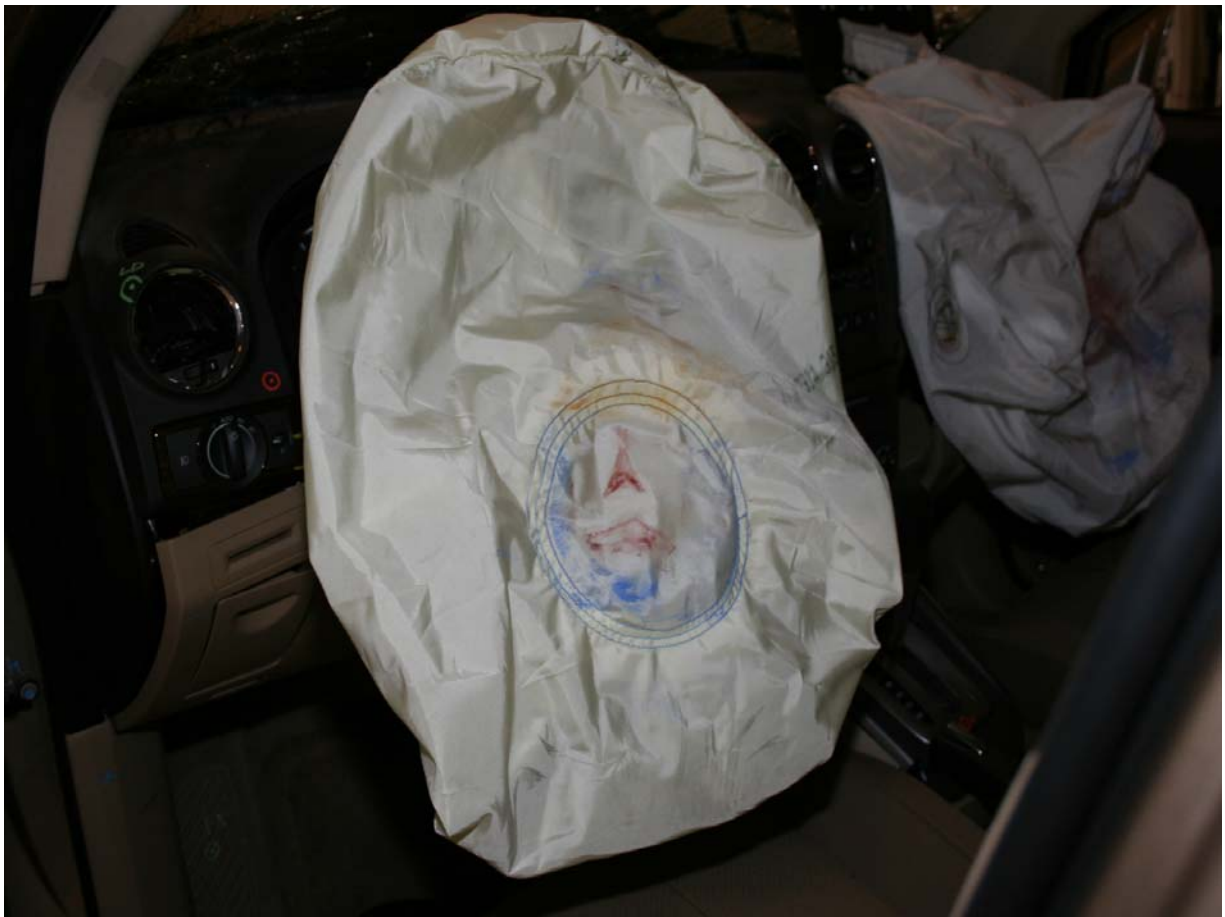
Post-Test Driver Dummy Airbag Contact
