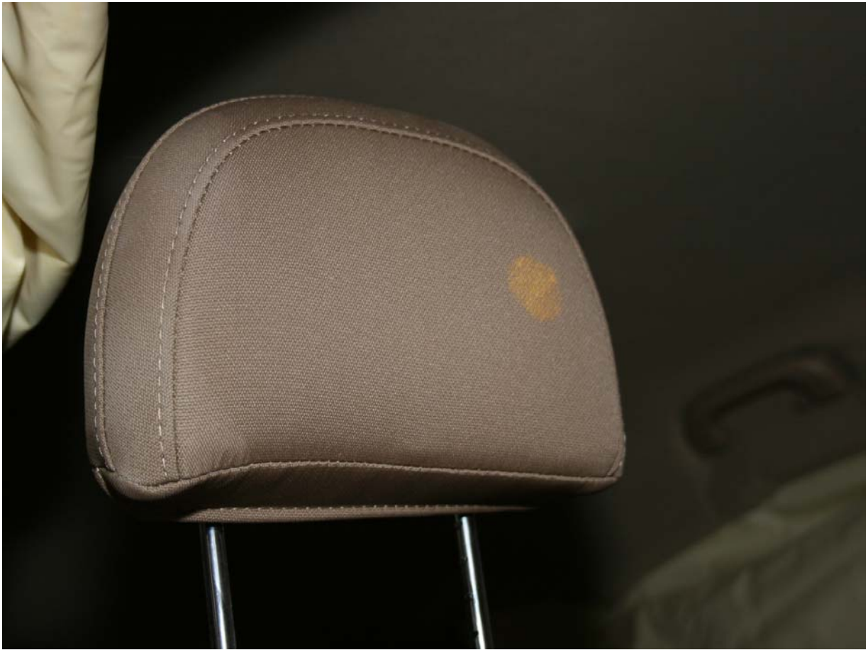
Post-Test Passenger Dummy Head Contact (Headrest)
