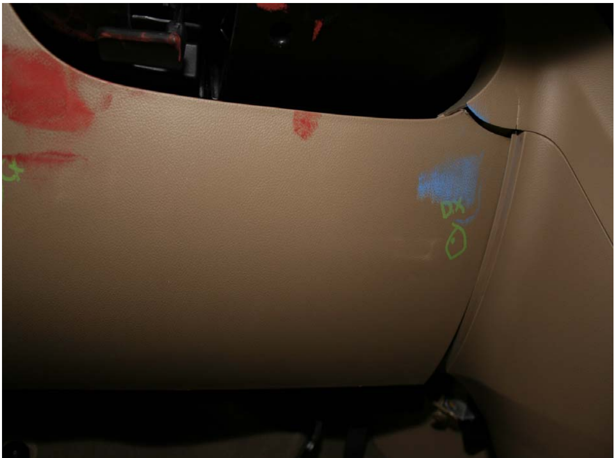
Post-Test Driver Dummy Knee Contact
