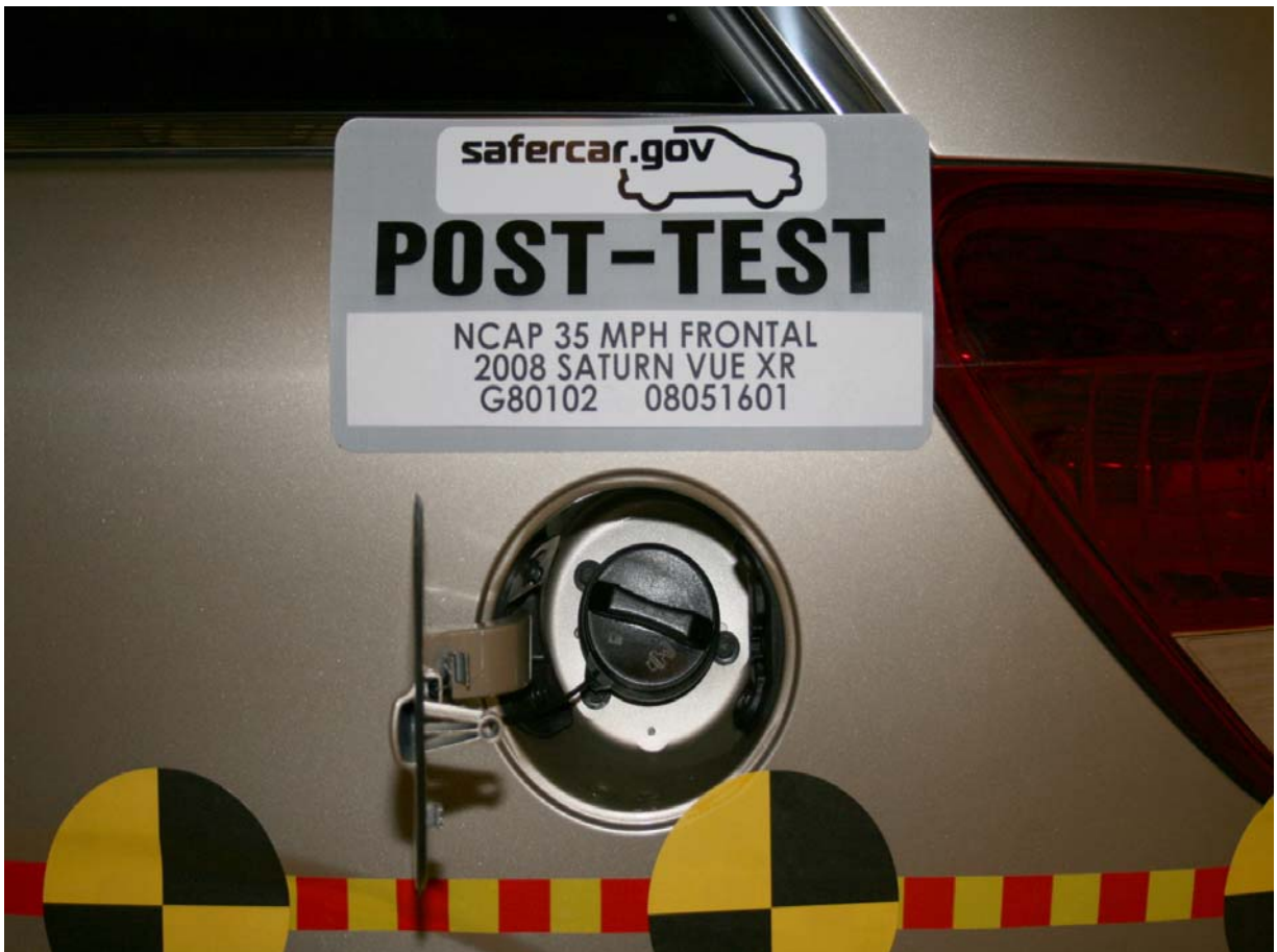
Post-Test Fuel Cap View
