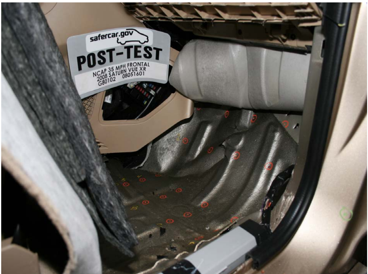
Post-Test Passenger Side Floor Pan
