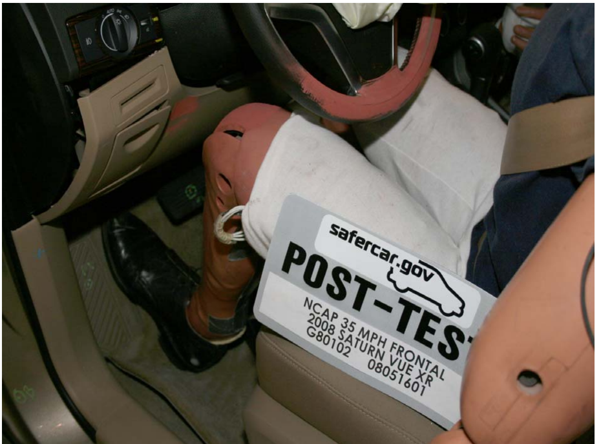
Post-Test Driver Side Knee Bolster
