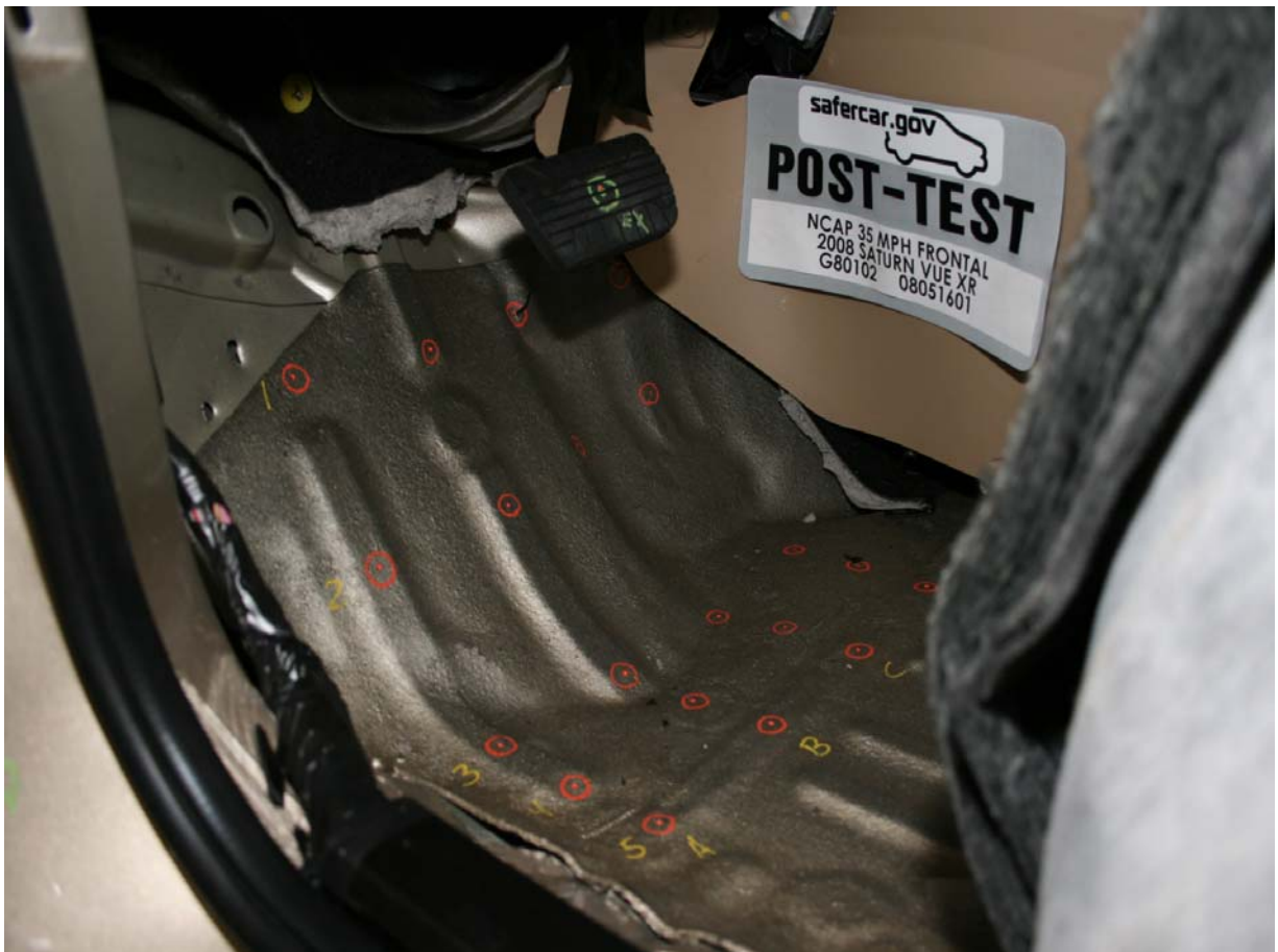
Post-Test Driver Side Floor Pan
