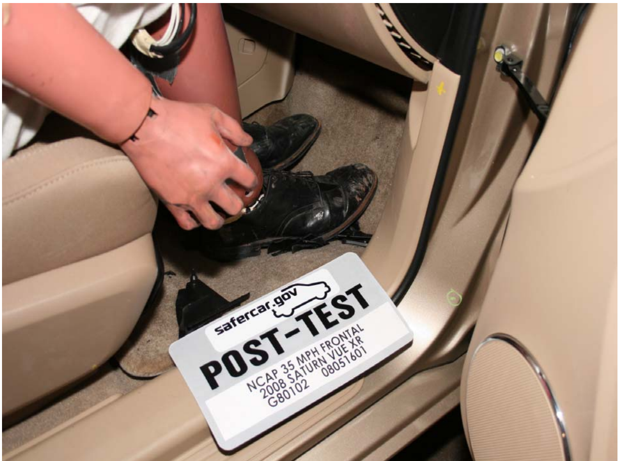
Post-Test Passenger Dummy Feet
