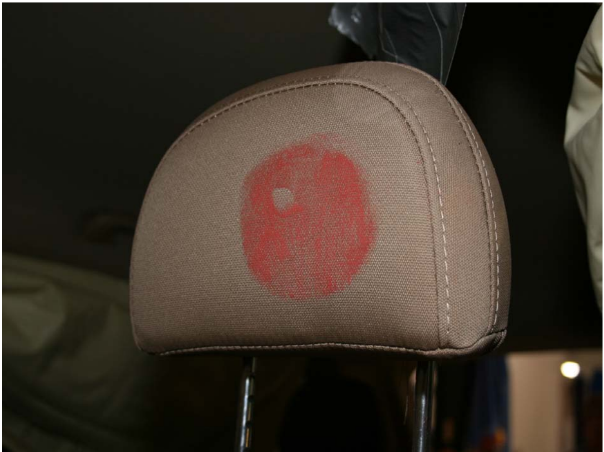
Post-Test Driver Dummy Head Contact (Headrest)
