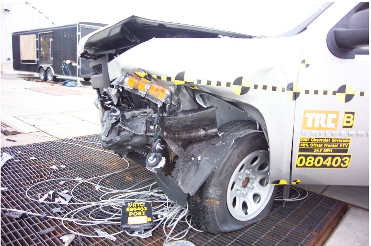
Figure A-8 Post-Test Bullet Vehicle Impact - View 2
