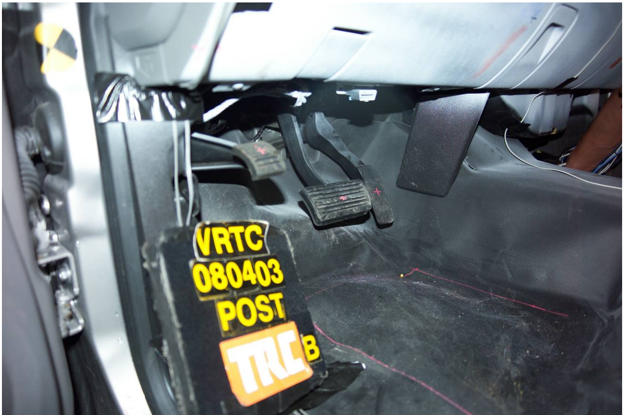
Figure A-131 Post-Test Bullet Vehicle Driver Toeboard Deformation View
