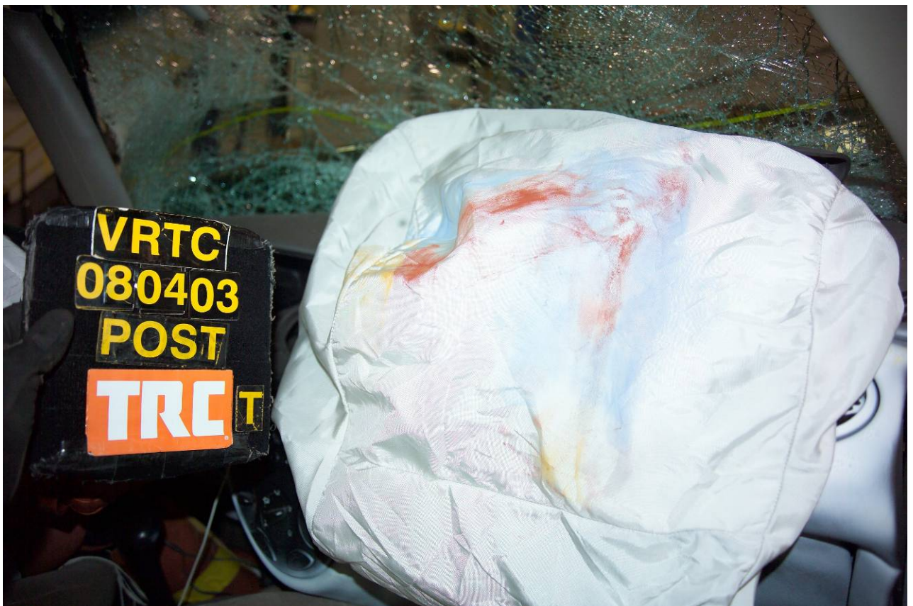
Figure A-121 Post-Test Target Vehicle Passenger Dummy Head Contact - View 1
