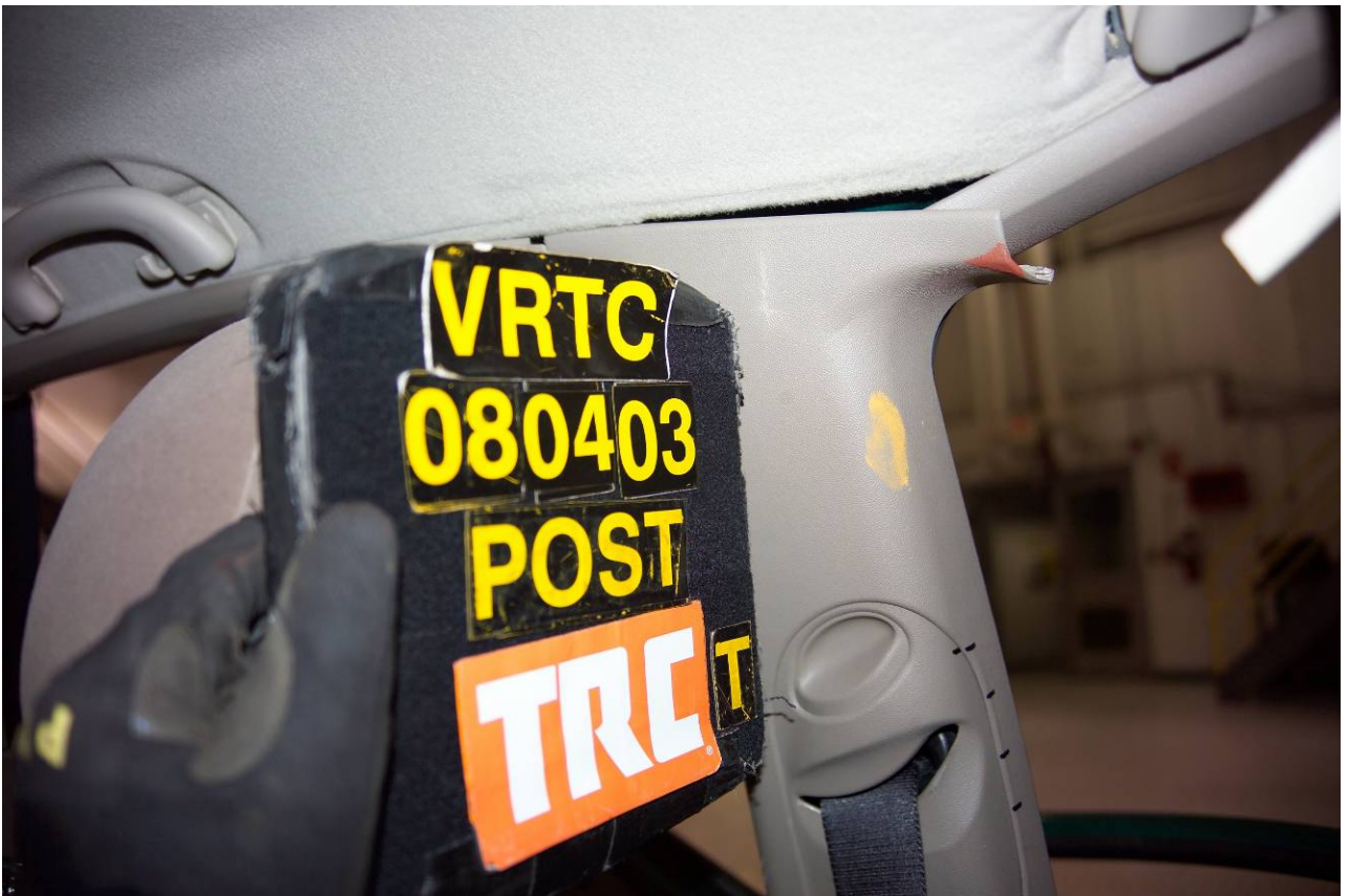
Figure A-117 Post-Test Target Vehicle Driver Dummy Head Contact - View 3
