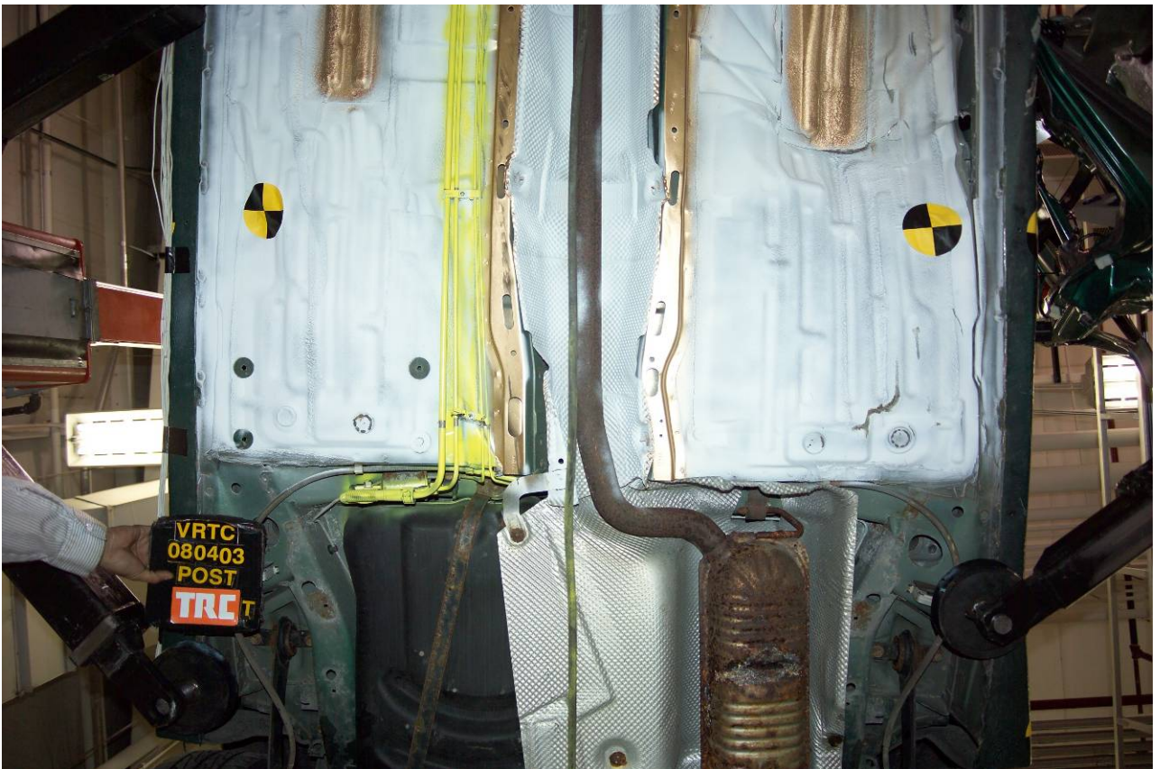
Figure A-39 Post-Test Target Vehicle Mid Underbody View
