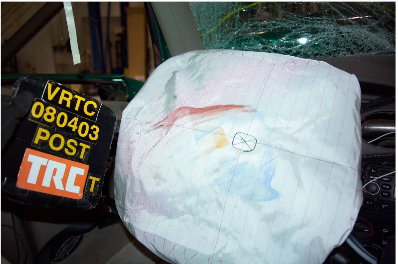
Figure A-115 Post-Test Target Vehicle Driver Dummy Head Contact - View 1
