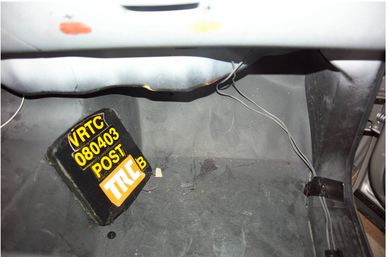
Figure A-137 Post-Test Bullet Vehicle Passenger Toeboard Deformation View
