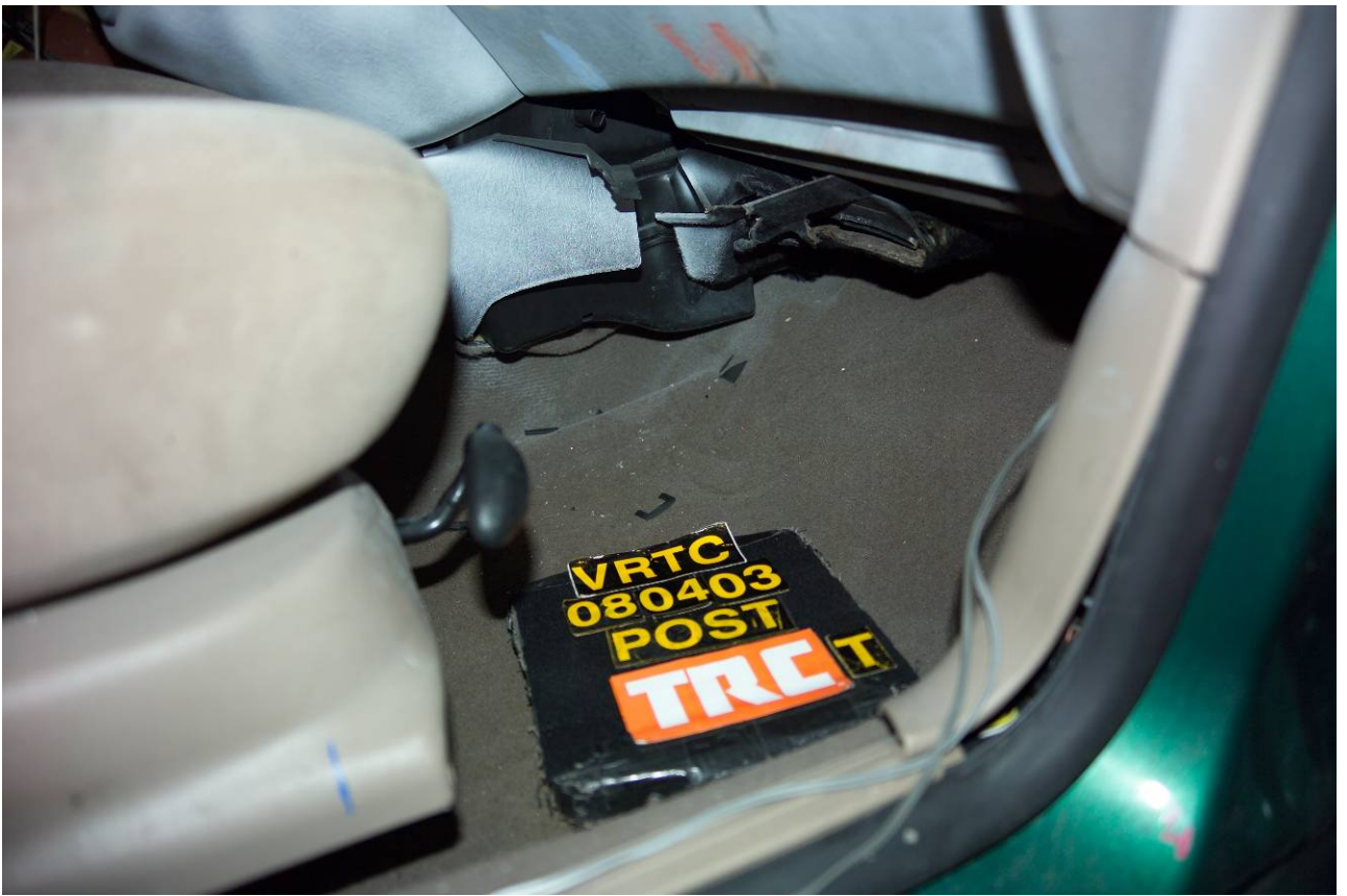
Figure A-124 Post-Test Target Vehicle Passenger Floorboard Deformation View
