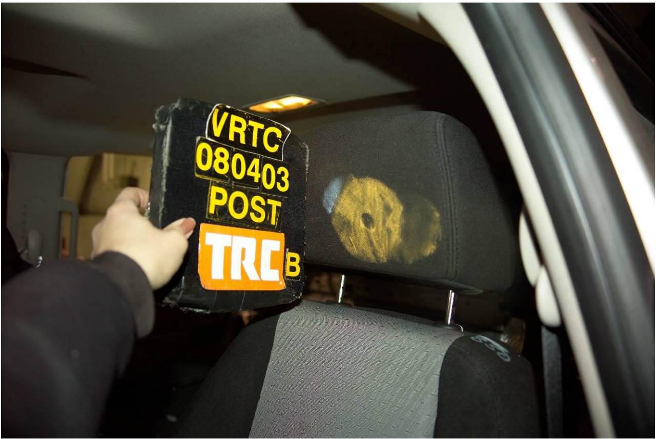
Figure A-128 Post-Test Bullet Vehicle Driver Dummy Head Contact - View 2
