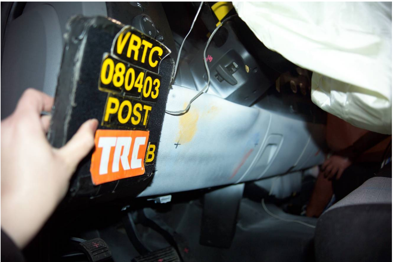
Figure A-129 Post-Test Bullet Vehicle Driver Dummy Knee Contact View
