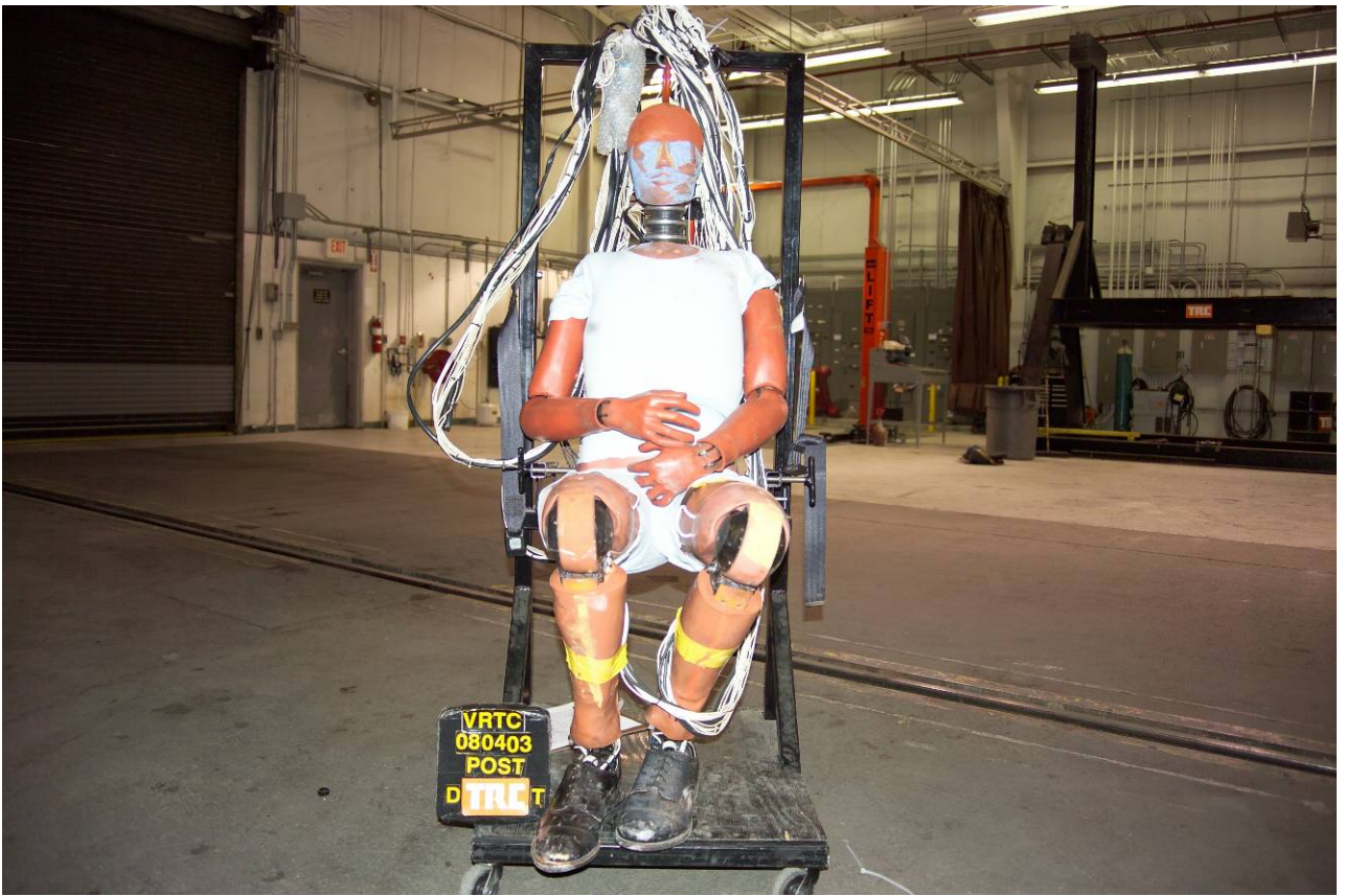
Figure A-114 Post-Test Target Vehicle Driver Dummy Overall Contact View
