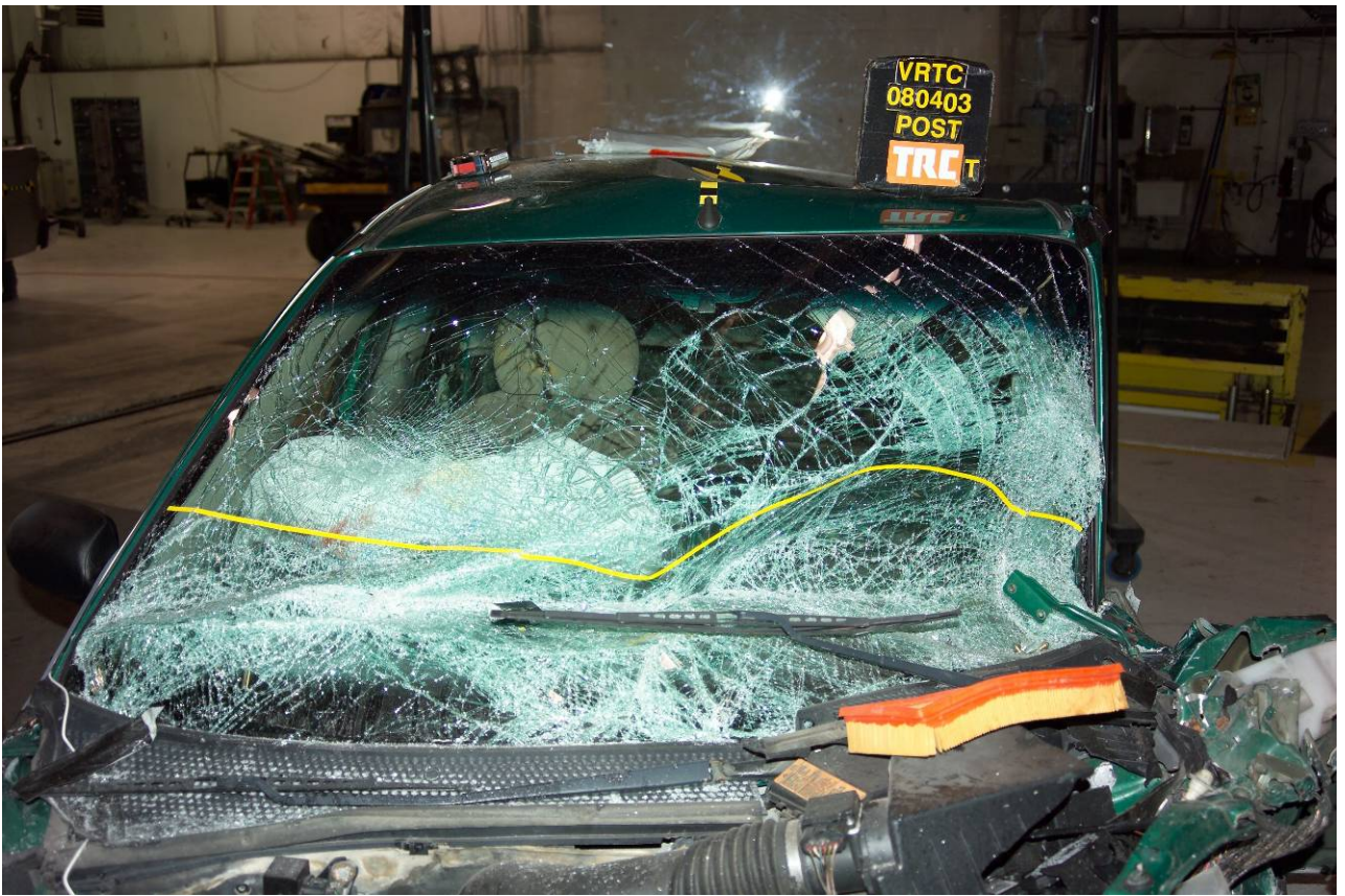
Figure A-141 Post-Test Target Vehicle Windshield Damage Front View
