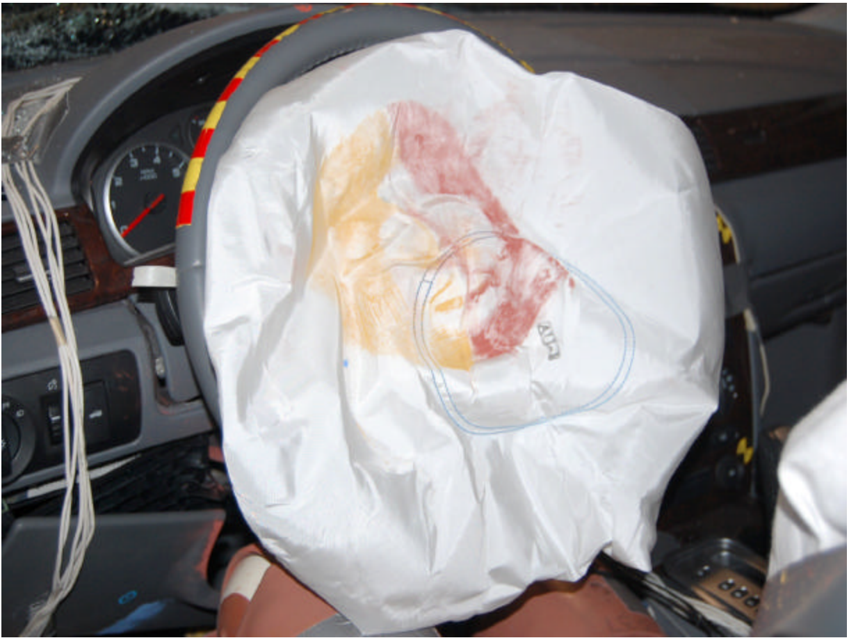
Post-Test Driver Dummy Airbag Contact
