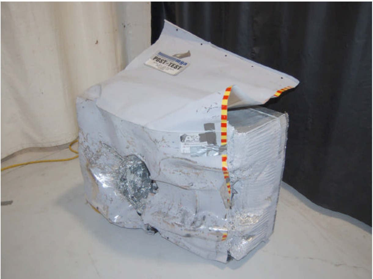
Post-Test Offset Deformable Barrier Right Side \frac{3}{4} View
