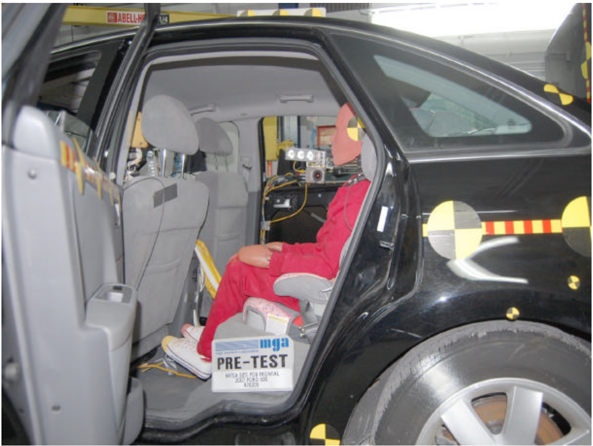
Pre-Test Left Rear Passenger Dummy (Door Open)
