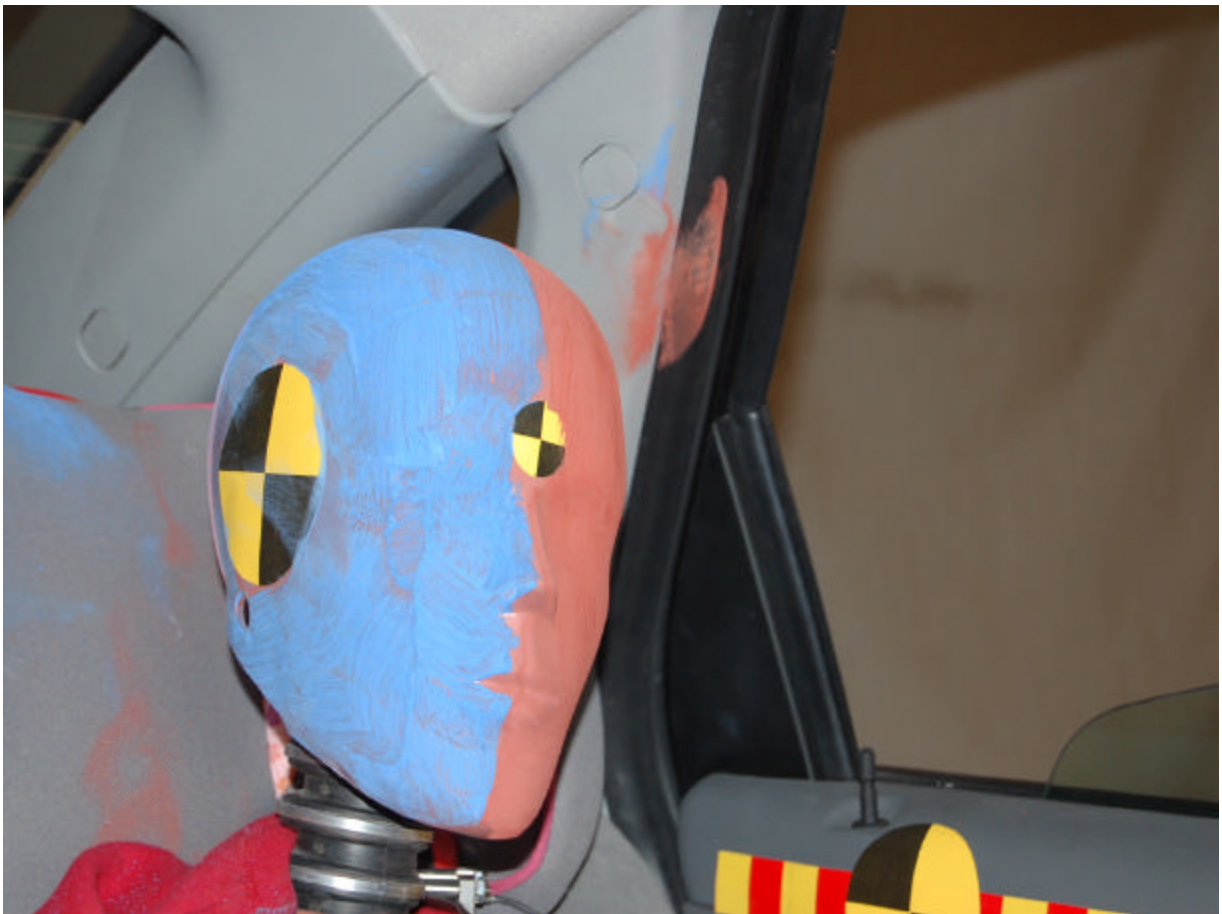
Post-Test Left Rear Passenger Dummy Head Contact View 2
