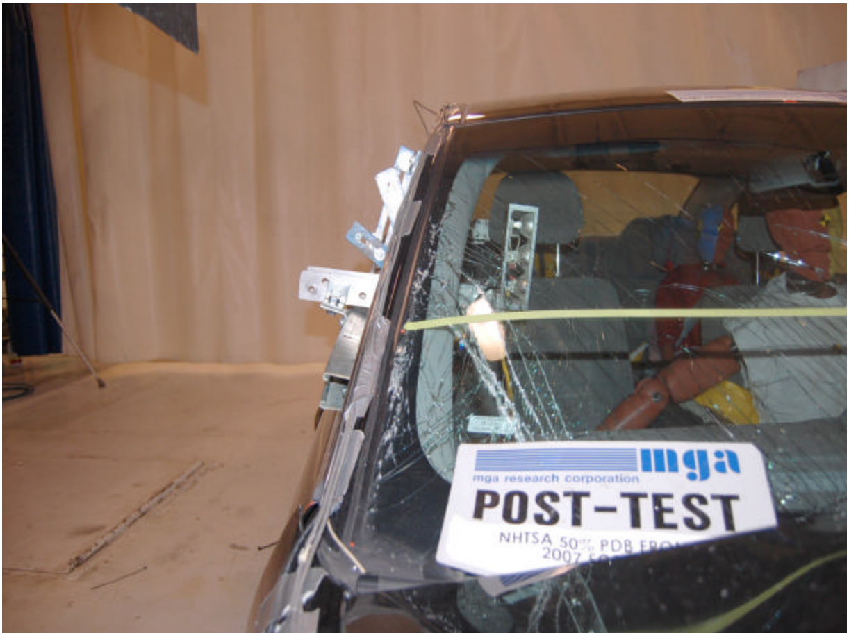
Post-Test Right Side A Pillar (Frontal View)
