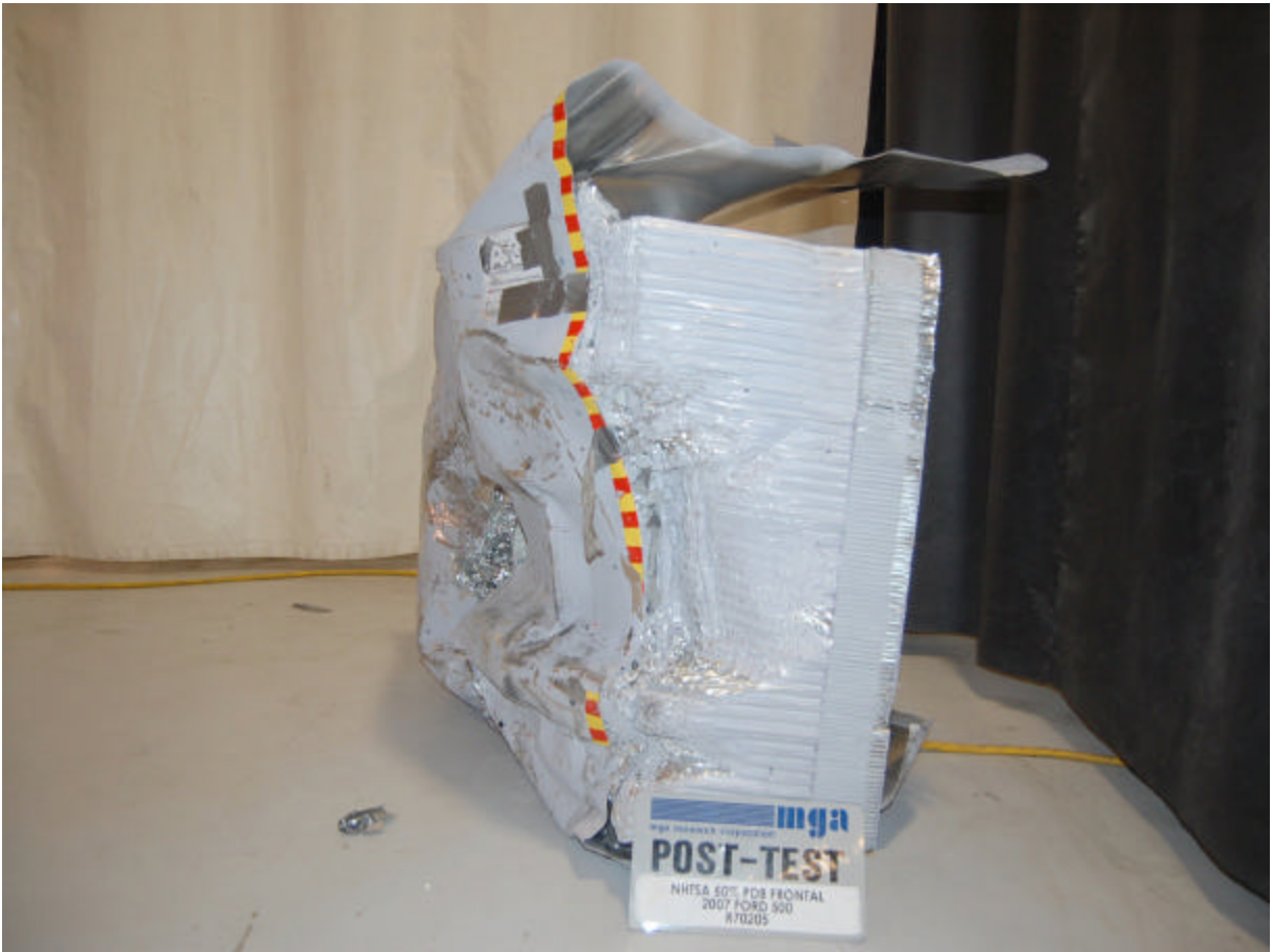
Post-Test Offset Deformable Barrier Right Side View
