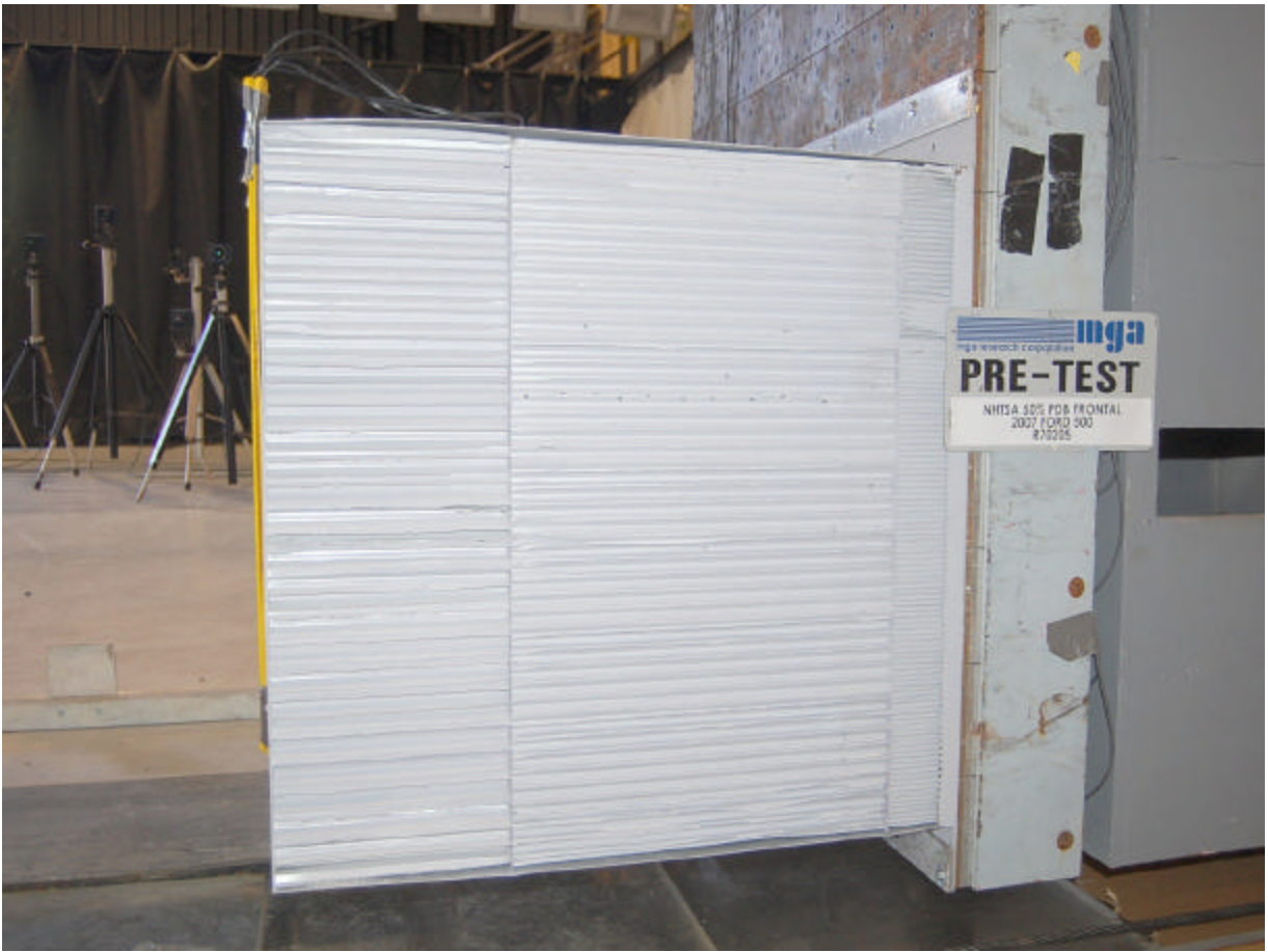
Pre-Test Offset Deformable Barrier Right Side View
