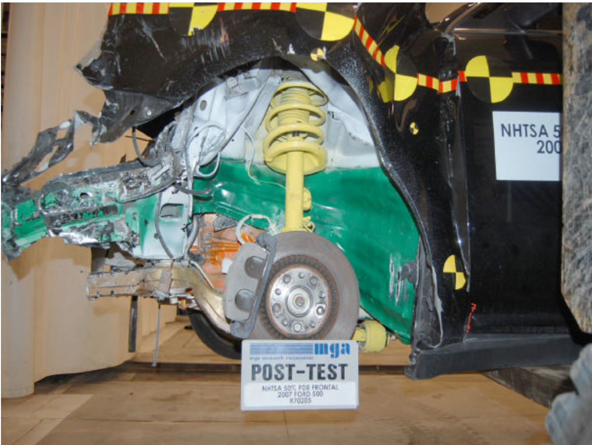
Post-Test Left Front Wheel Well
