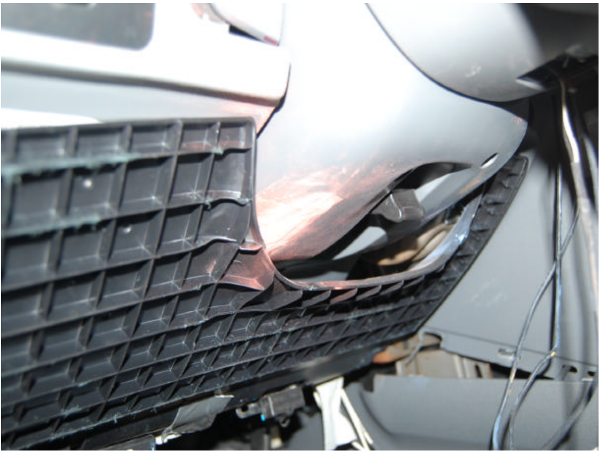
Post-Test Driver Dummy Knee Contact View 1
