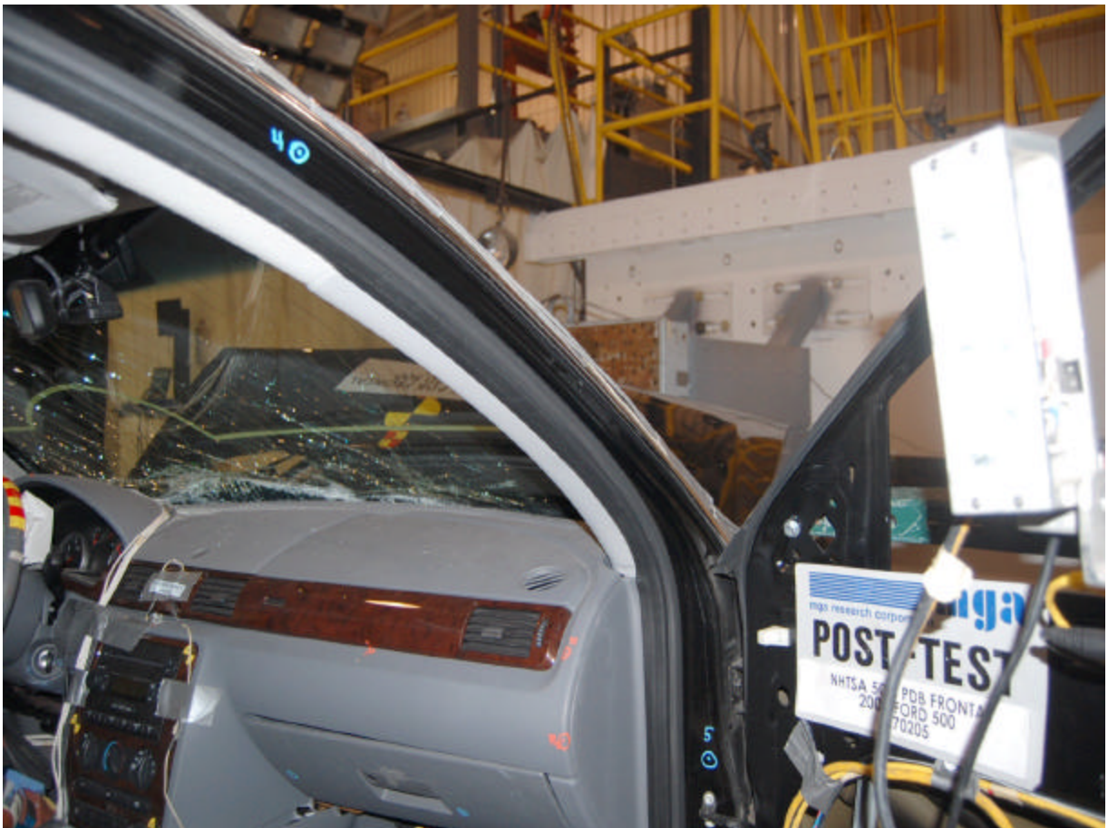
Post-Test Right Side A Pillar (¾ Rear View)
