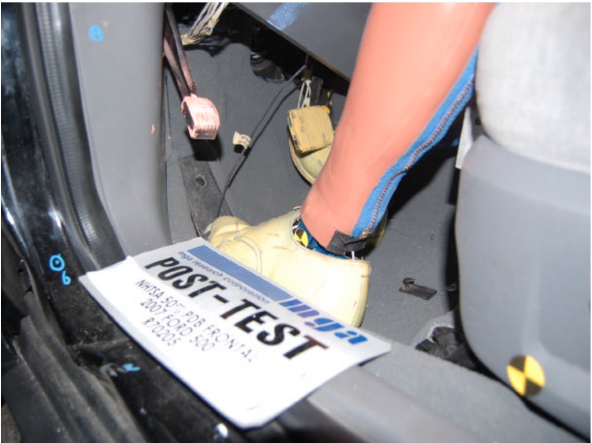
Post-Test Driver Dummy Foot/Leg Close-Up
