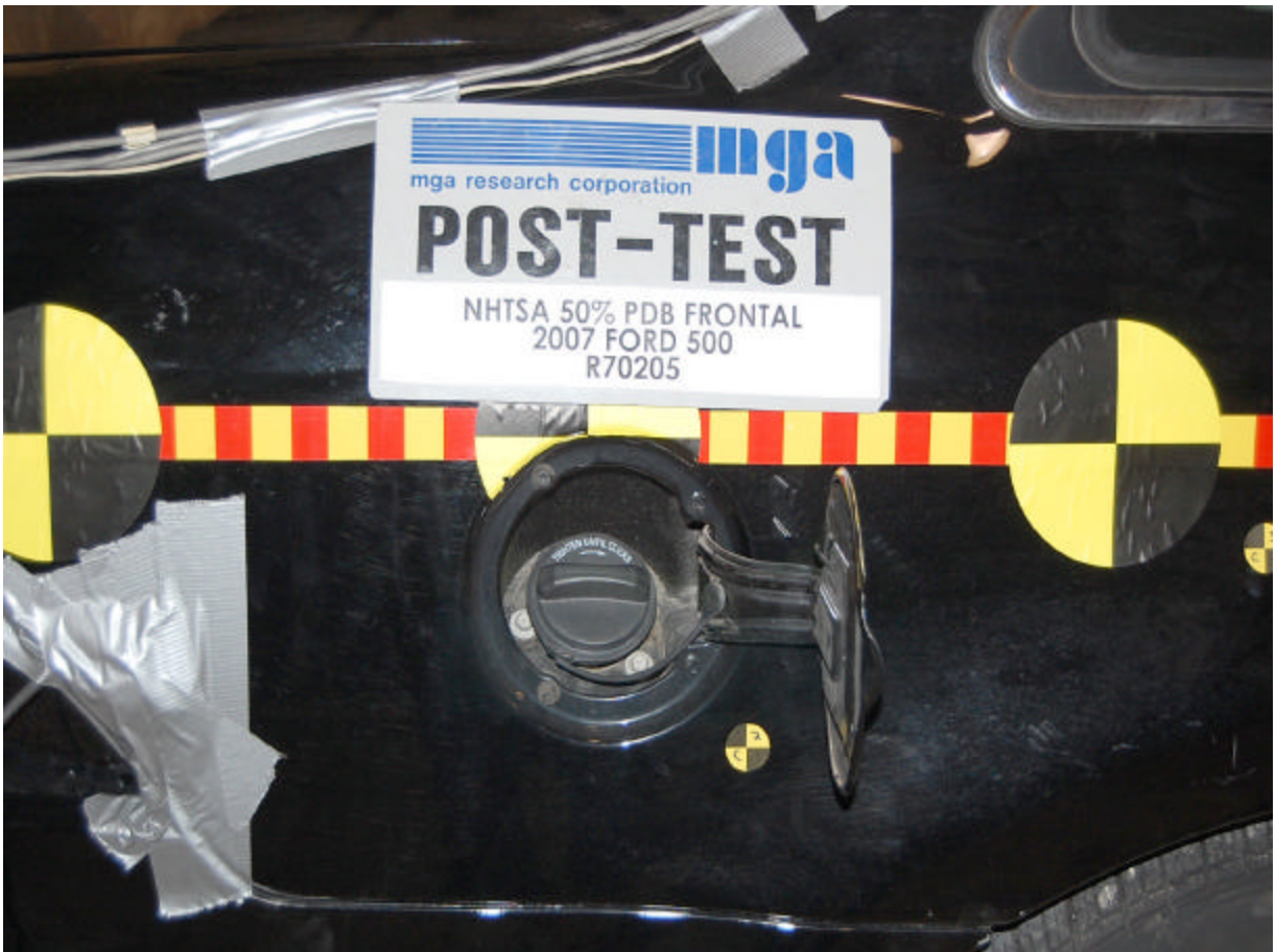
Post-Test Fuel Cap View
