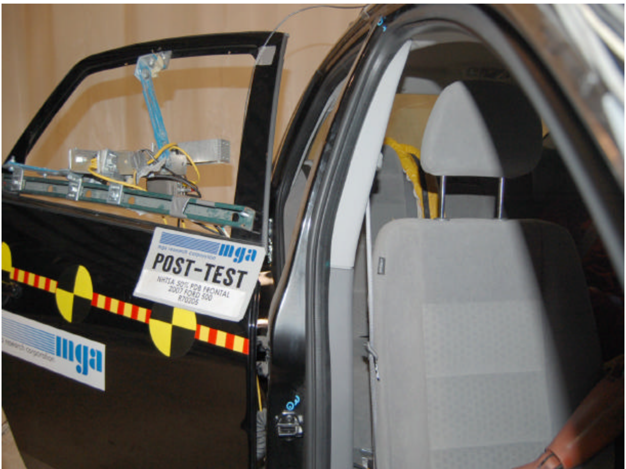
Post-Test Right Side B Pillar (¾ Front View)
