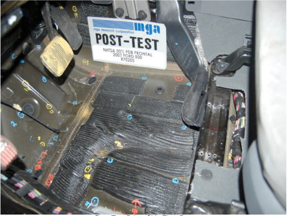
Post-Test Driver Side Floor Pan
