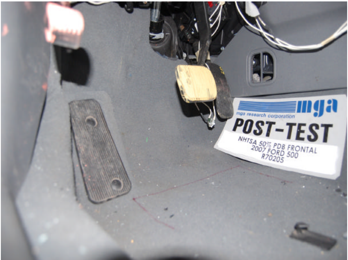
Post-Test Over Toepan/Floorpan Left of Seat, Sill Height
