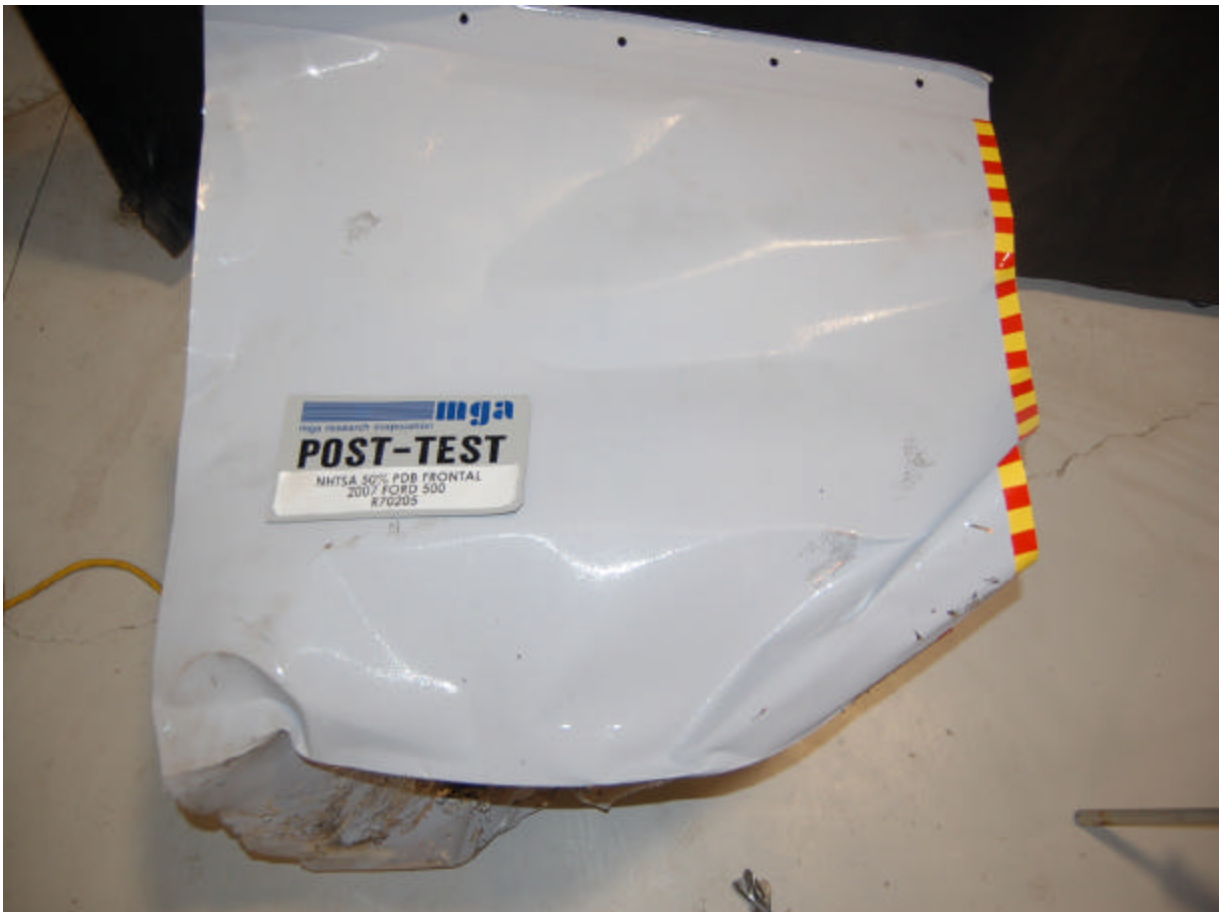
Post-Test Offset Deformable Barrier Overhead View
