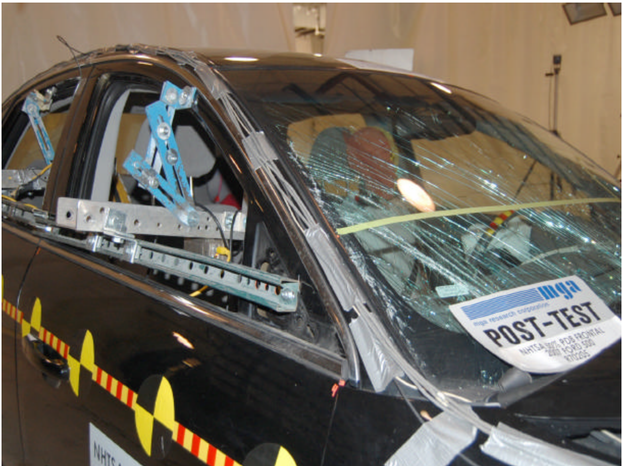
Post-Test Right Side A Pillar (¾ Front View)
