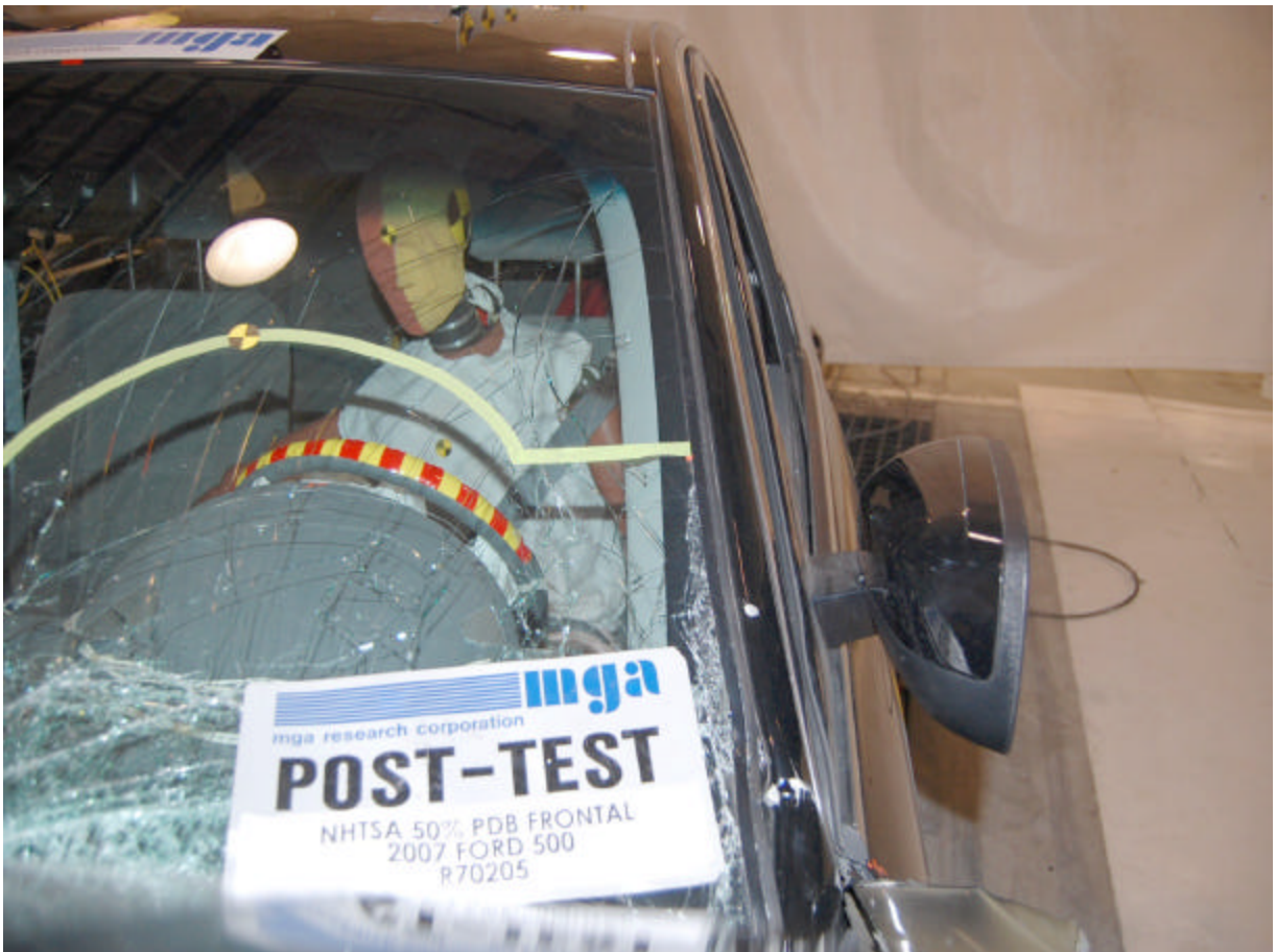
Post-Test Left Side A Pillar (Frontal View)
