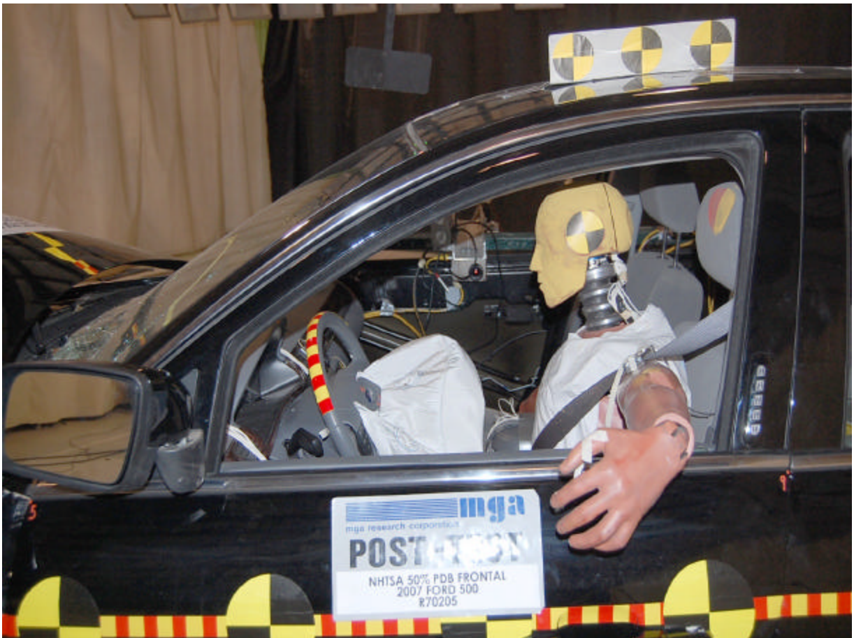
Post-Test Driver Dummy (Through Window)
