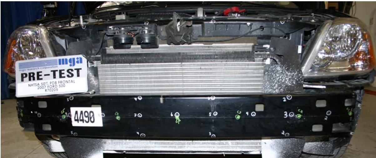
Lower Bumper Beam / Upper Bumper Beam / Center Bumper Beam / Upper Radiator Support
