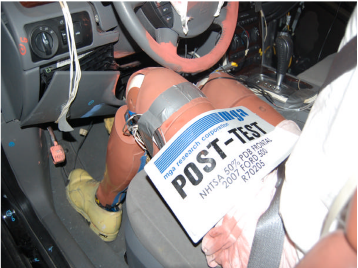
Post-Test Driver Side Knee Bolster
