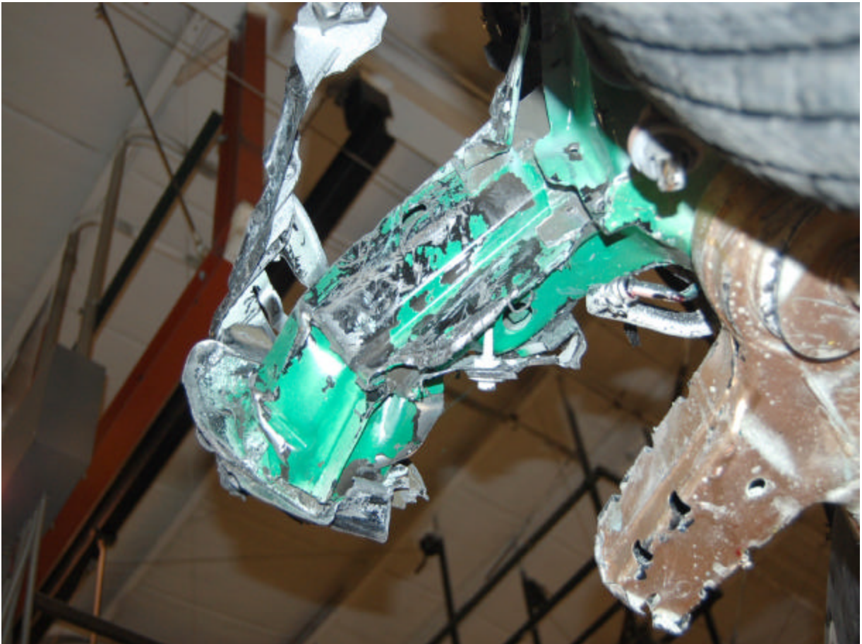
Post-Test Left Bumper to Rail Attachment View
