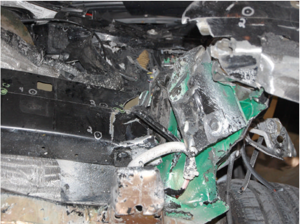
Post-Test Right Bumper to Rail Attachment View
