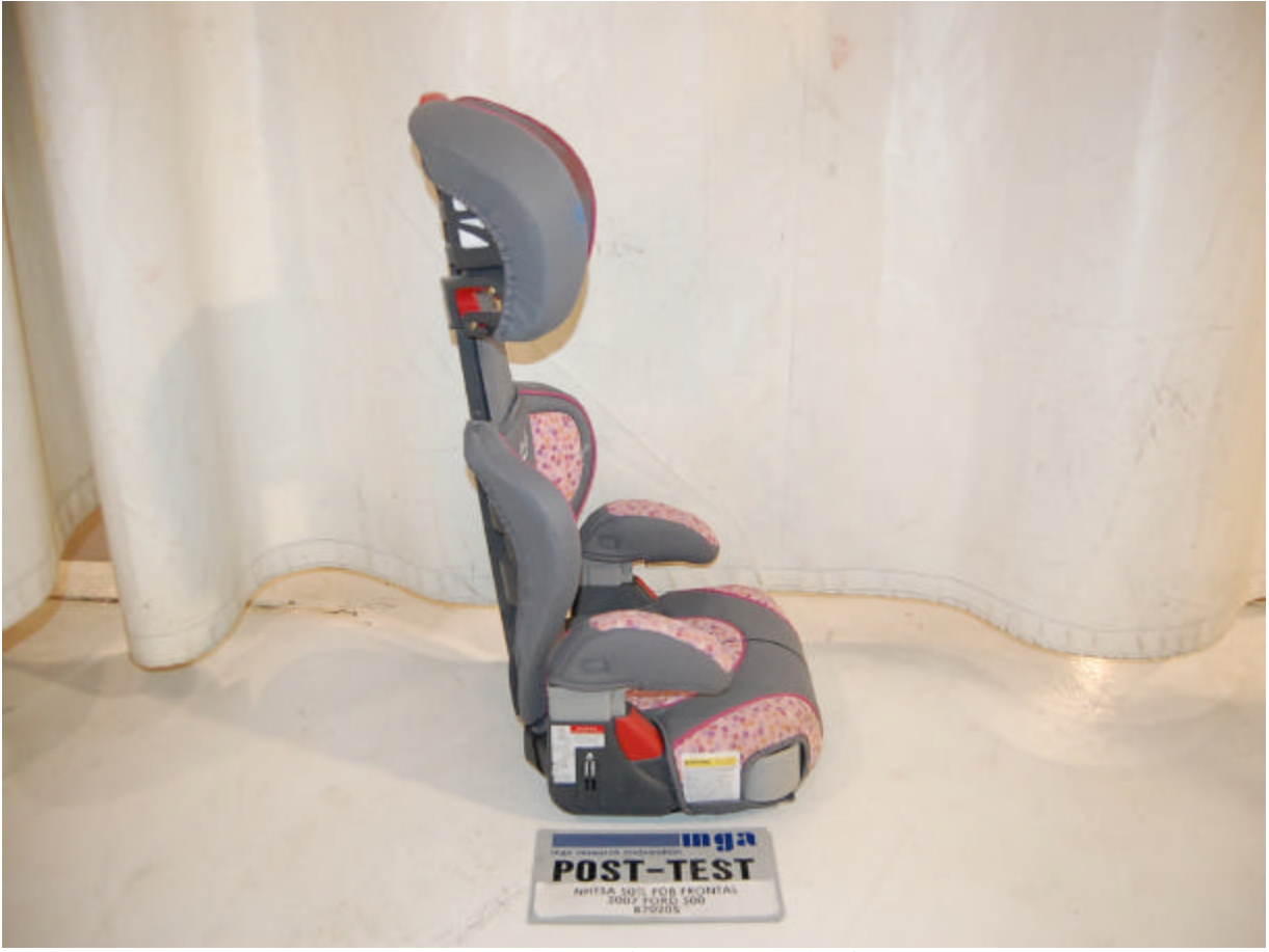
Post-Test Right Side View of CRS
