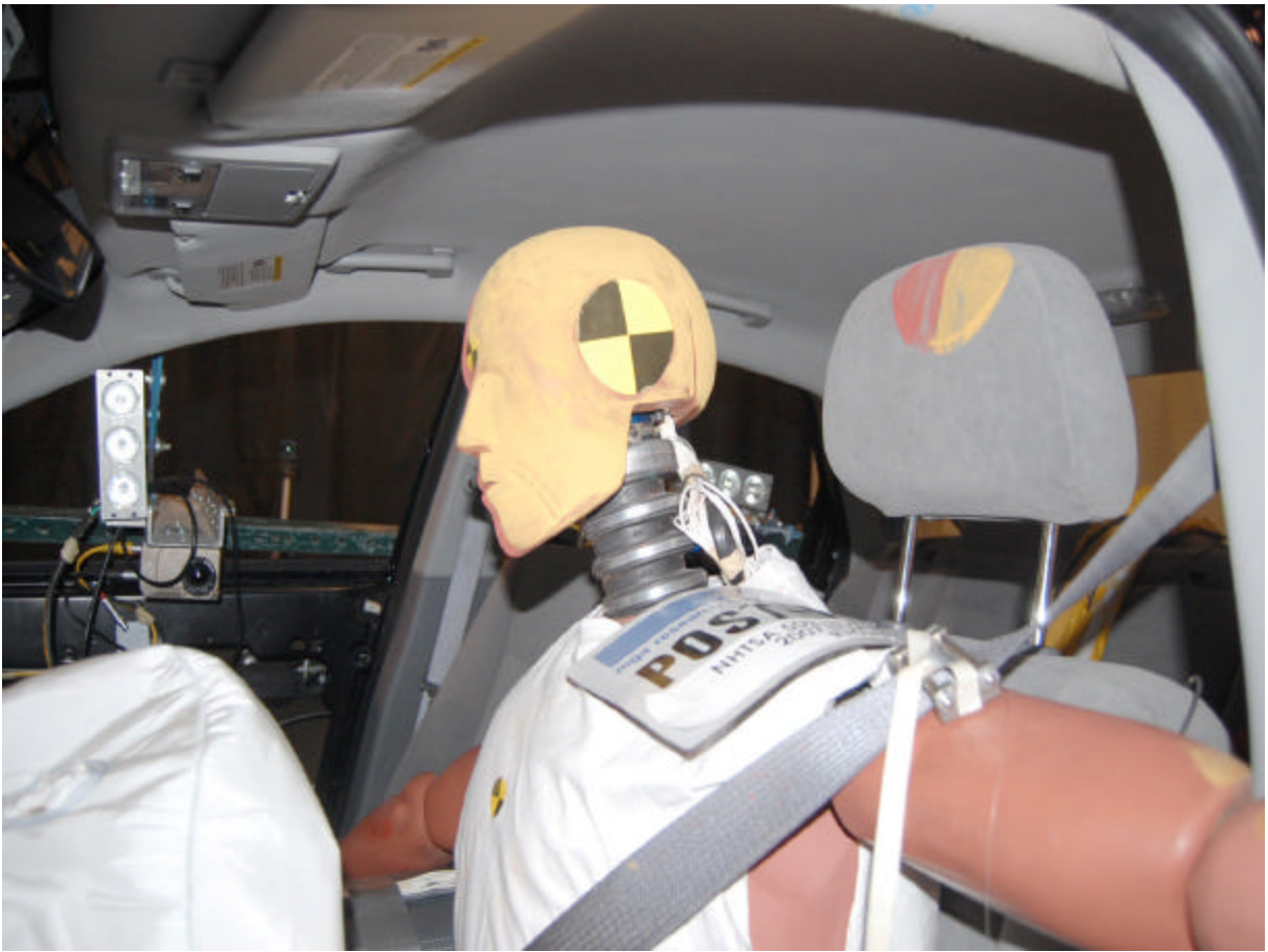
Post-Test Driver Dummy Head Contact (headrest)
