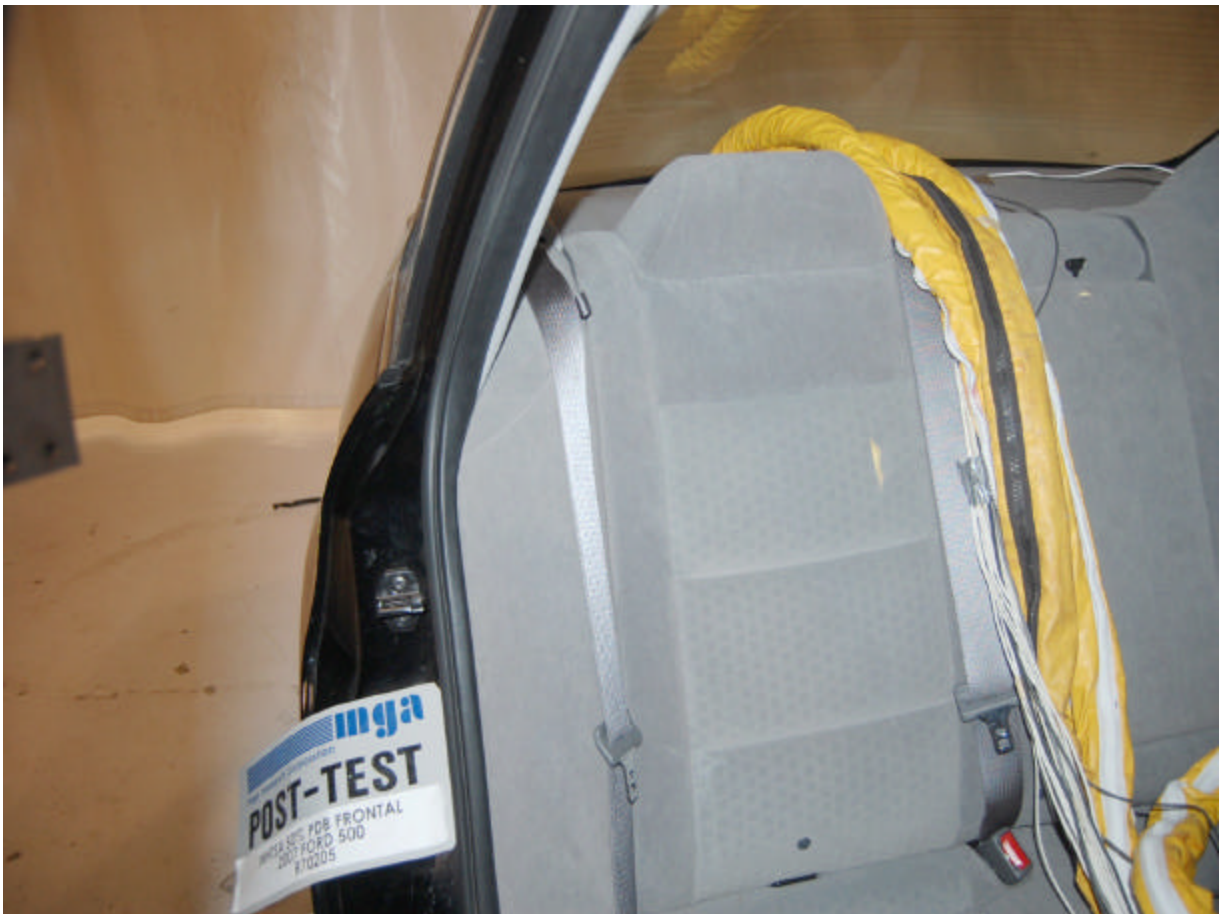
Post-Test Right Side C Pillar (Frontal View)
