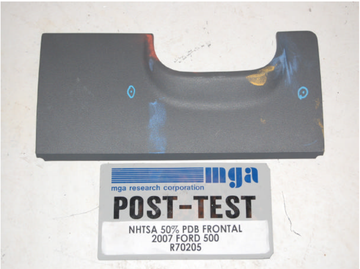
Post-Test Driver Dummy Knee Contact View 2
