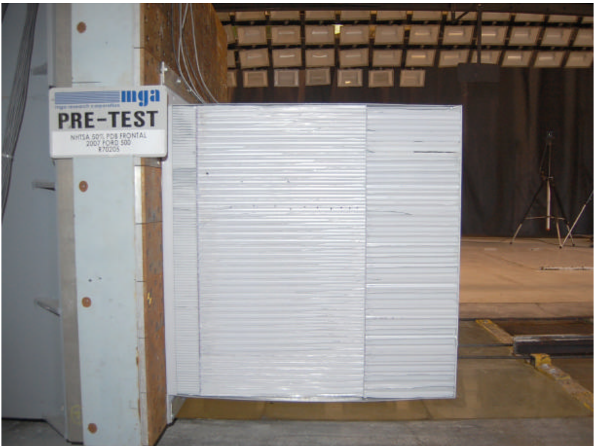
Pre-Test Offset Deformable Barrier Left Side View
