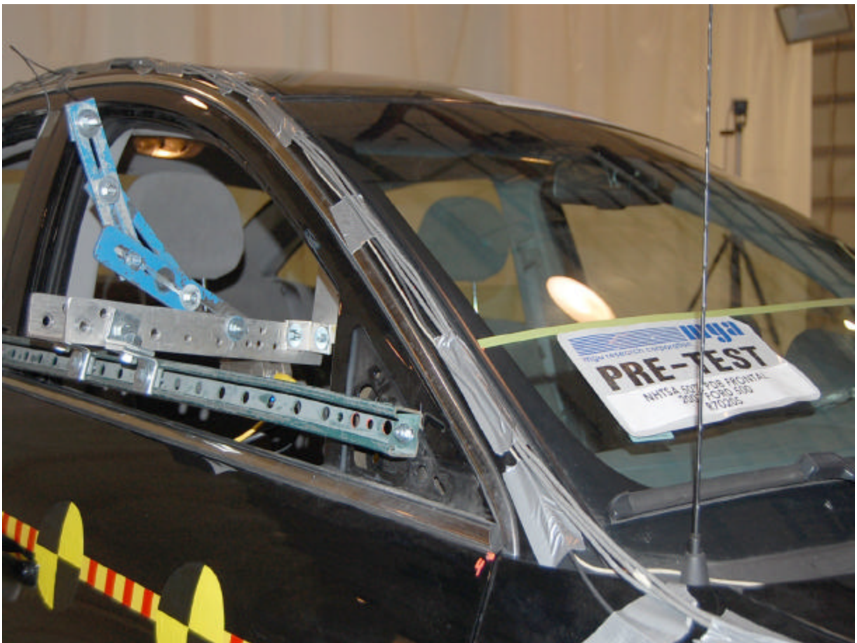
Pre-Test Right Side A Pillar (¾ Front View)
