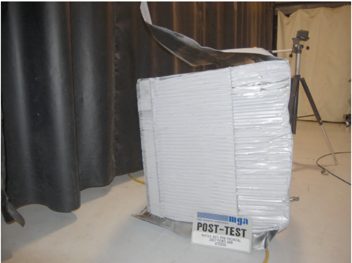
Post-Test Offset Deformable Barrier Left Side View
