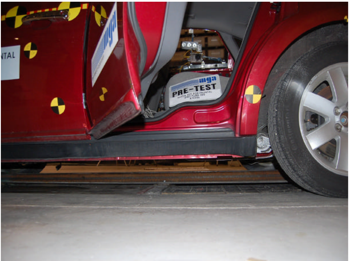
Pre-Test Left Side Sill Rear Half View
