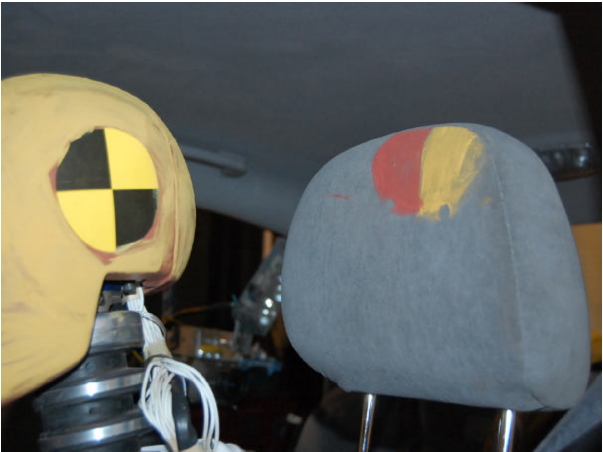
Post-Test Driver Dummy Head Contact (headrest)
