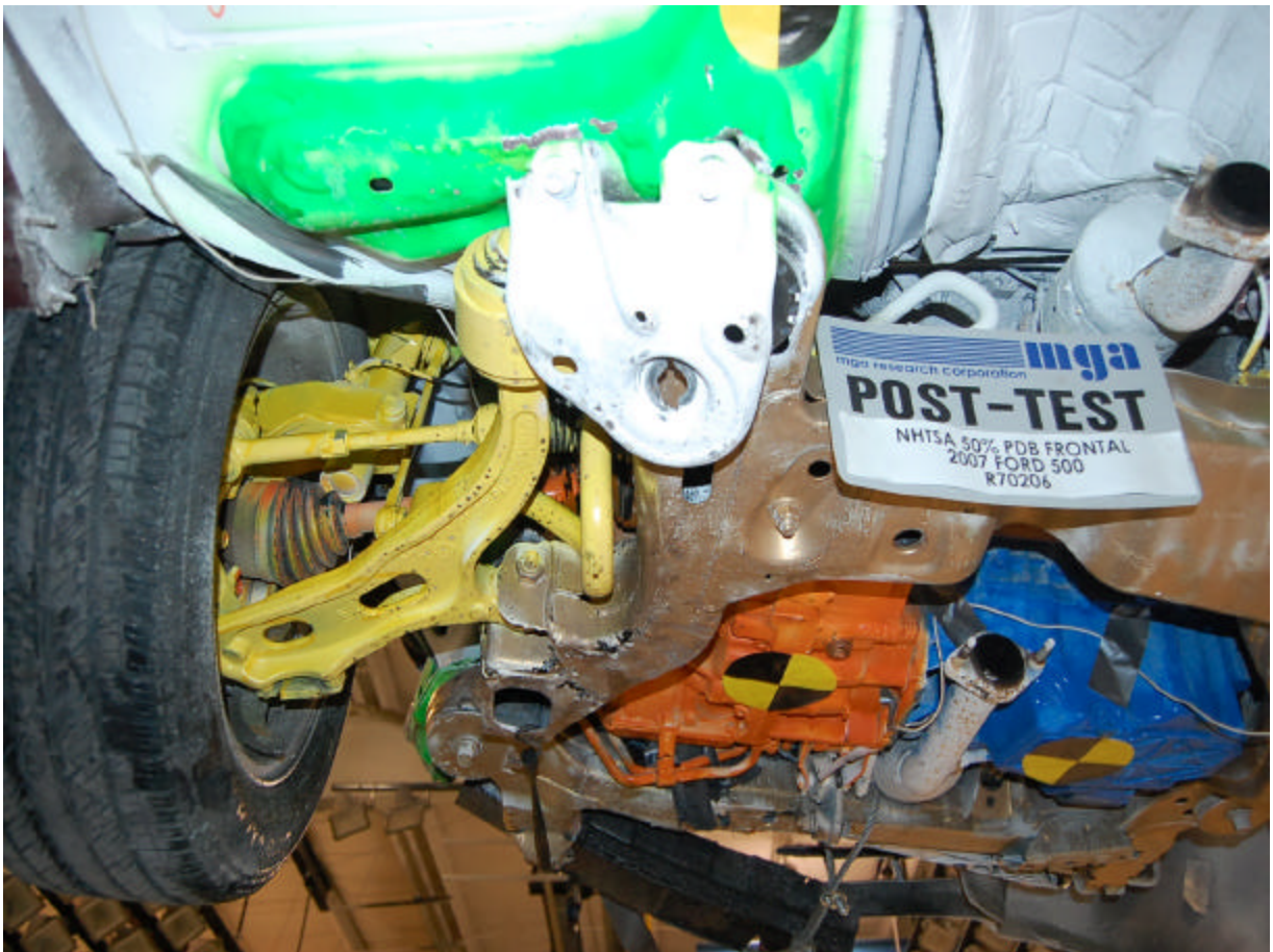
Post-Test Sway Bar Left Side View
