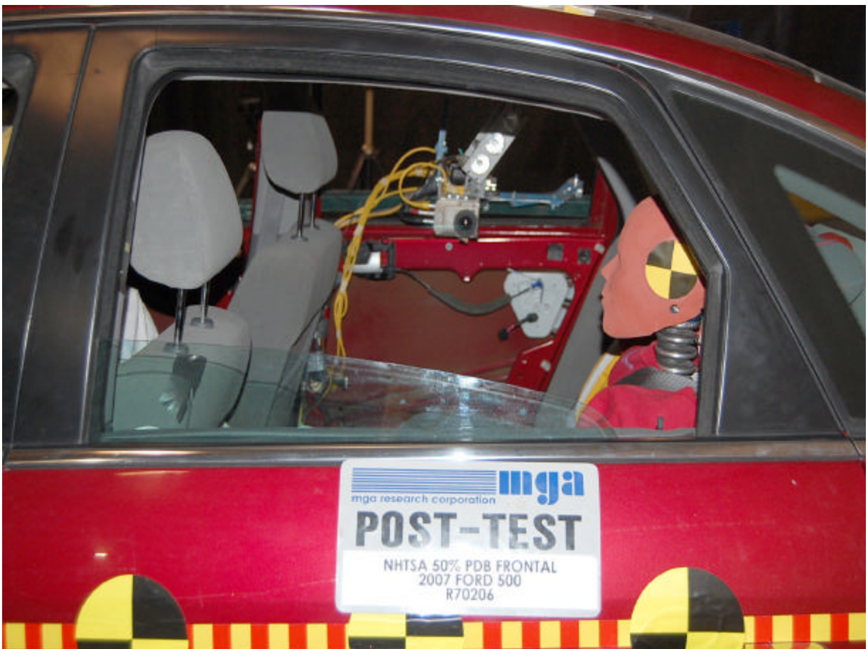
Post-Test Left Rear Passenger Dummy (Through Window)
