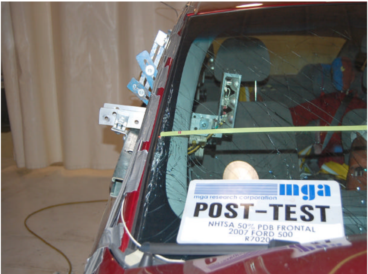
Post-Test Right Side A Pillar (Frontal View)
