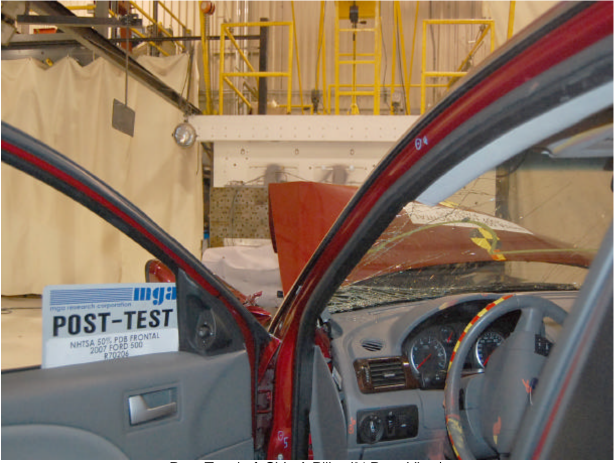
Post-Test Left Side A Pillar (¾ Rear View)
