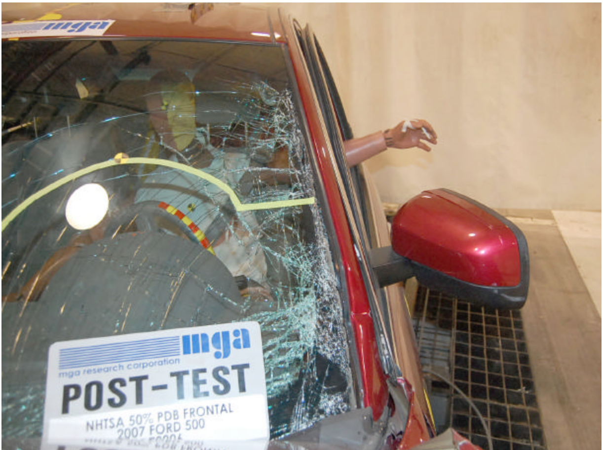
Post-Test Left Side A Pillar (Frontal View)
