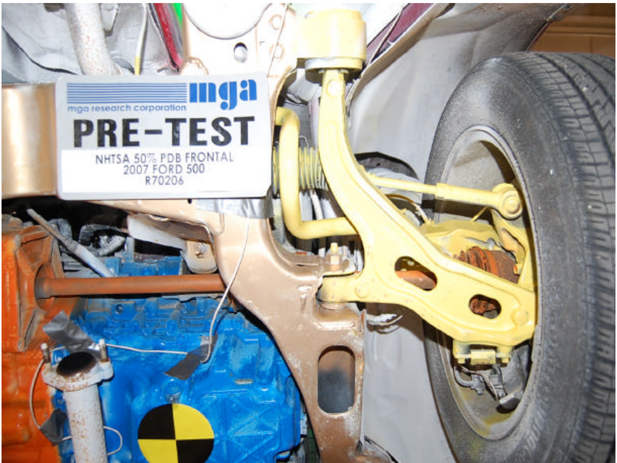
Pre-Test Sway Bar Right Side View
