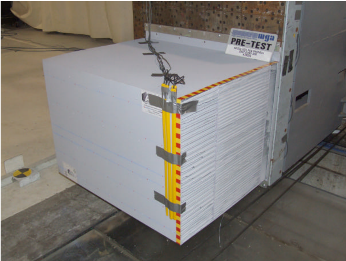
Pre-Test Offset Deformable Barrier Right Side \frac{3}{4} View
