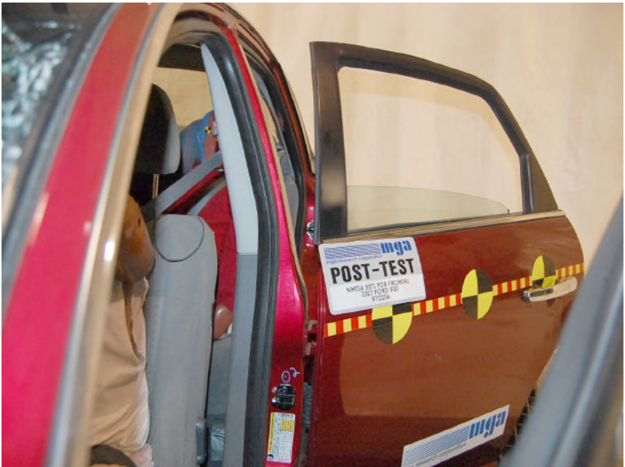
Post-Test Left Side B Pillar (¾ Front View)
