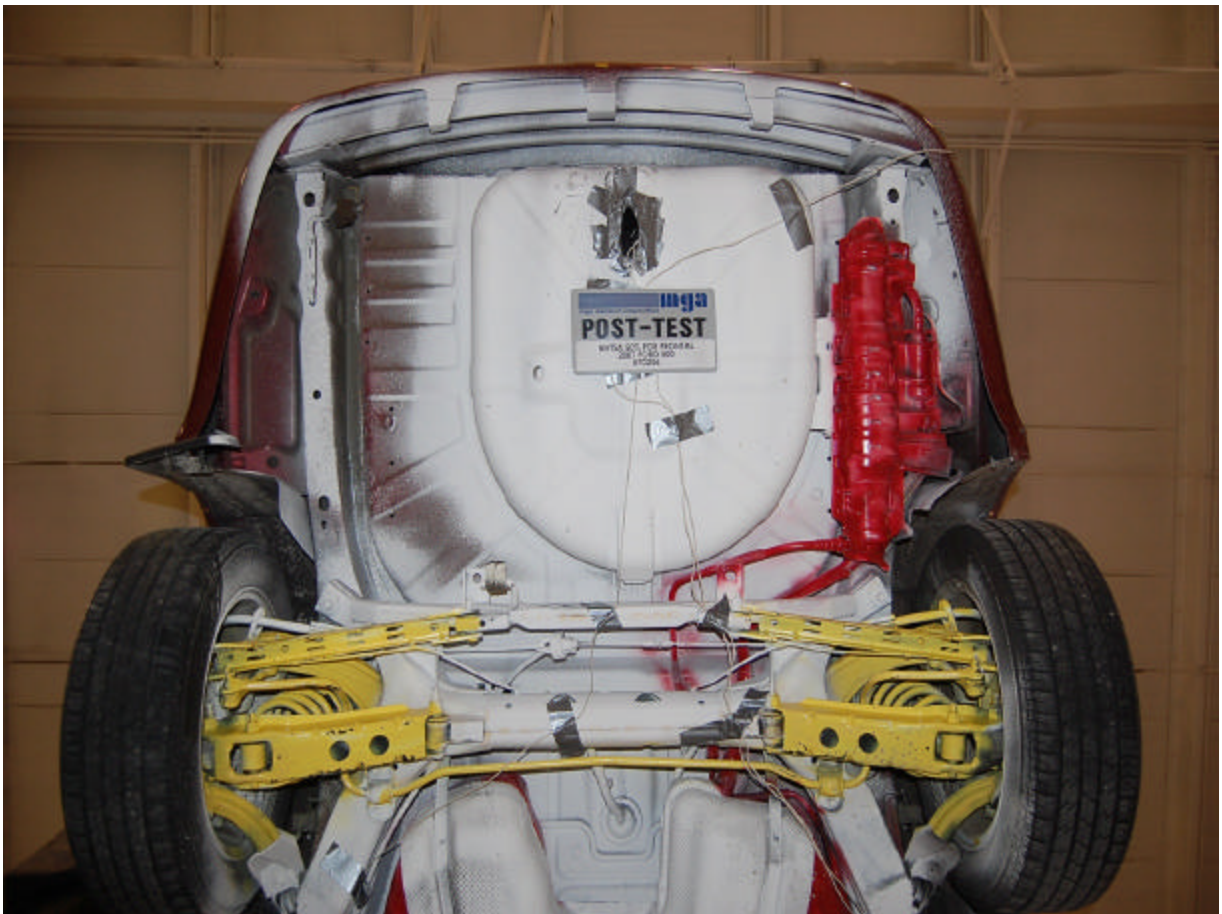
Post-Test Rear Underbody View
