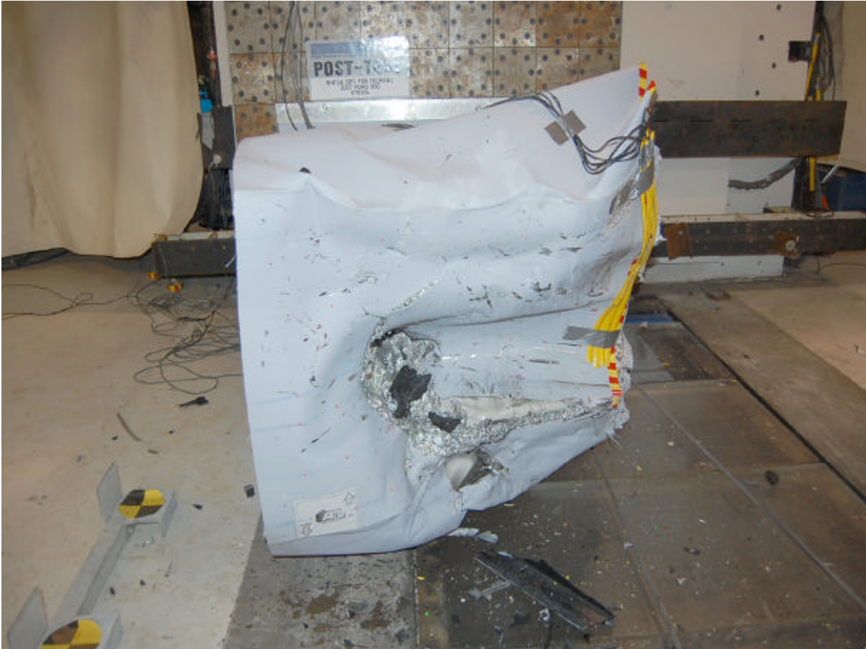
Post-Test Offset Deformable Barrier Front View
