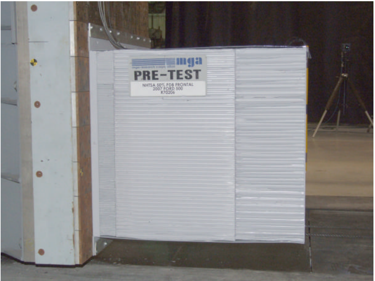
Pre-Test Offset Deformable Barrier Left Side View
