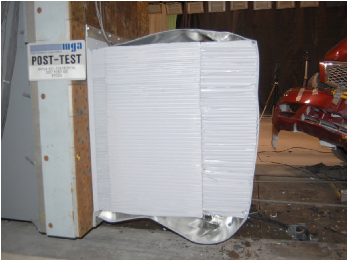
Post-Test Offset Deformable Barrier Left Side View
