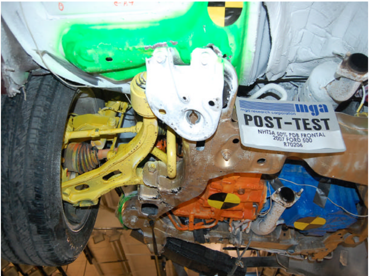
Post-Test Steering Rack Left Side View
