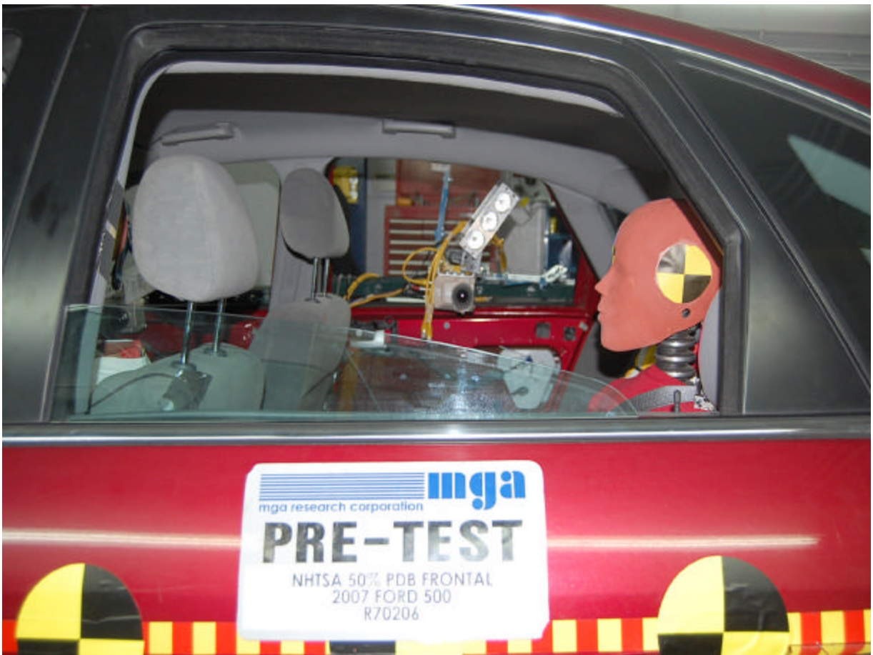
Pre-Test Left Rear Passenger Dummy (Through Window)
