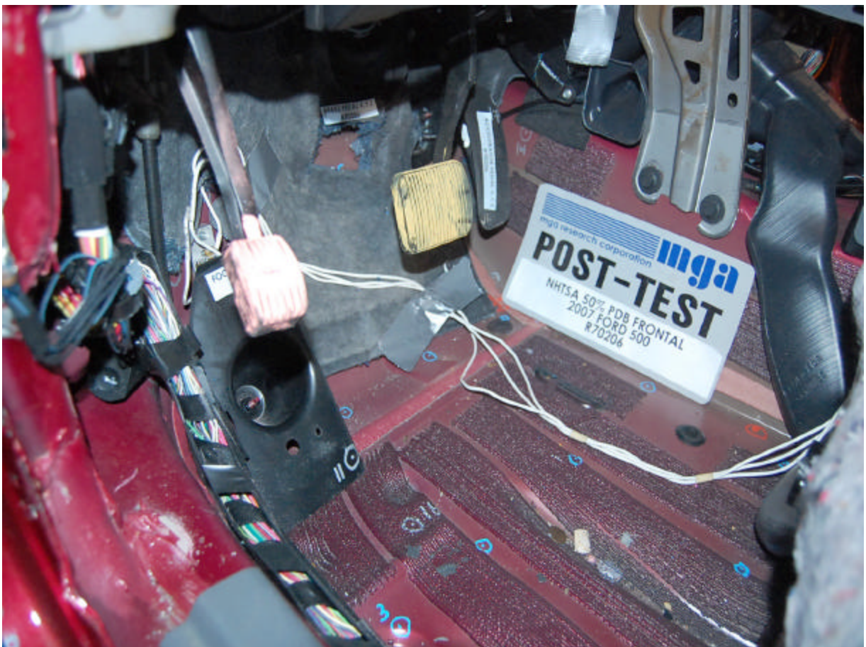
Post-Test Driver Side Floor Pan
