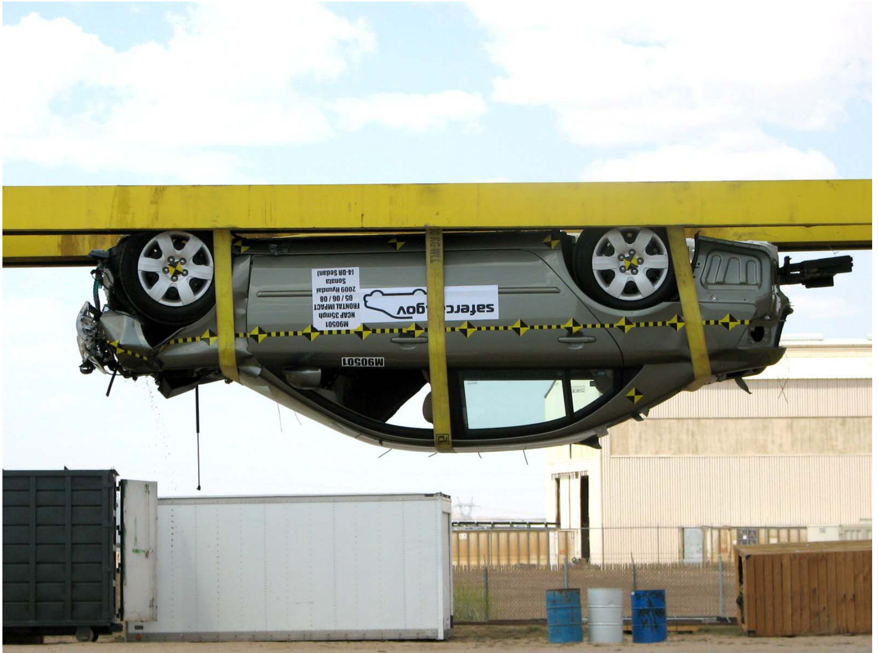
Figure A-60: Vehicle on Rollover Device (180°)
