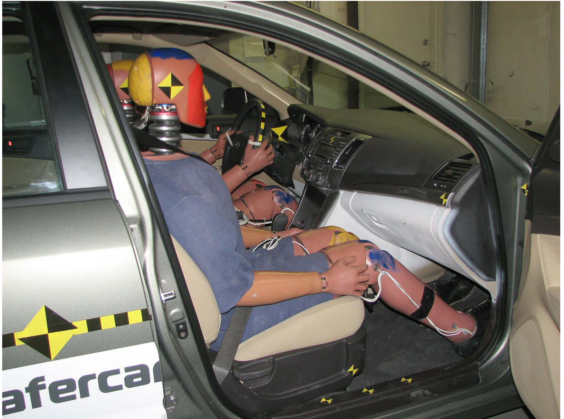
Figure A-48: Pre-Test Passenger Dummy (Door Open)
