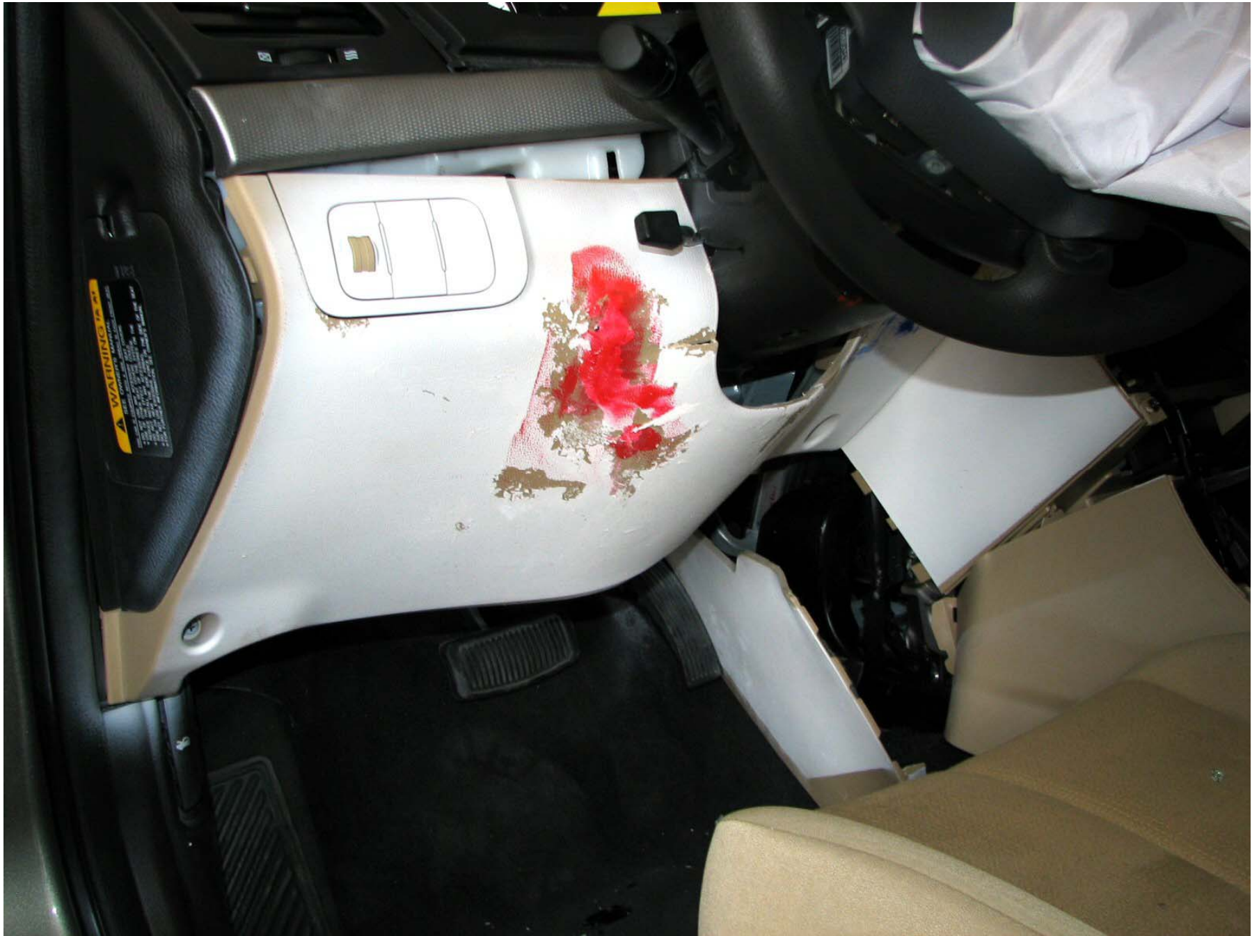
Figure A-39: Post-Test Driver Side Knee Bolster
