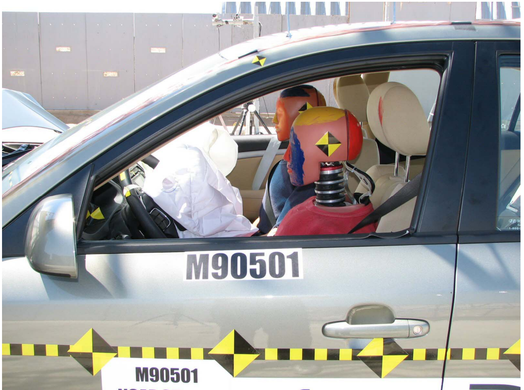
Figure A-33: Post-Test Driver Dummy (Through Window)
