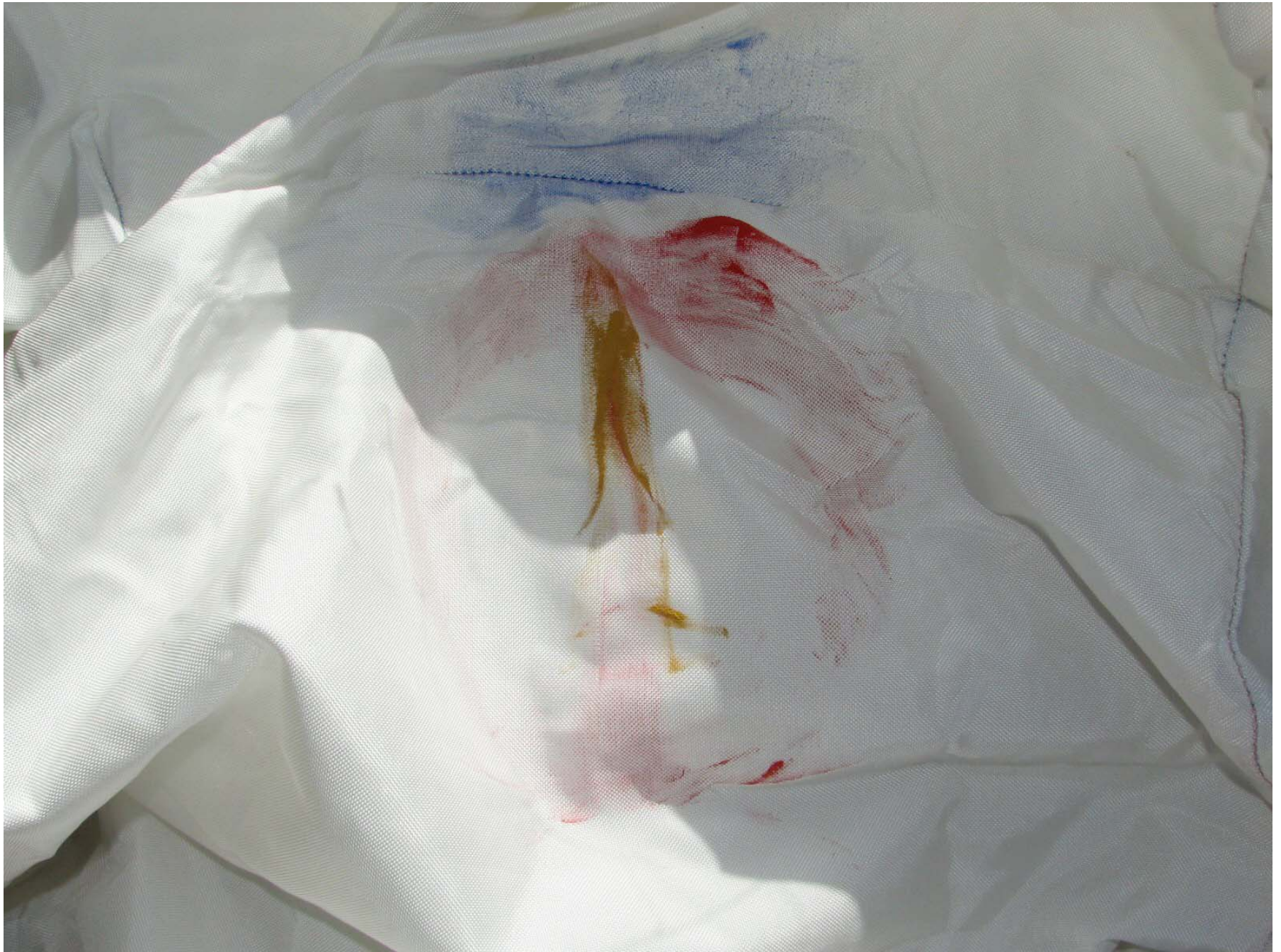
Figure A-57: Post-Test Passenger Dummy Airbag Contact
