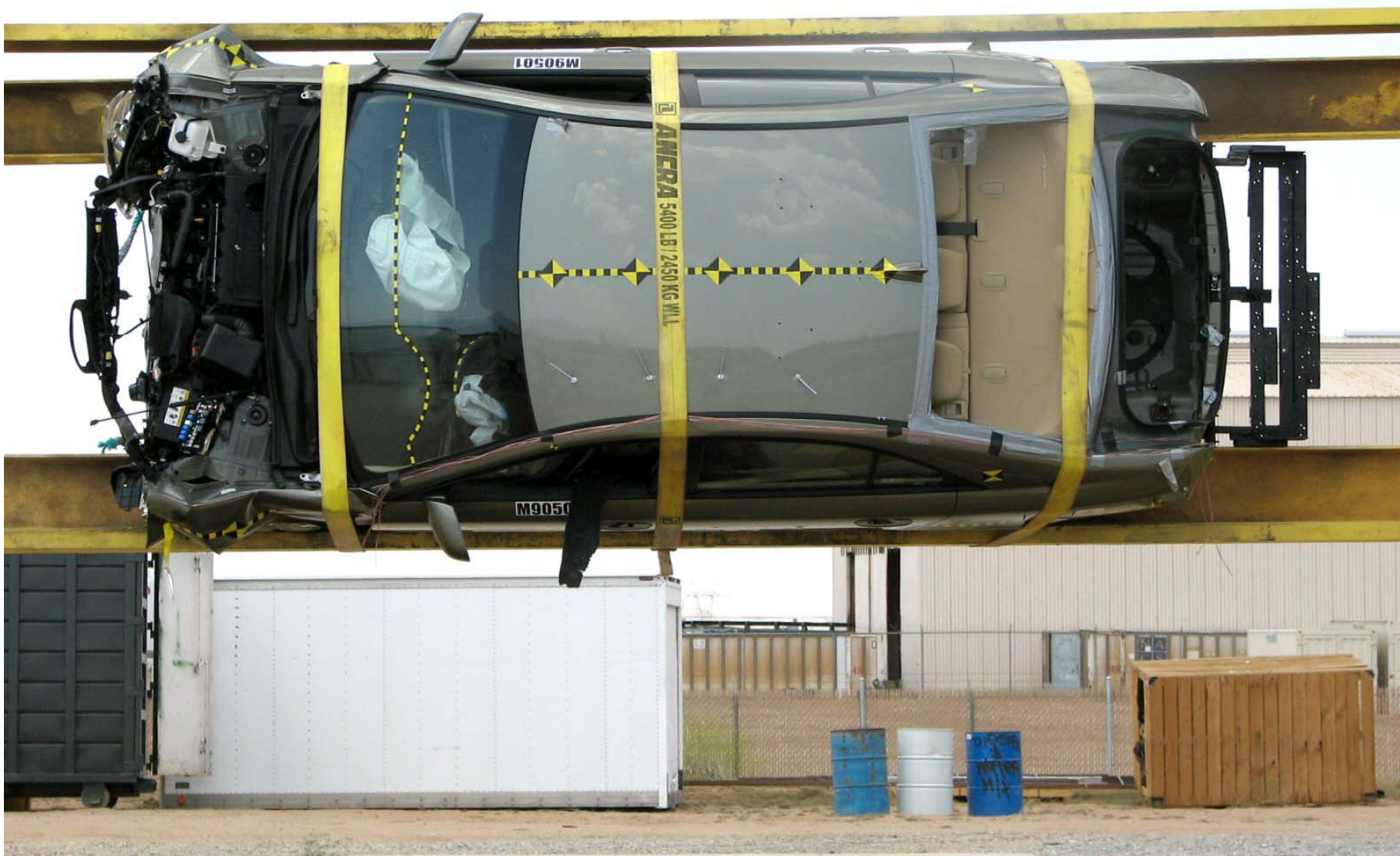
Figure A-59: Vehicle on Rollover Device (90°)
