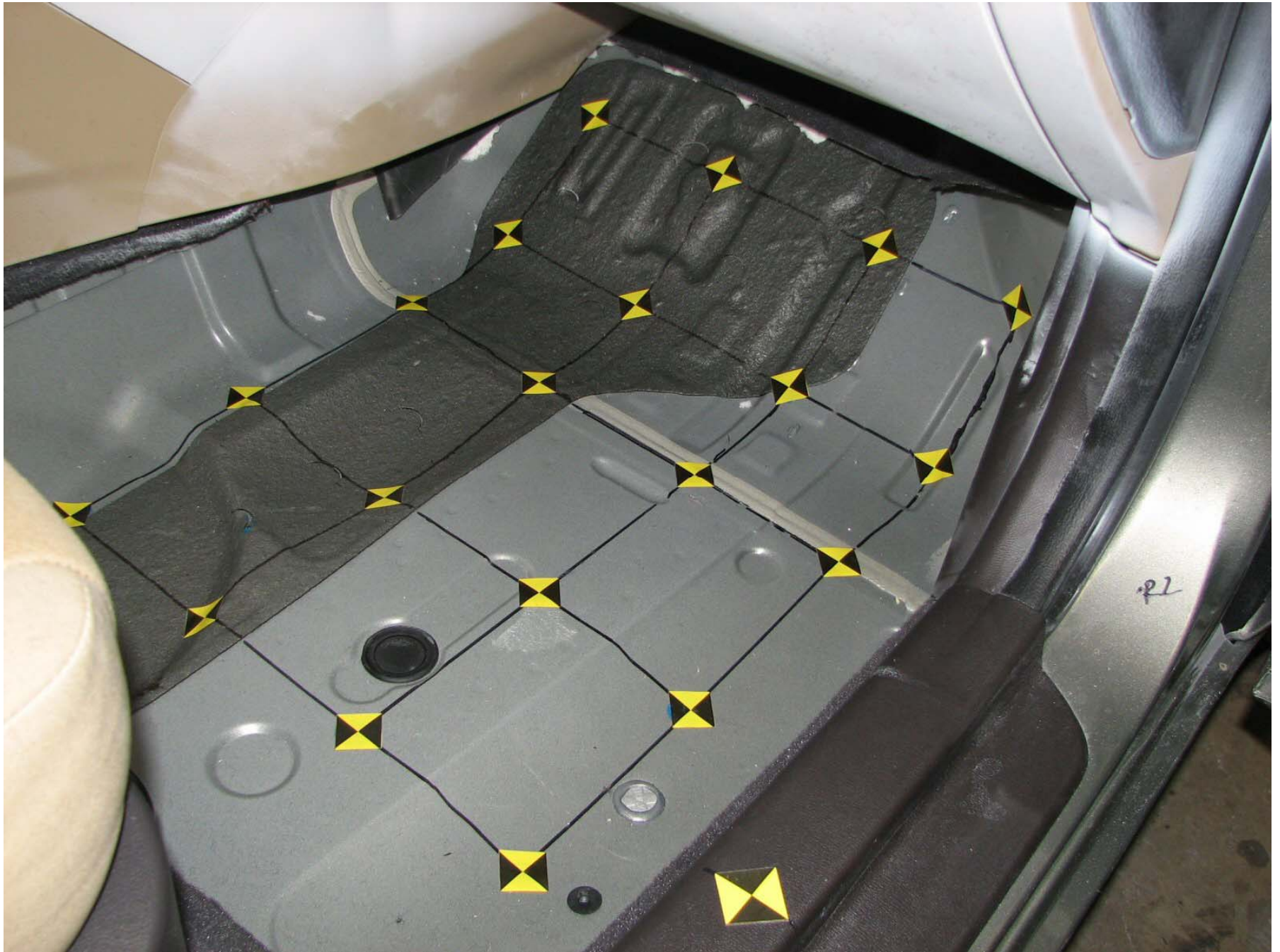
Figure A-54: Pre-Test Passenger Side Floor Pan
