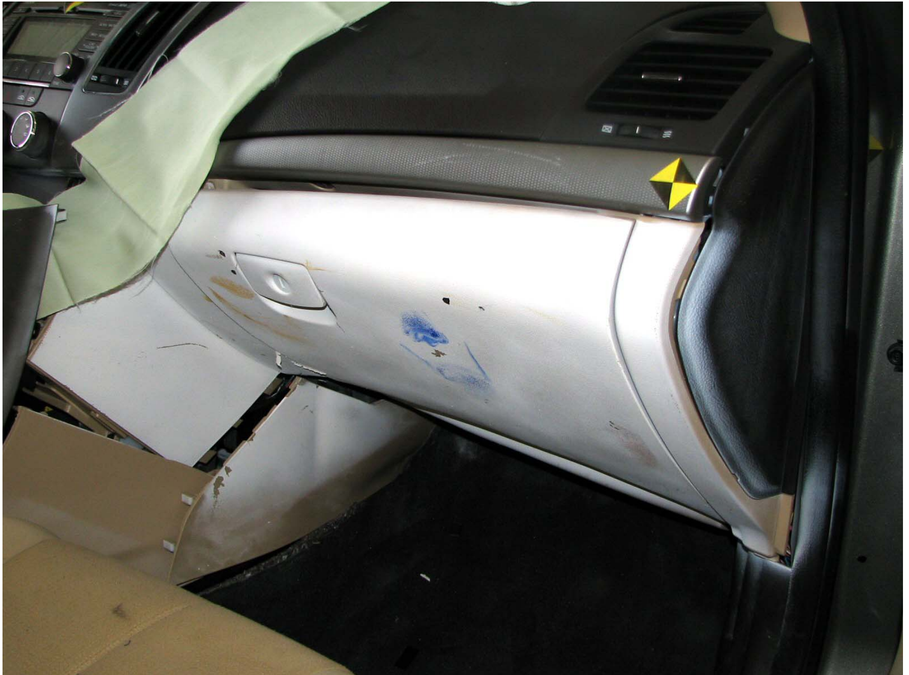
Figure A-53: Post-Test Passenger Side Glove Box
