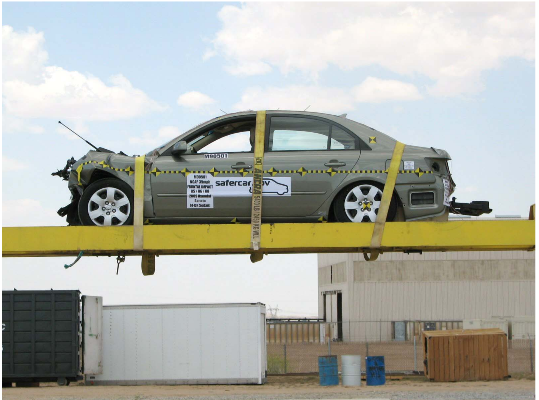
Figure A-58: Vehicle on Rollover Device (0°)
