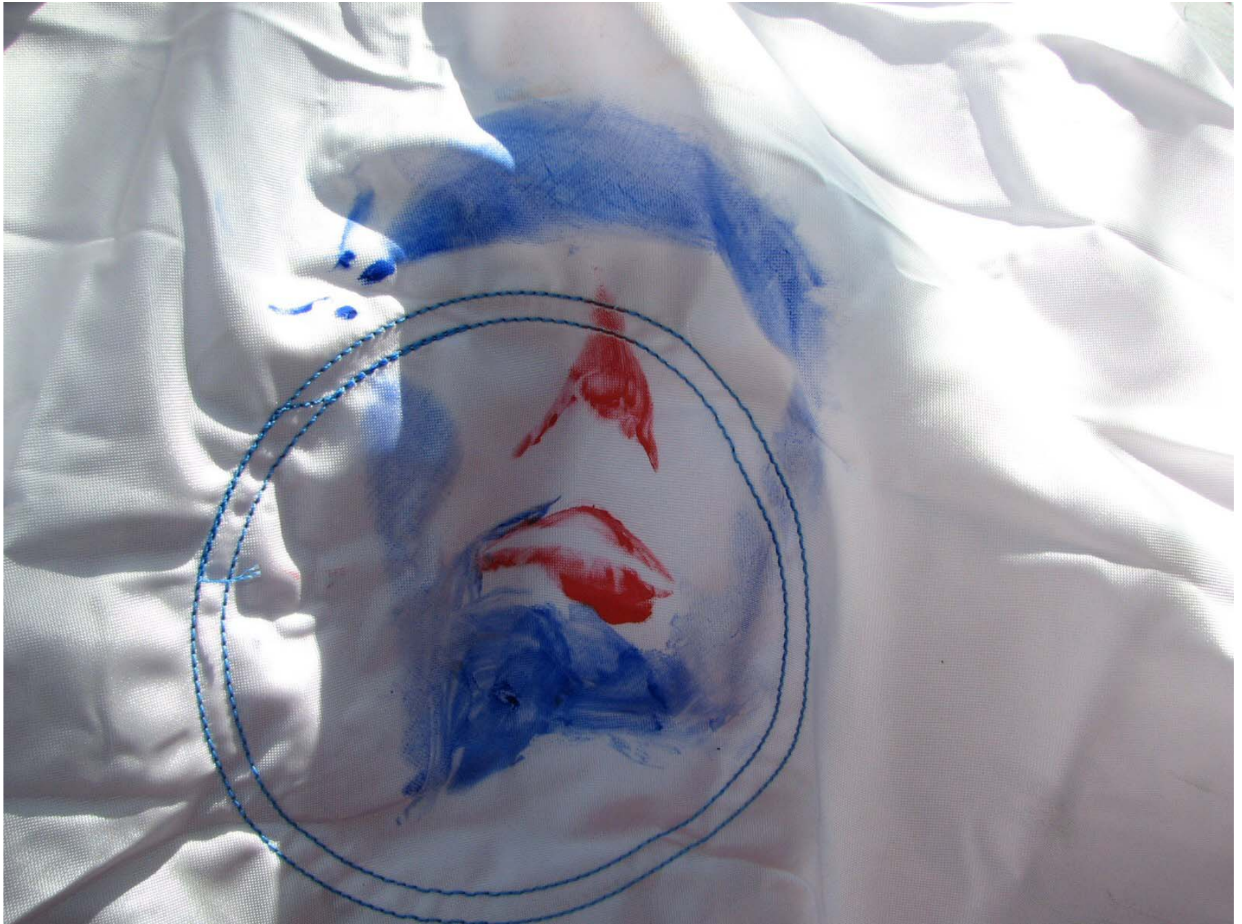
Figure A-43: Post-Test Driver Dummy Airbag Contact
