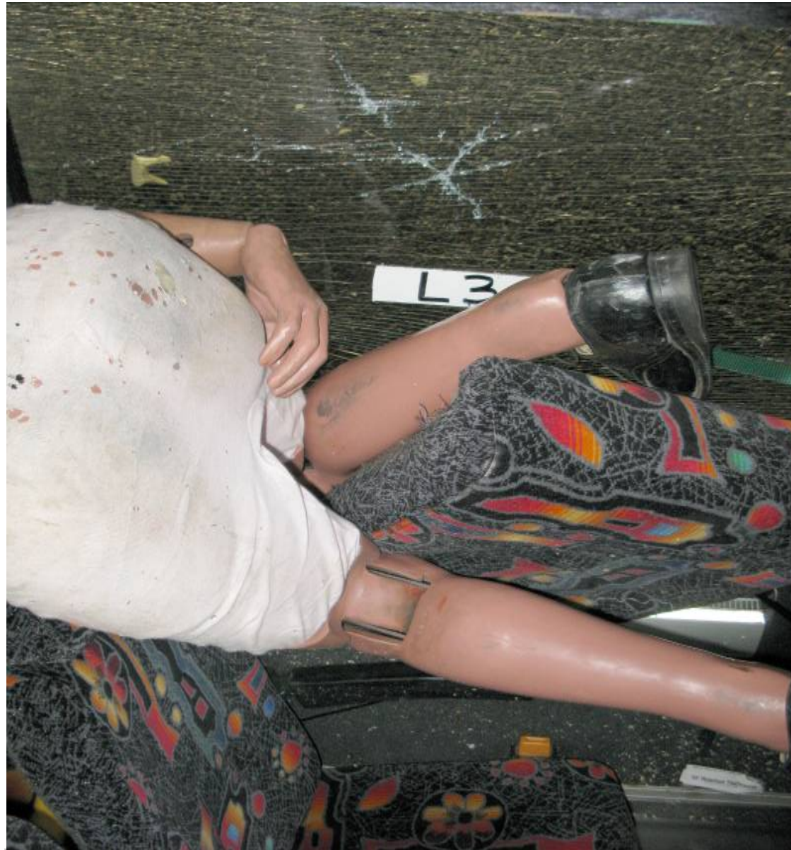
Post-Test Window Damage (Left Window 3)
