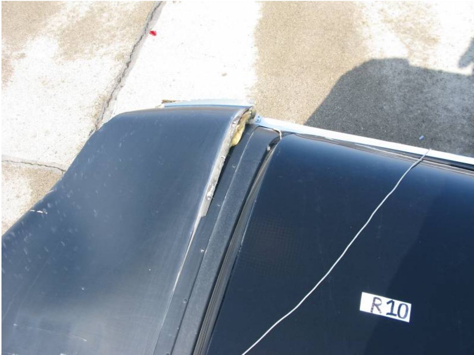
Post-Test Exterior Right Rear Side of Bus Damage
