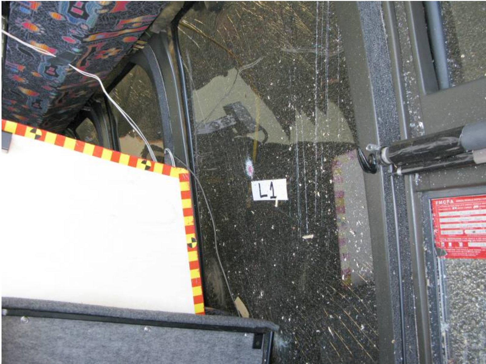
Post-Test Window Damage (Left Window 1)
