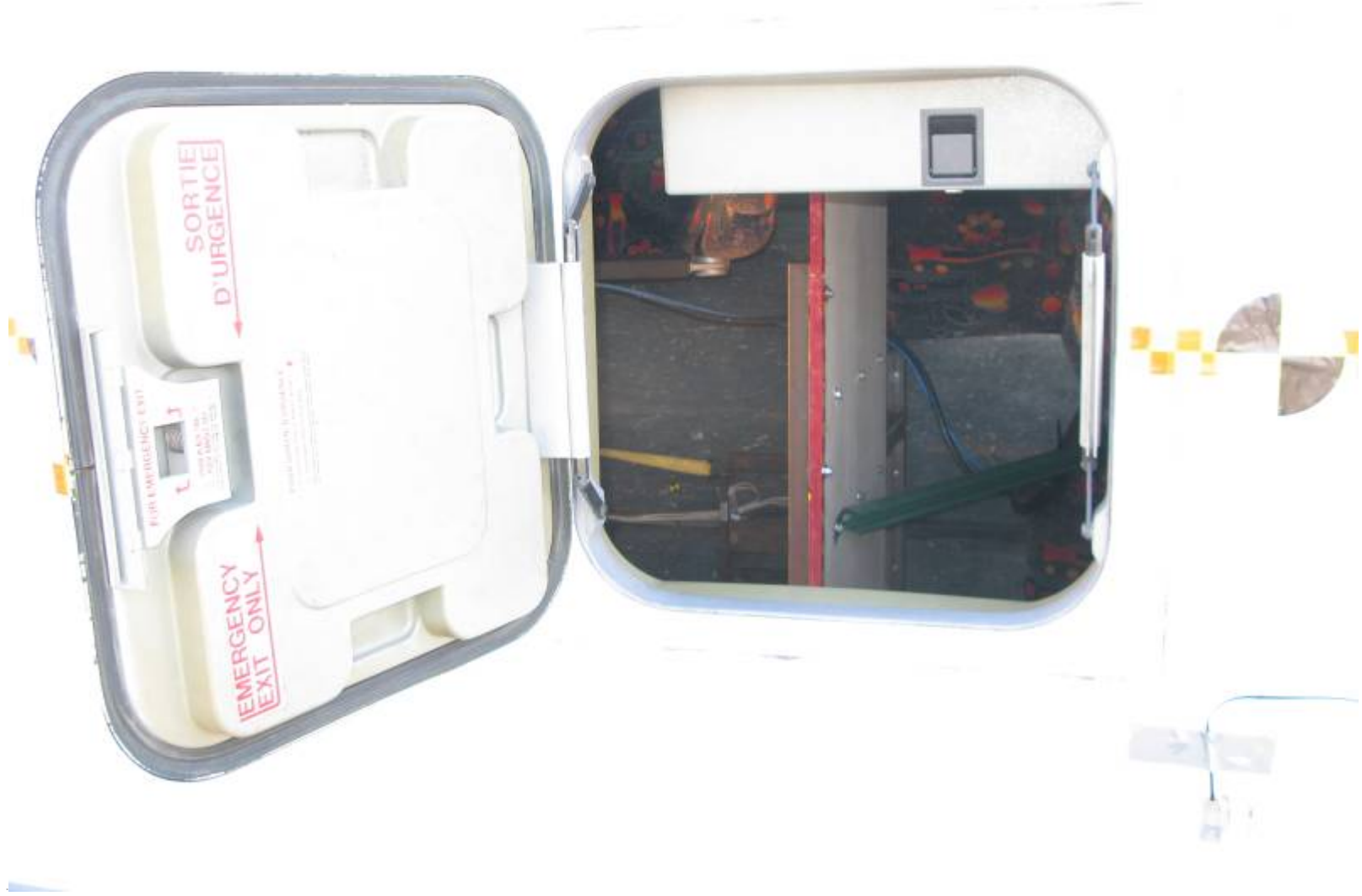
Post-Test Roof Exit Exterior View
