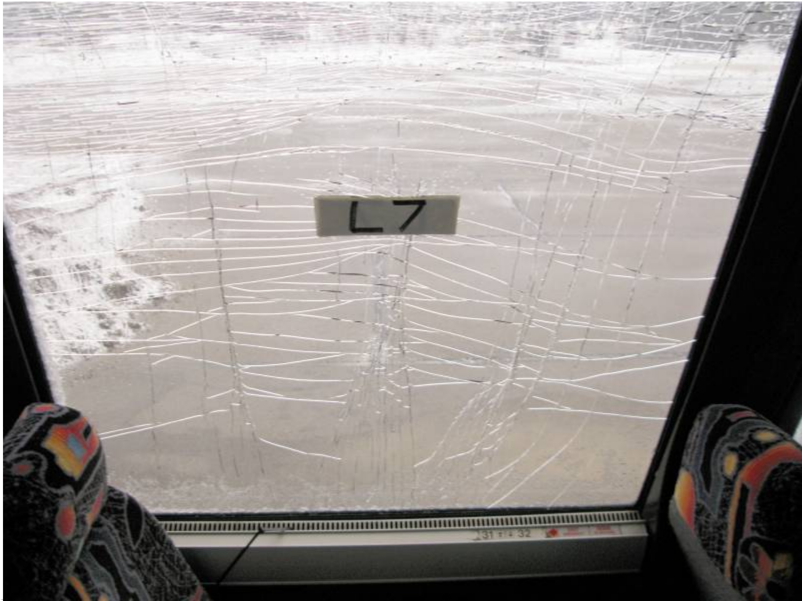
Post-Test Left Side Window 7 Interior View
