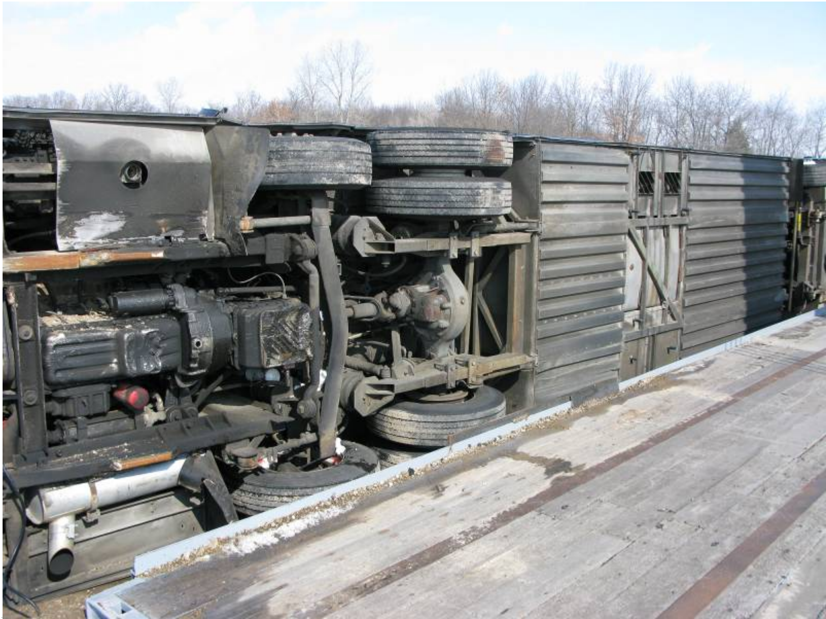
Post-Test Rear Underbody of Bus after Roll
