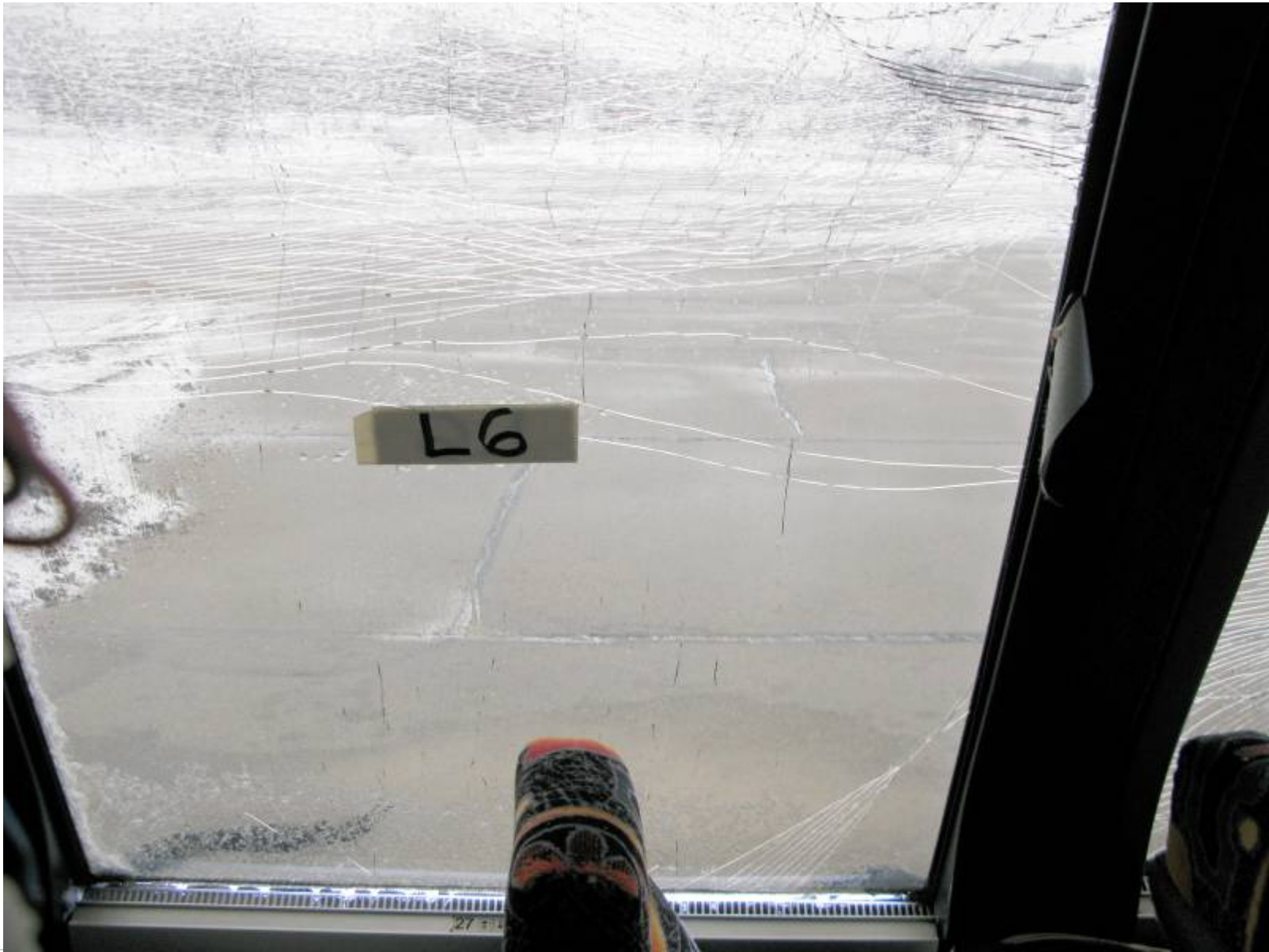
Post-Test Left Side Window 6 Interior View
