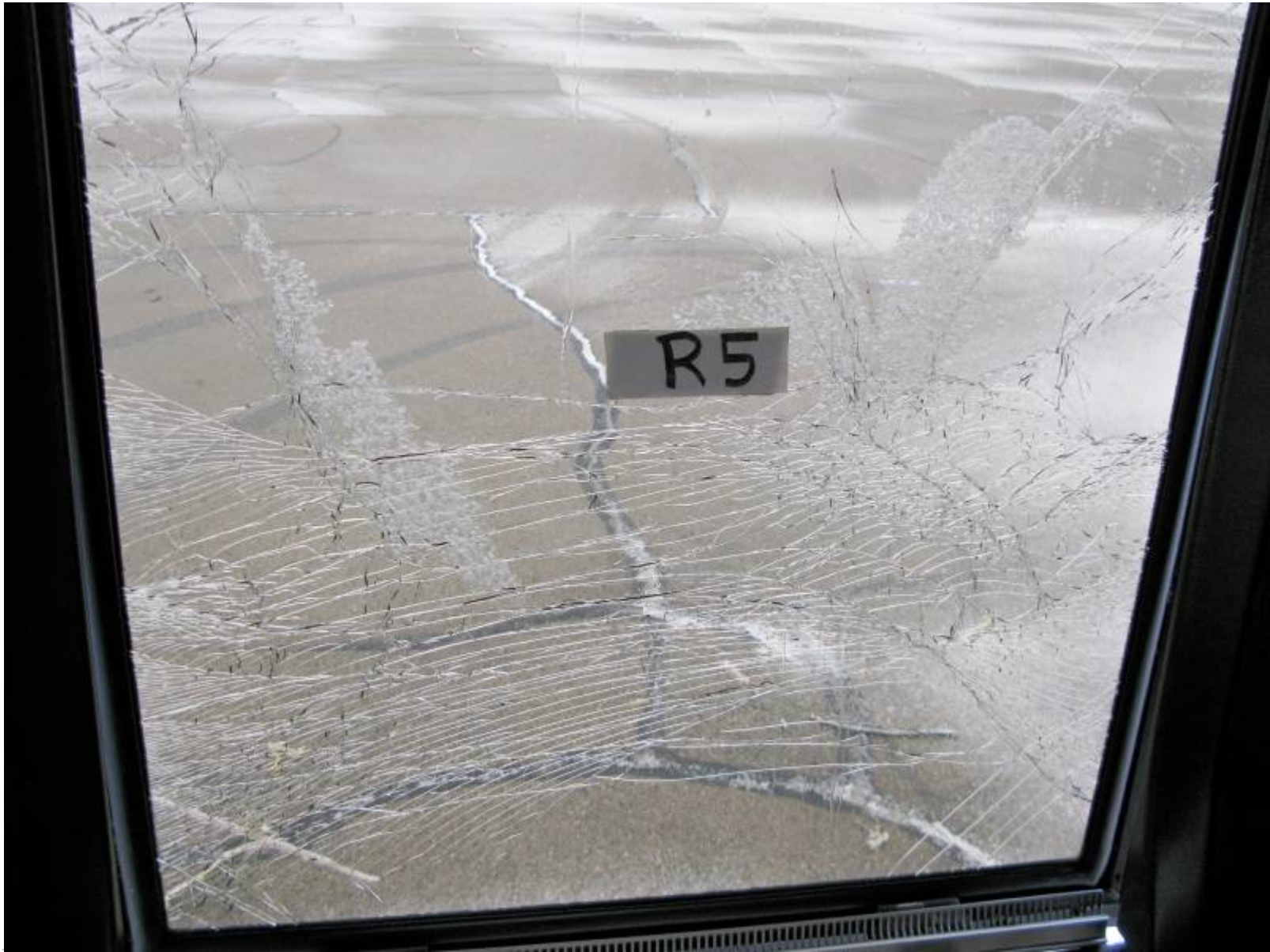
Post-Test Right Side Window 5 Interior View
