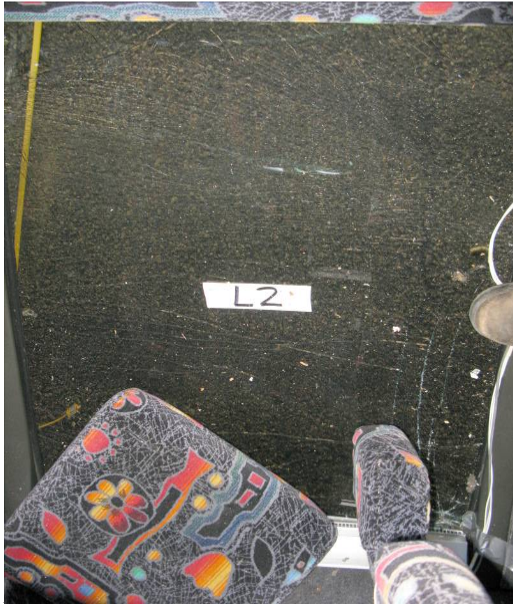
Post-Test Window Damage (Left Window 2)
