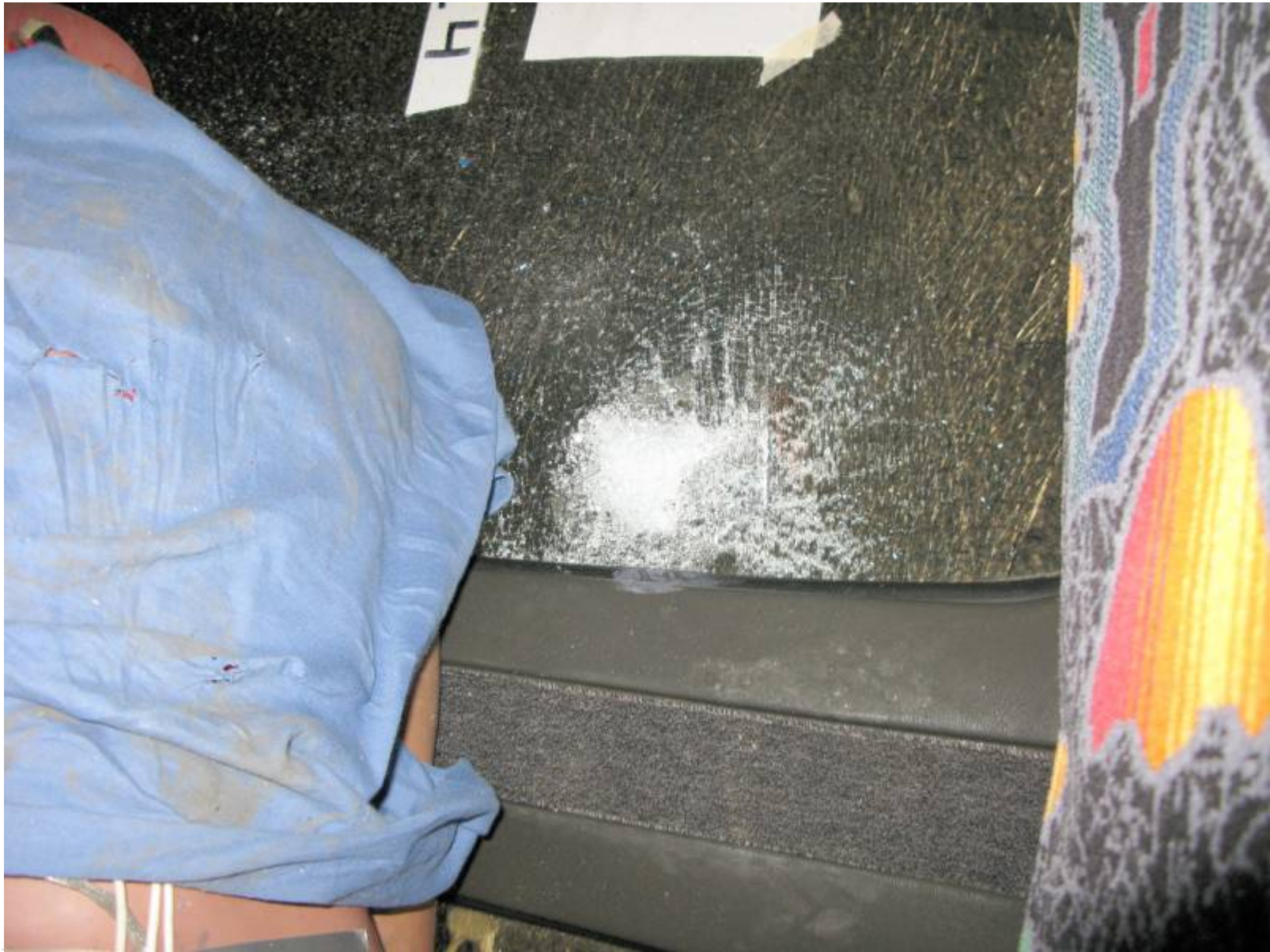
Post-Test Window Damage (Left Window 4)
