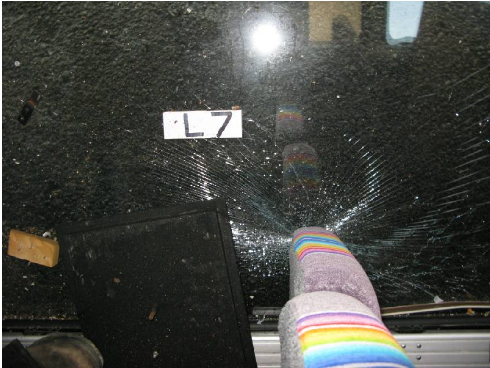
Post-Test Window Damage (Left Window 7)
