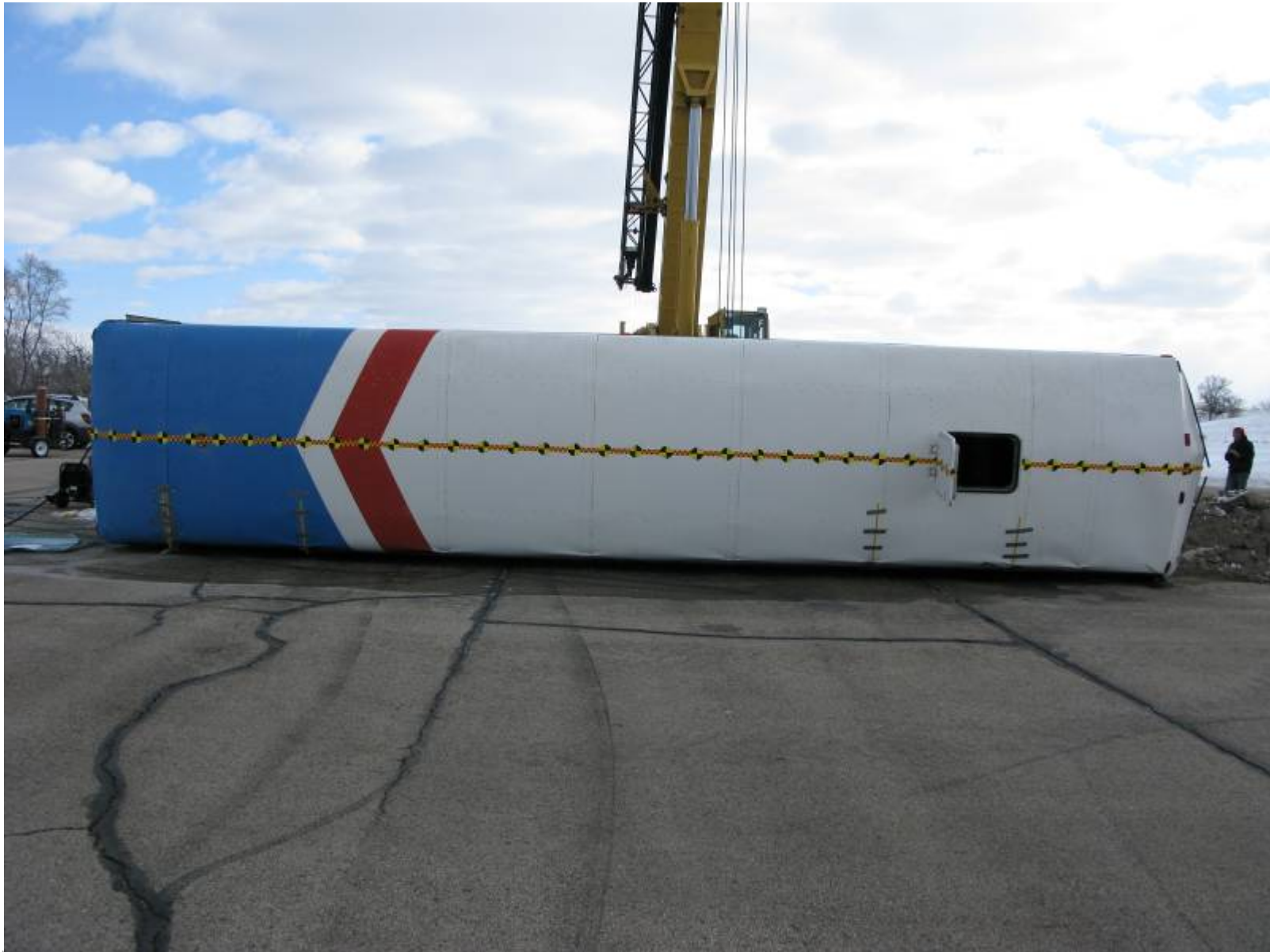
Post-Test View of Bus Roof after Roll
