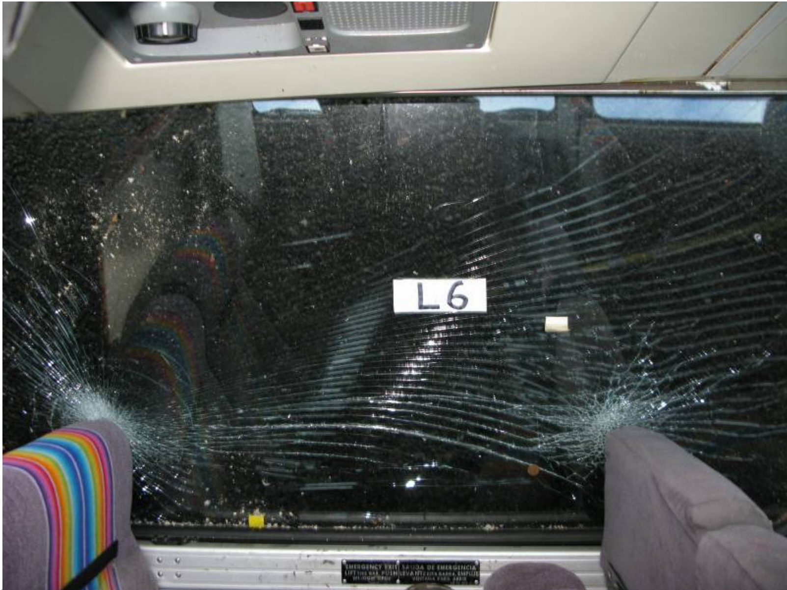
Post-Test Window Damage (Left Window 6)
