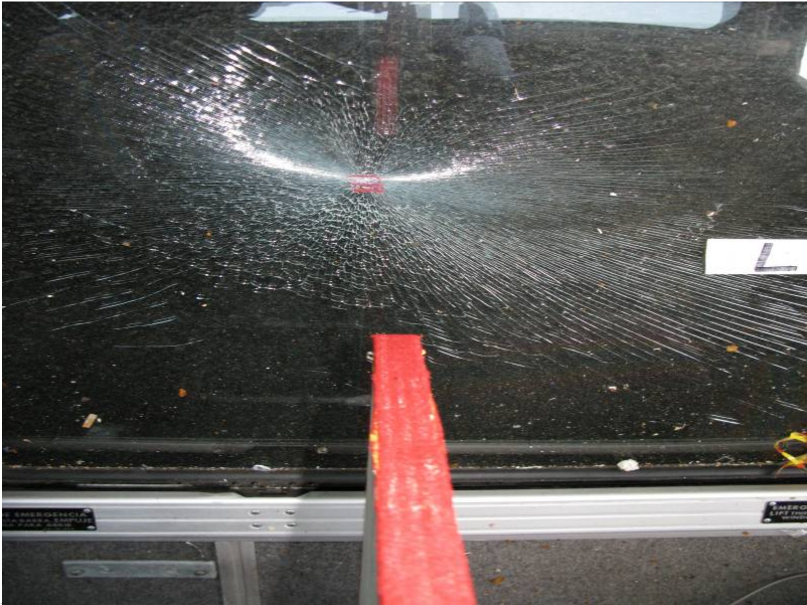
Post-Test Window Damage (Left Window 1)
