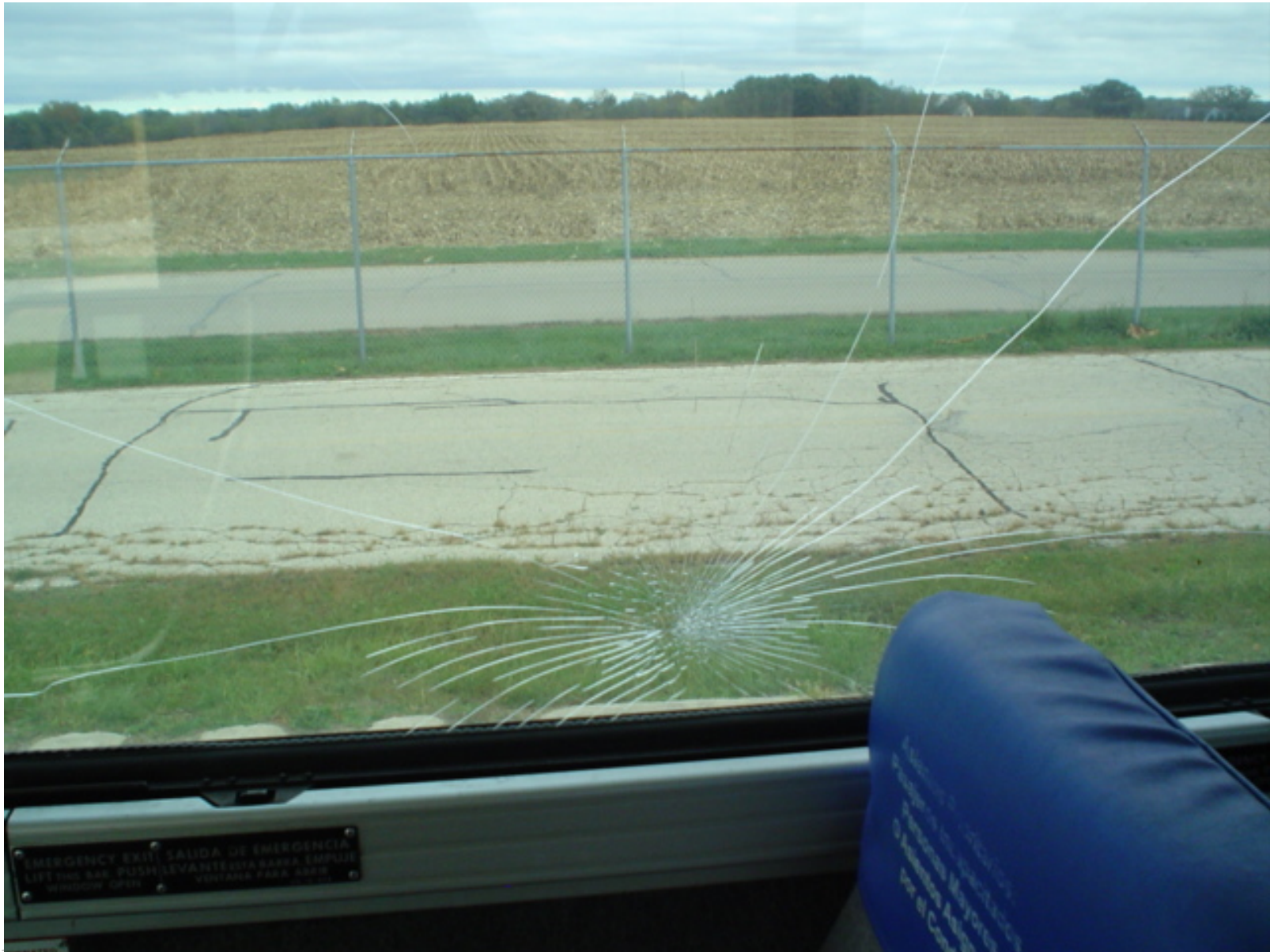
Pre-Test Right Window 1 Damage
