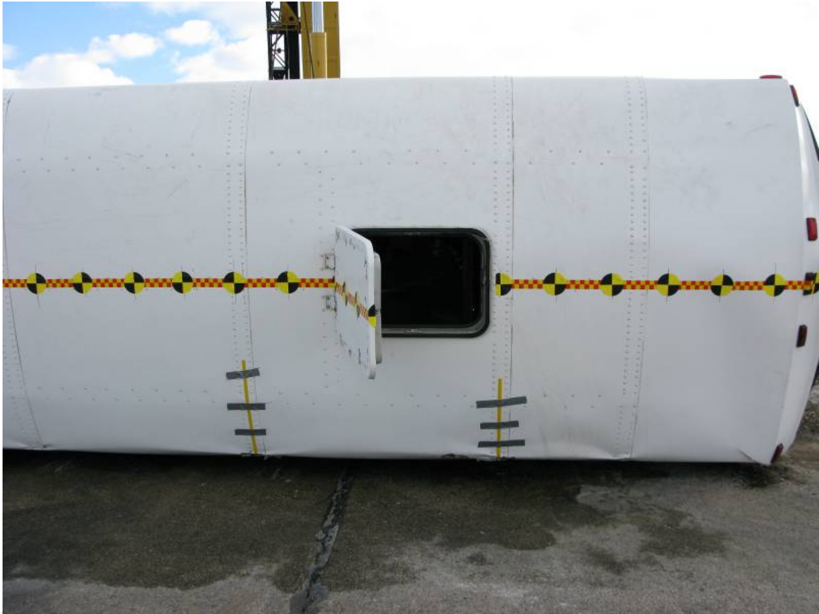
Post-Test Roof Exit Exterior View
