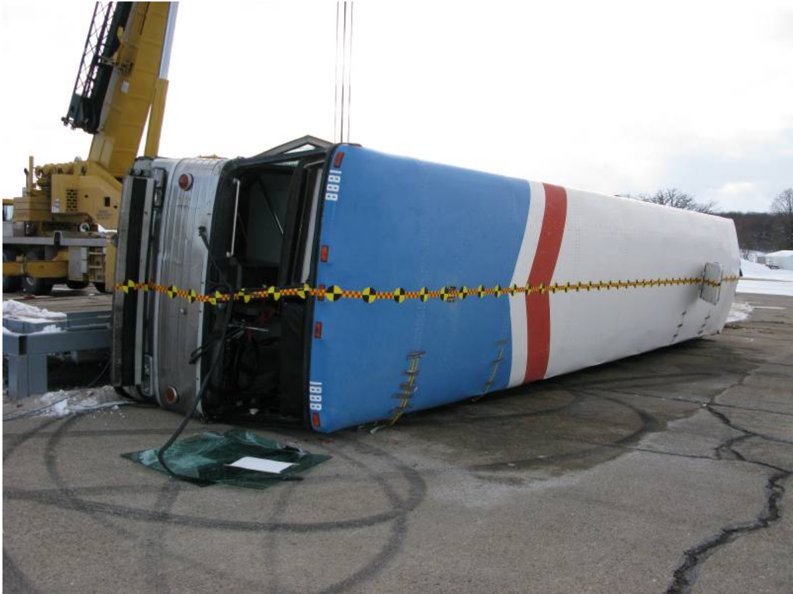
Post-Test ¾ View of Bus Roof after Roll
