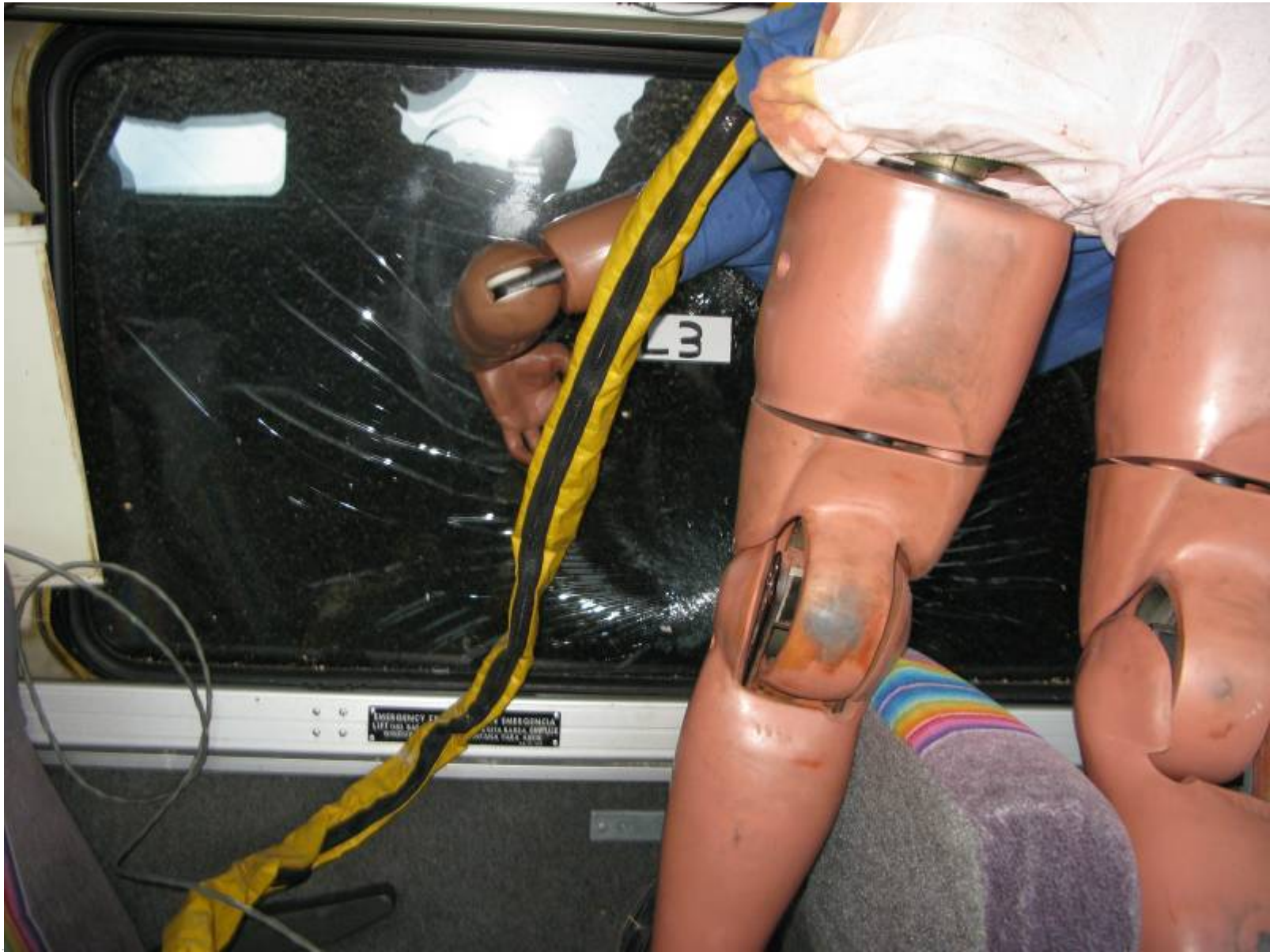
Post-Test Window Damage (Left Window 3)
