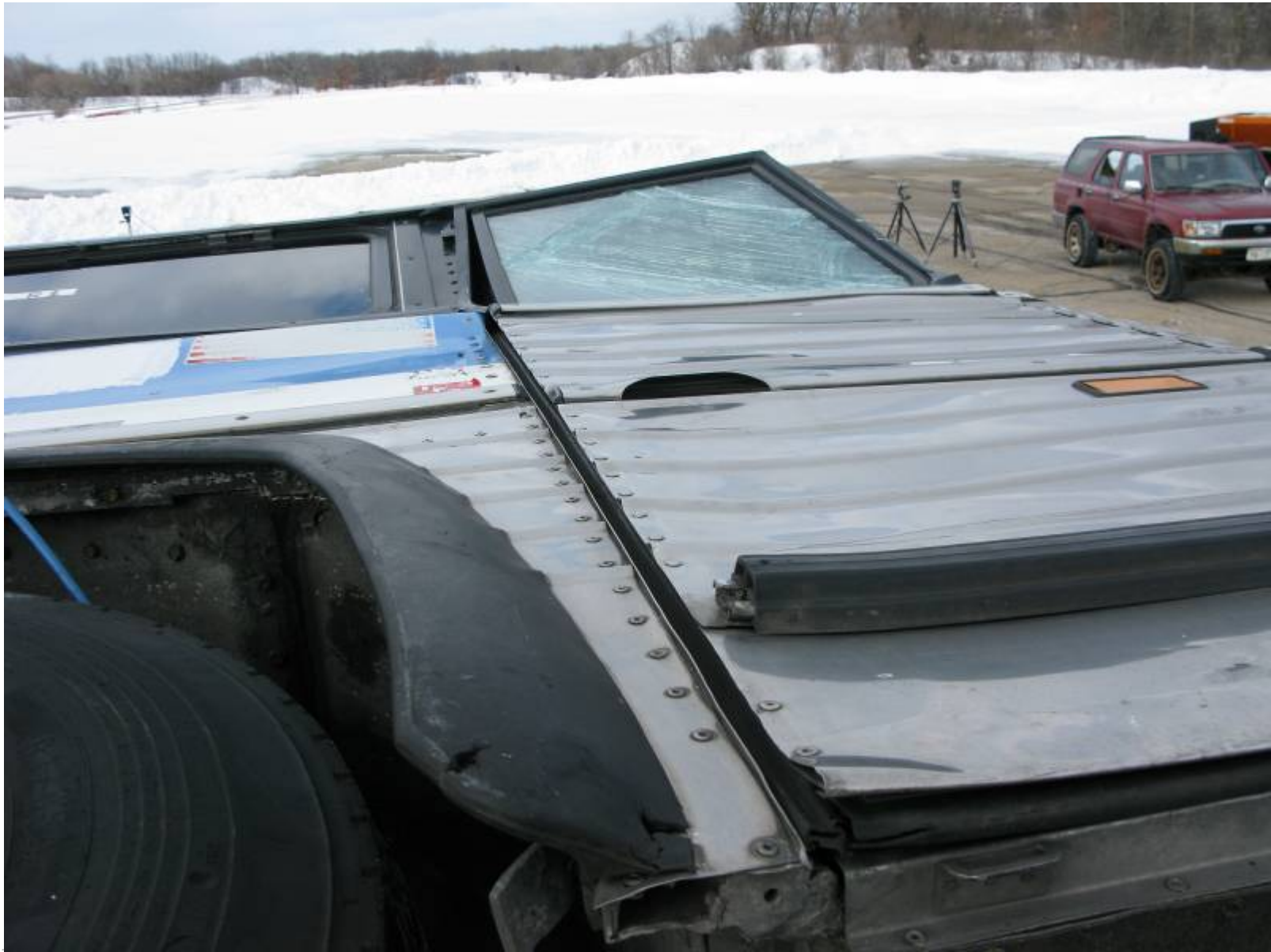
Post-Test Front Door Exterior Damage
