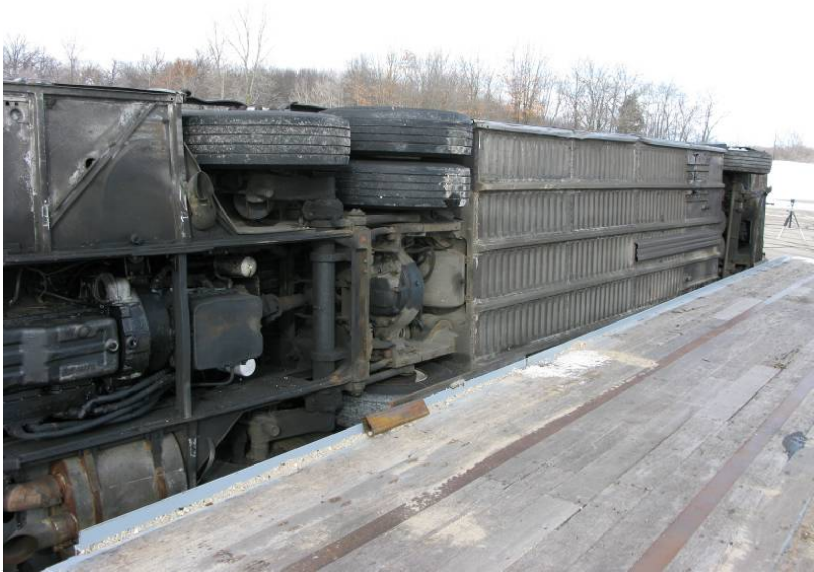
Post-Test Rear Underbody of Bus after Roll
