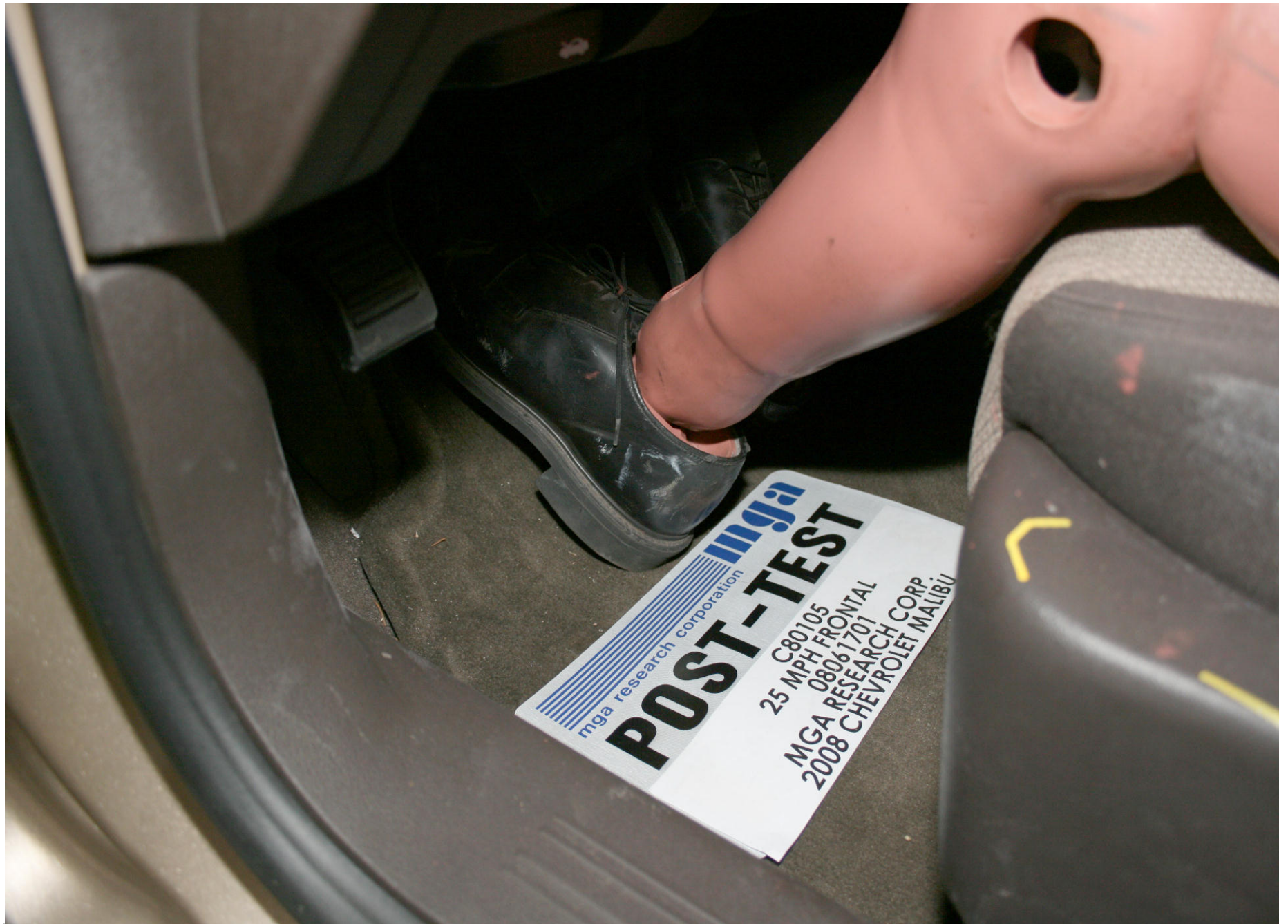
Post-Test Driver Dummy Feet Position
