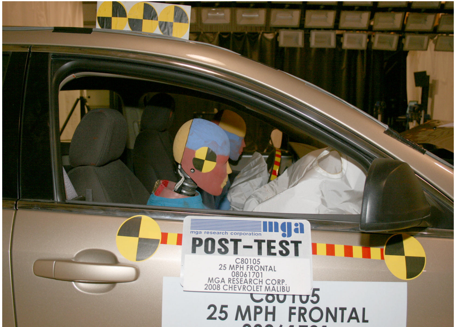
Post-Test Passenger Dummy Position Right Side View
