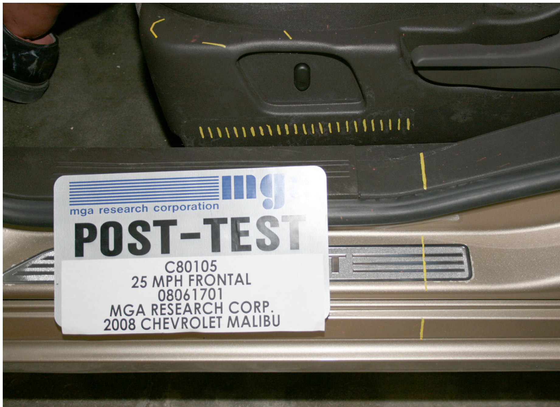
Post-Test Driver Dummy Seat Position
