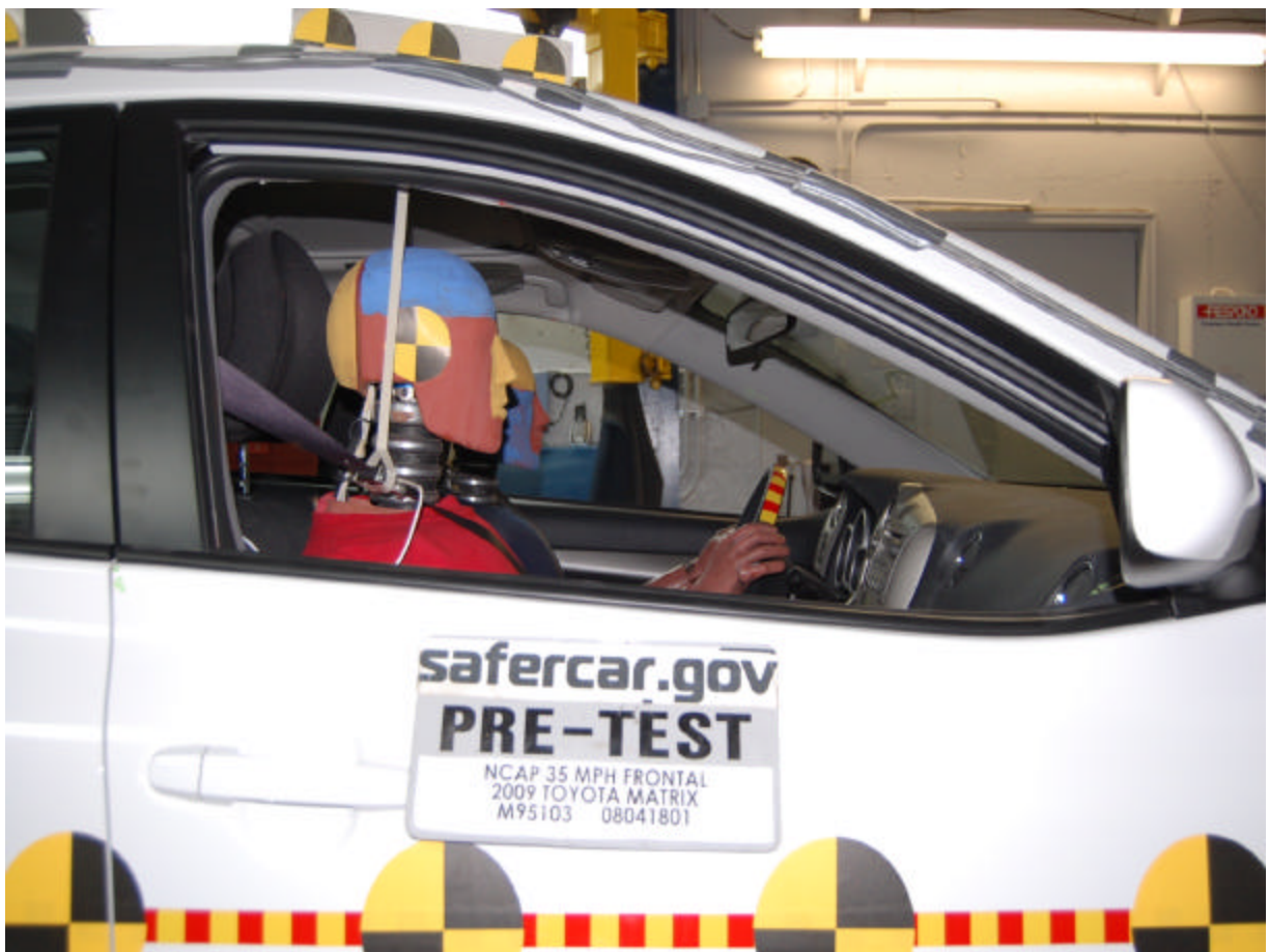
Pre-Test Passenger Dummy (Through Window)
