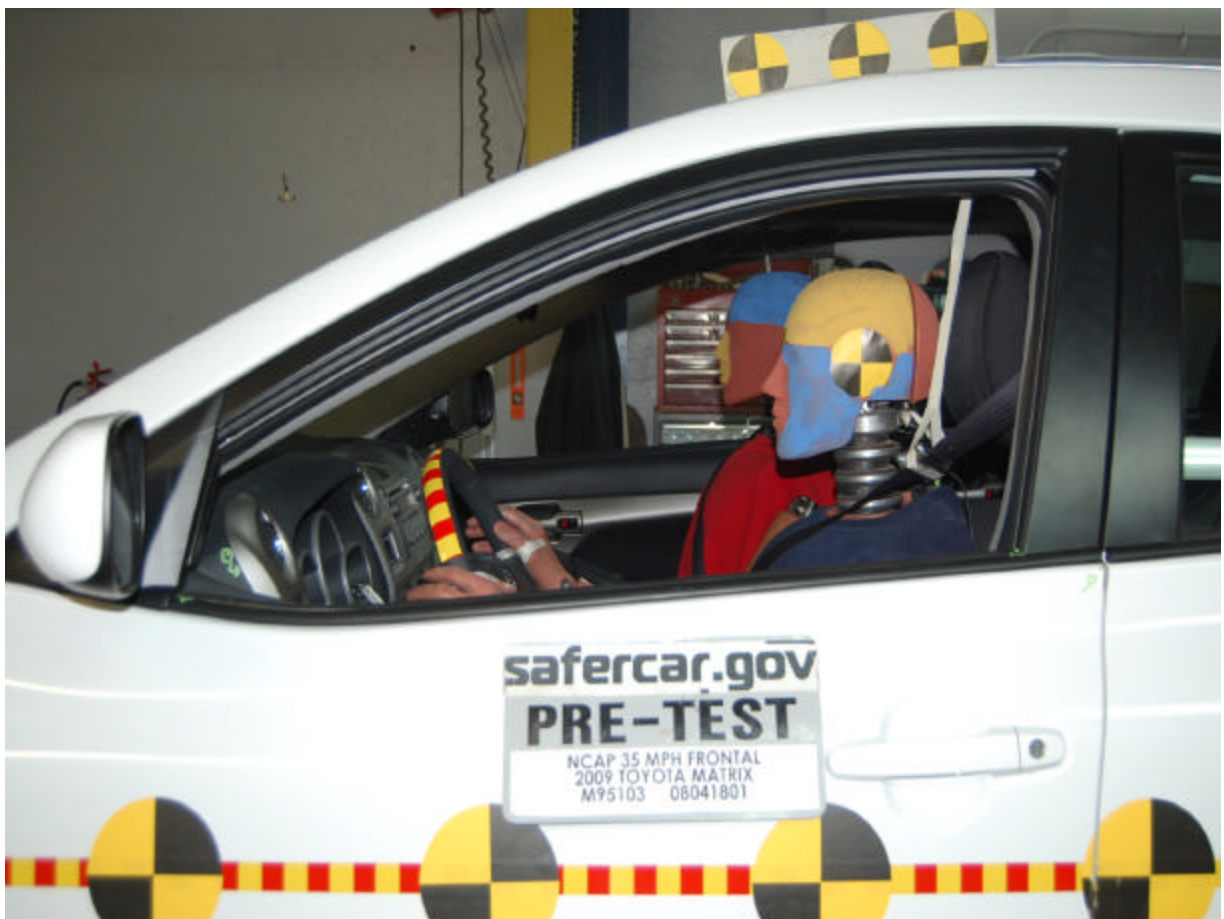
Pre-Test Driver Dummy (Through Window)
