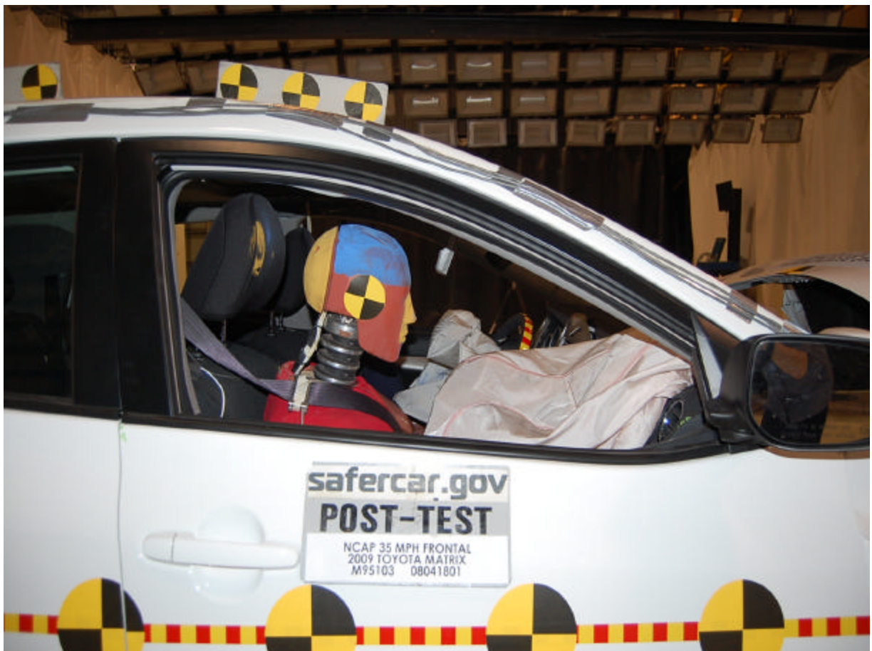
Post-Test Passenger Dummy (Through Window)
