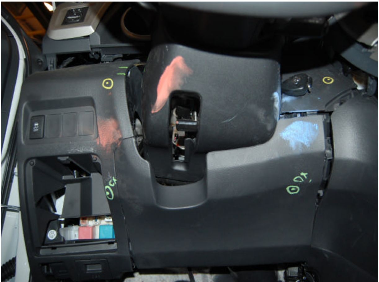
Post-Test Driver Dummy Knee Contact
