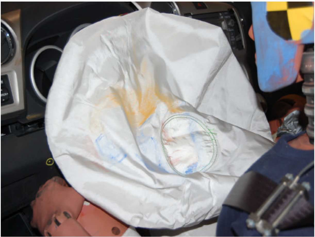
Post-Test Driver Dummy Airbag Contact
