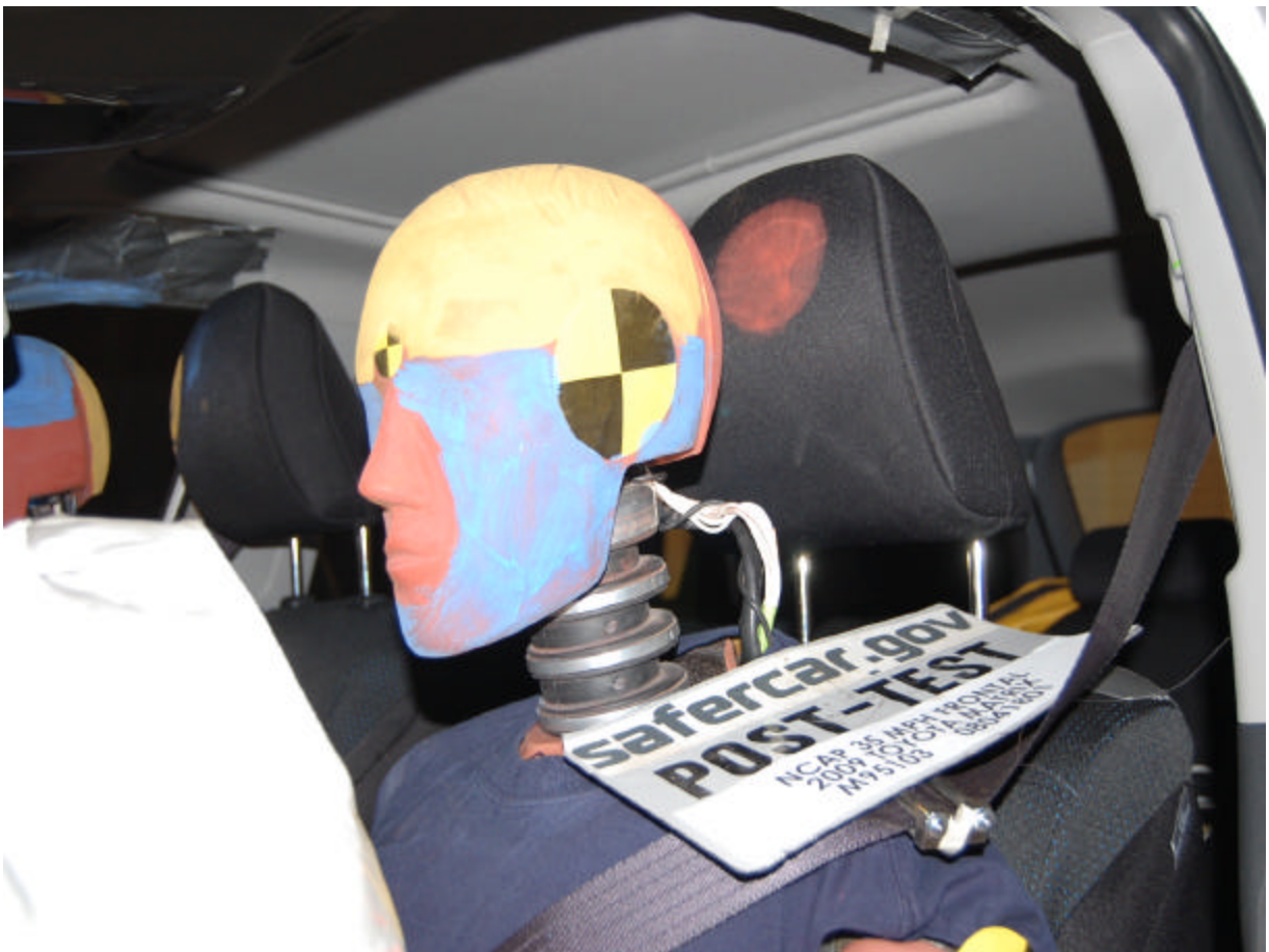
Post-Test Driver Dummy Head Contact (Headrest)
