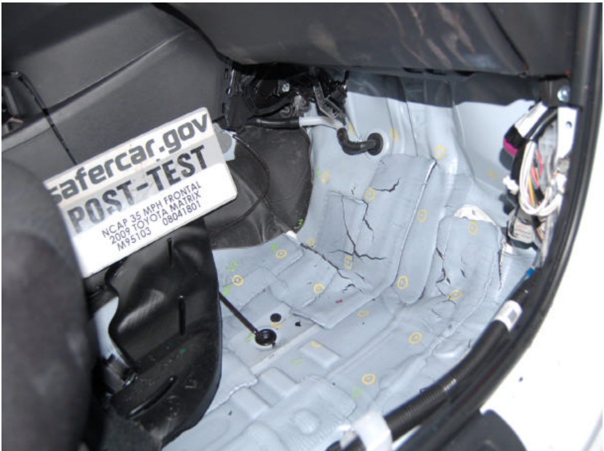
Post-Test Passenger Side Floor Pan
