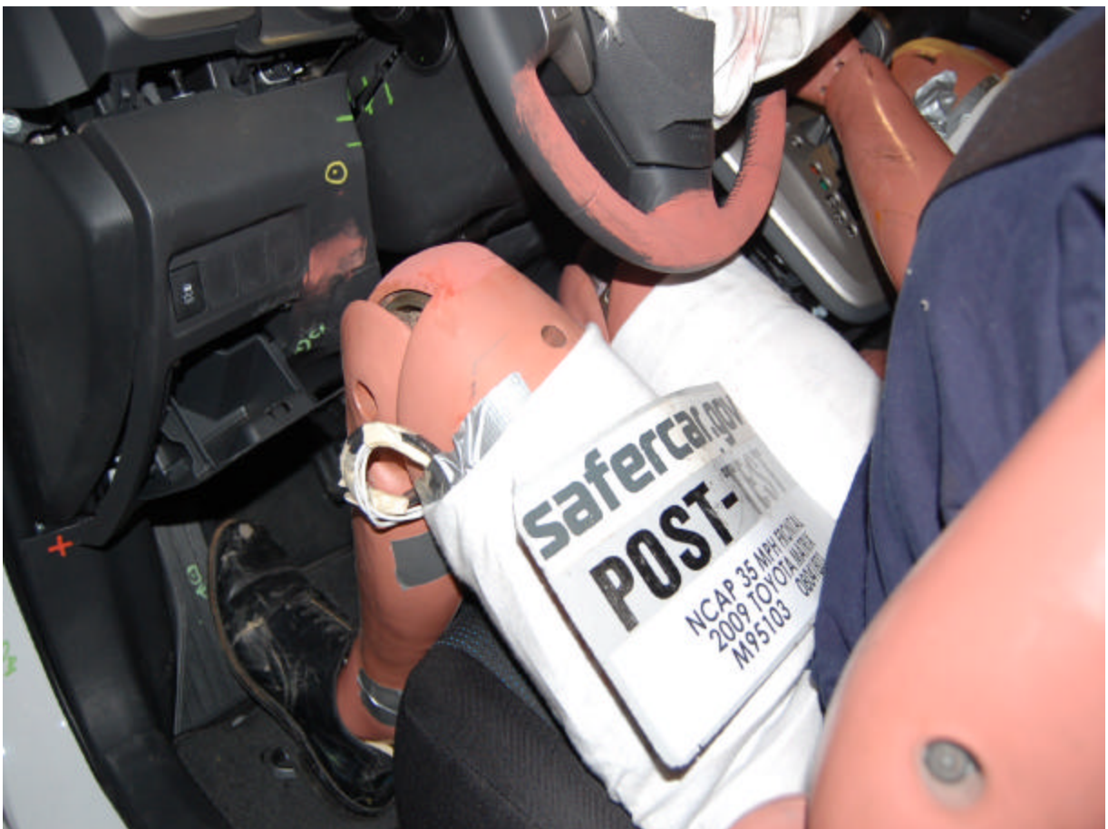
Post-Test Driver Side Knee Bolster
