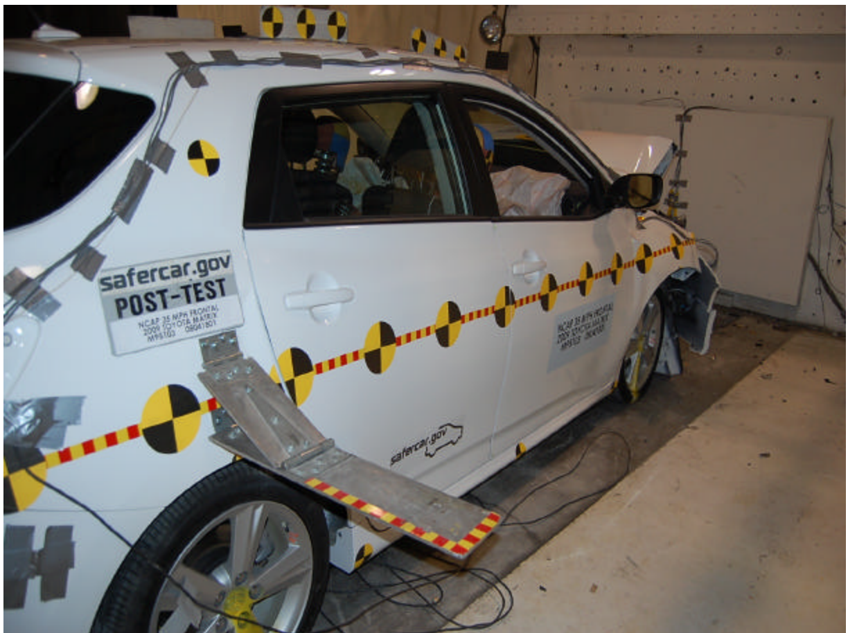
Post-Test Right Side 3/4 View of Doors After Impact
