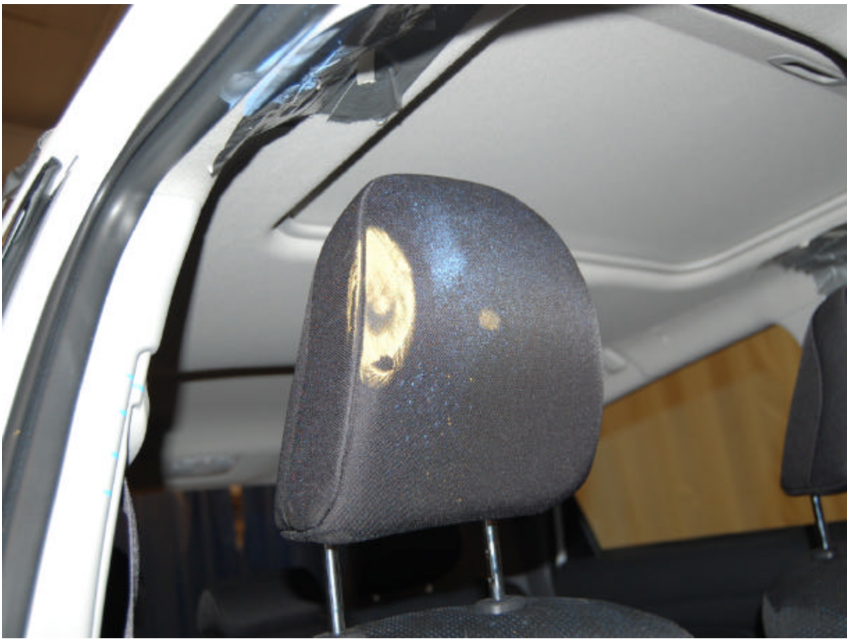
Post-Test Passenger Dummy Head Contact (Headrest)
