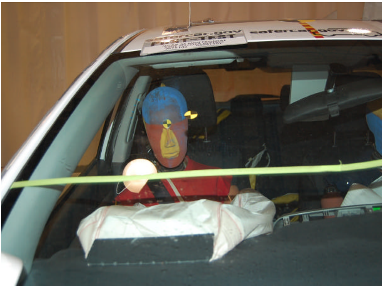
Post-Test Passenger Dummy Front View (Head Position)
