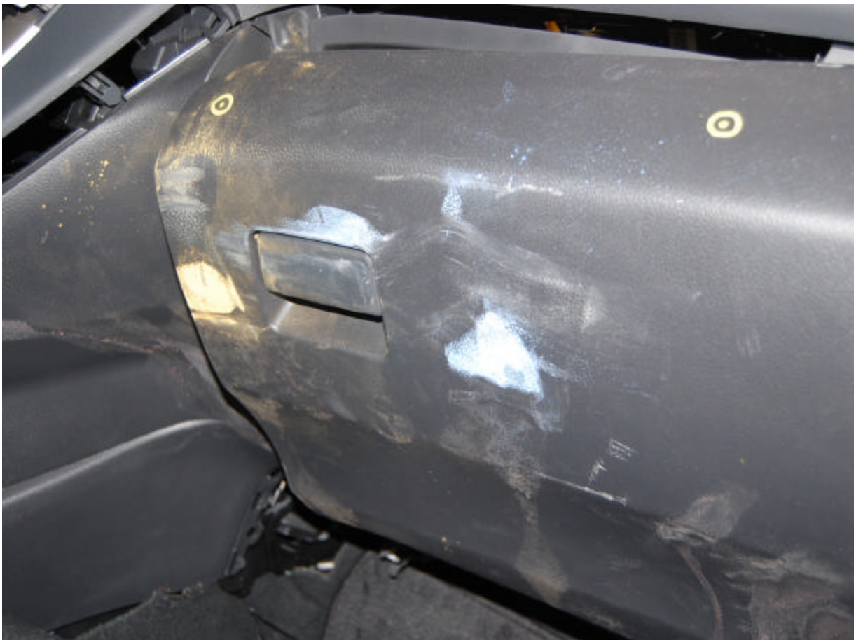
Post-Test Passenger Dummy Knee Contact
