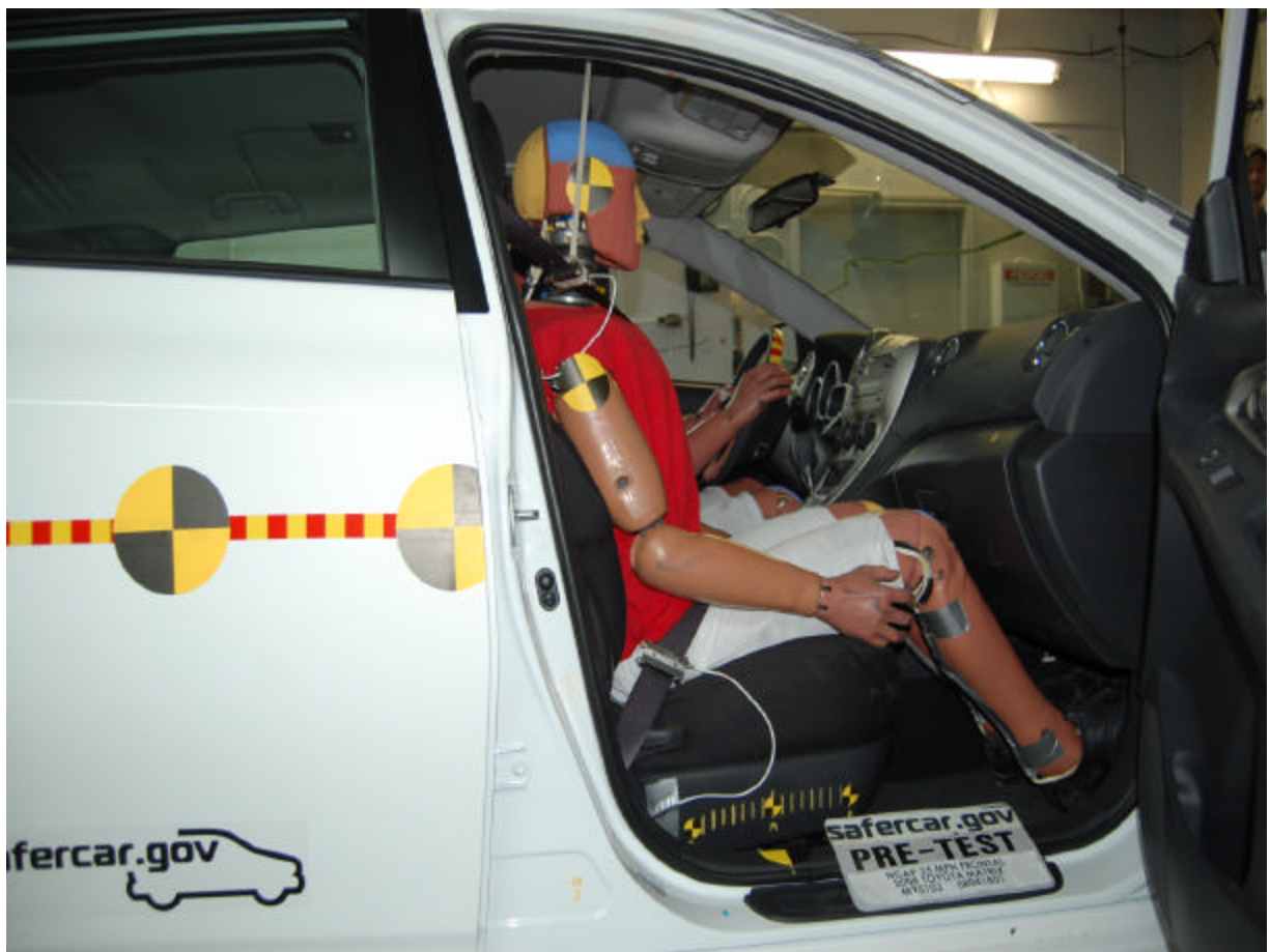
Pre-Test Passenger Dummy (Door Open)
