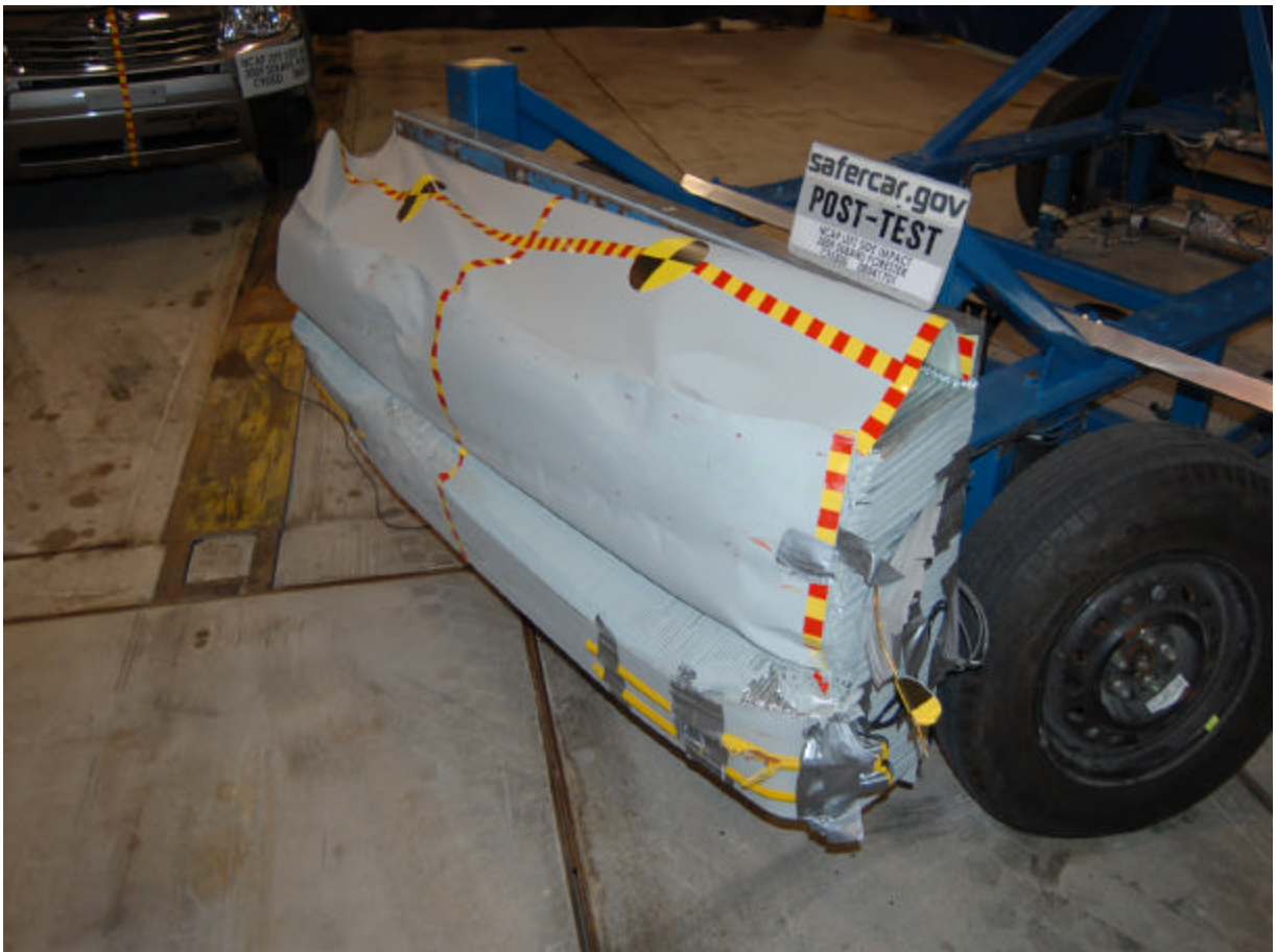
Post-Test Left Side View of Deformable Barrier
