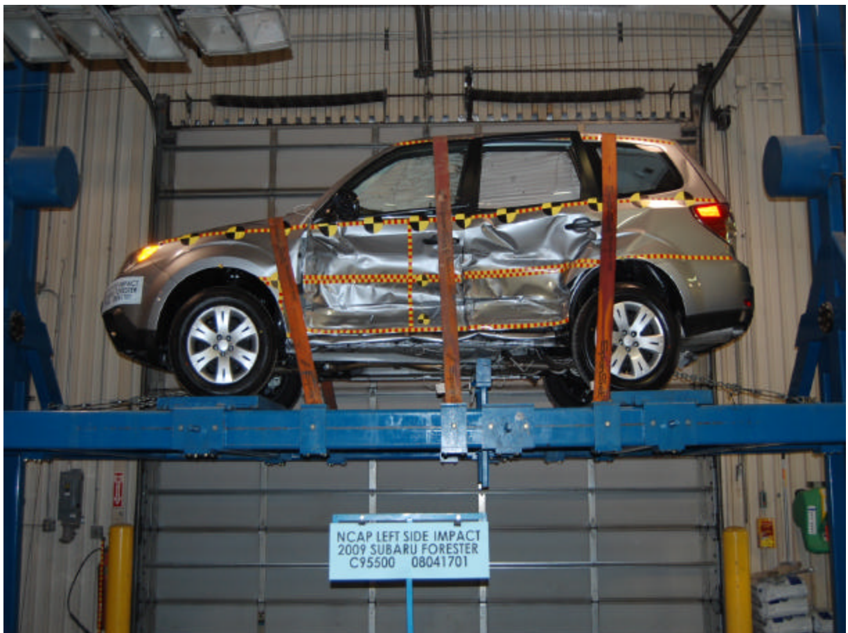
Vehicle on Rollover Device (360 Degrees)
