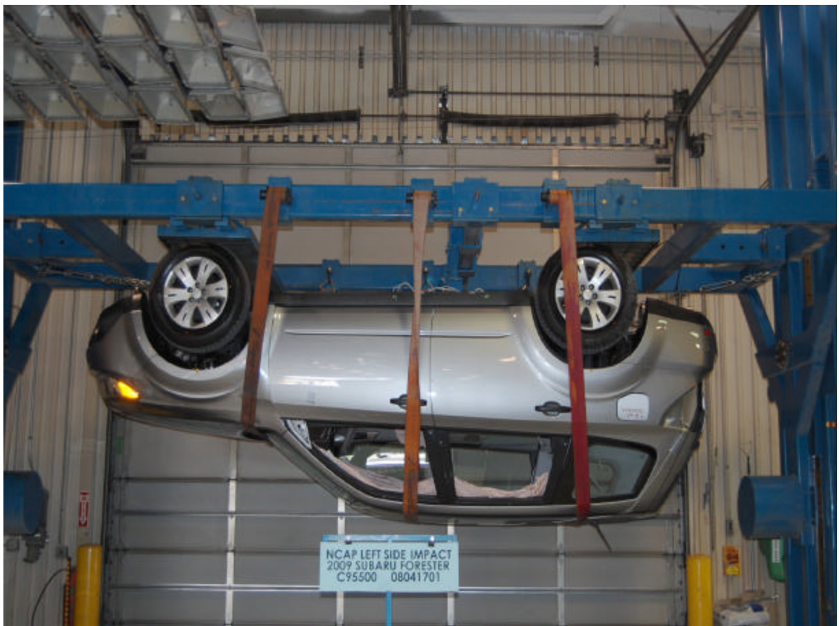
Vehicle on Rollover Device (180 Degrees)
