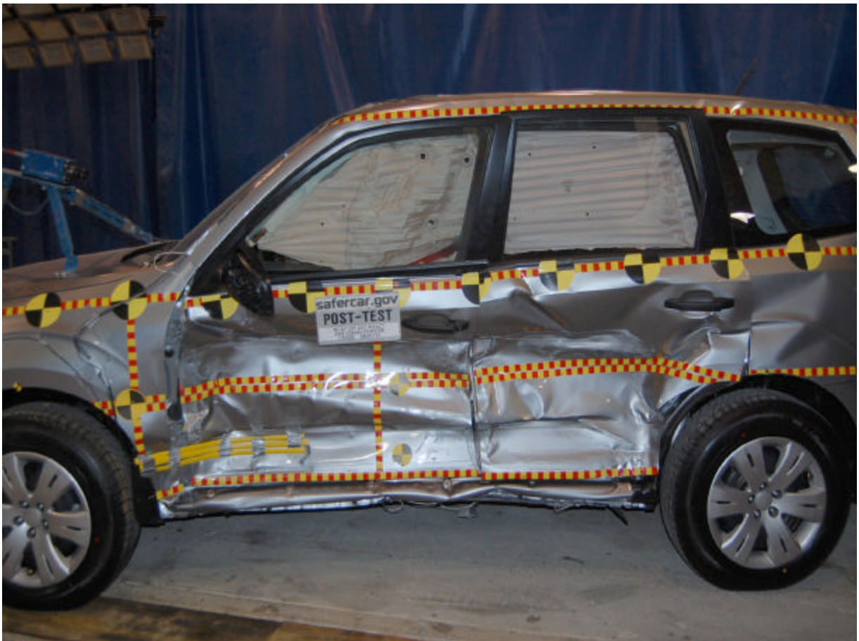
Post-Test Left Side Impact Close-Up View
