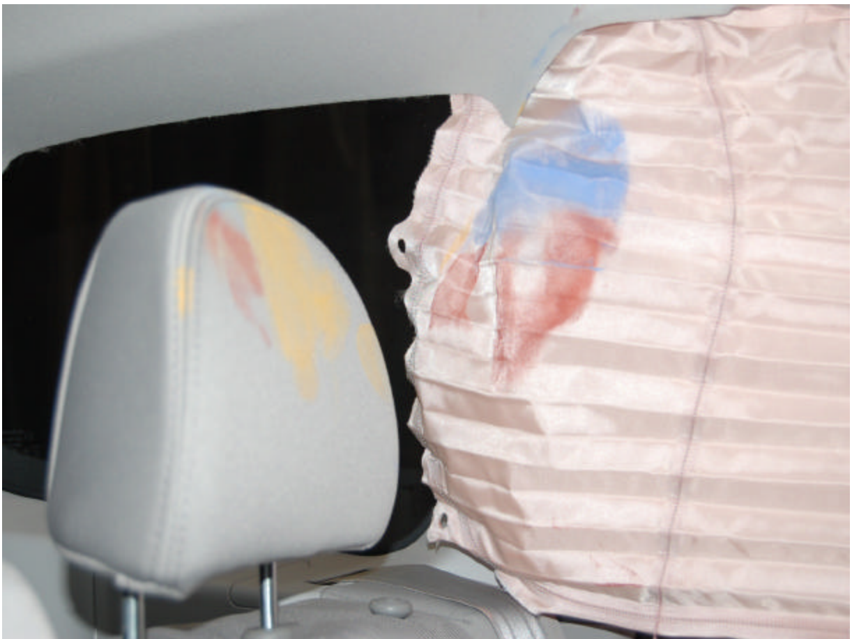
Post-Test Passenger Dummy Head Contact
