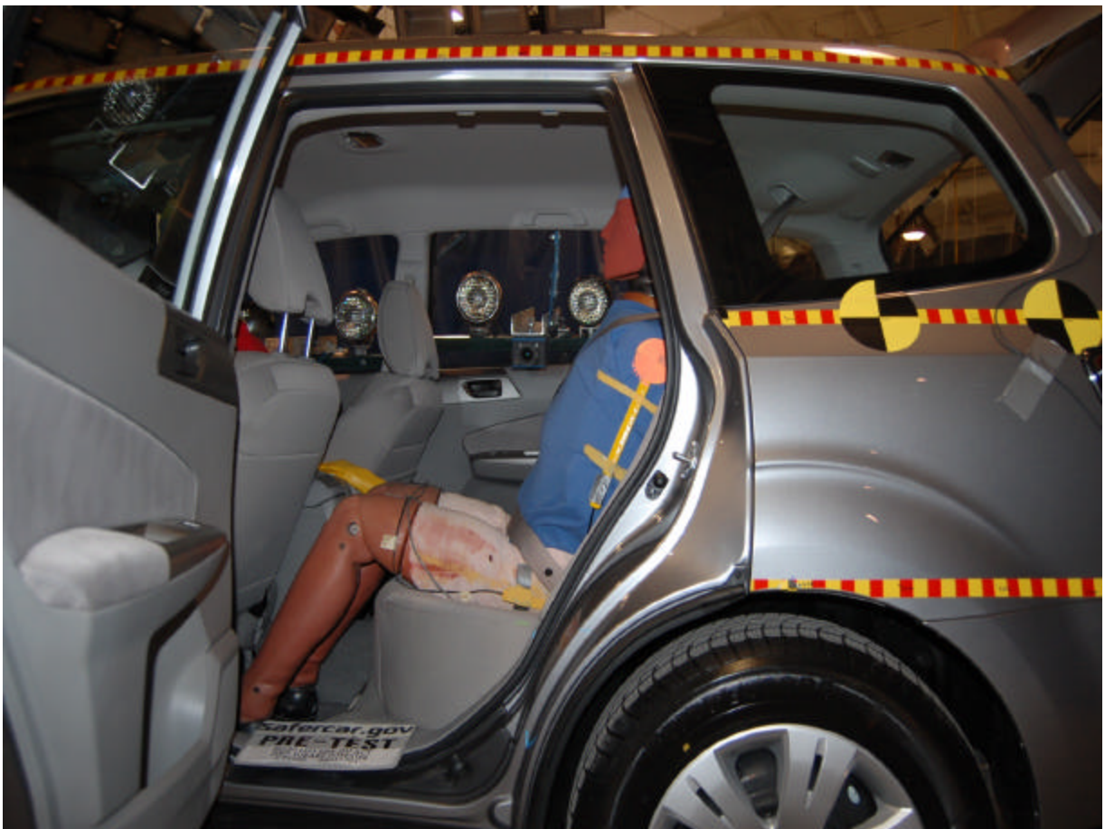
Pre-Test Passenger Dummy (Door Open)
