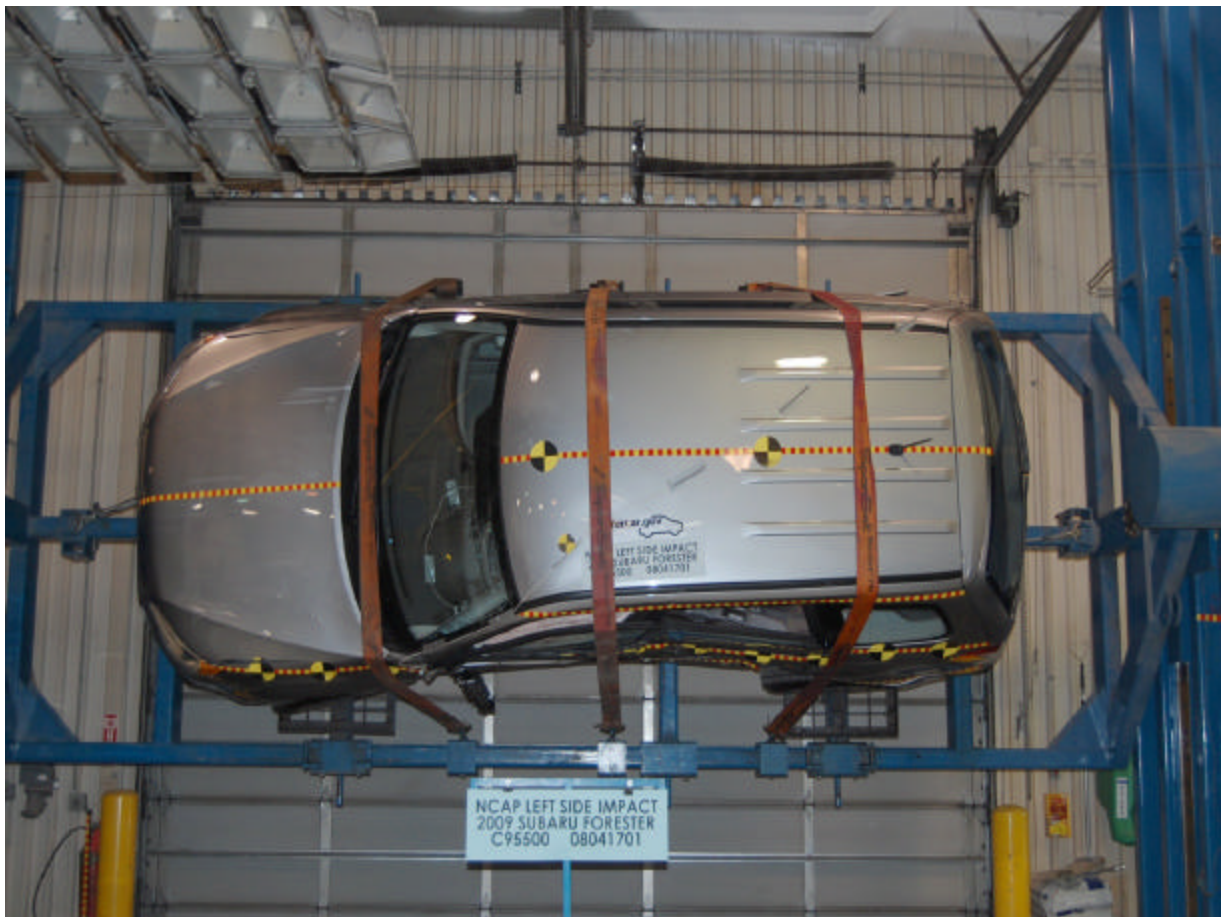
Vehicle on Rollover Device (270 Degrees)
