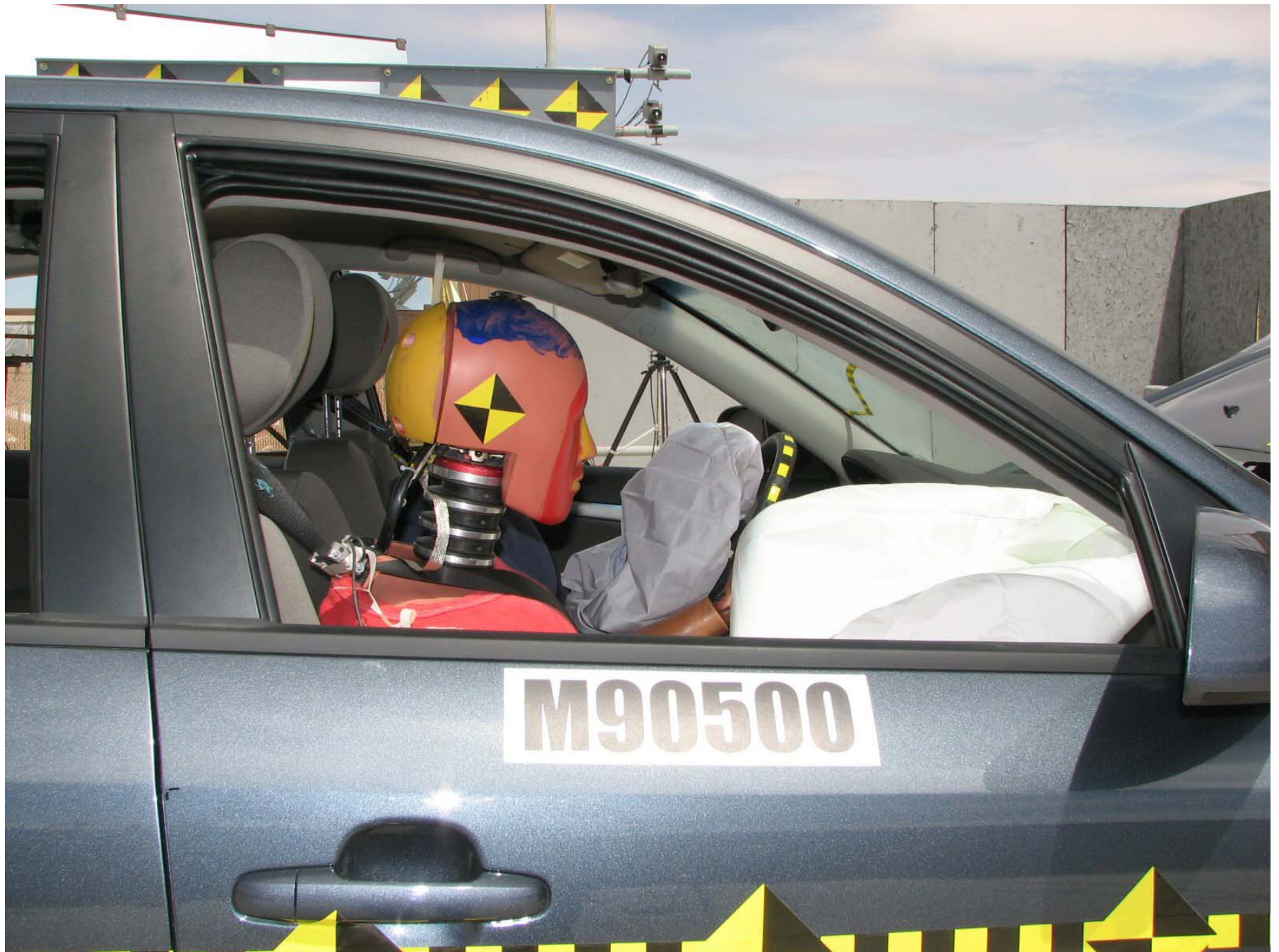
Figure A-47: Post-Test Passenger Dummy (Through Window)
