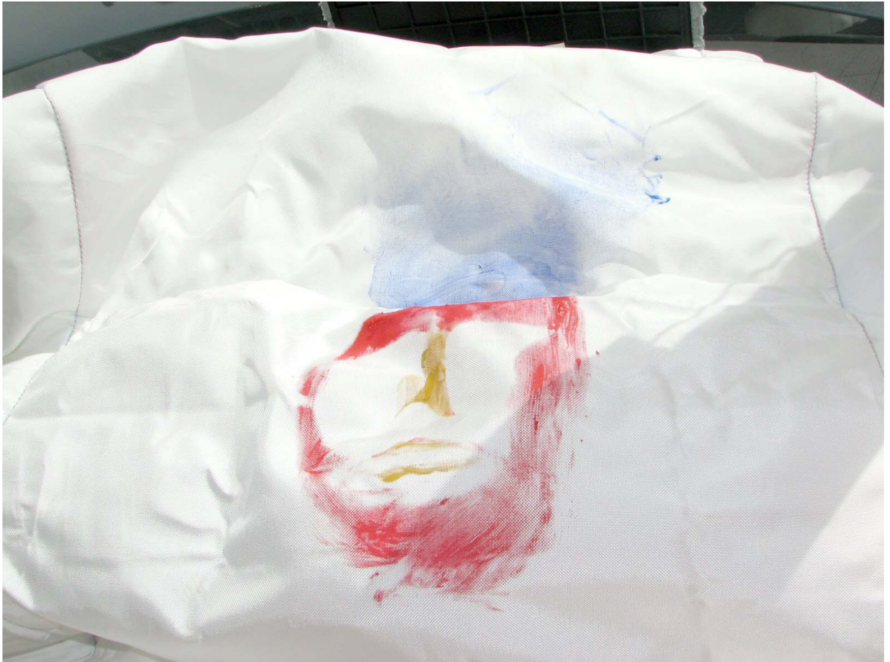
Figure A-57: Post-Test Passenger Dummy Airbag Contact
