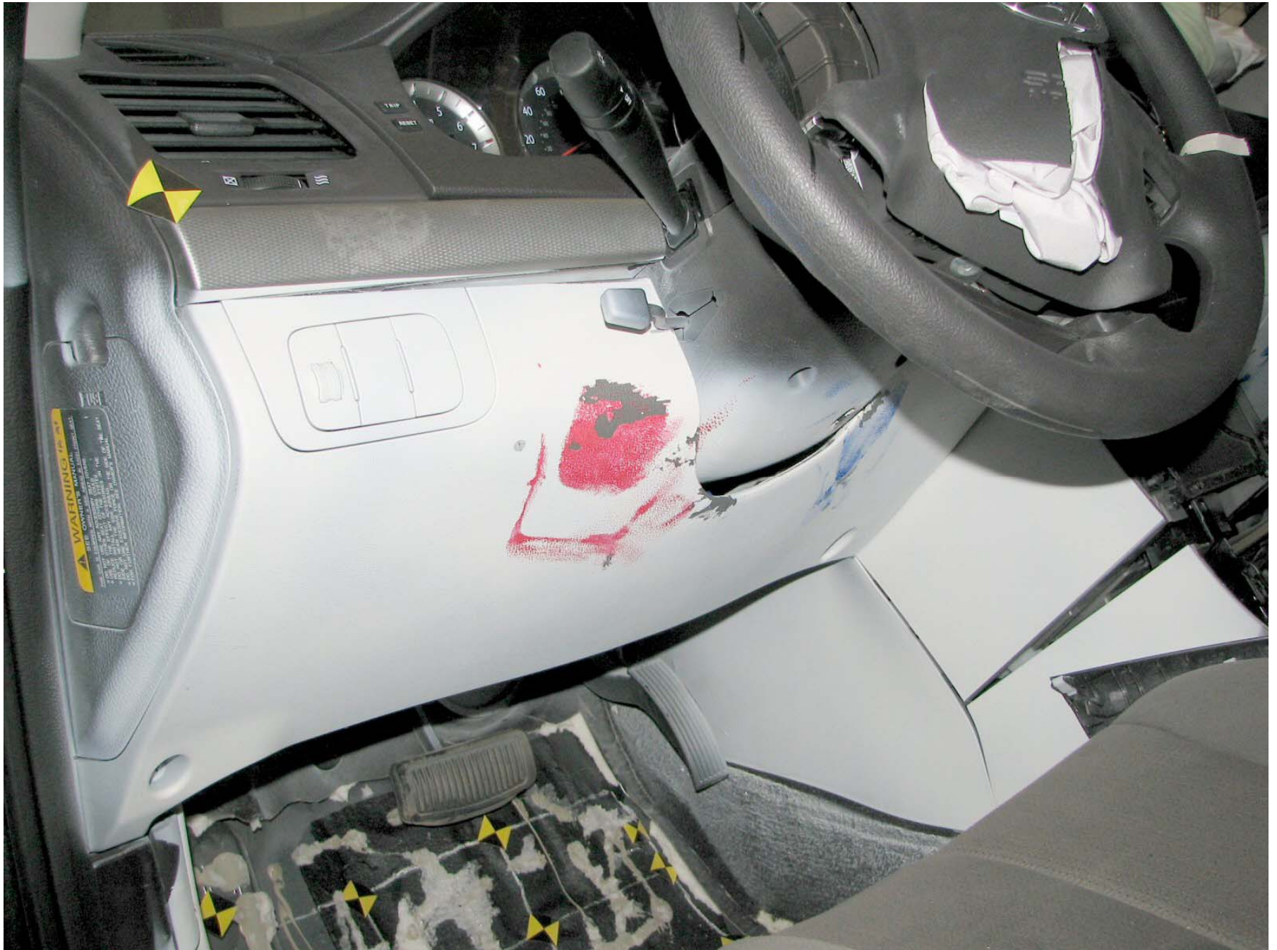
Figure A-39: Post-Test Driver Side Knee Bolster
