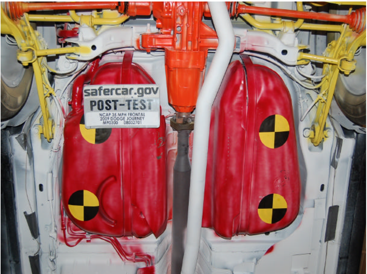
Post-Test Mid Rear Underbody View
