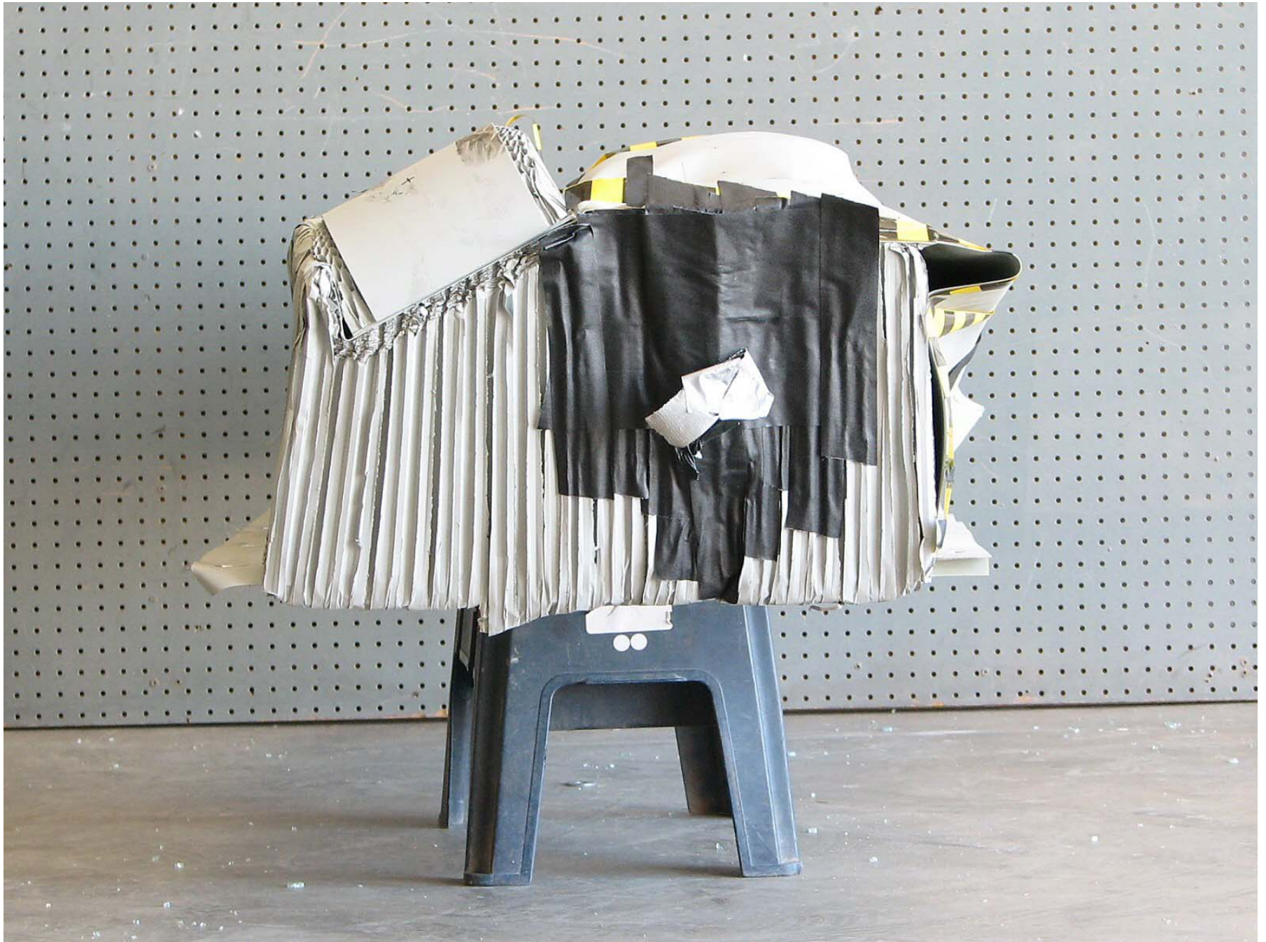
Figure A-49: Post-Test Left Side View of Deformable Barrier
