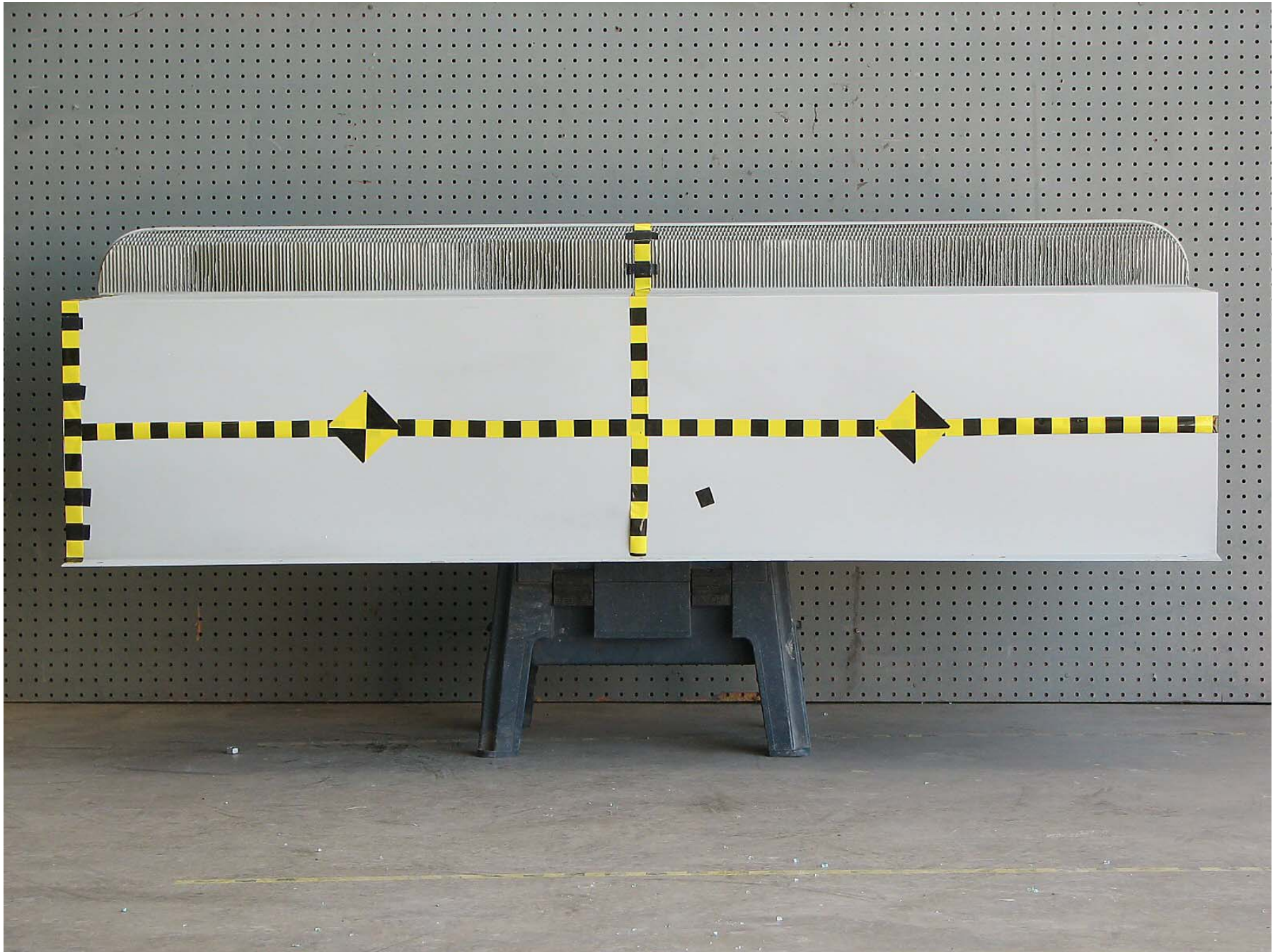
Figure A-44: Pre-Test Top View of Deformable Barrier
