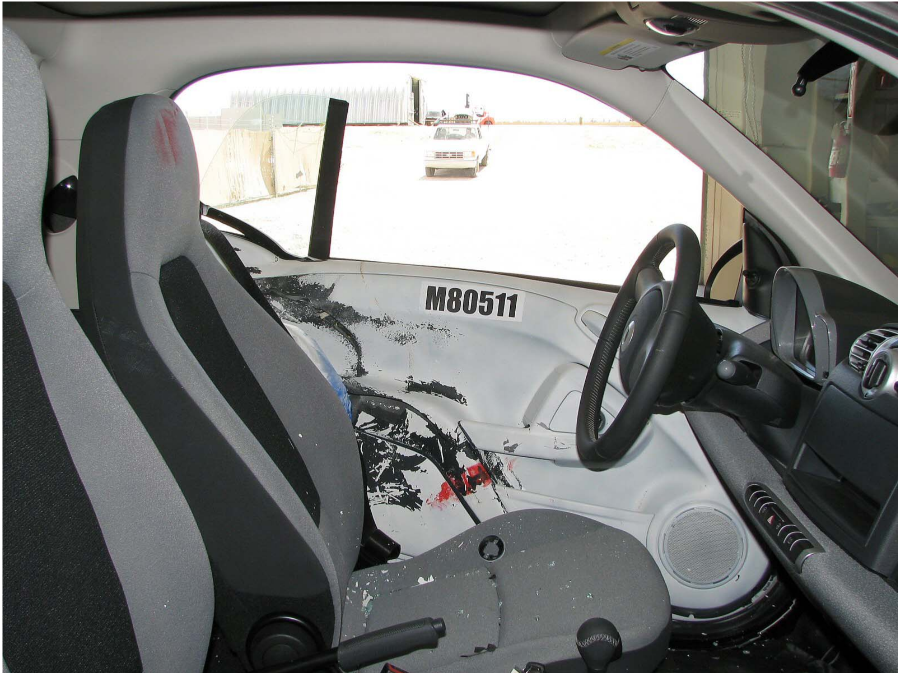
Figure A-41: Post-Test Front Door Panel (Interior)
