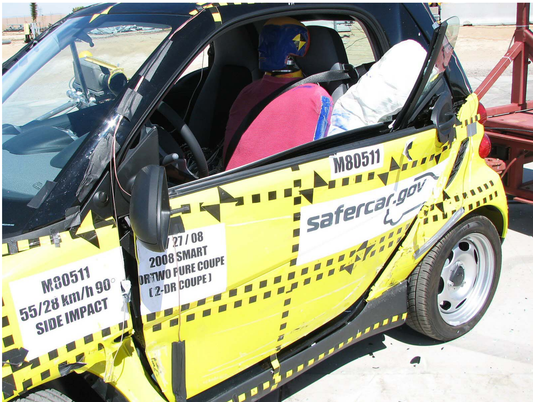
Figure A-28: Post-Test Front \frac{3}{4} View of Left Side Door
