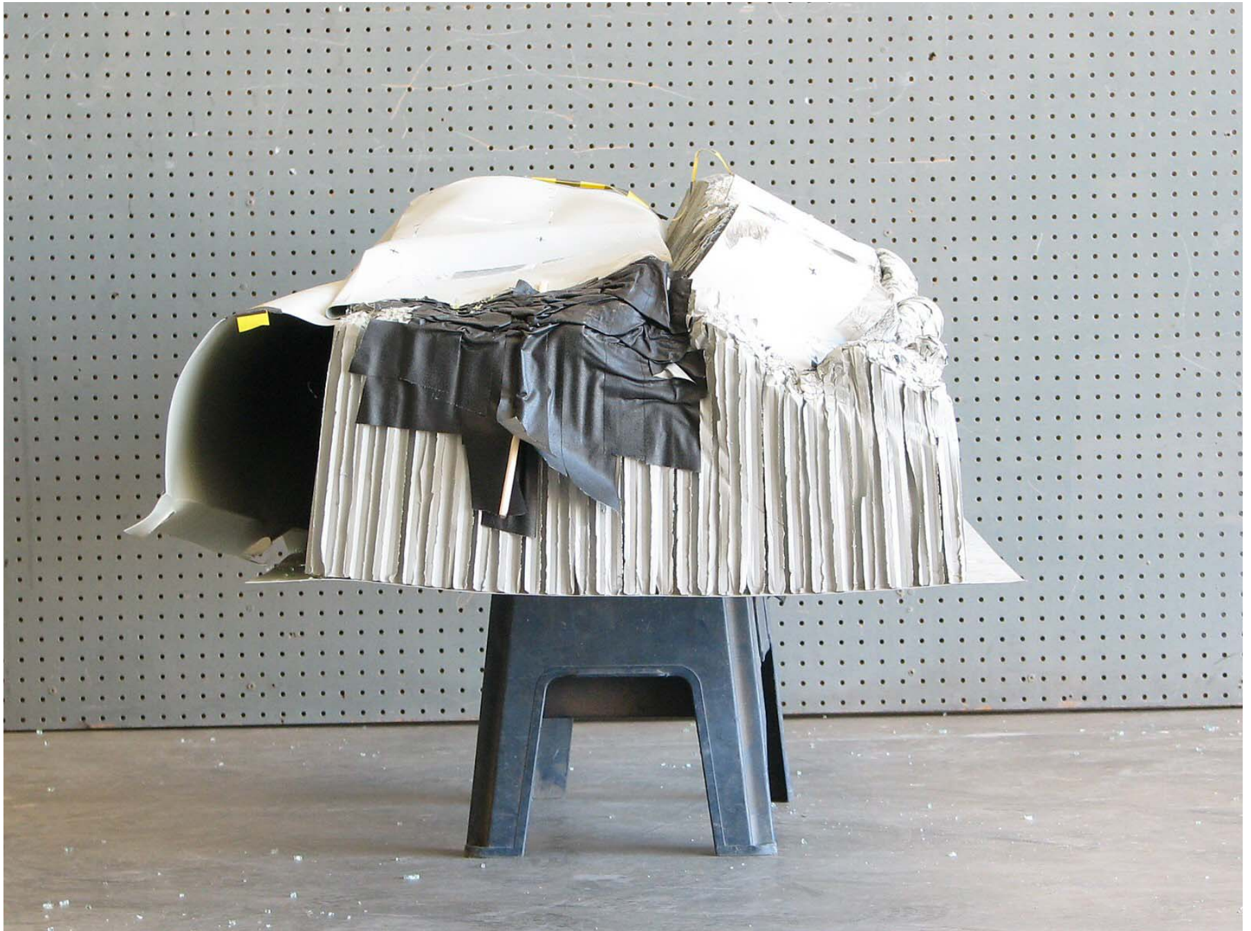
Figure A-47: Post-Test Right Side View of Deformable Barrier
