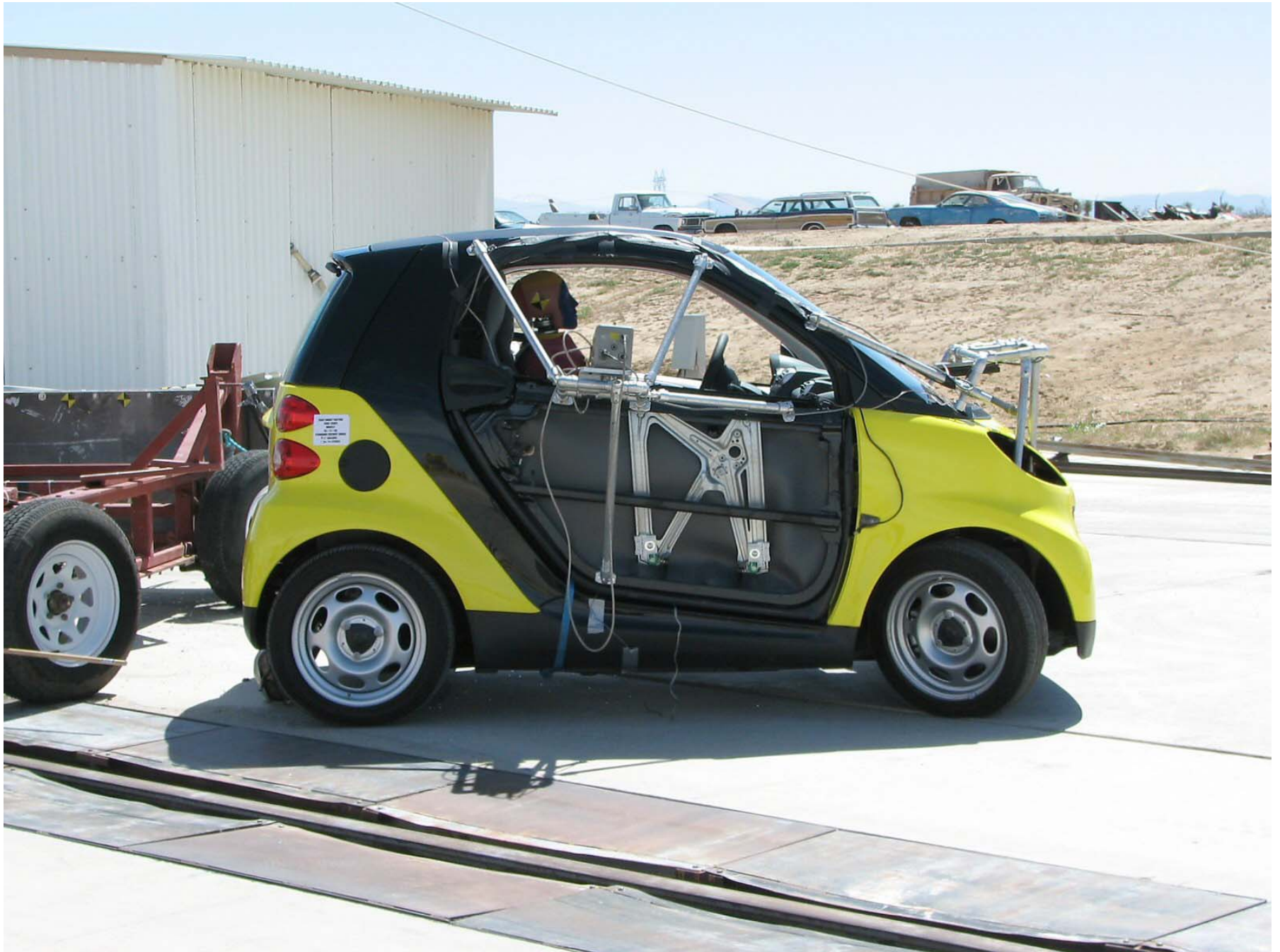
Figure A-18: Post-Test Right Side View
