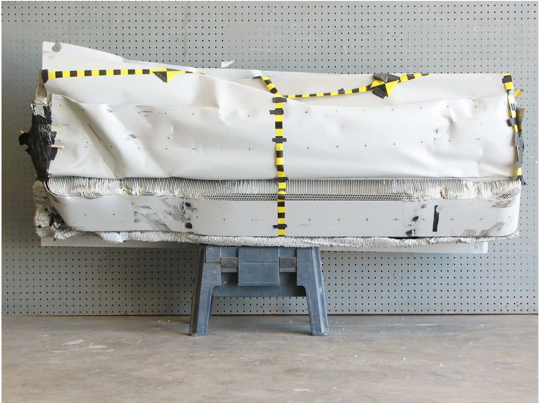
Figure A-43: Post-Test Front View of Deformable Barrier
