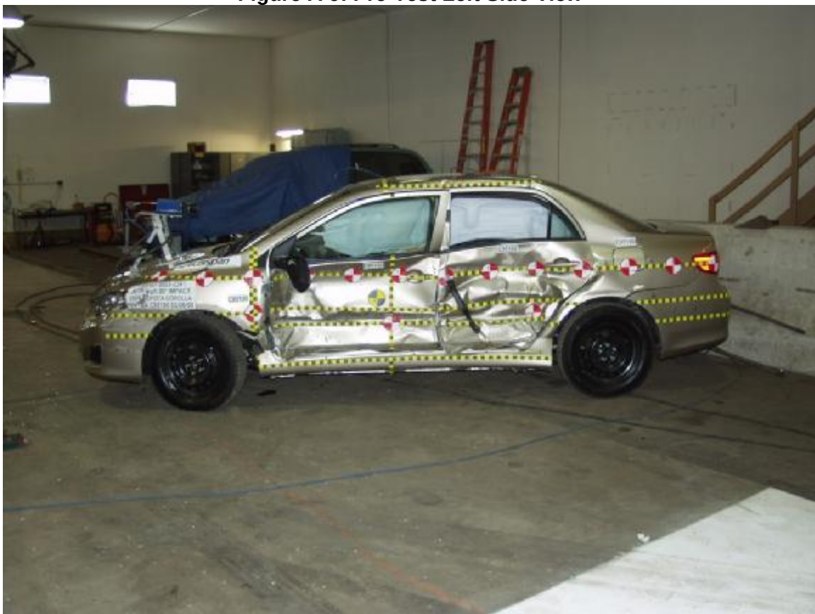
Figure A-10: Post-Test Left Side View
