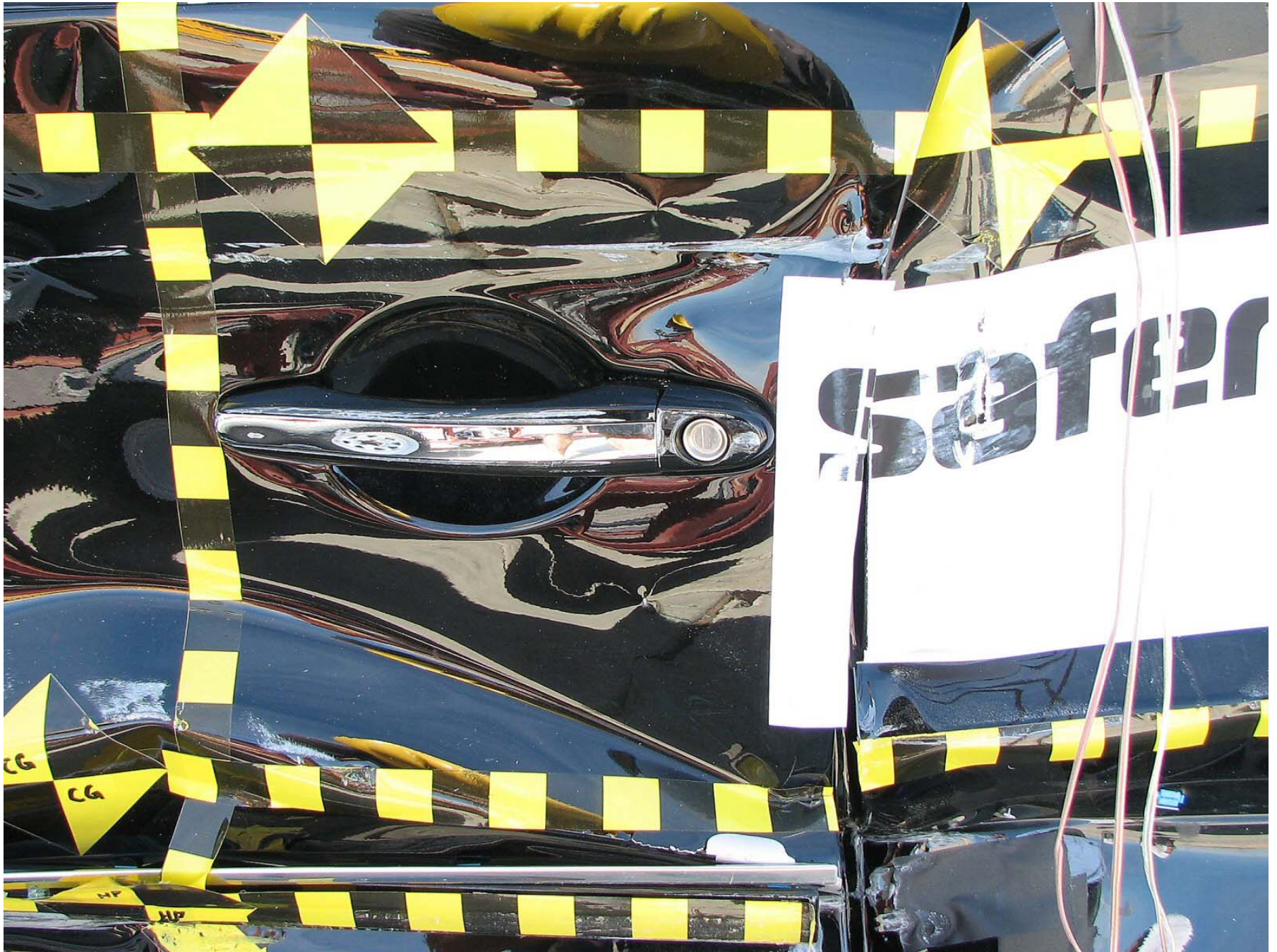
Figure A-32: Post-Test Left Front Door
