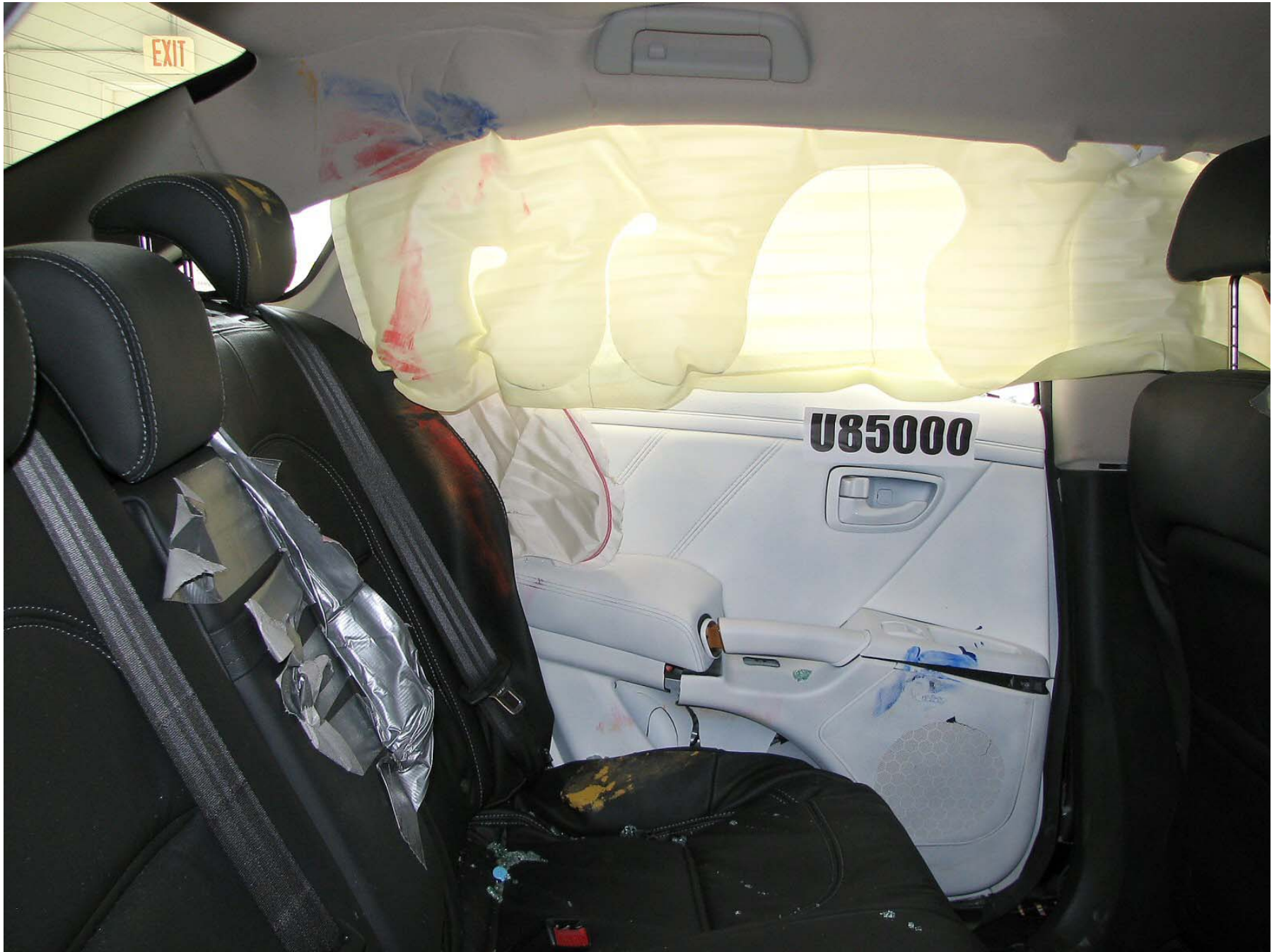
Figure A-52: Post-Test Rear Door Panel (Interior)
