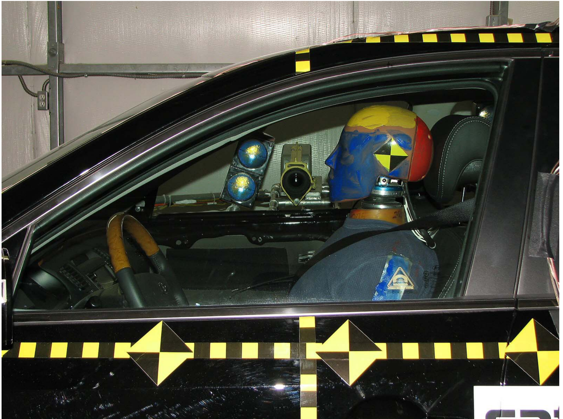
Figure A-36: Pre-Test Driver Dummy (Through Window)
