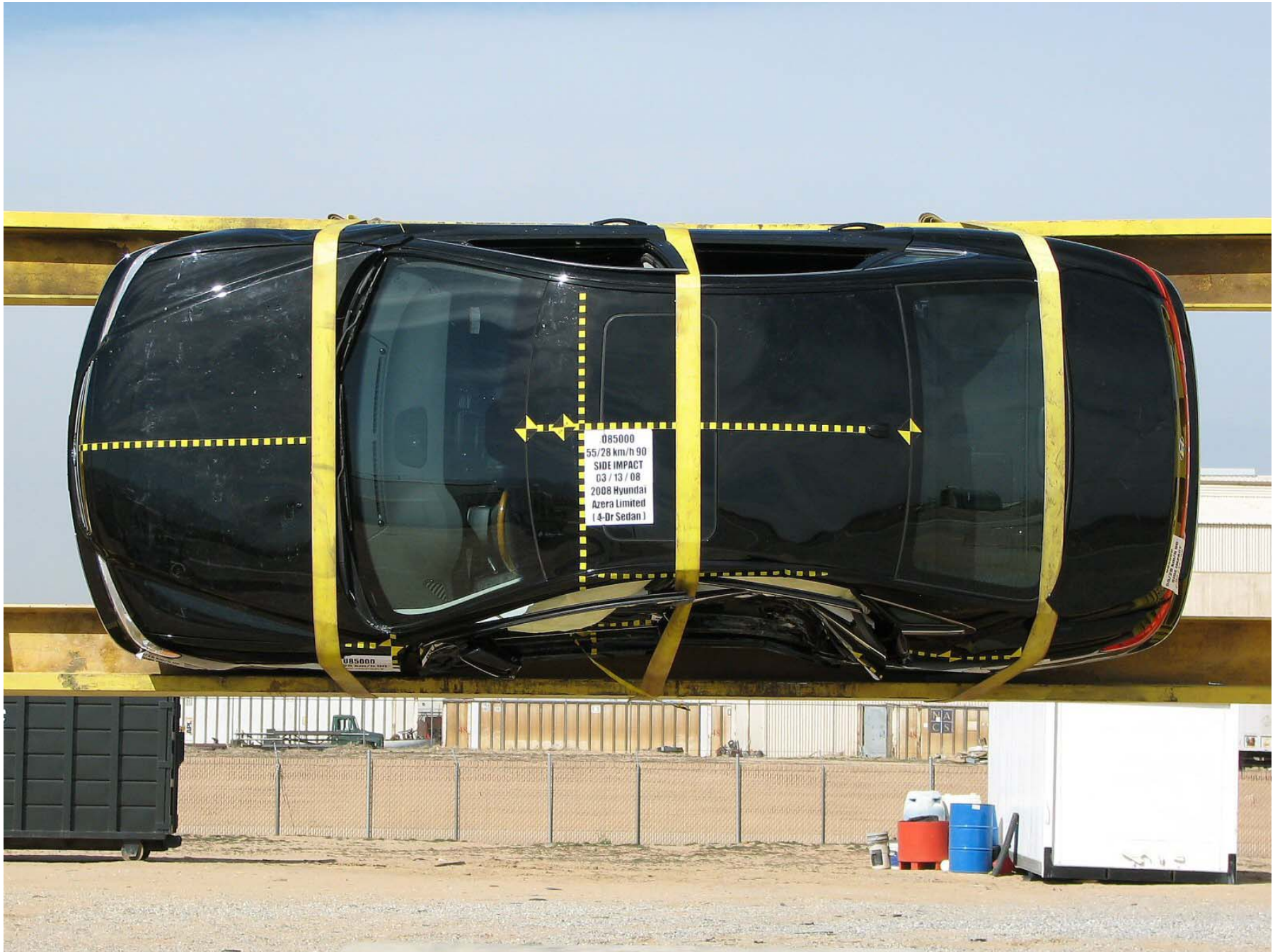
Figure A-62: Vehicle on Rollover Device (90°)
