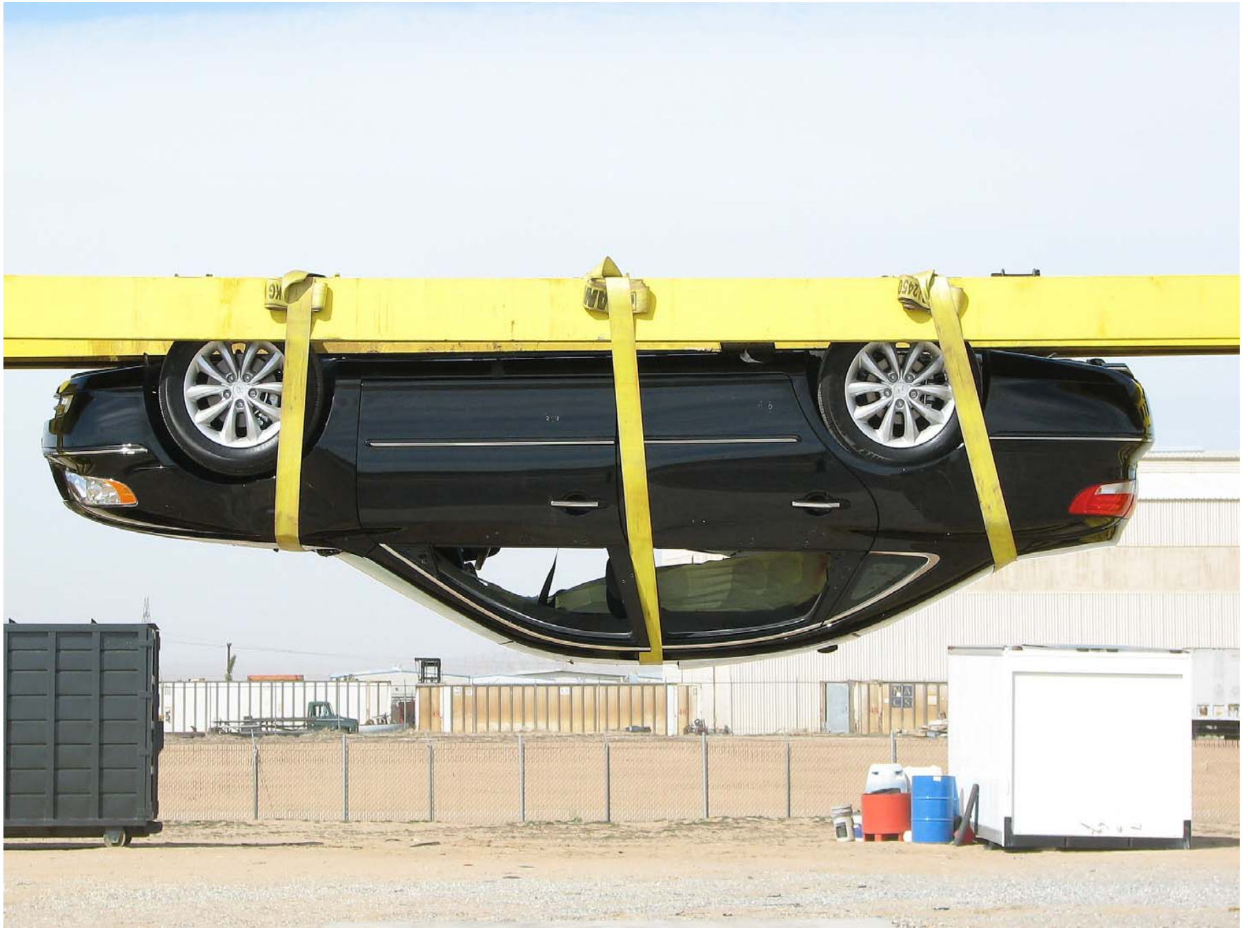
Figure A-63: Vehicle on Rollover Device (180°)
