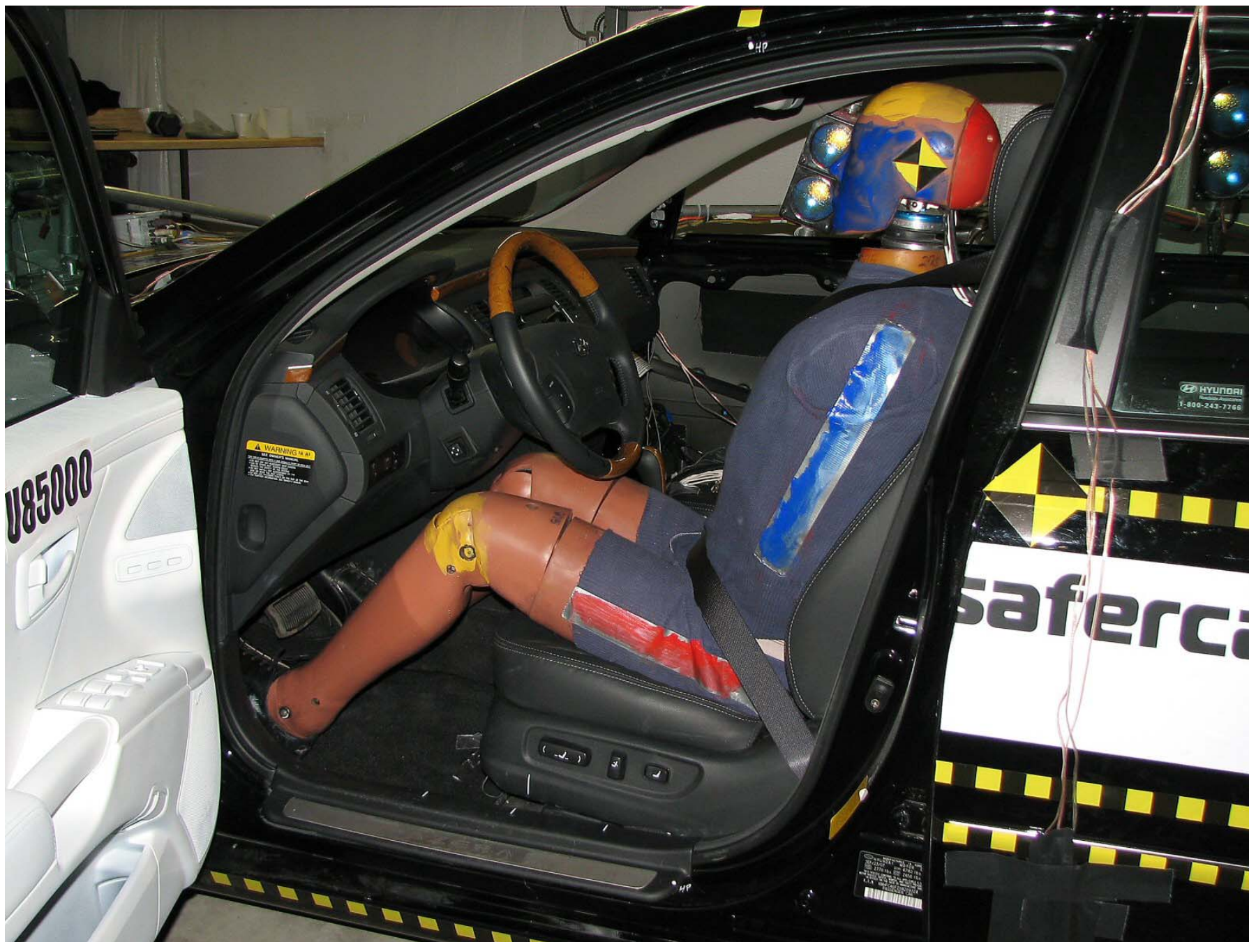
Figure A-35: Pre-Test Driver Dummy (Door Open)
