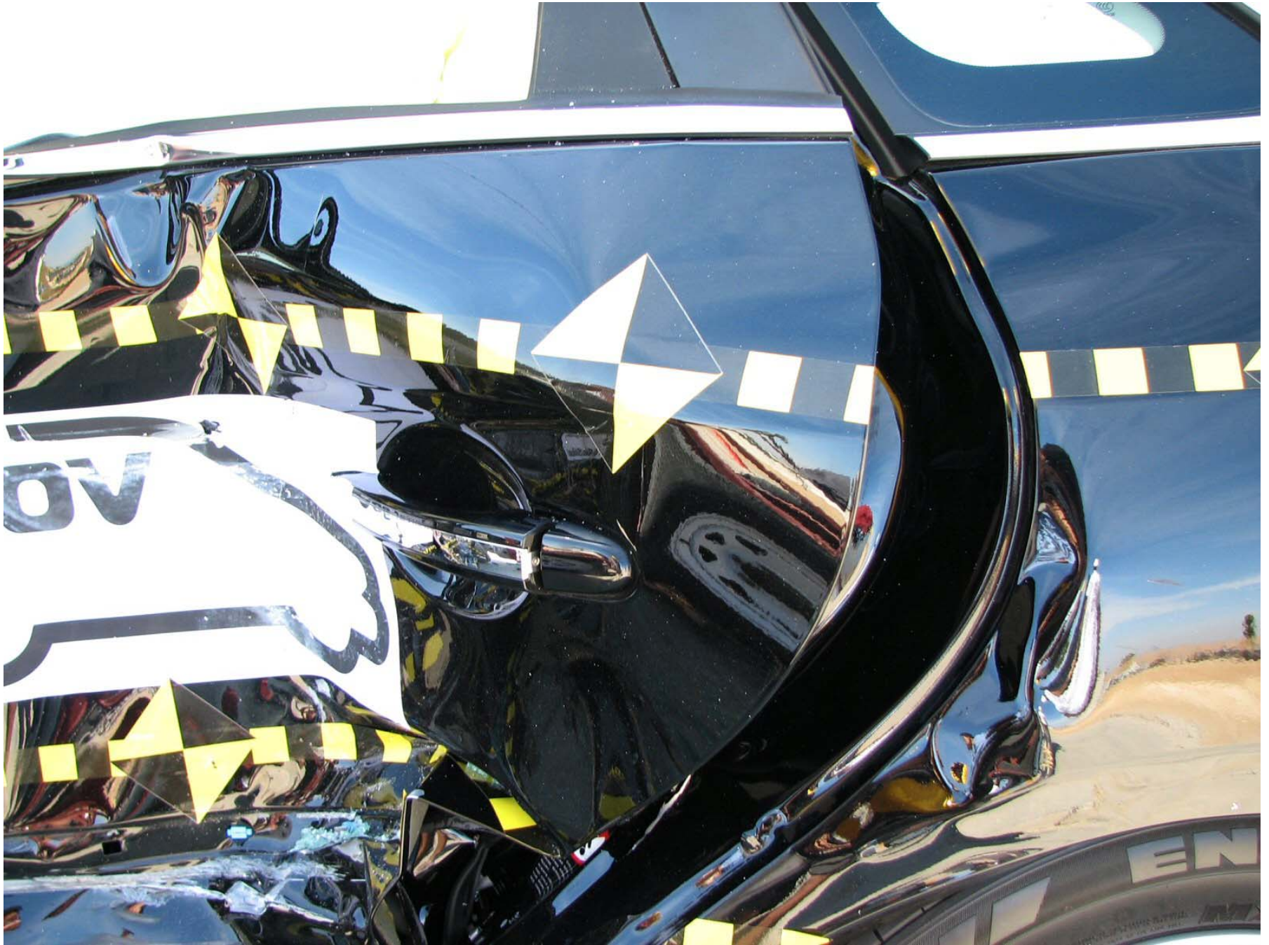
Figure A-34: Post-Test Left Rear Door
