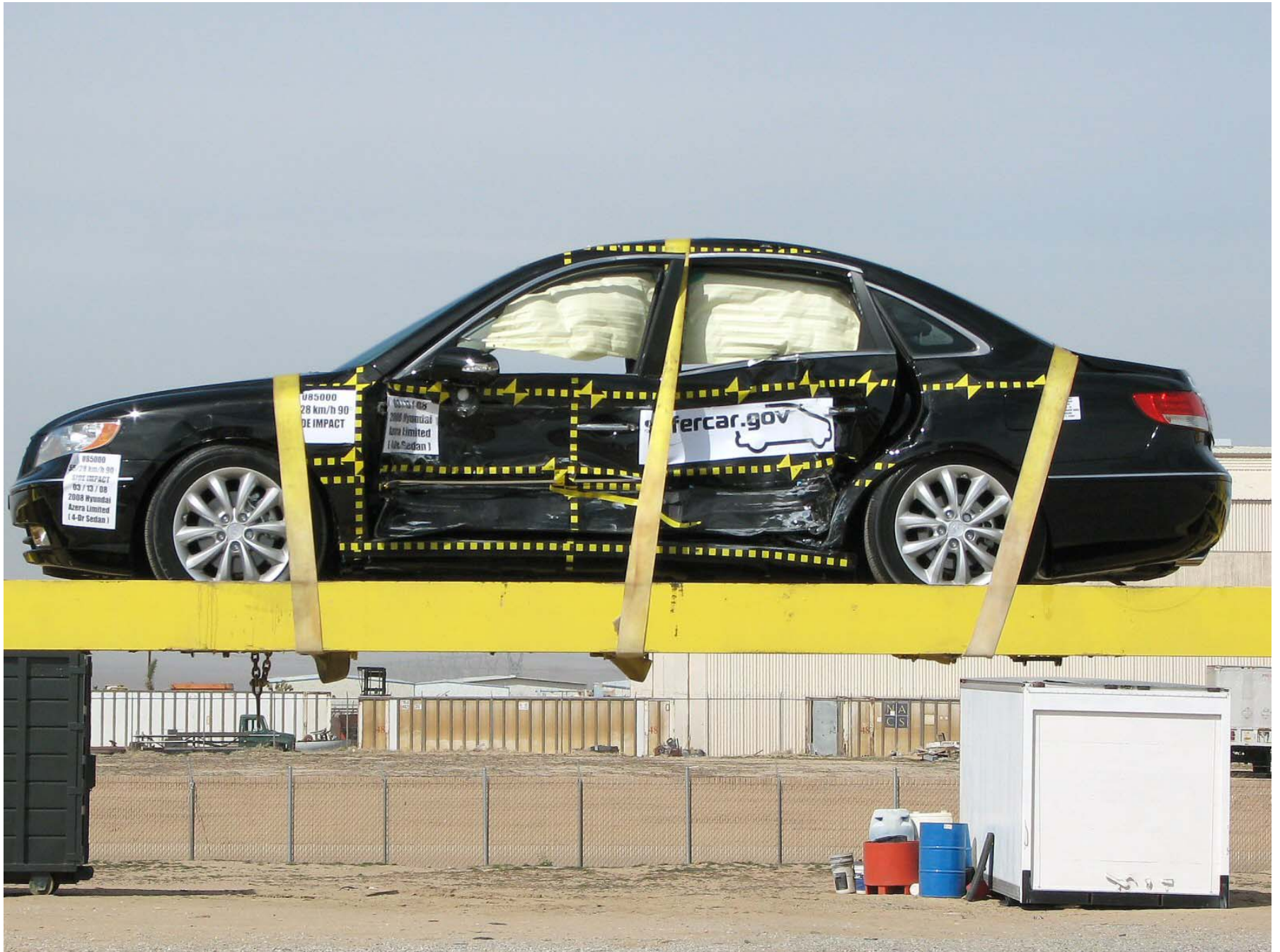
Figure A-61: Vehicle on Rollover Device (0°)
