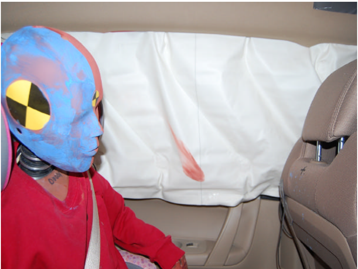
Post-Test Left Rear Passenger Dummy Head Contact View
