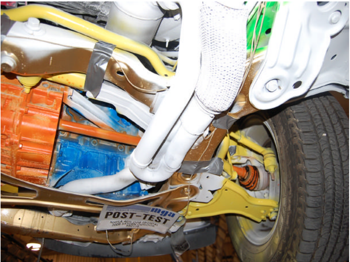
Post-Test Sway Bar Right Side View
