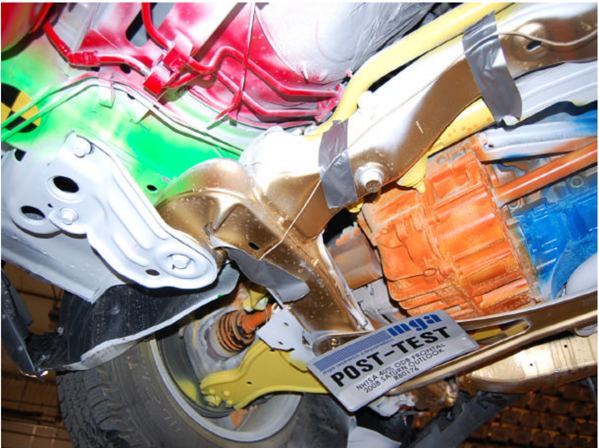
Post-Test Steering Rack \frac{3}{4} Left Side View
