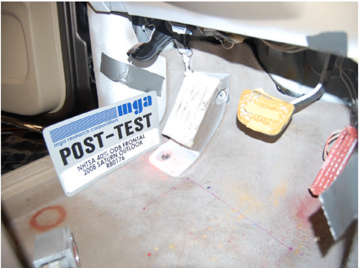
Post-Test Over Toeplan/ Floorpan Right of Seat, Seat Cushion Height
