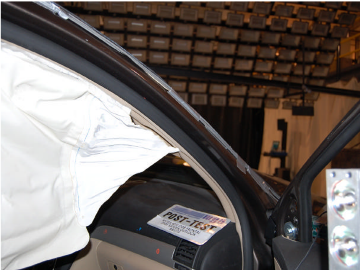
Post-Test Right Side A Pillar
