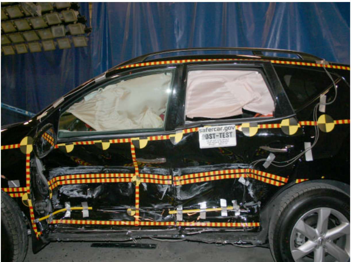
Post-Test Left Side Impact Close-up
