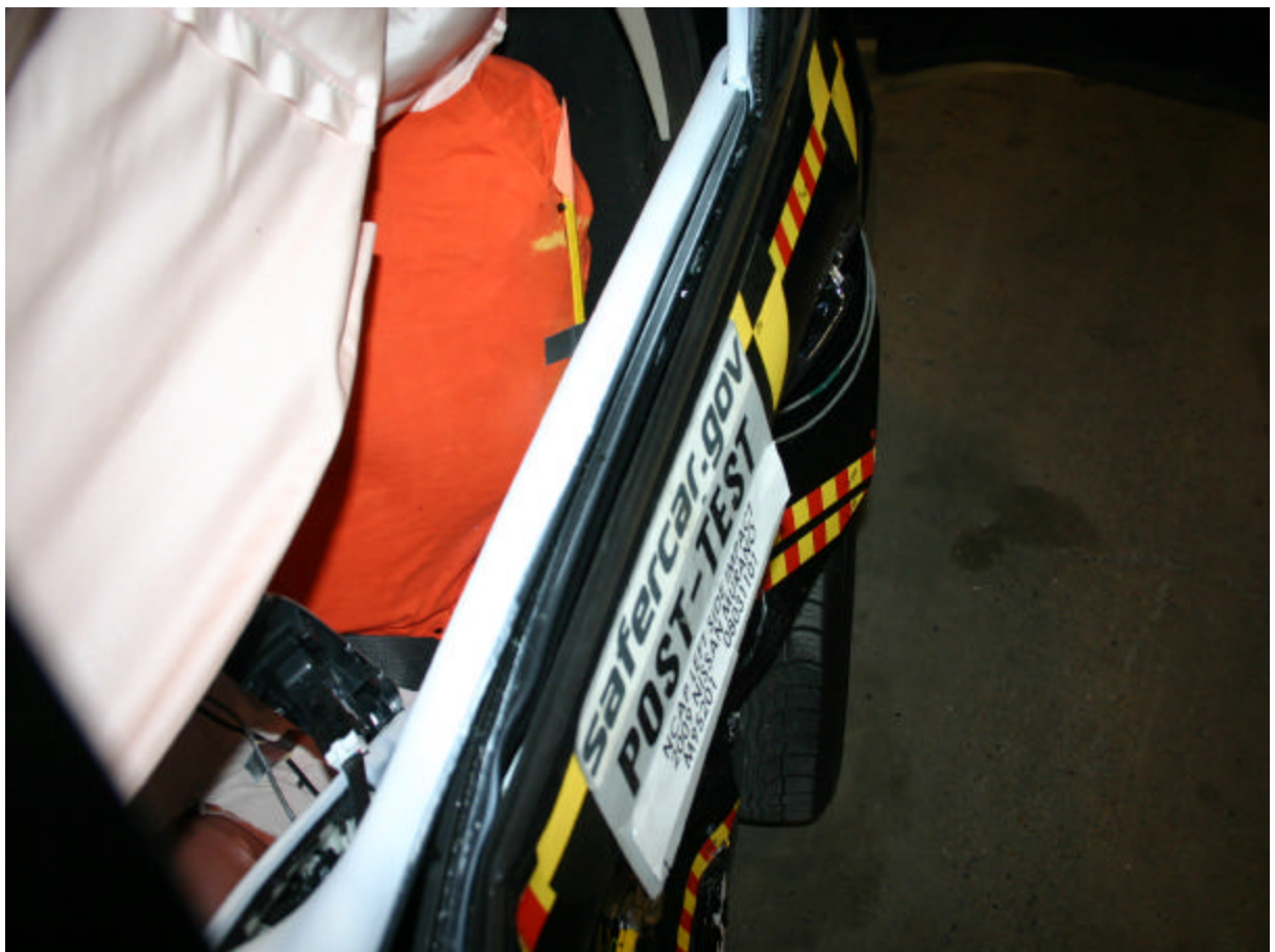
Post-Test Passenger Dummy Clearance From Door
