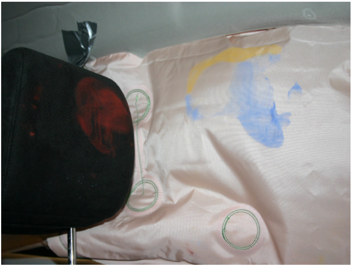
Post-Test Driver Dummy Head Contact
