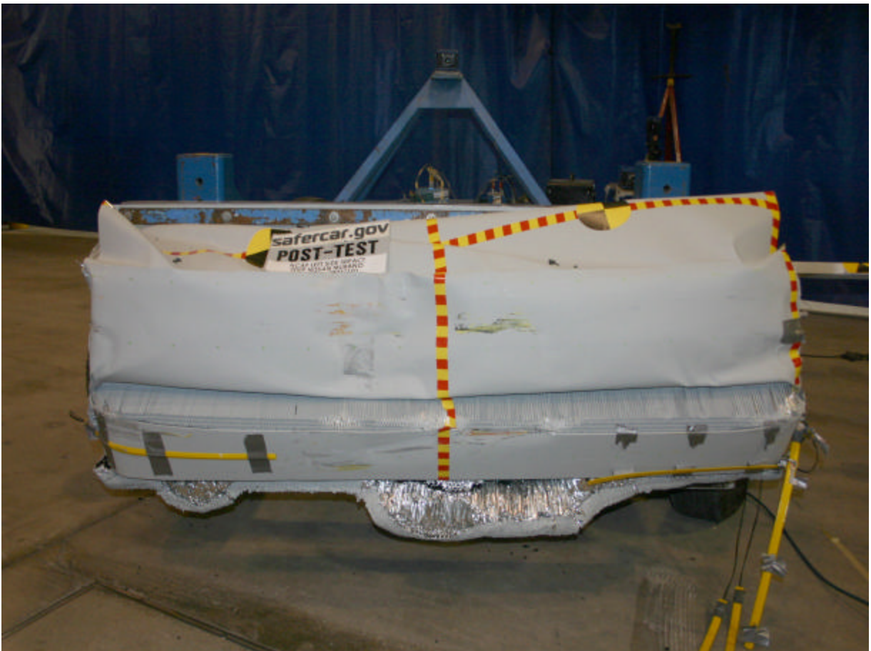
Post-Test Front View of Deformable Barrier
