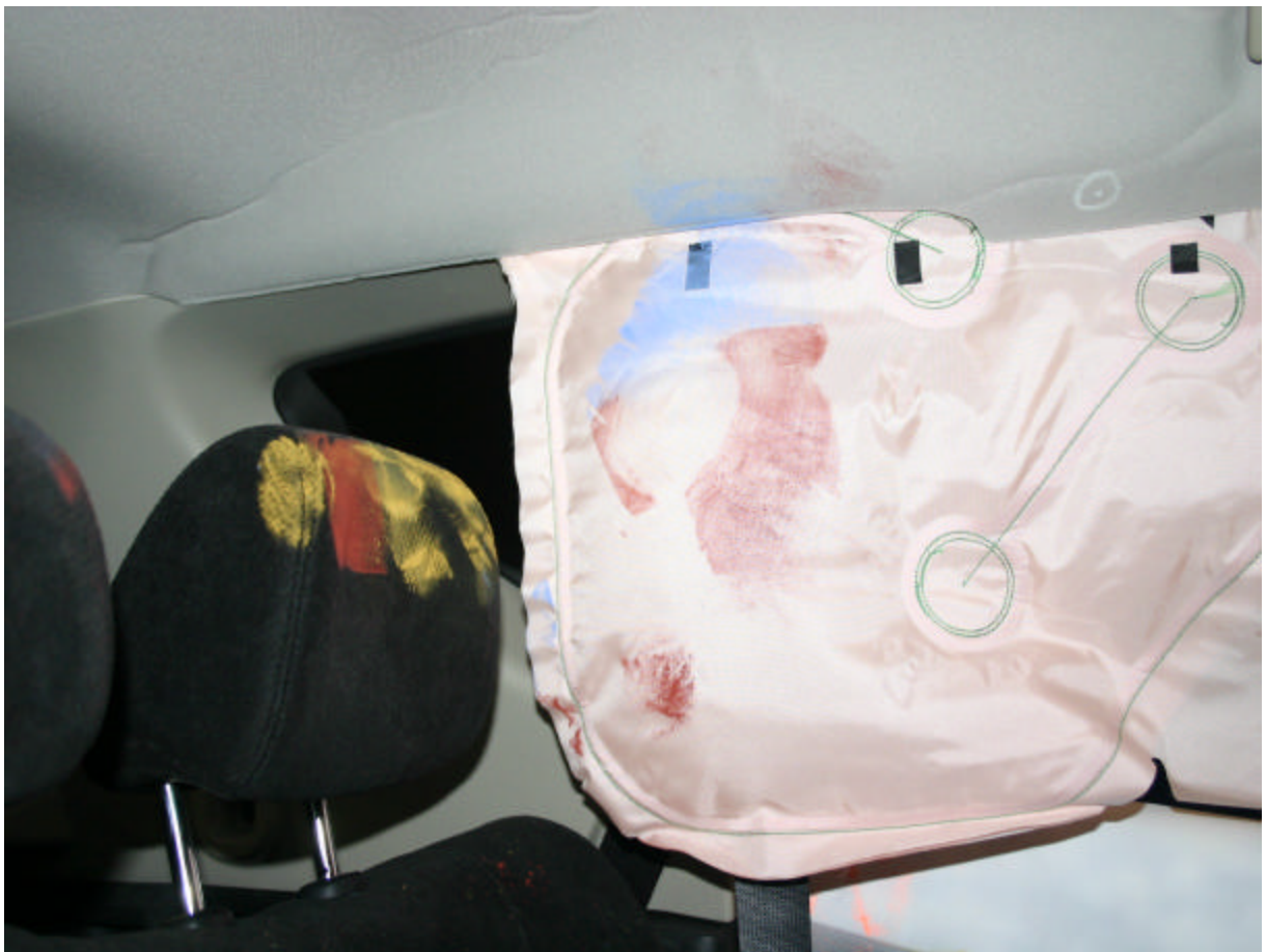
Post-Test Passenger Dummy Head Contact
