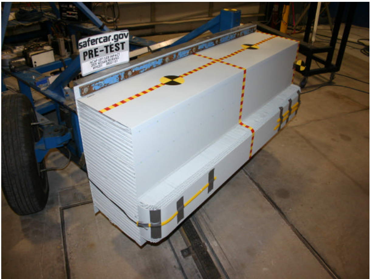
Pre-Test Right Side View of Deformable Barrier
