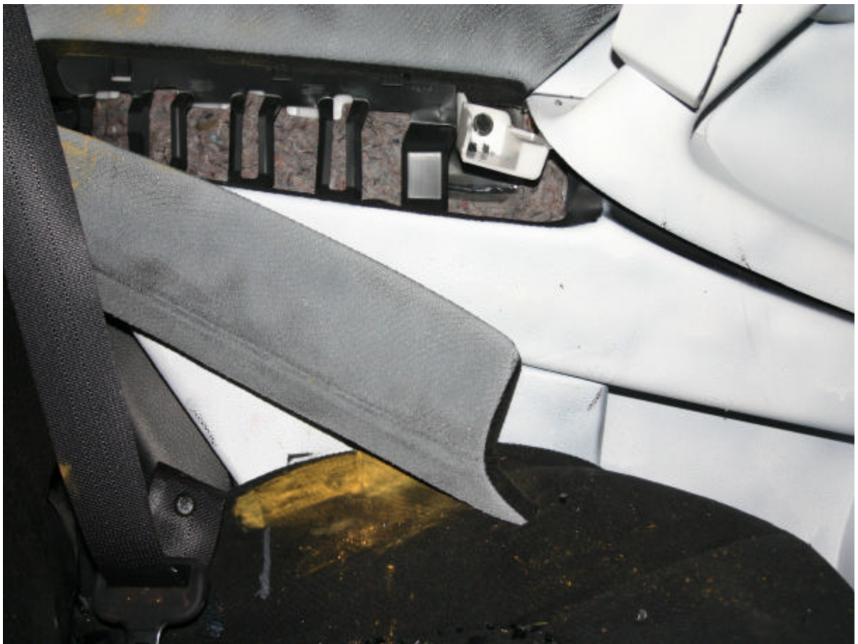
Post-Test Passenger Dummy Lower Torso Contact
