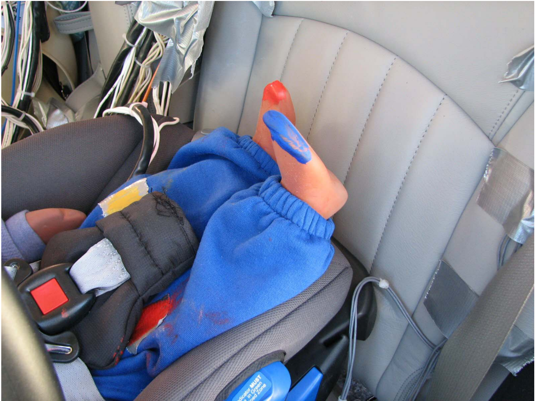
Figure D2-36: Post-Test Position 4 Dummy Legs
