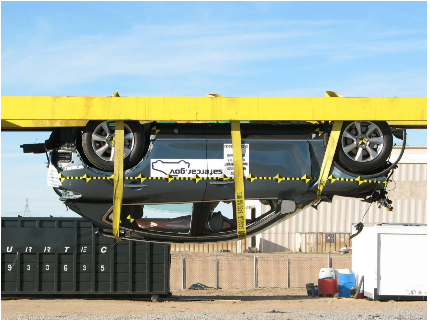
Figure A-60: Vehicle on Rollover Device (180°)
