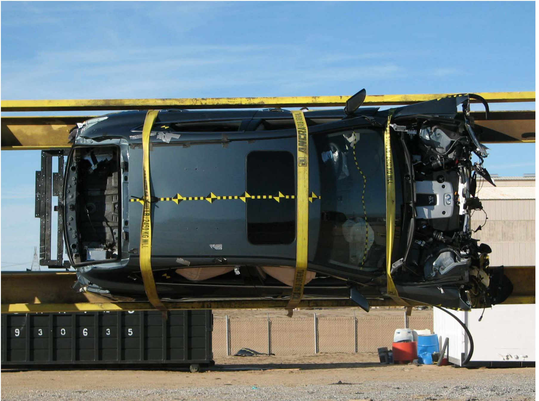
Figure A-59: Vehicle on Rollover Device (90°)
