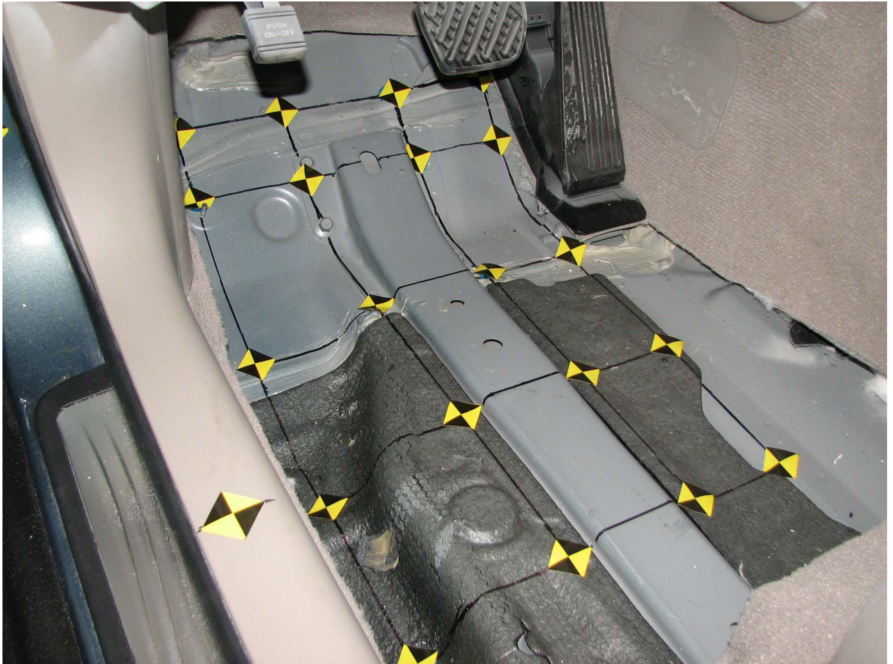
Figure A-40: Pre-Test Driver Side Floor Pan
