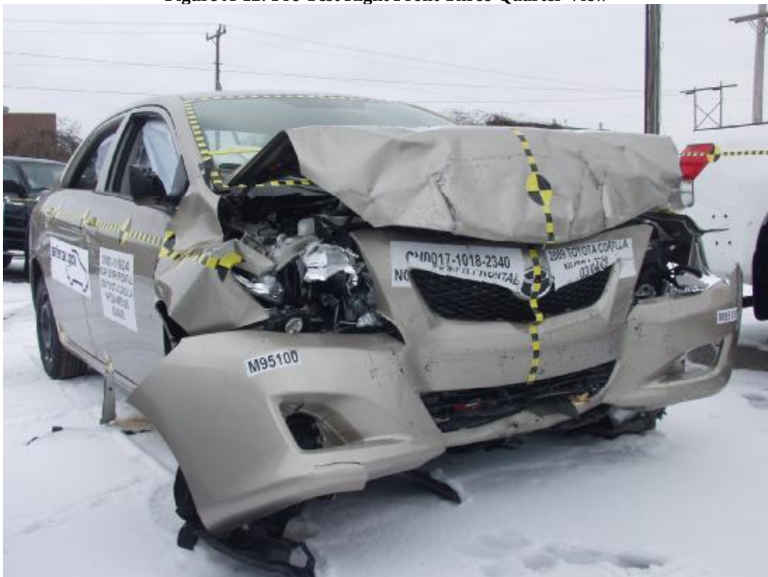
Figure A-13: Post-Test Right Front Three-Quarter View
