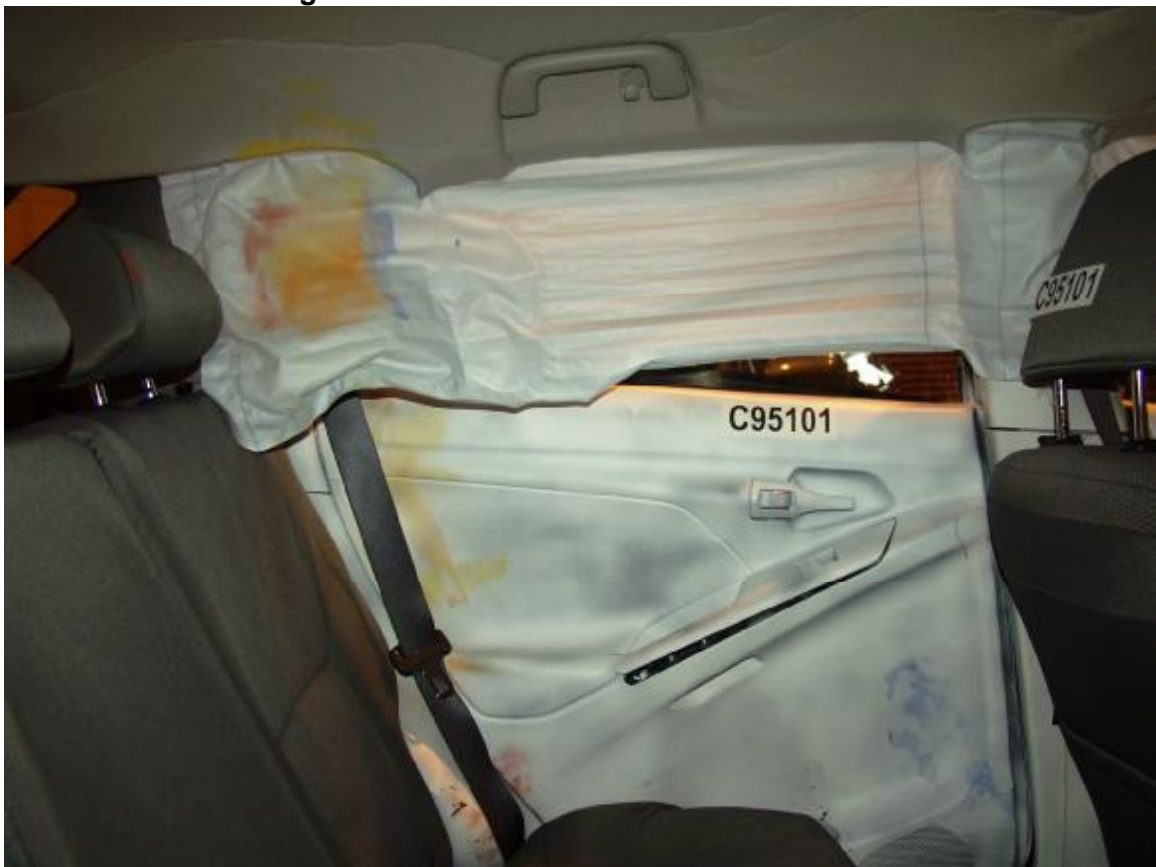
Figure A-46: Post-Test Left Rear Interior Trim
