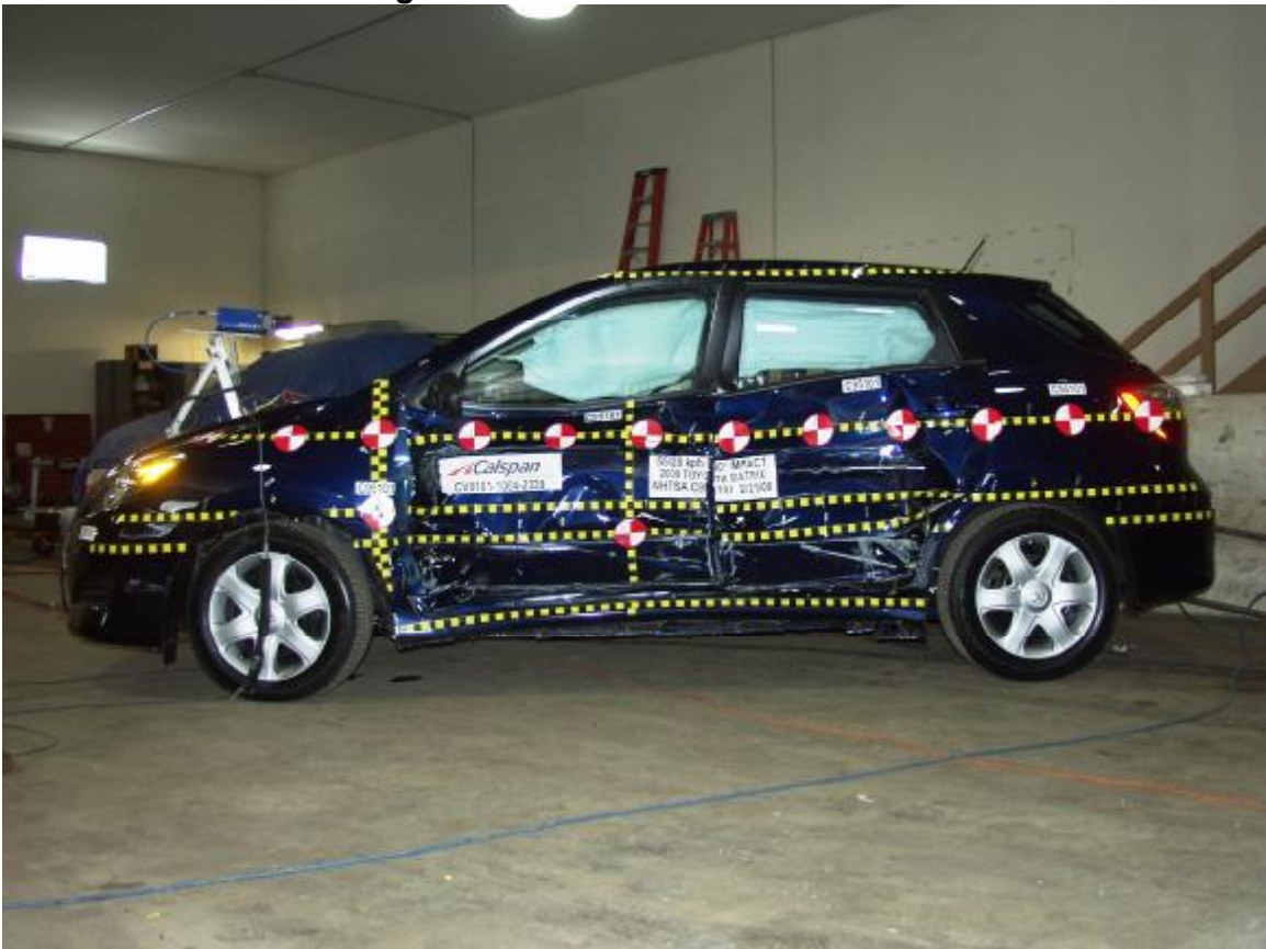
Figure A-10: Post-Test Left Side View
