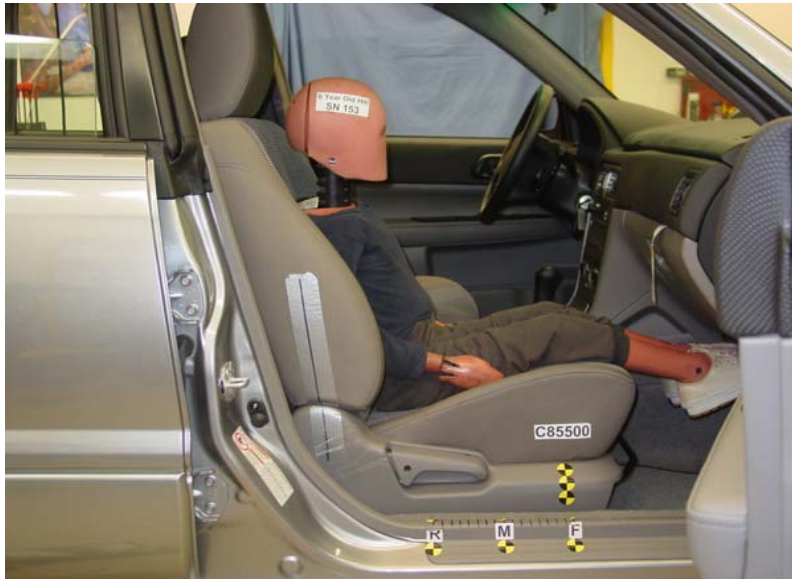
6-Year-Old Unbelted, Forward Seat Track, Position 2
