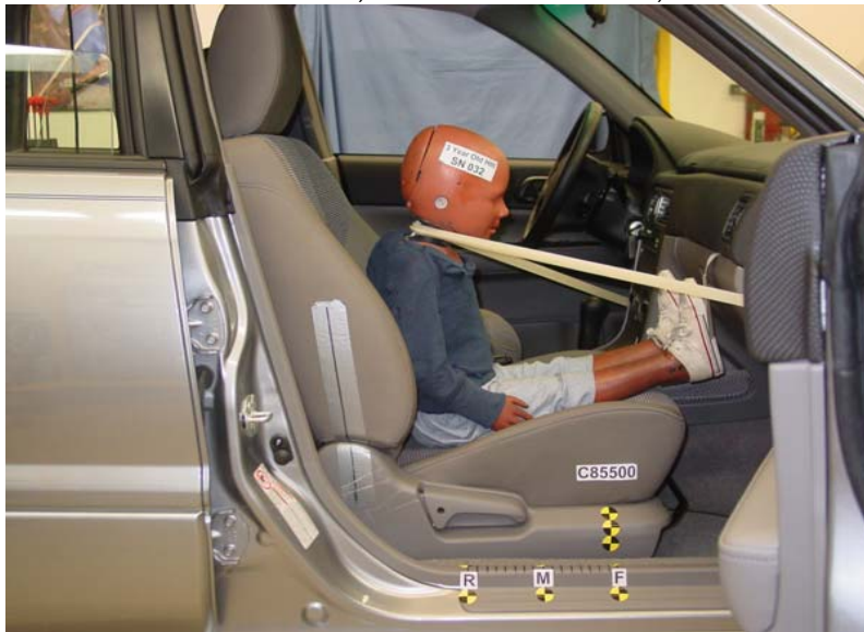
3-Year-Old Unbelted, Forward Seat Track, Position 3
