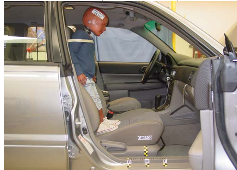
3-Year-Old Unbelted, Middle Seat Track, Position 5
