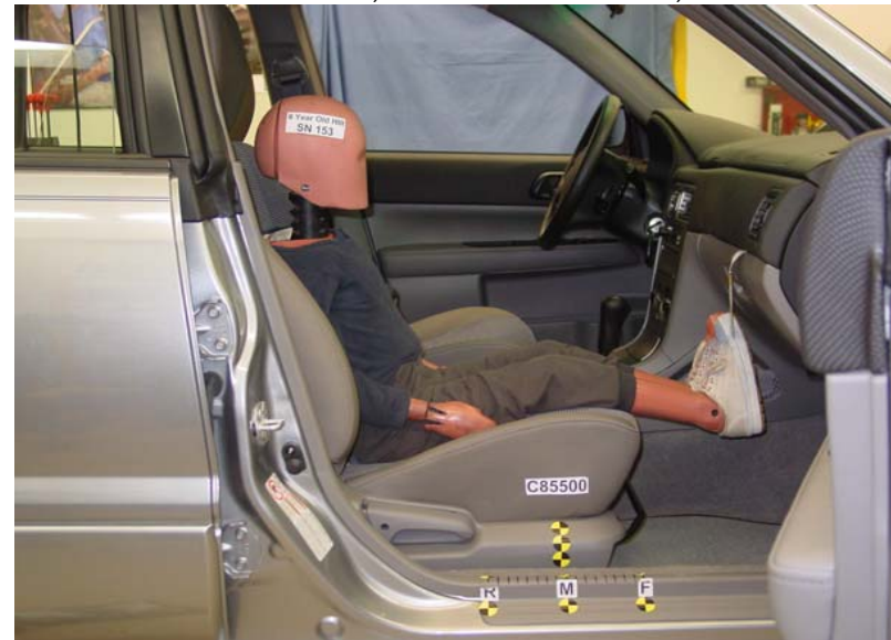
6-Year-Old Unbelted, Middle Seat Track, Position 1
