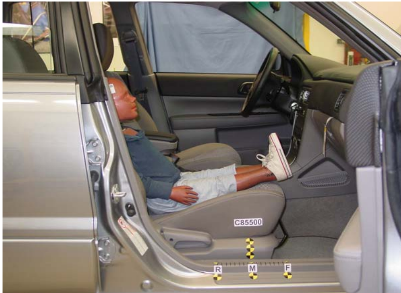
3-Year-Old Unbelted, Middle Seat Track, Position 2
