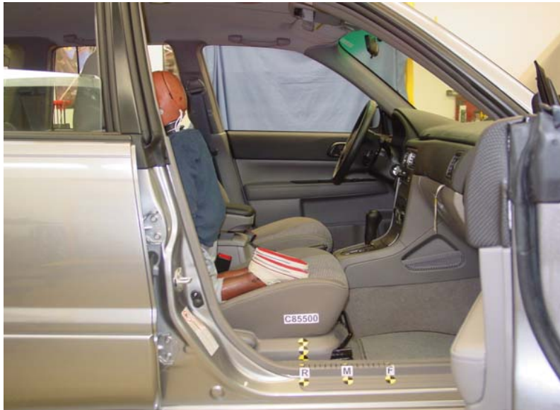
3-Year-Old Unbelted, Rearward Seat Track, Position 7
