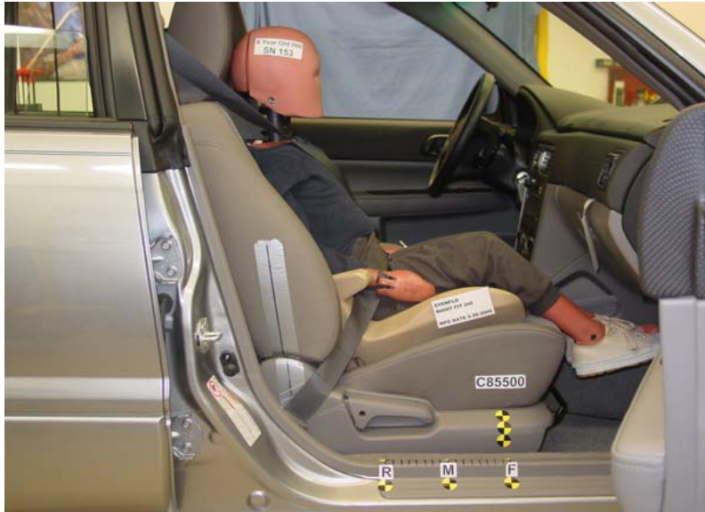
6-Year-Old Evenflo Right Fit Belted, Forward Seat Track
