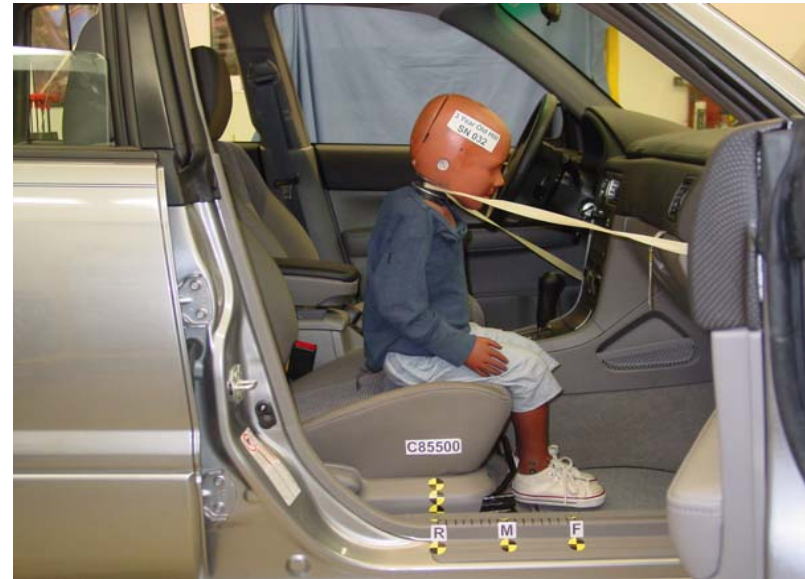
3-Year-Old Unbelted, Rearward Seat Track, Position 4
