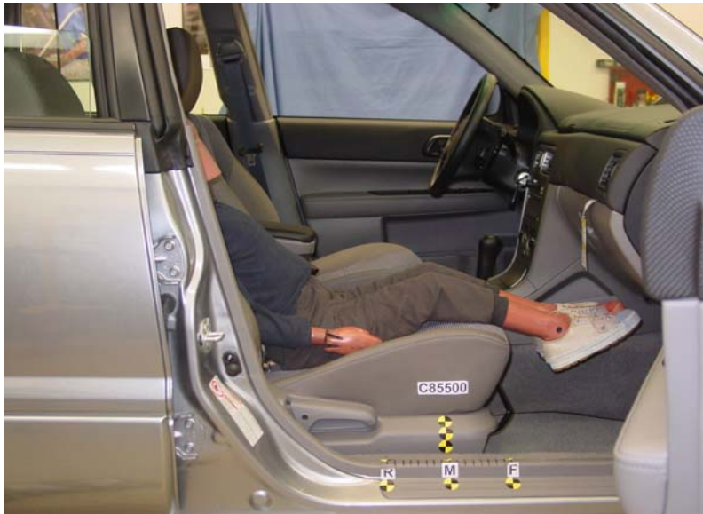
6-Year-Old Unbelted, Middle Seat Track, Position 2
