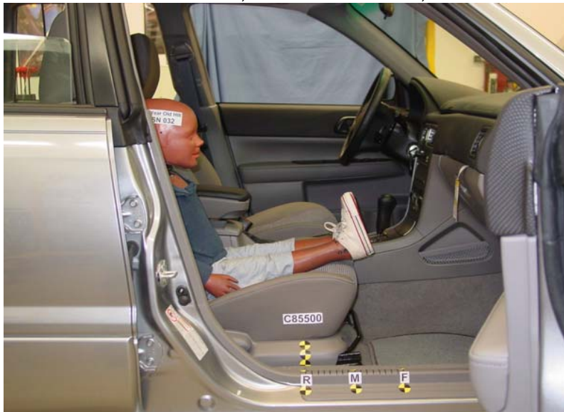
3-Year-Old Unbelted, Rearward Seat Track, Position 1
