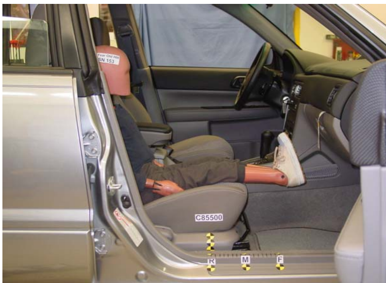
6-Year-Old Unbelted, Rearward Seat Track, Position 1
