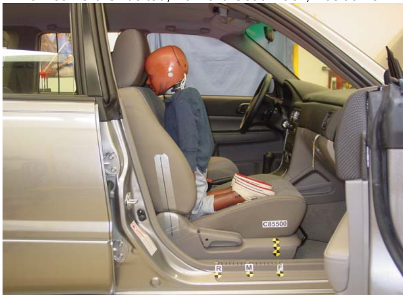
3-Year-Old Unbelted, Forward Seat Track, Position 7
