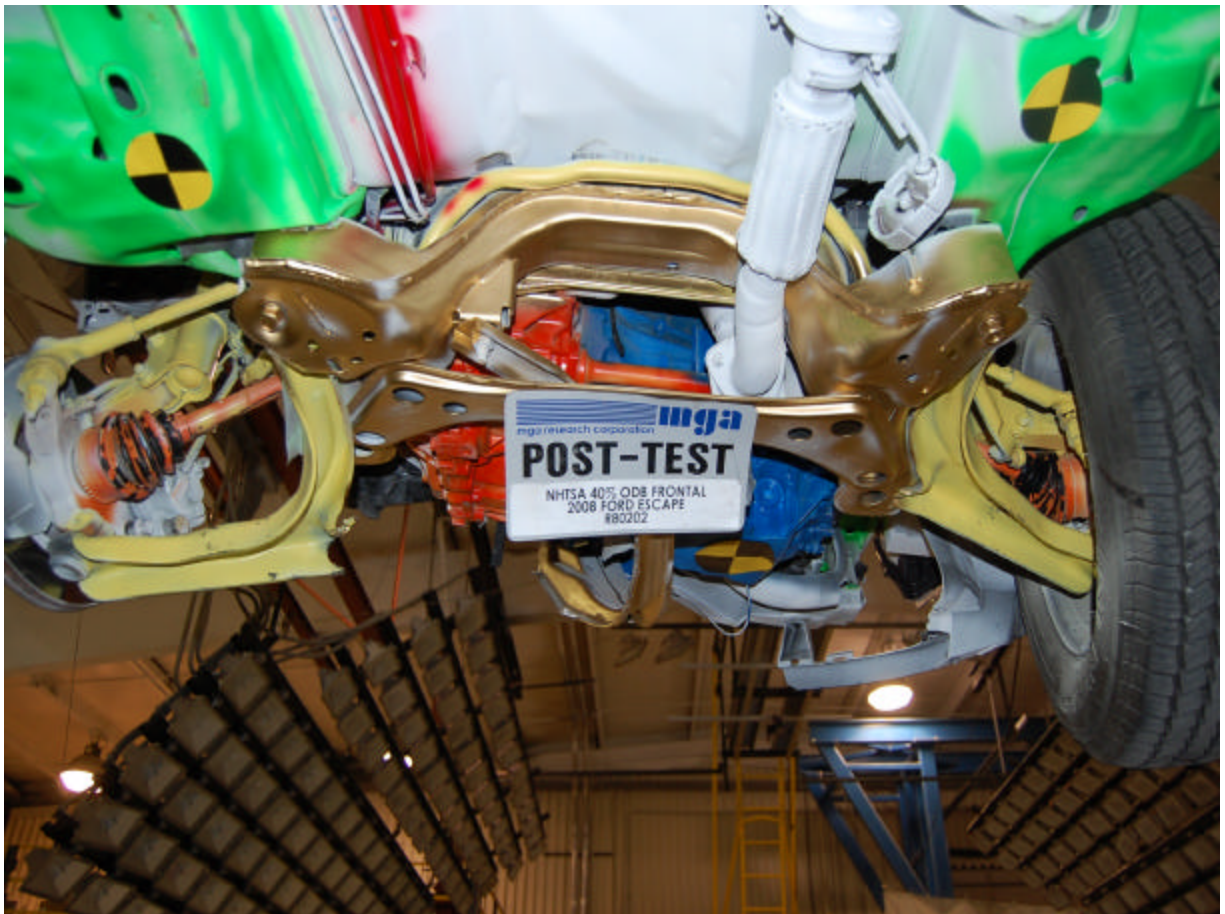
Post-Test Sway Bar View
