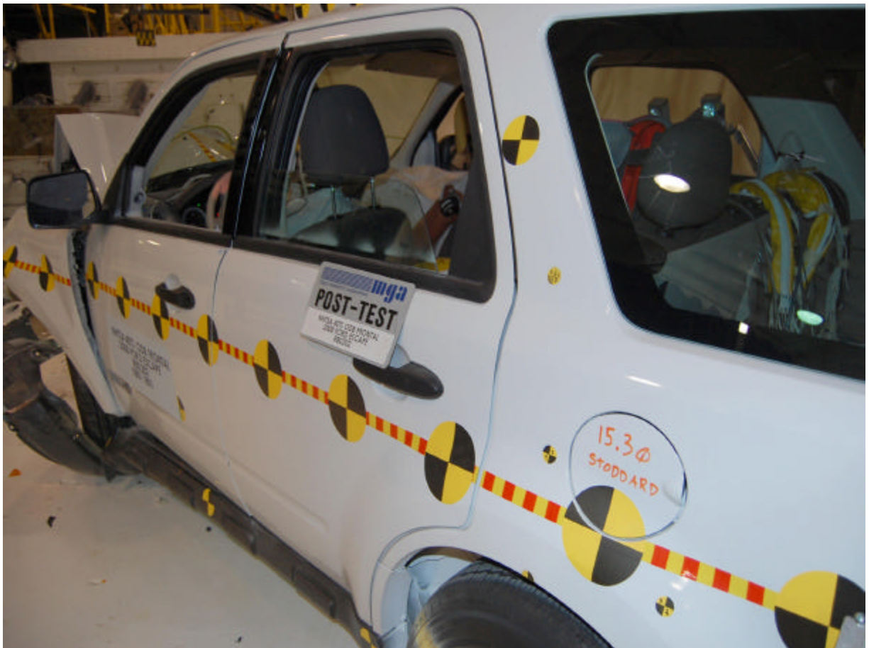
Post-Test Left Side ¾ View of Doors After Impact
