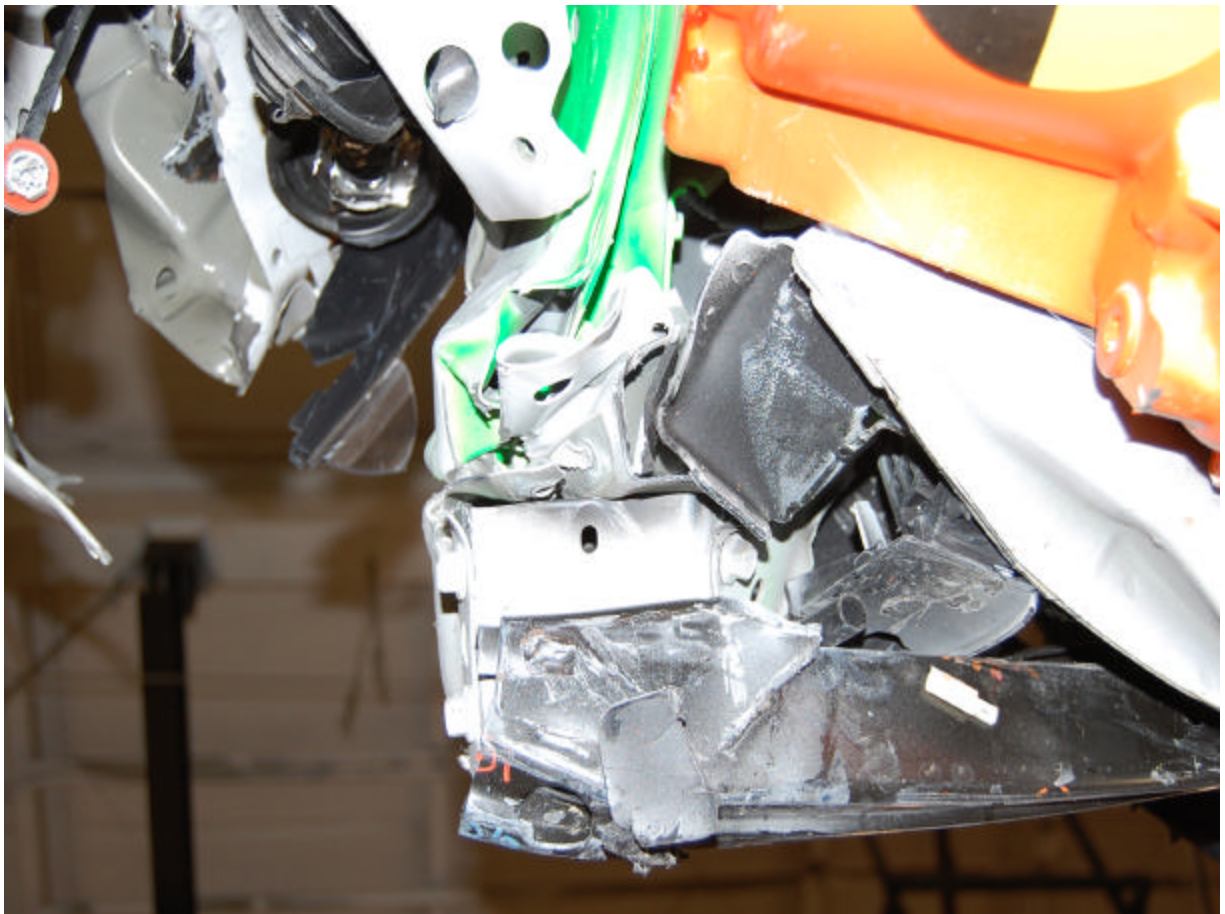
Post-Test Bumper to Rail Attachment View
