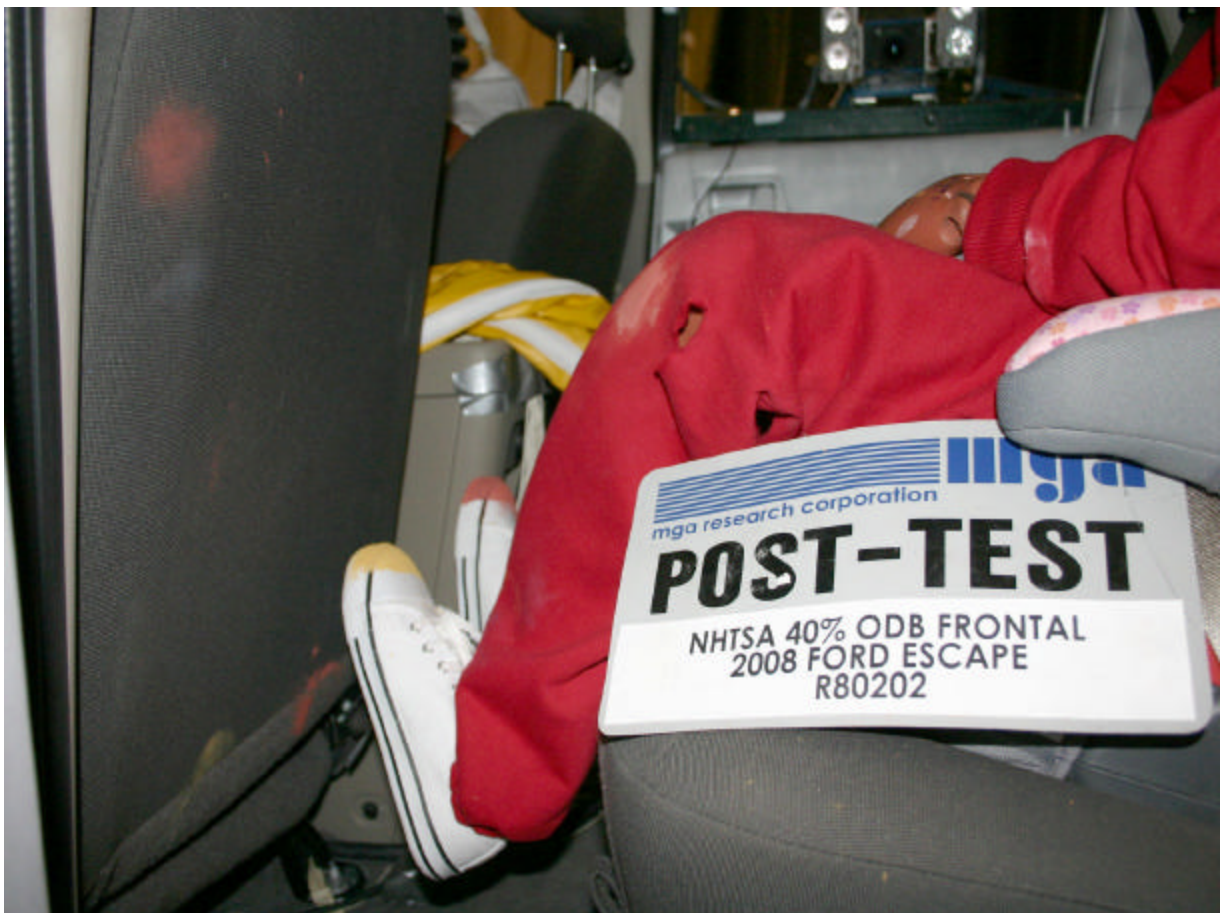
Post-Test Left Rear Passenger Dummy Leg Position View
