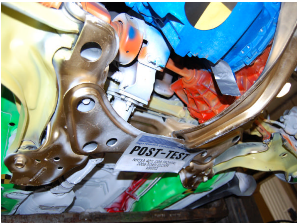
Post-Test Steering Rack \frac{3}{4} Right Side View
