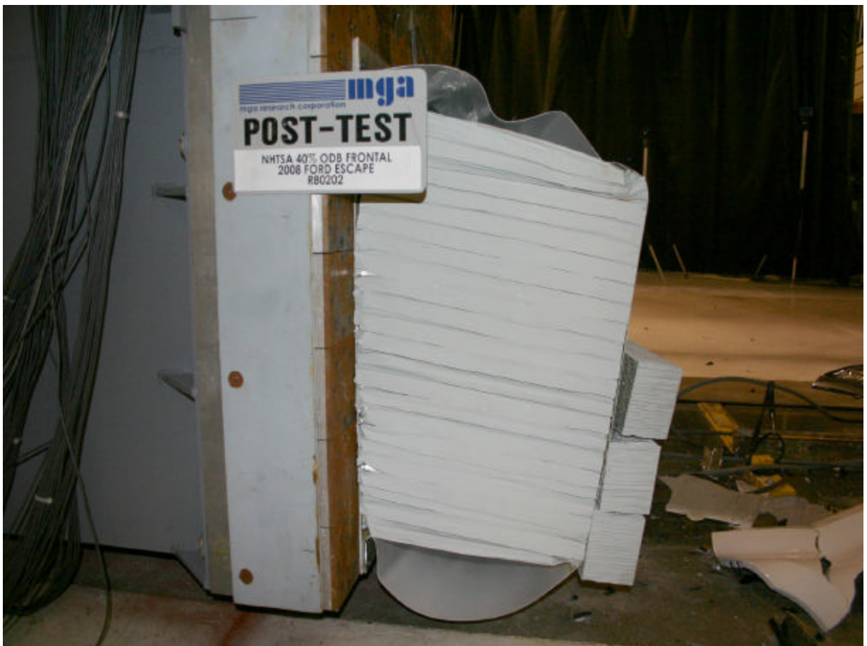
Post-Test Offset Deformable Barrier Left Side View
