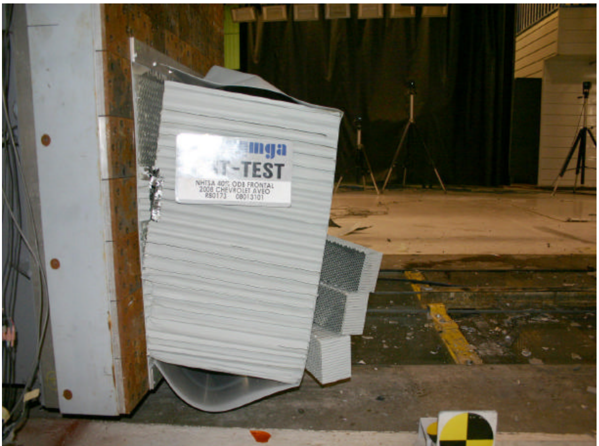
Post-Test Offset Deformable Barrier Left Side View
