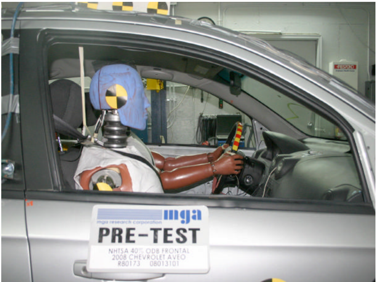
Pre-Test Passenger Dummy (Through Window)
