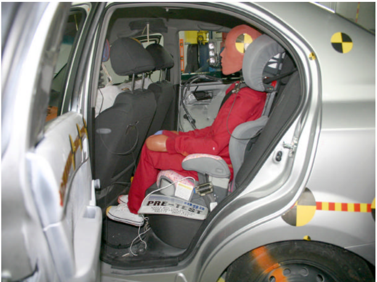
Pre-Test Left Rear Passenger Dummy (Door Open)
