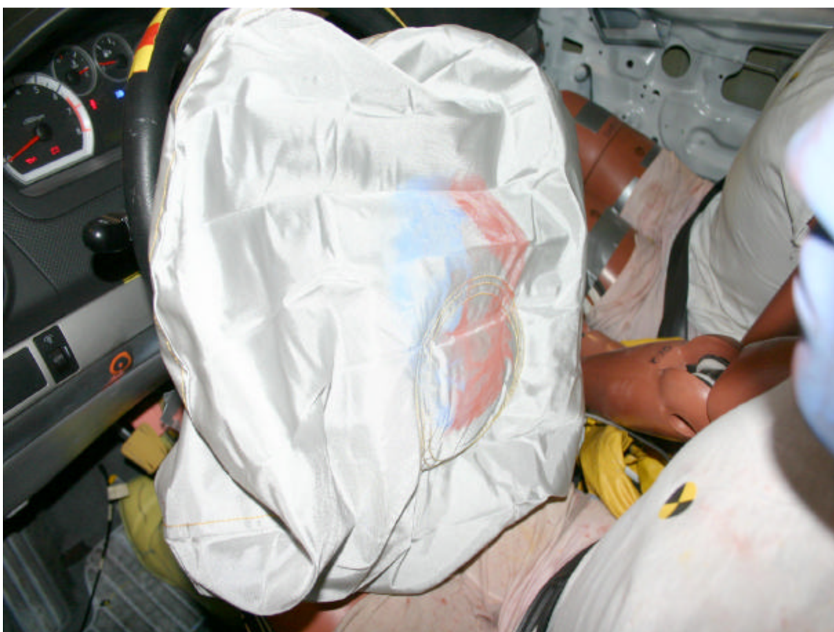
Post-Test Driver Dummy Airbag Contact
