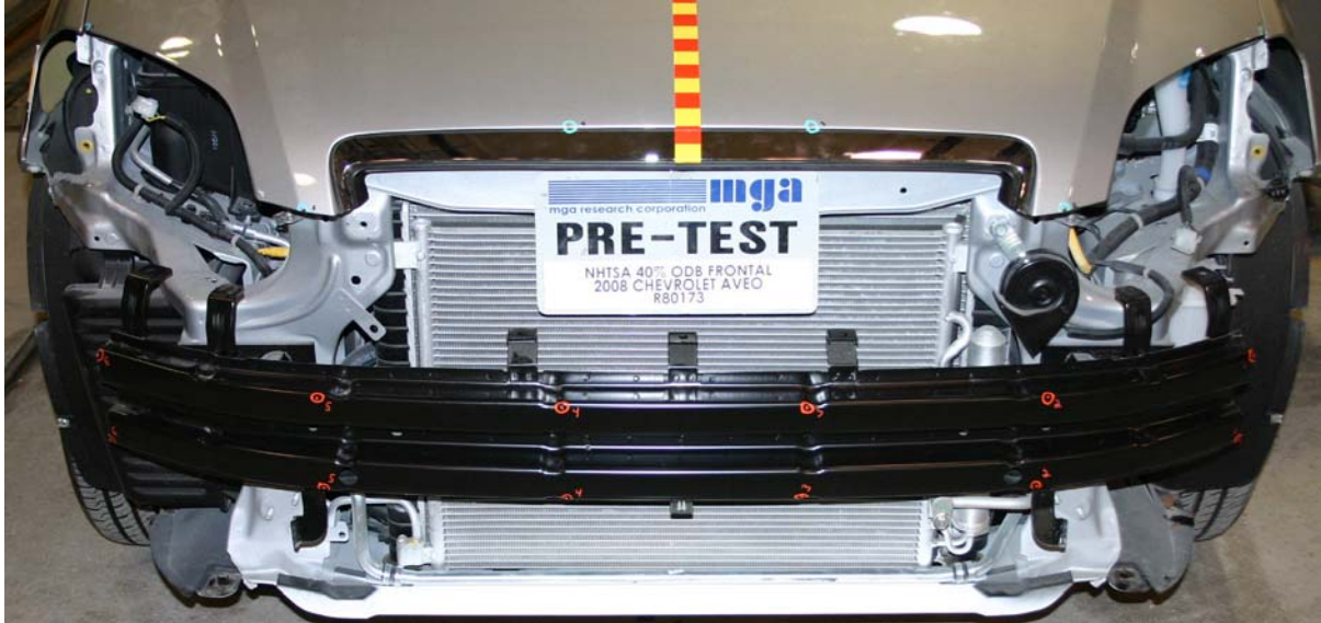
Lower Bumper Beam / Upper Bumper Beam / Front of Hood
