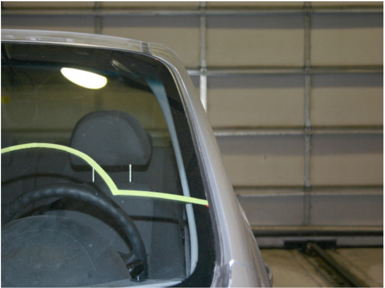
Pre-Test Left Side A Pillar (Frontal View)
