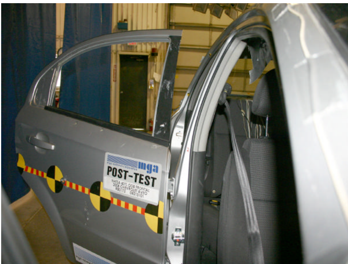
Post-Test Right Side B Pillar
