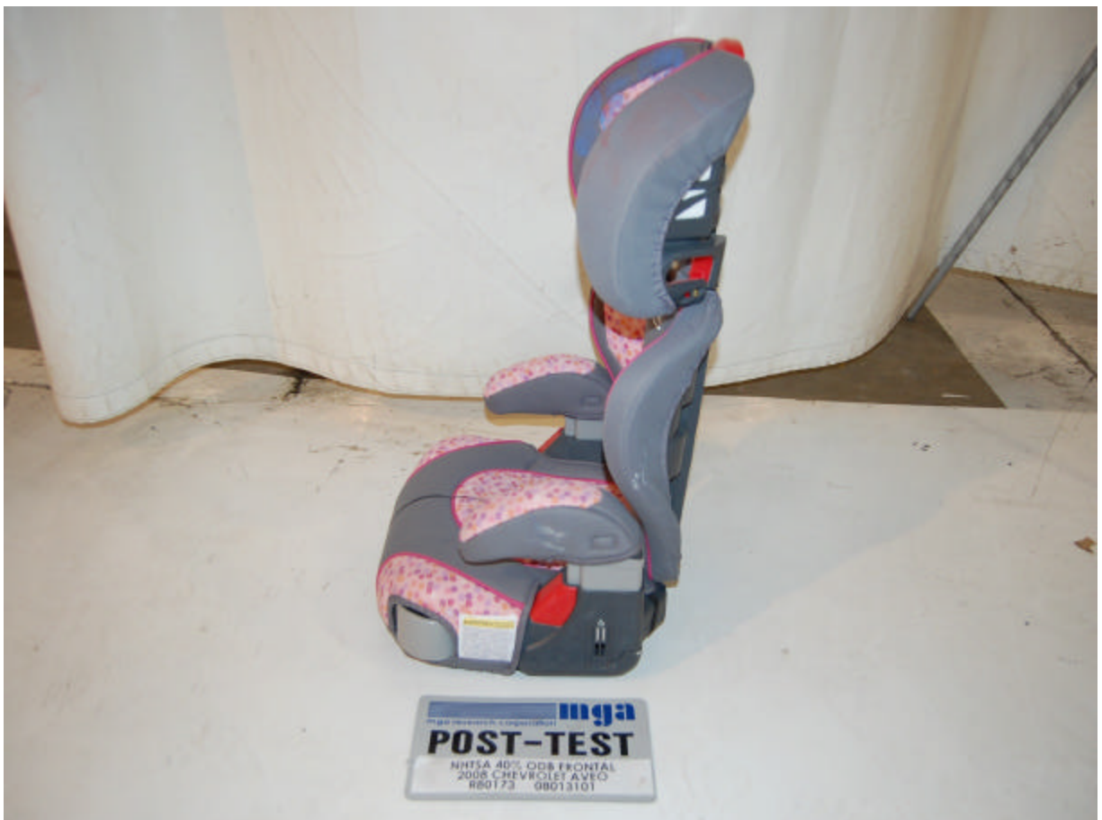
Post-Test Left Side View of CRS
