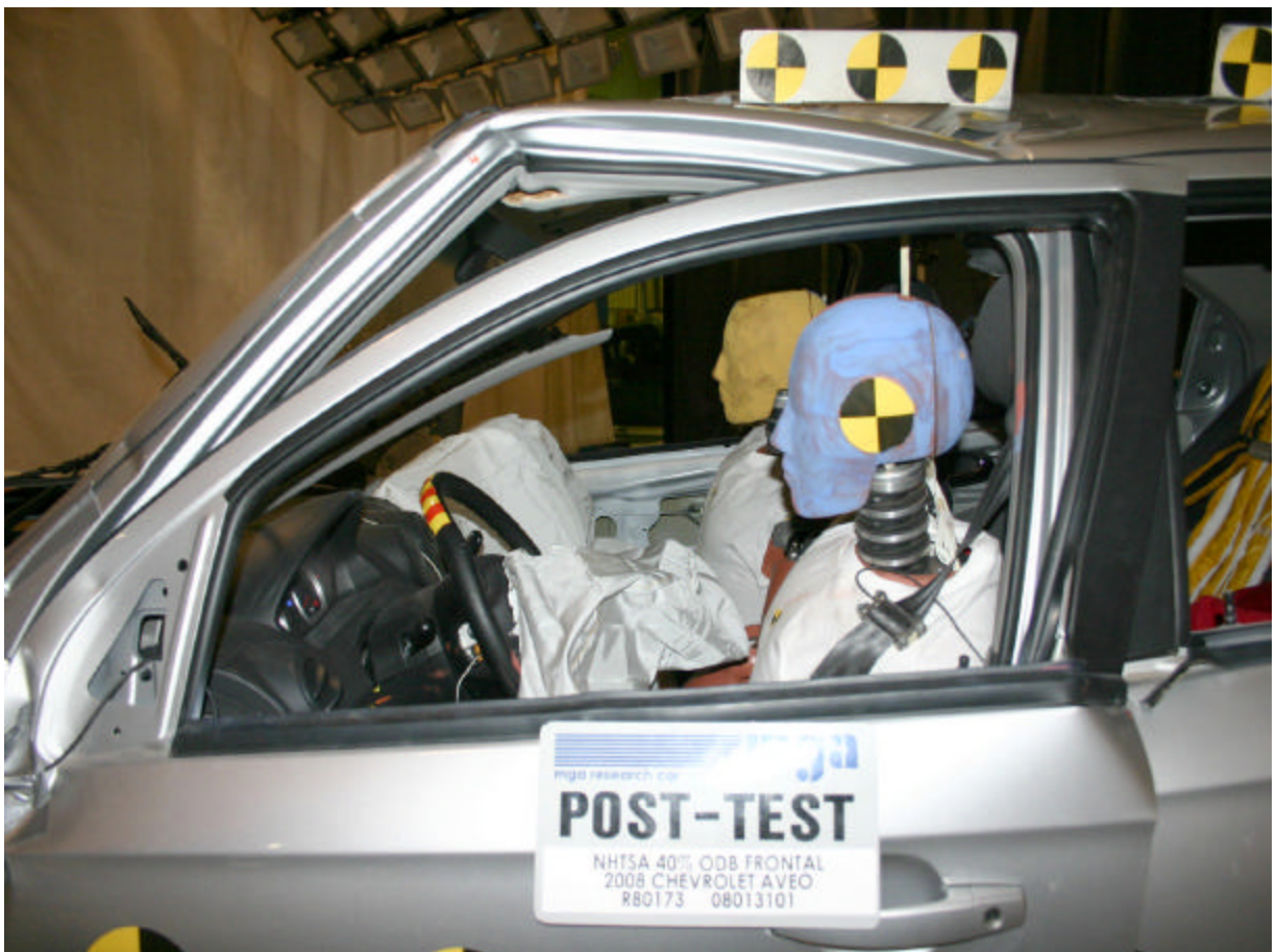
Post-Test Driver Dummy (Through Window)
