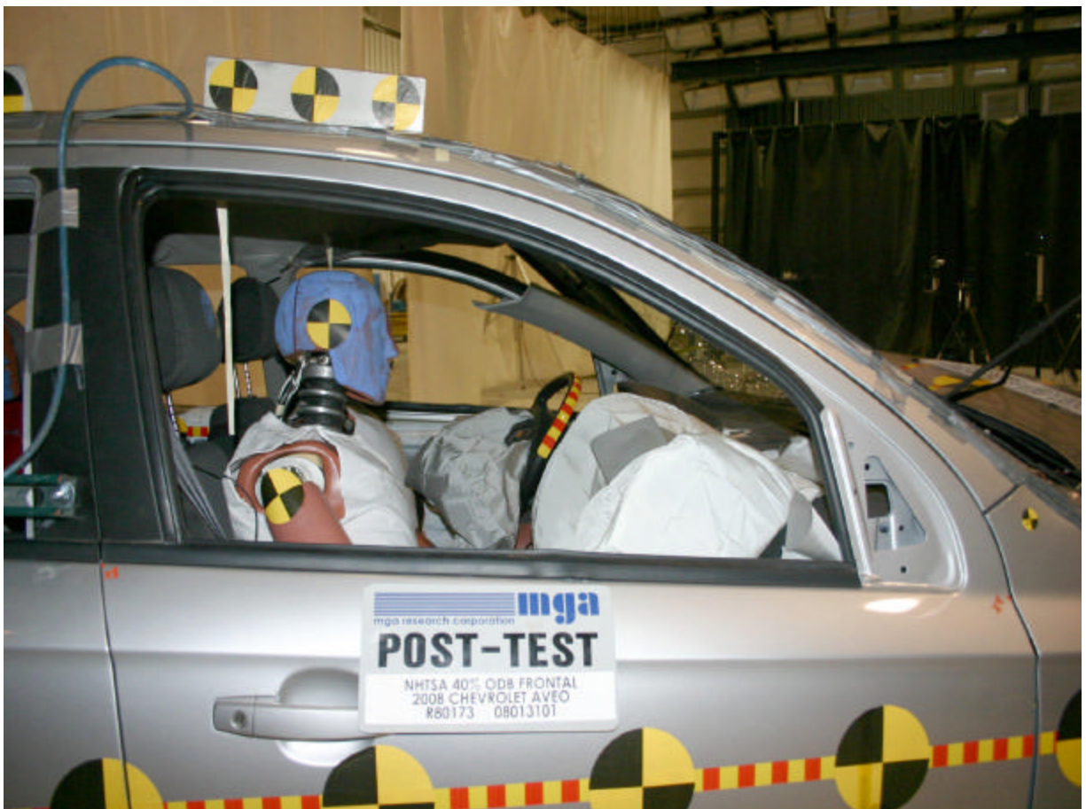
Post-Test Passenger Dummy (Through Window)
