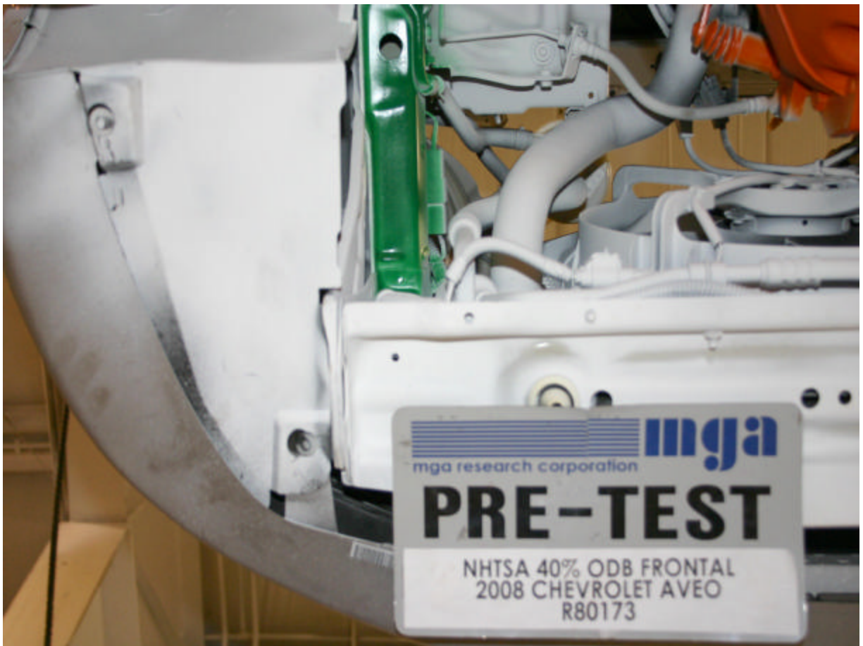
Pre-Test Bumper to Rail Attachment View
