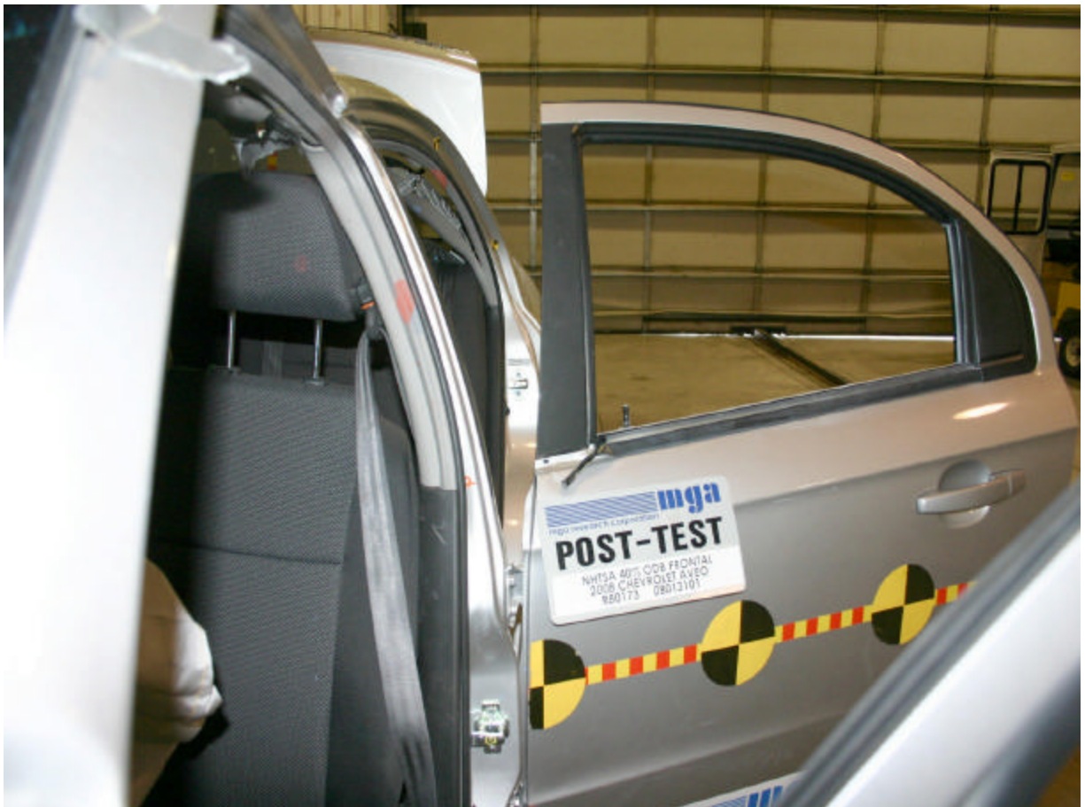
Post-Test Left Side B Pillar
