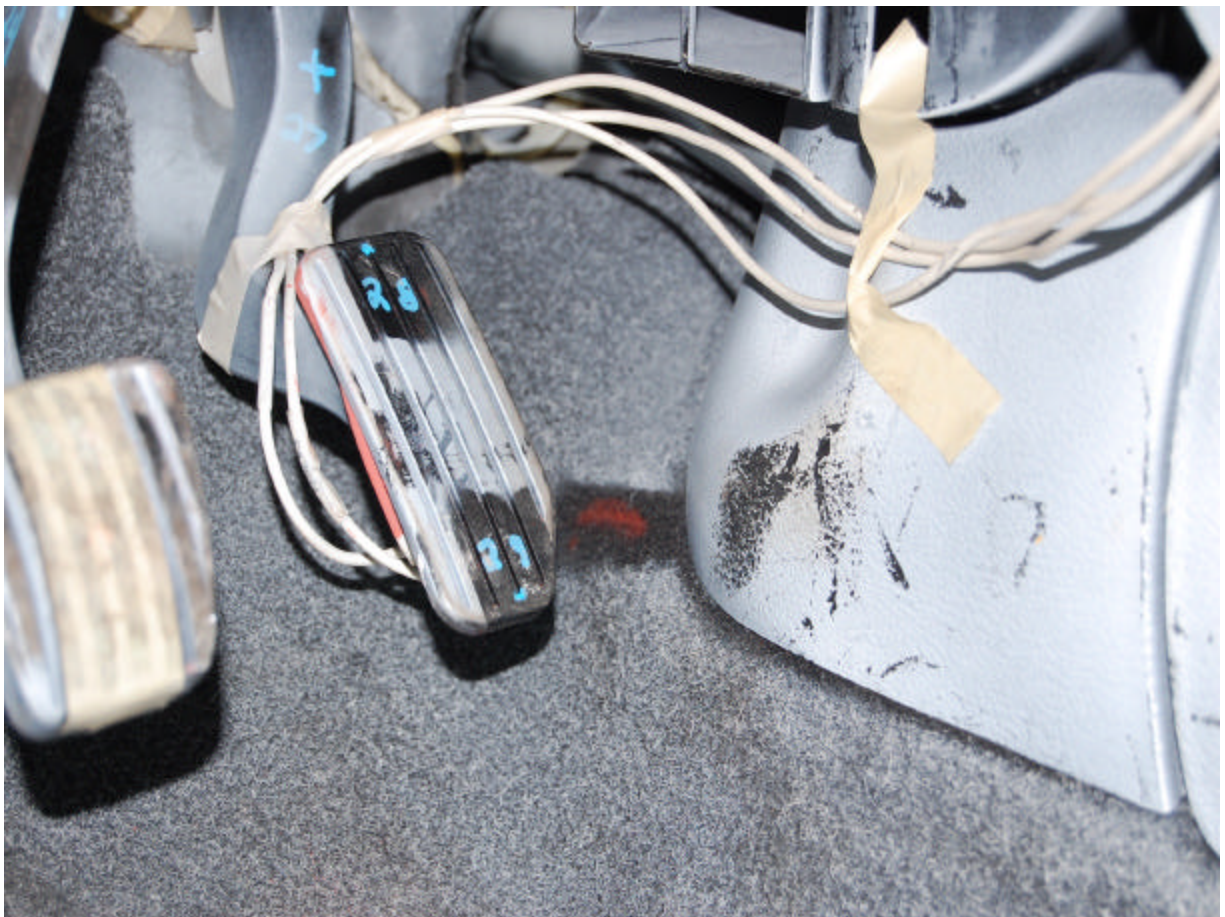
Pre-Test Accelerometer Pedal Close Up
