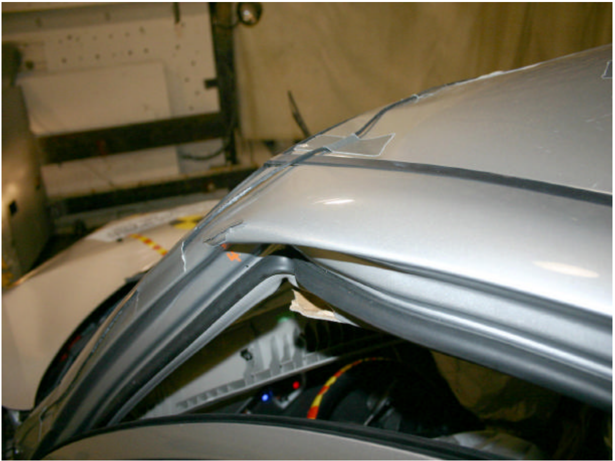
Post-Test Left Side A-Pillar Close Up \frac{3}{4} View
