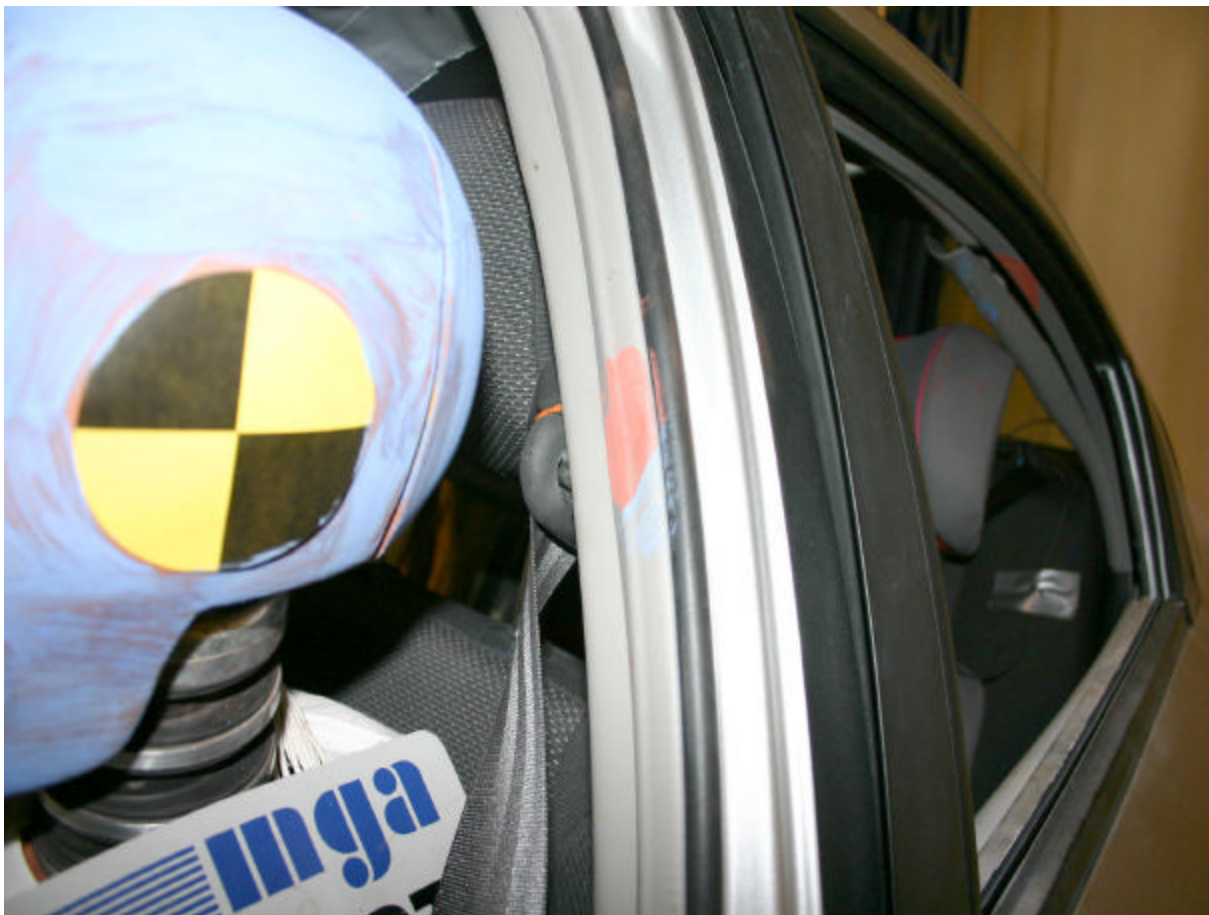
Post-Test Driver Dummy Head Contact (B-pillar)
