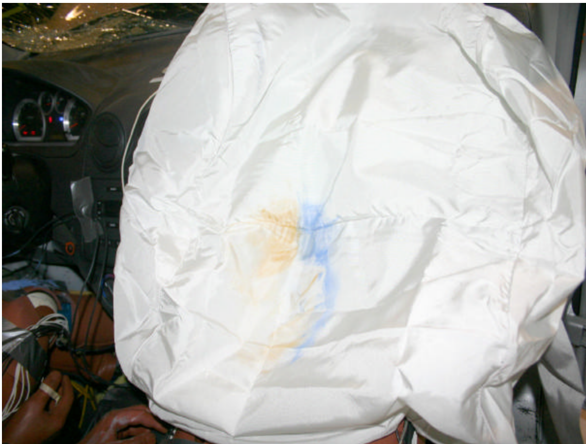
Post-Test Passenger Dummy Airbag Contact
