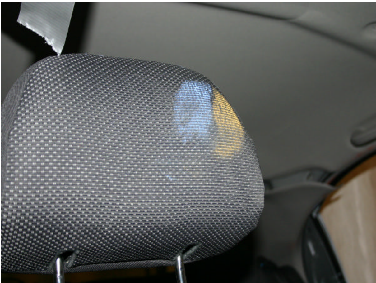
Post-Test Passenger Dummy Head Contact (headrest)
