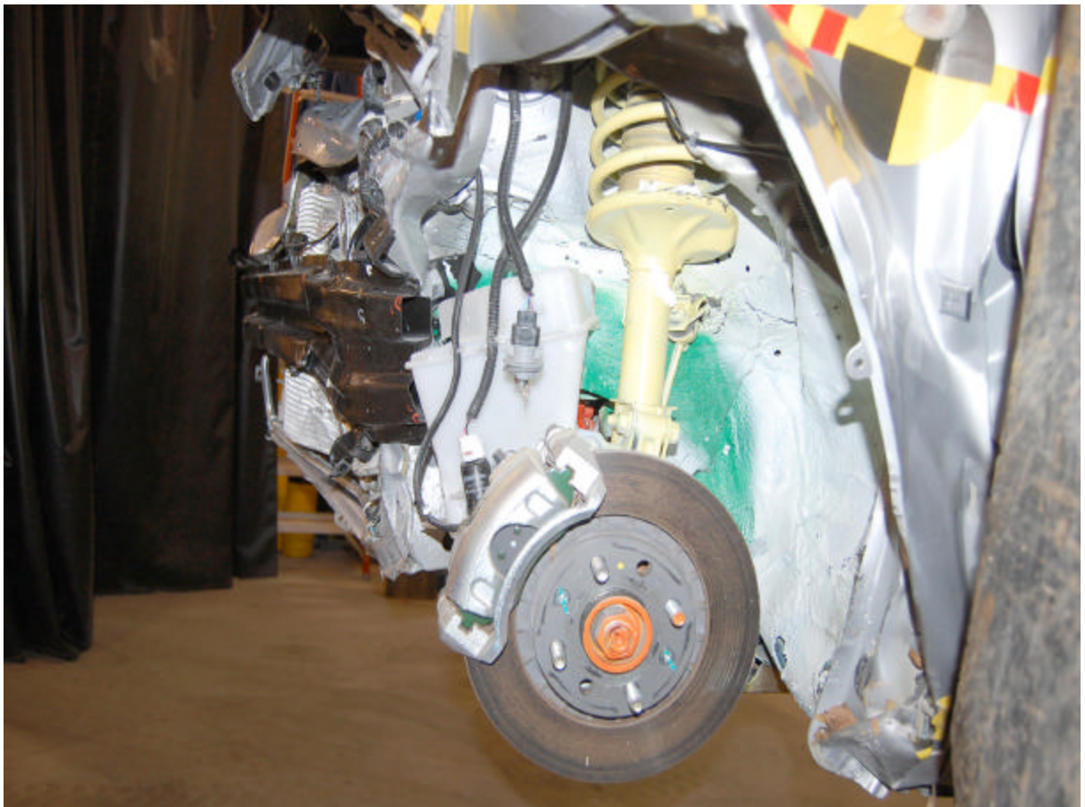
Post-Test Left Front Wheel Well
