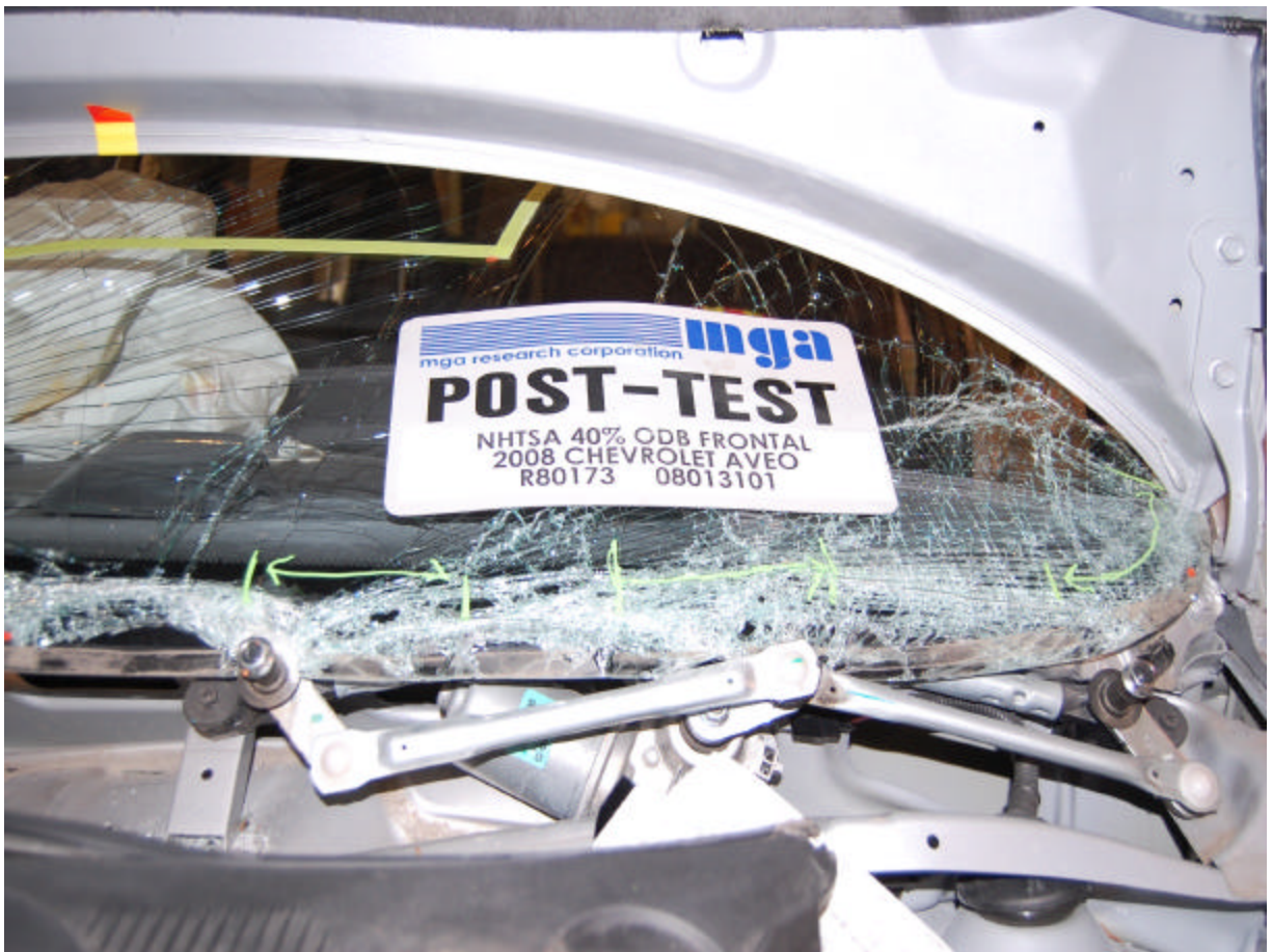
Post-Test Windshield Damage
