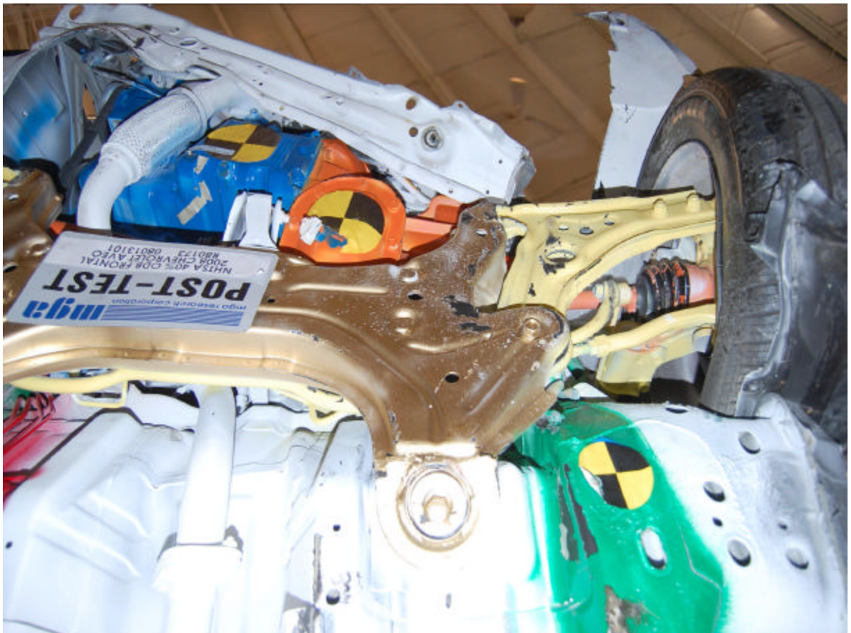
Post-Test Steering Rack ¾ Left Side View
