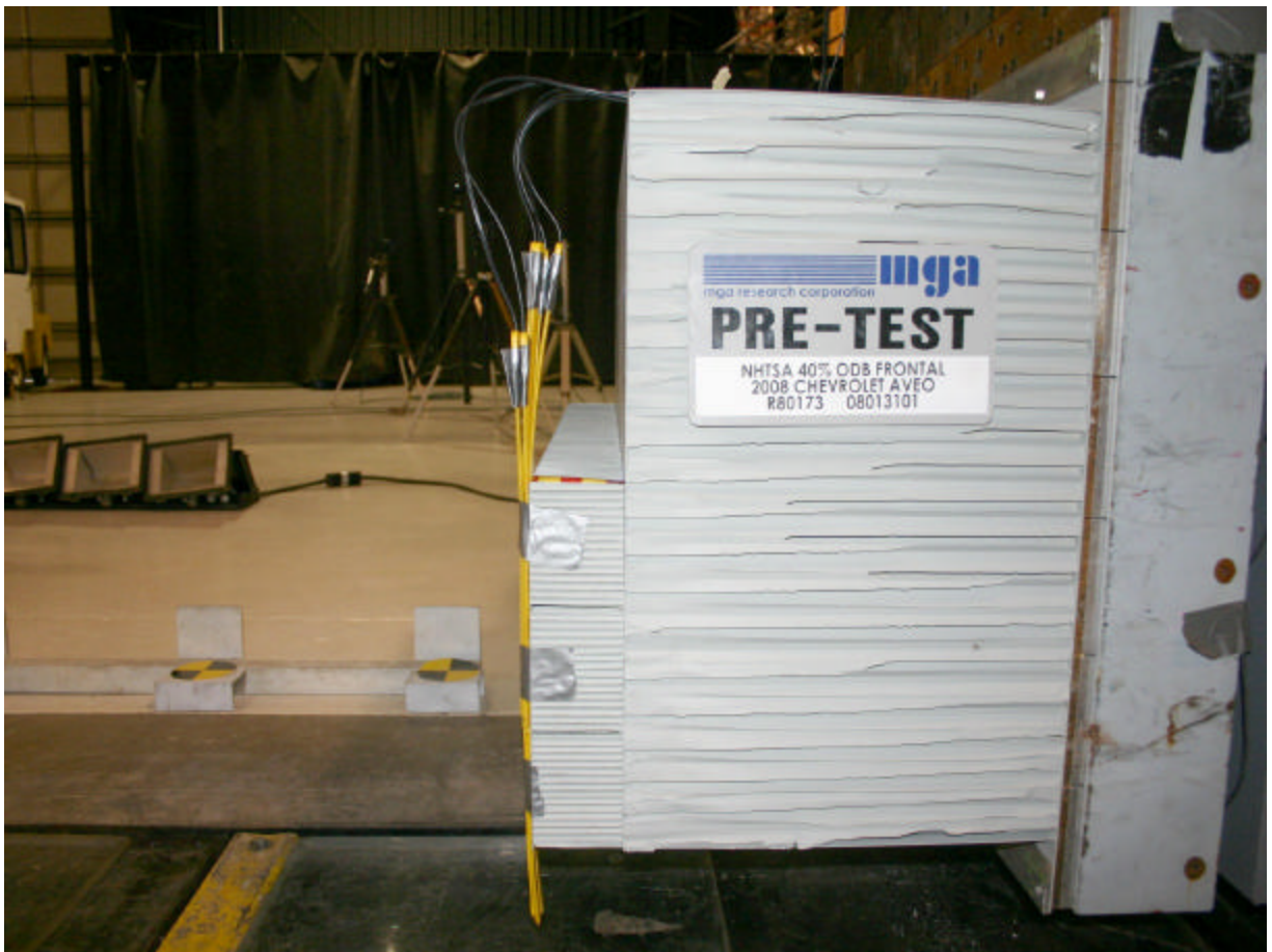
Pre-Test Offset Deformable Barrier Right Side View
