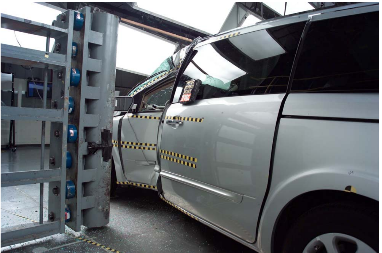
Figure A-21 Post-Test Impact Point View
