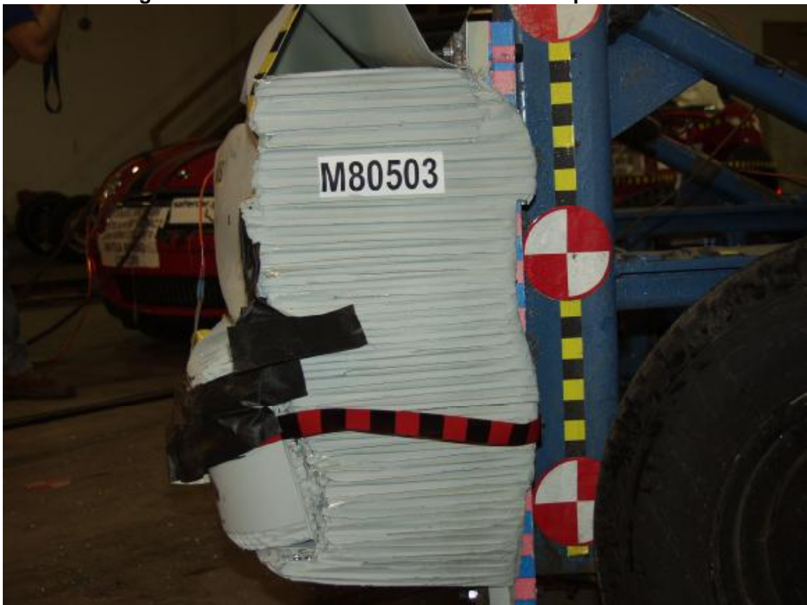
Figure A-24: Post-Test Left Side View of MDB Impactor Face
