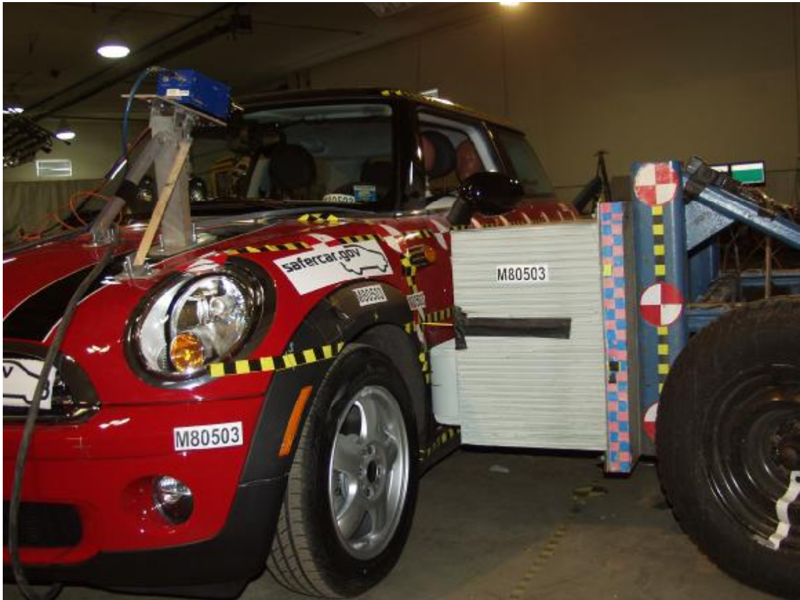
Figure A-29: Pre-Test Left Side View of Aligned MDB and Vehicle
