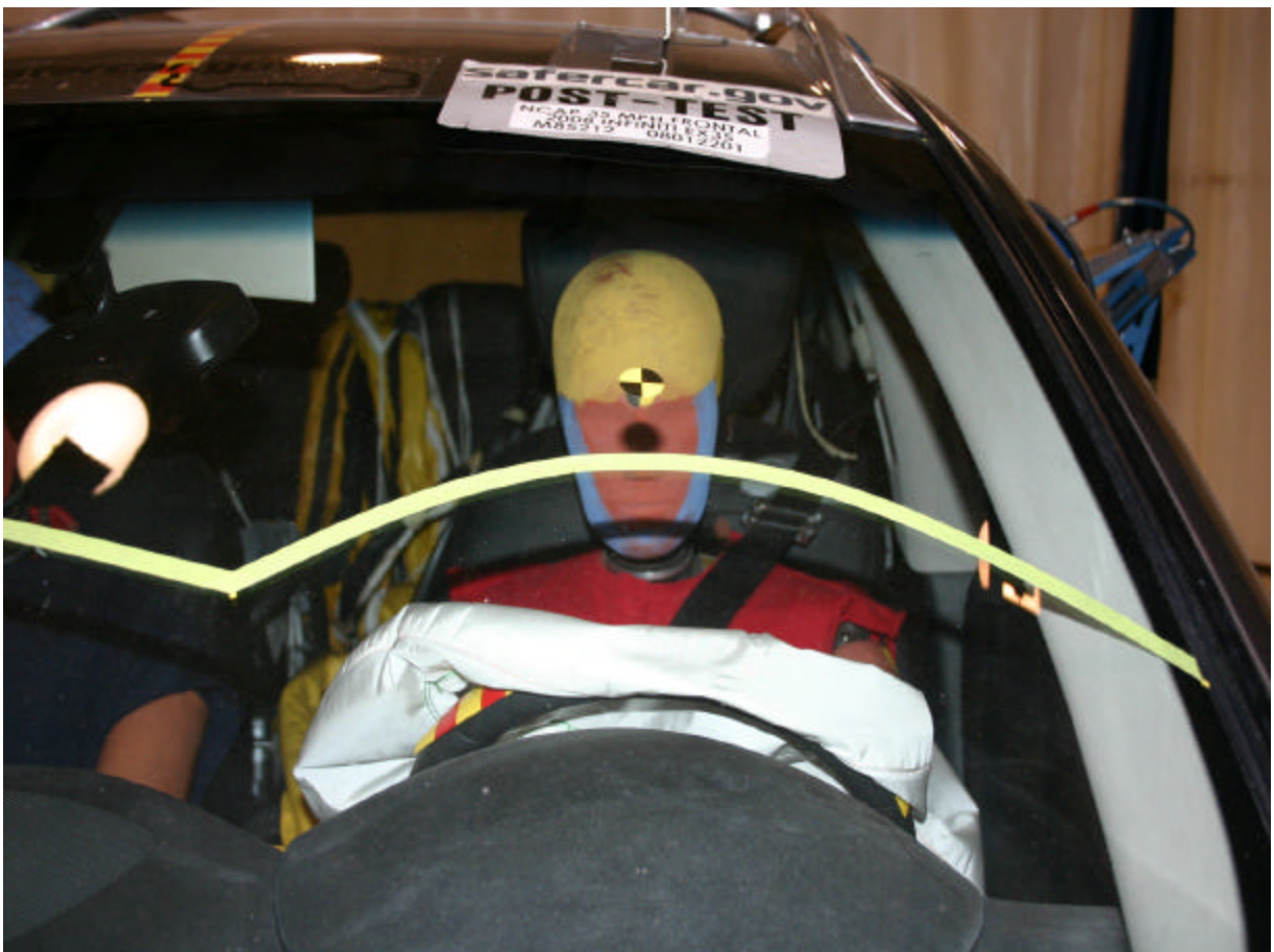
Post-Test Driver Dummy Front View (Head Position)
