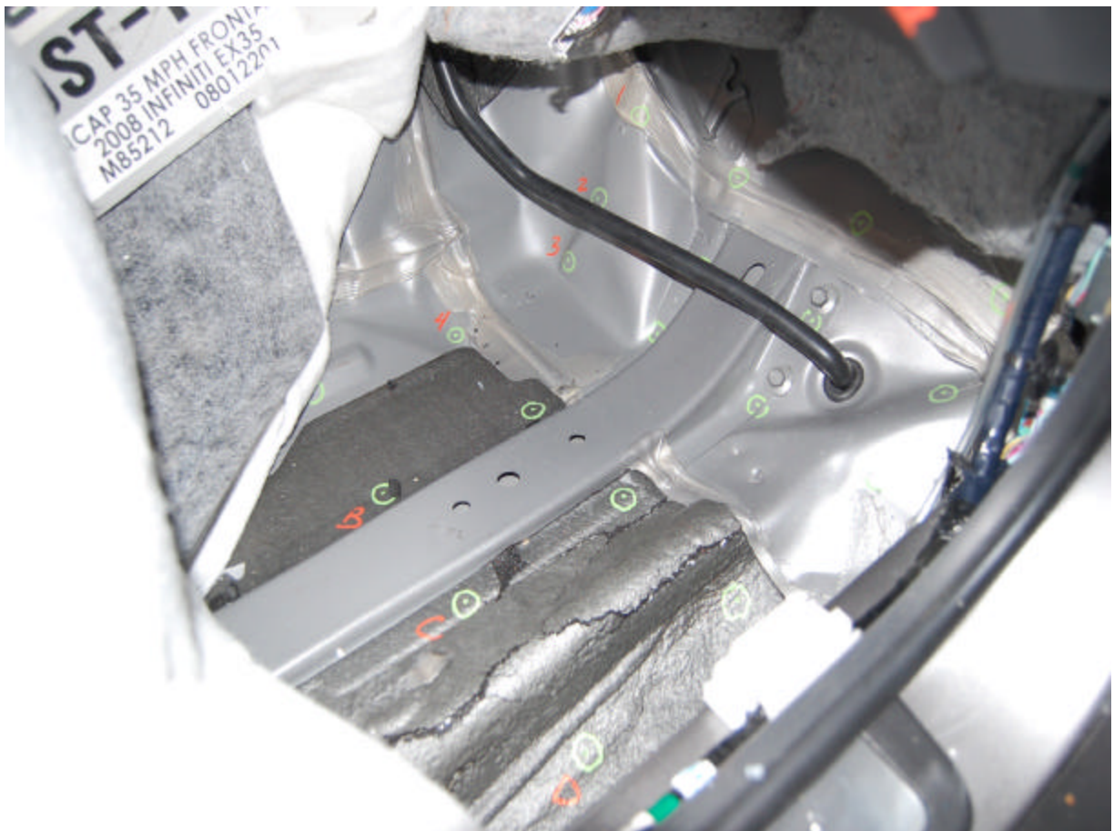
Post-Test Passenger Side Floor Pan
