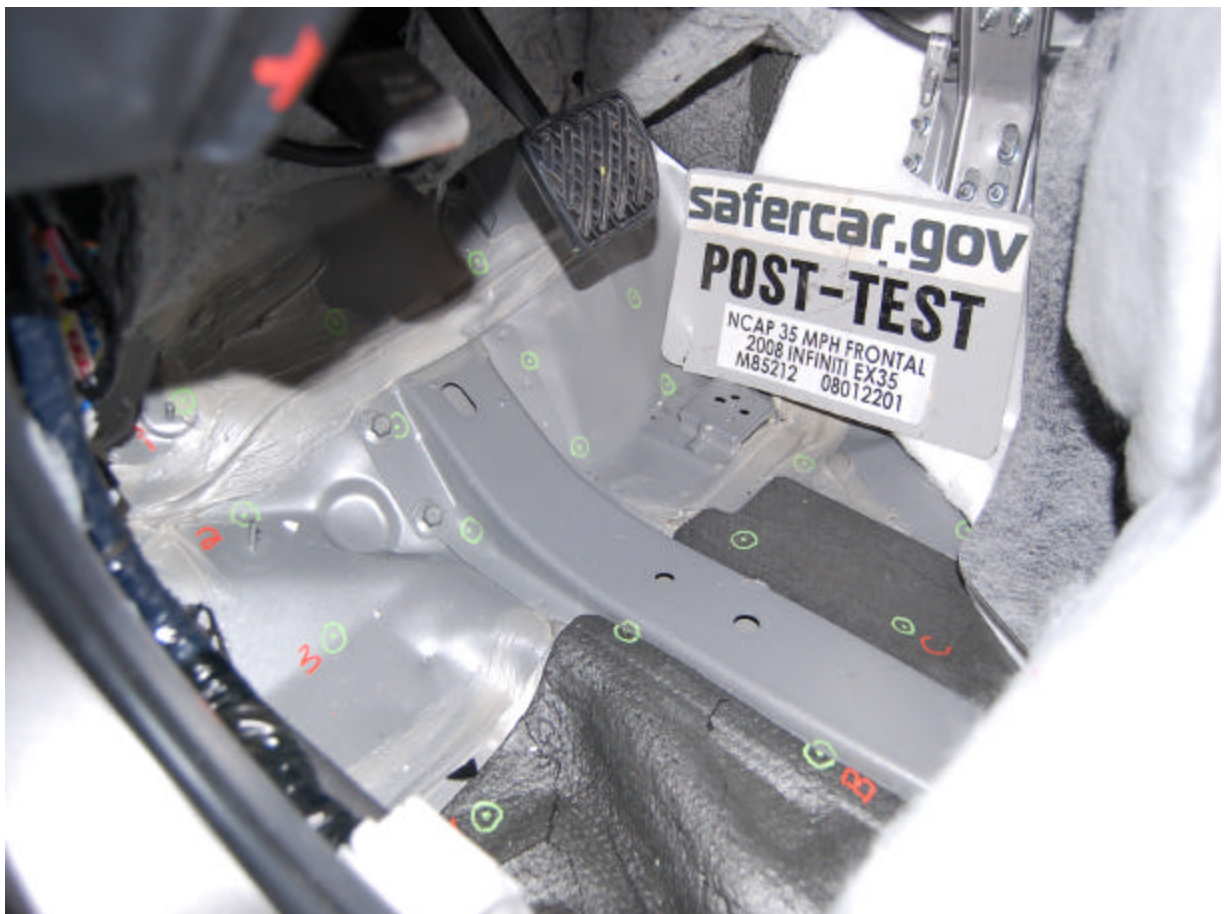
Post-Test Driver Side Floor Pan
