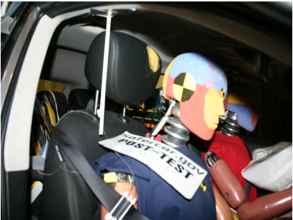
Post-Test Passenger Dummy Head Contact (Headrest)
