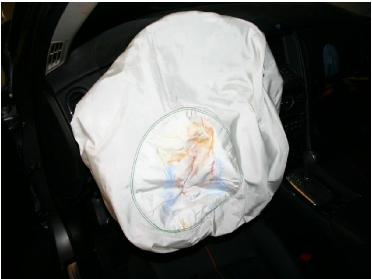
Post-Test Driver Dummy Airbag Contact
