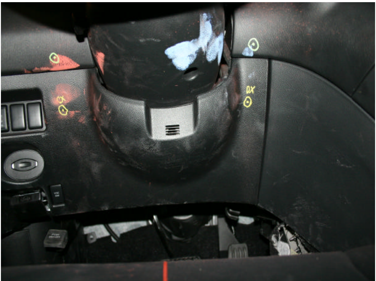
Post-Test Driver Dummy Knee Contact
