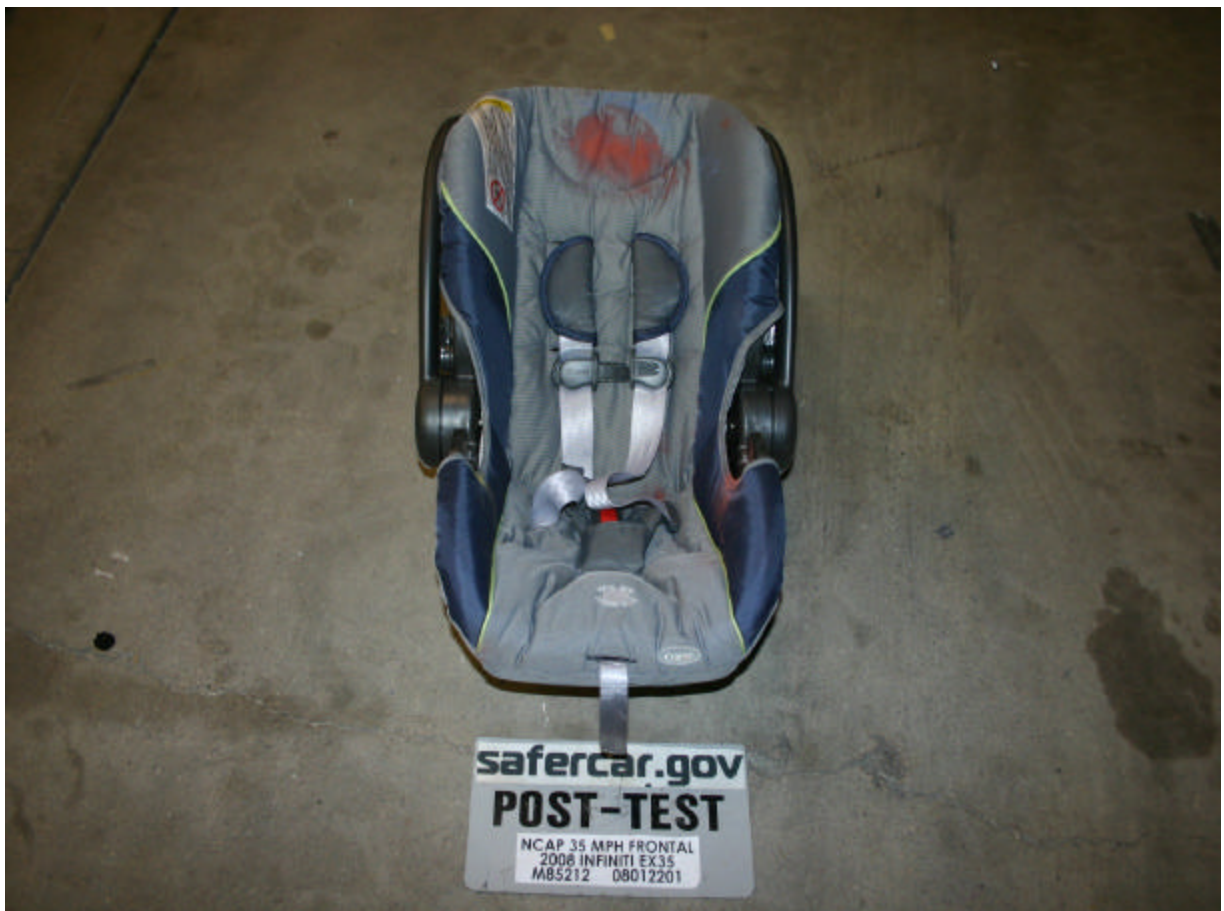
Post-Test Front View of Position 3 CRS
