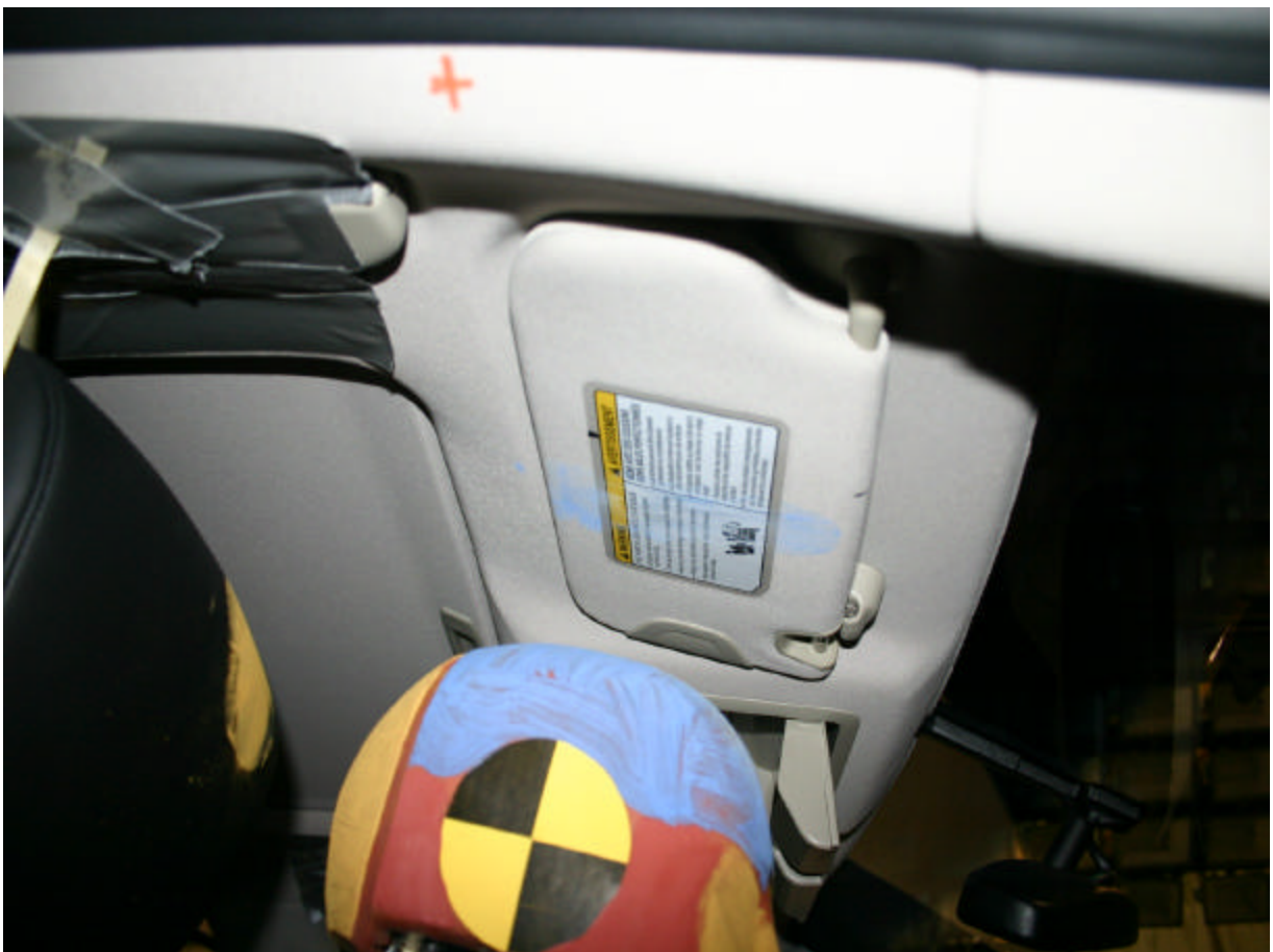
Post-Test Passenger Dummy Head Contact (Visor & Headliner)
