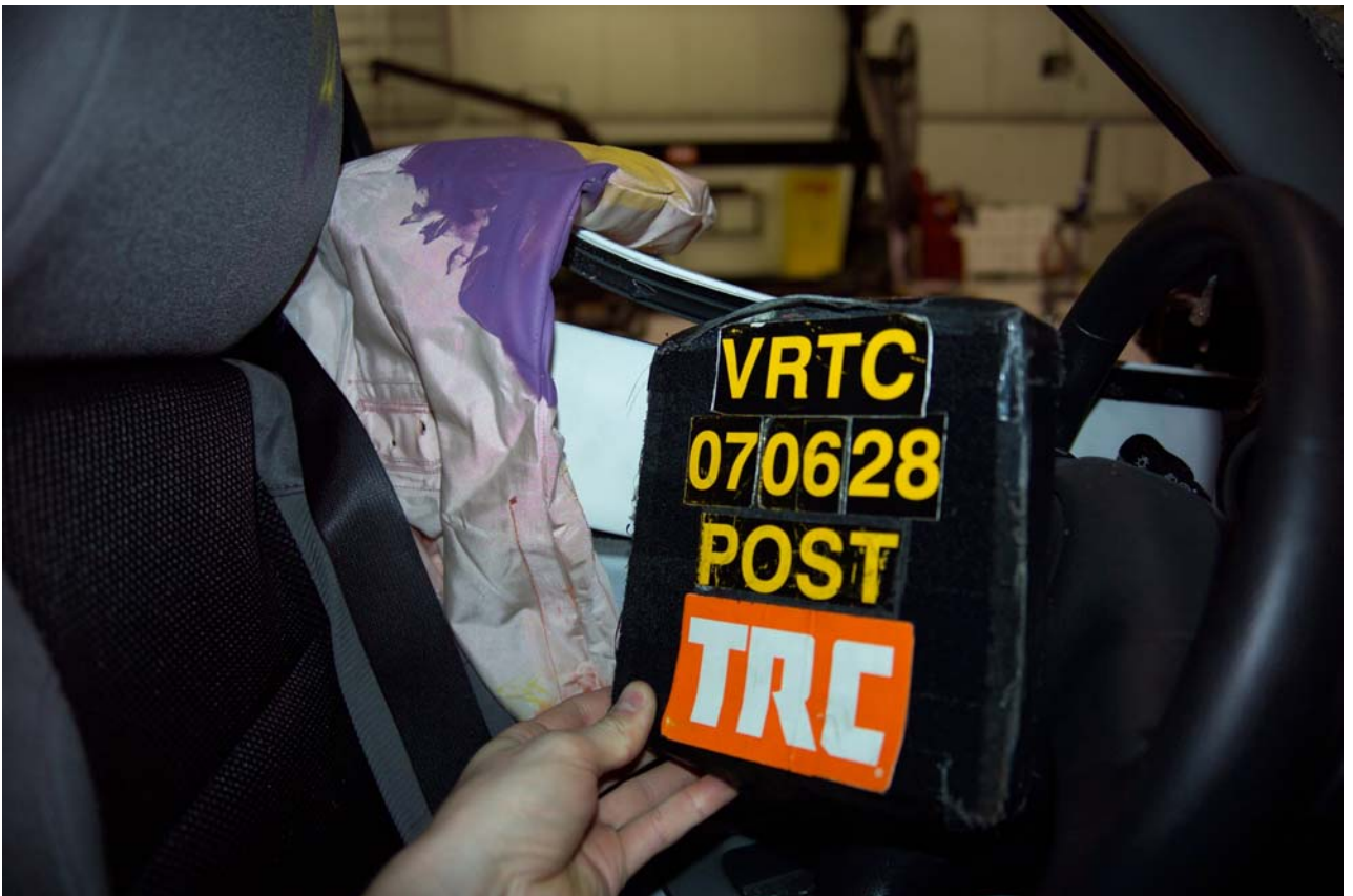
Figure A-36 Post-Test Driver Dummy Door Contact View
