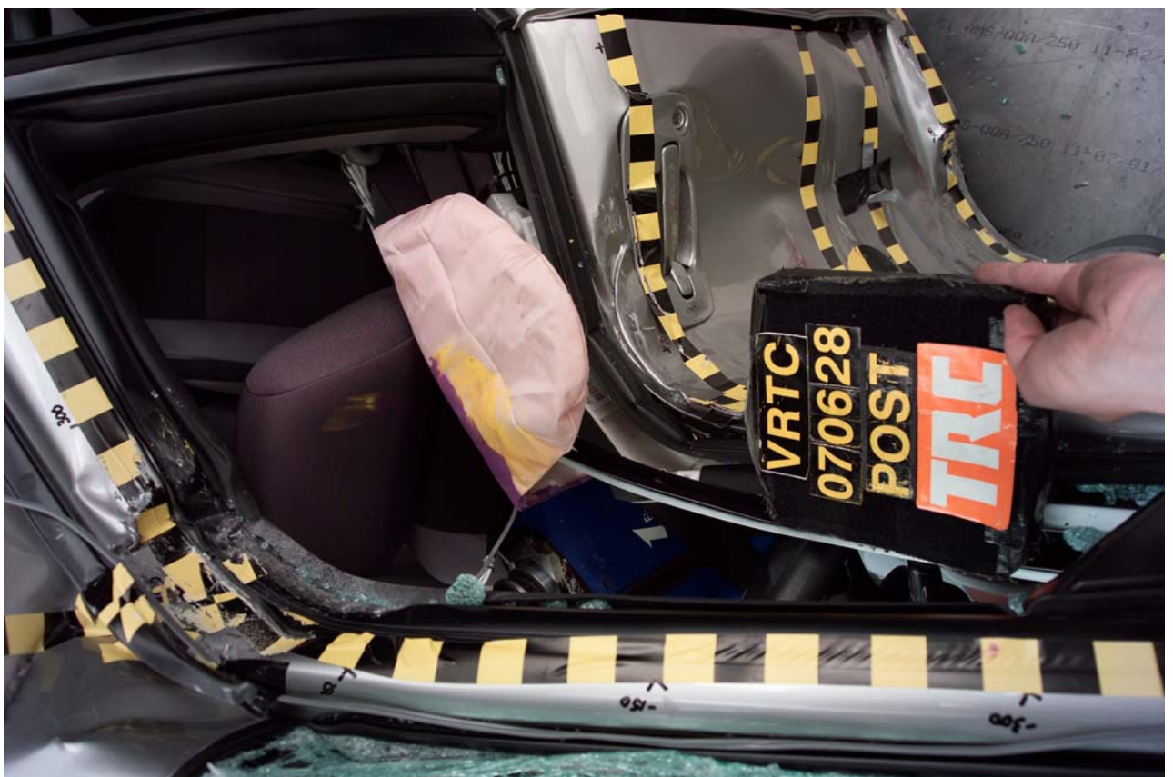
Figure A-31 Post-Test Driver Dummy and Door Clearance View
