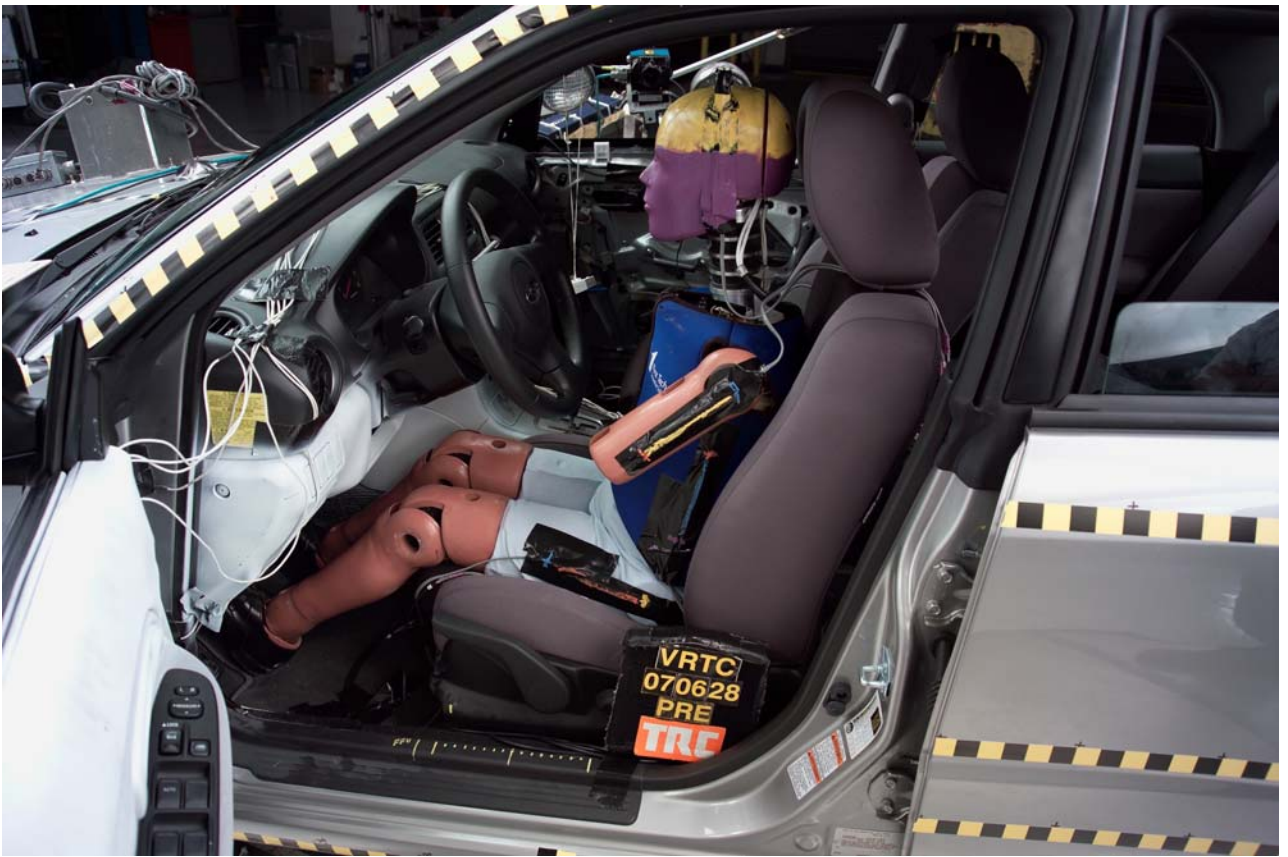
Figure A-32 Pre-Test Driver Dummy Showing Belts, Chalking, and Contact Switches
