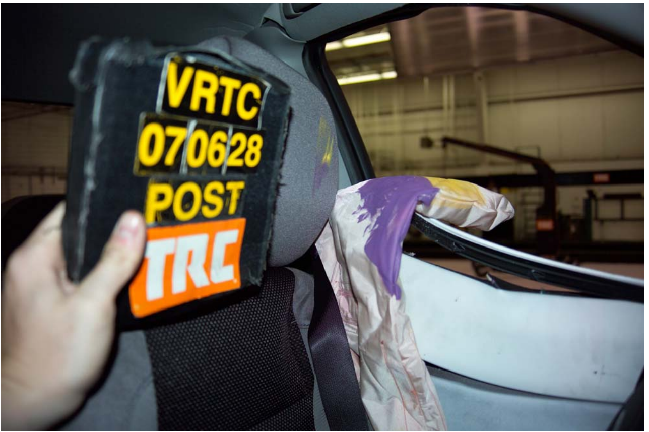
Figure A-35 Post-Test Driver Dummy Head Contact View
