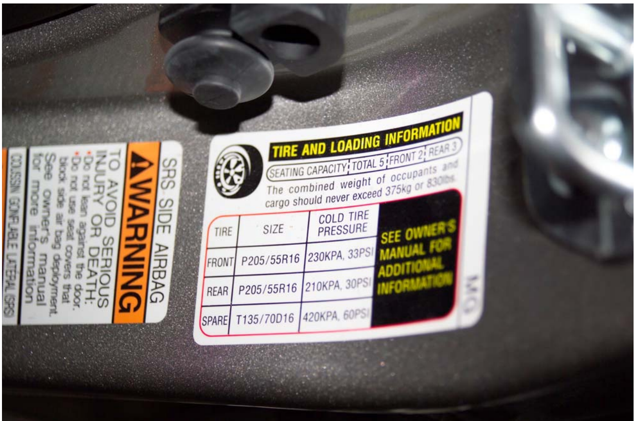
Figure A-38 Recommended Tire Pressure Label View
