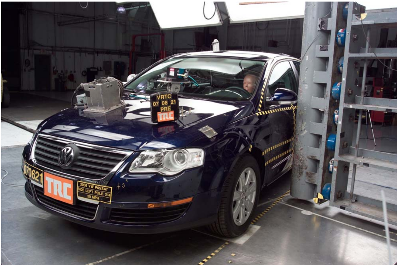
Figure A-19 Pre-Test Left Front Alignment View
