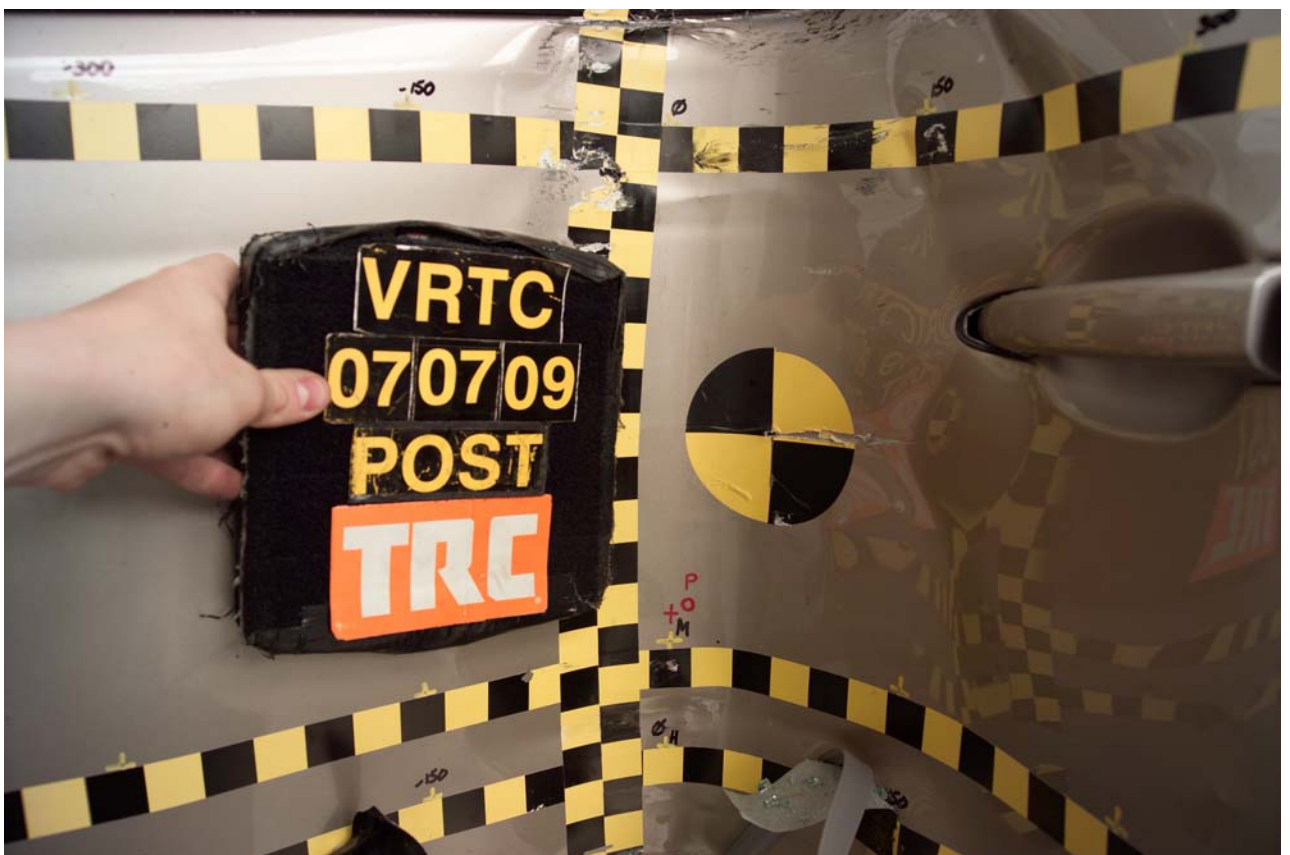
Figure A-20 Post-Test Impact Point View
