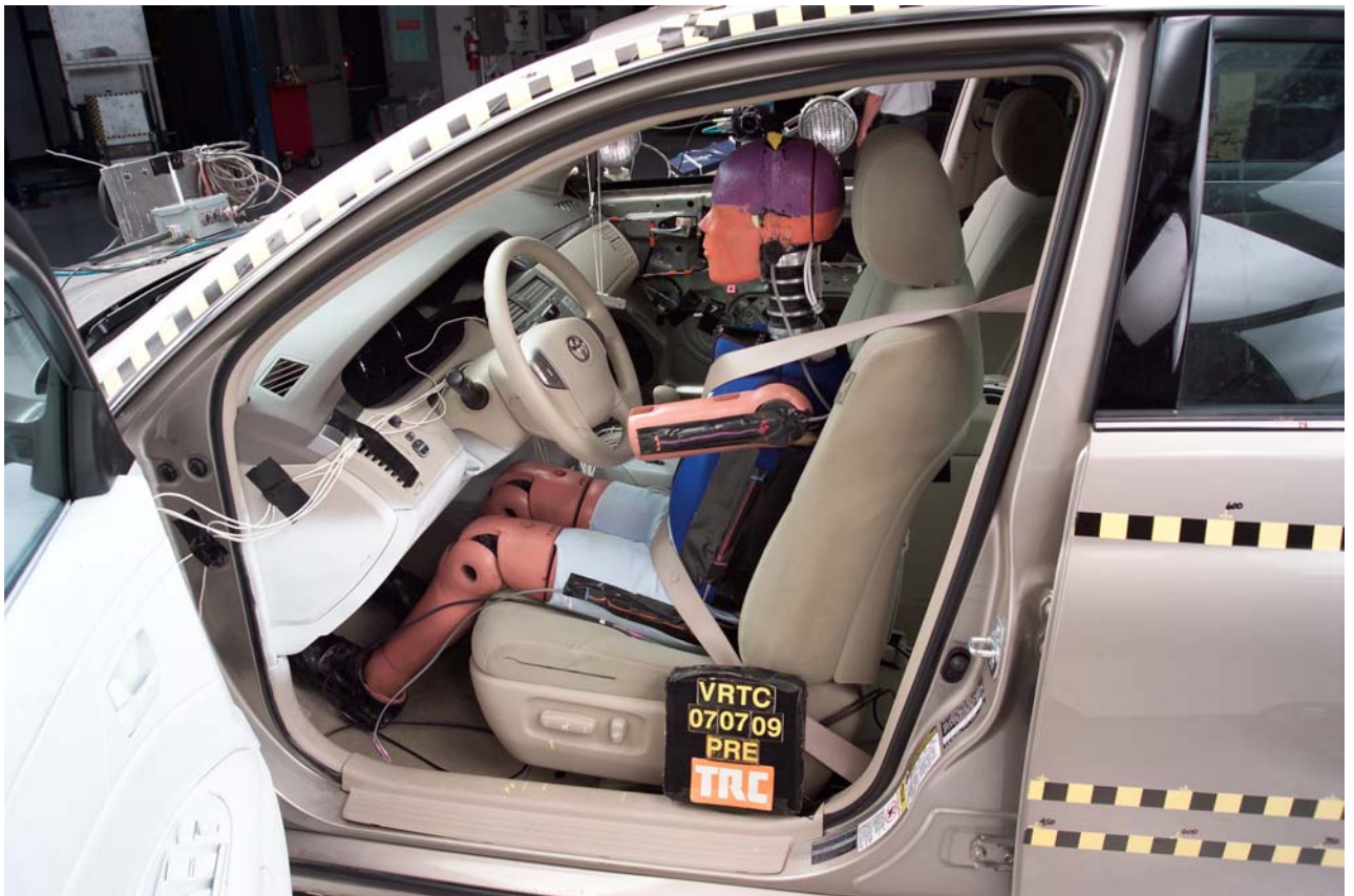
Figure A-33 Pre-Test Driver Dummy Showing Belts, Chalking, and Contact Switches
