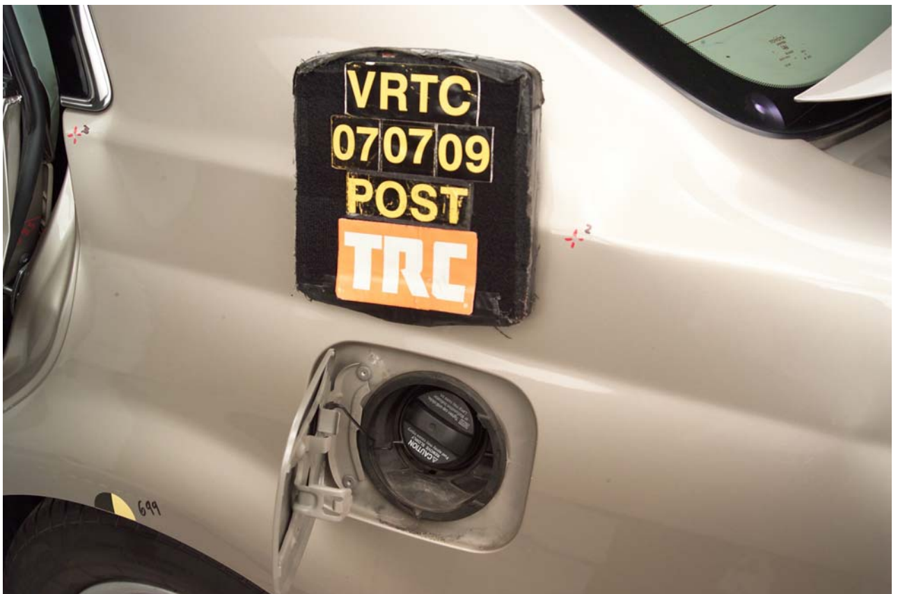
Figure A-24 Post-Test Fuel Filler Cap View
