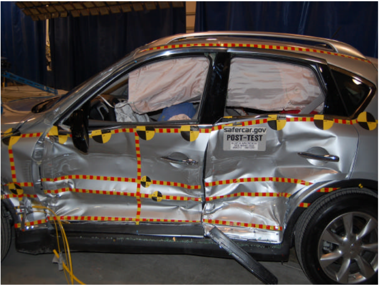
Post-Test Left Side Impact Close-up
