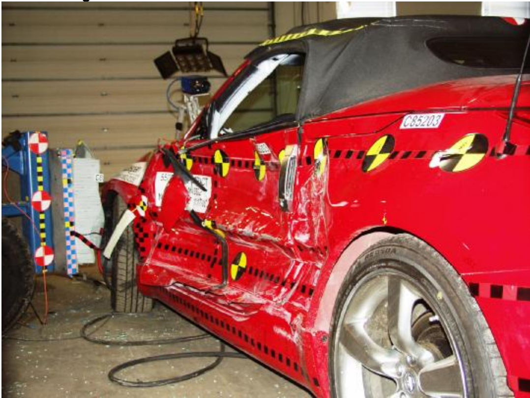
Figure A-44: Post-Test Left Rear \frac{3}{4} View of Left Side Doors
