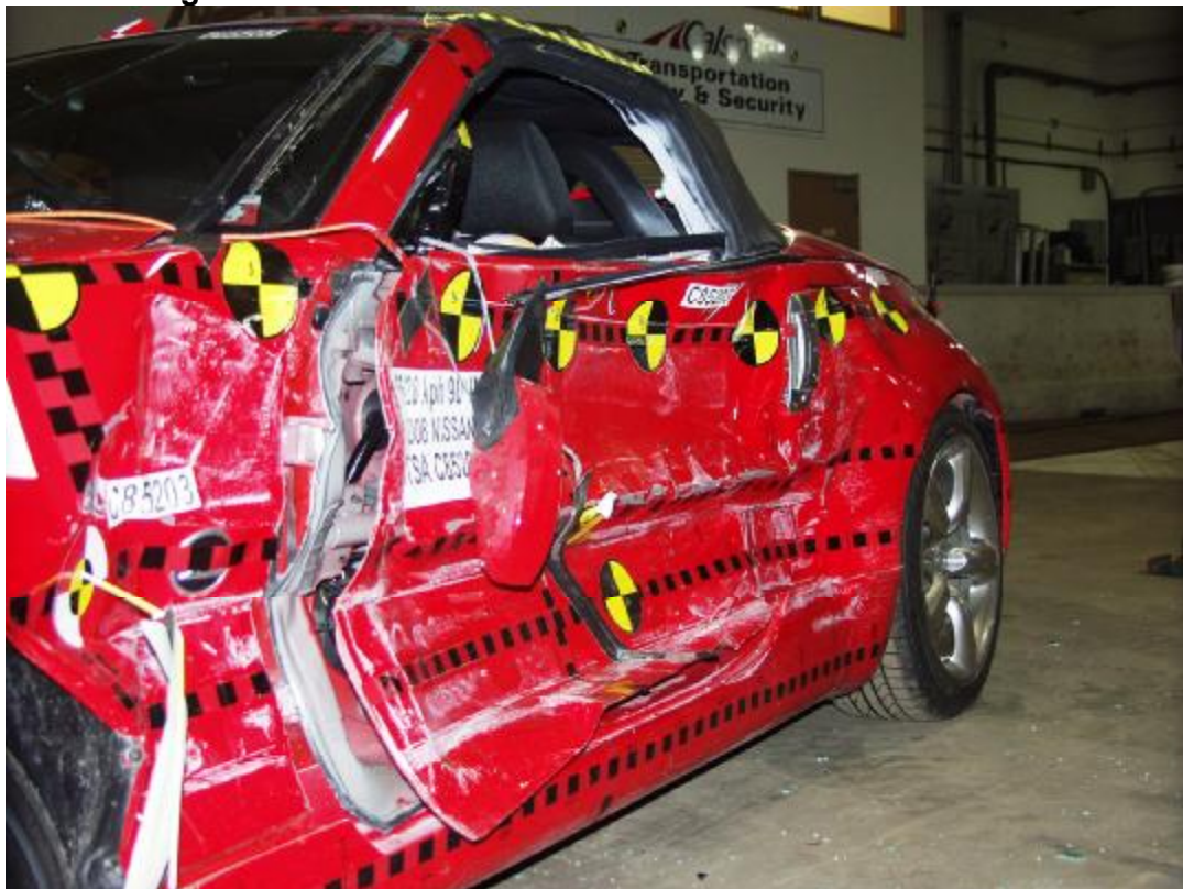
Figure A-42: Post-Test Left Front \frac{3}{4} View of Left Side Doors
