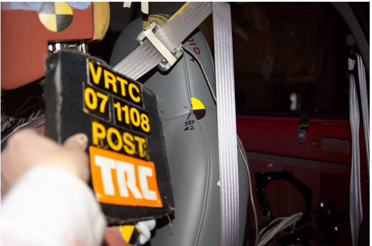
Figure A-69 Post-Test Driver Dummy Belt Spoolout View
