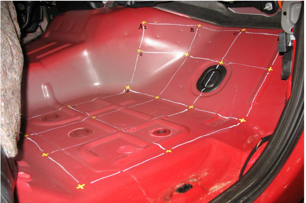
Figure A-127 Pre-Test Passenger Floorpan – View 6
