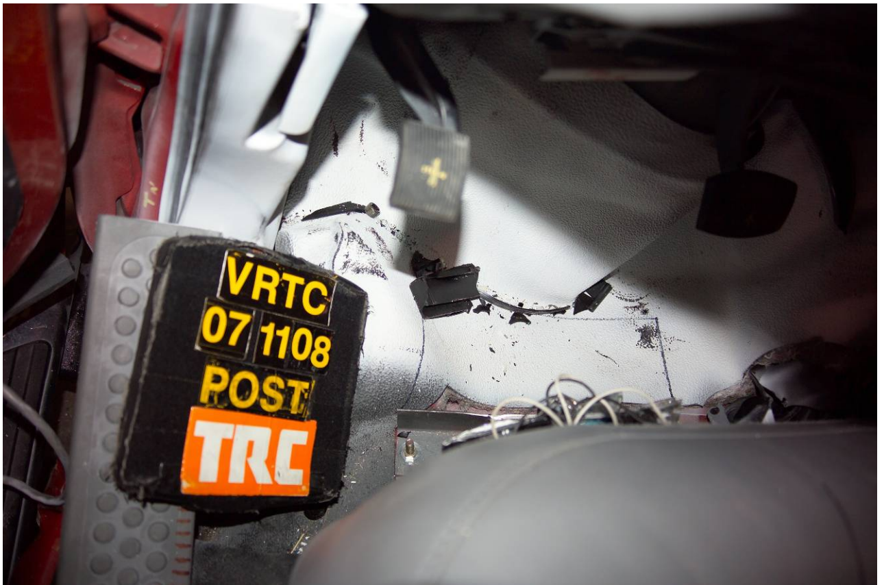
Figure A-62 Post-Test Driver Floorpan Deformation View
