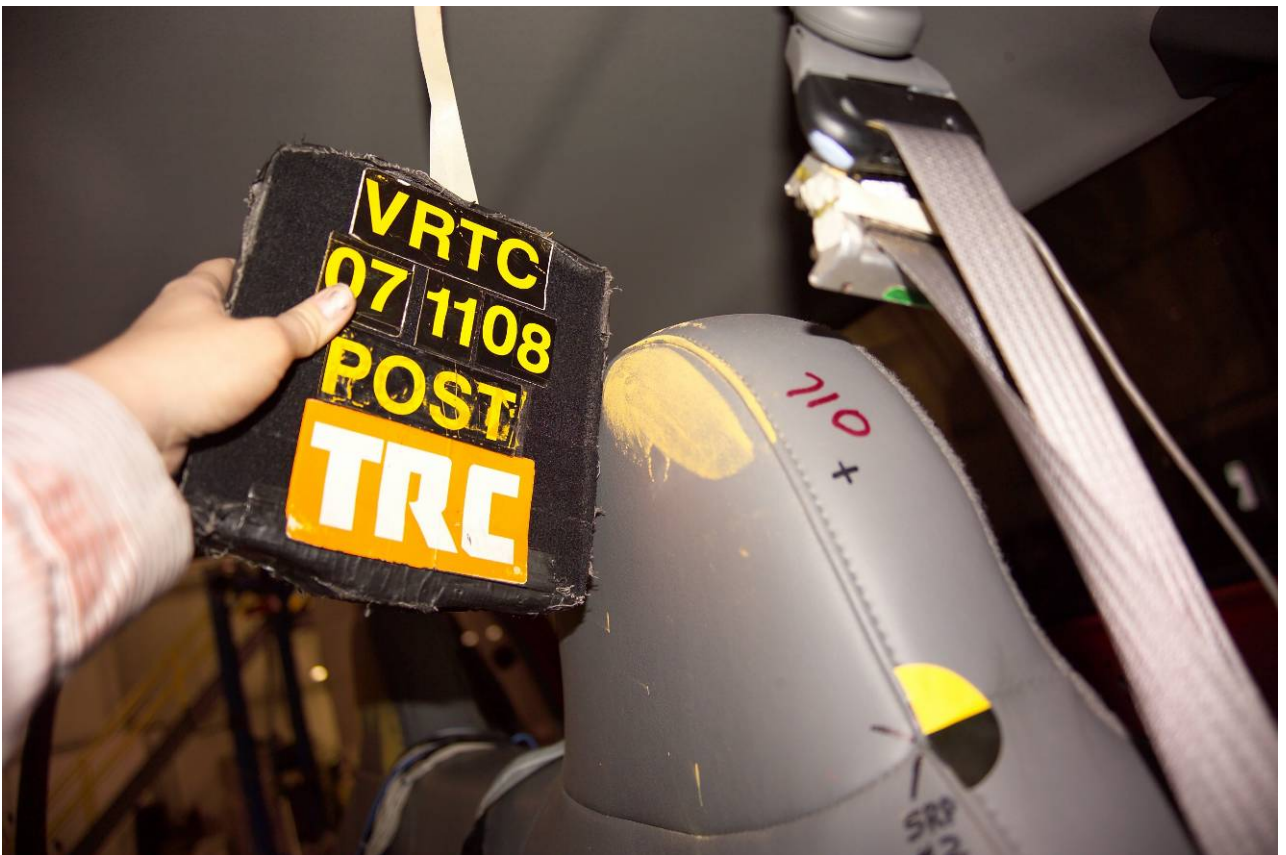
Figure A-65 Post-Test Driver Dummy Head Contact View
