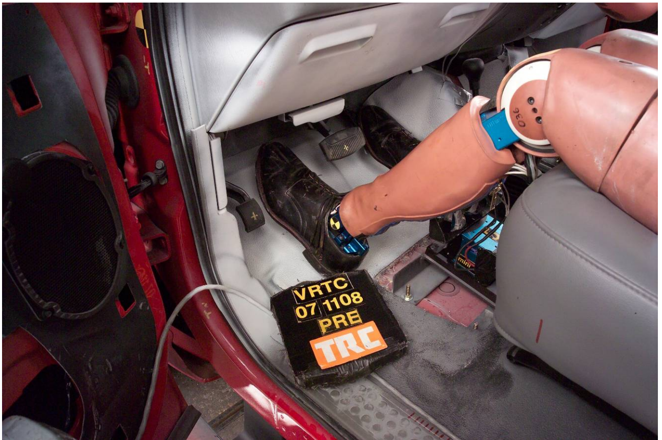
Figure A-59 Pre-Test Driver Dummy Foot Placement View
