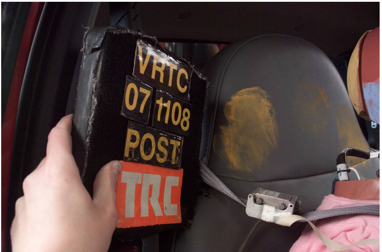
Figure A-81 Post-Test Passenger Dummy Head Contact – View 1
