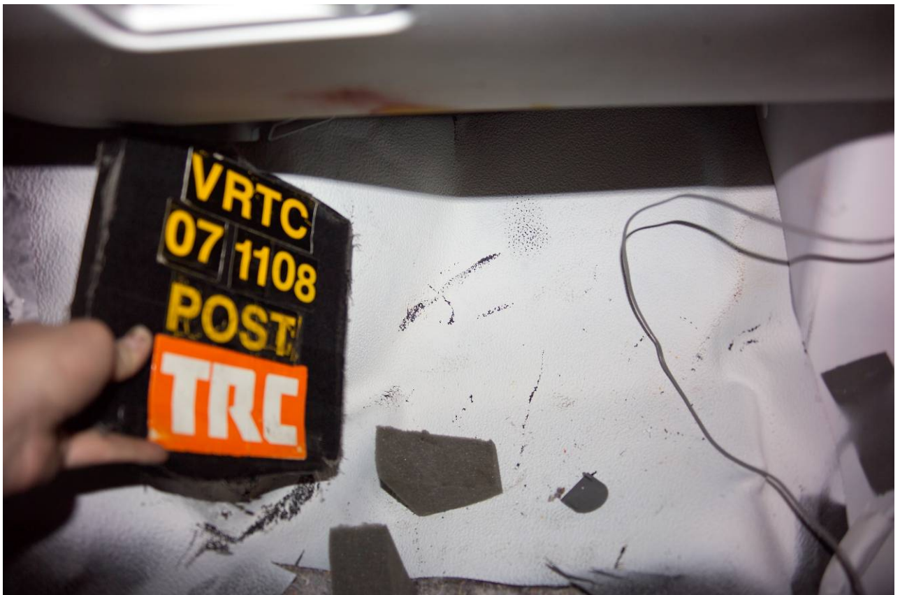
Figure A-79 Post-Test Passenger Toeboard Deformation View
