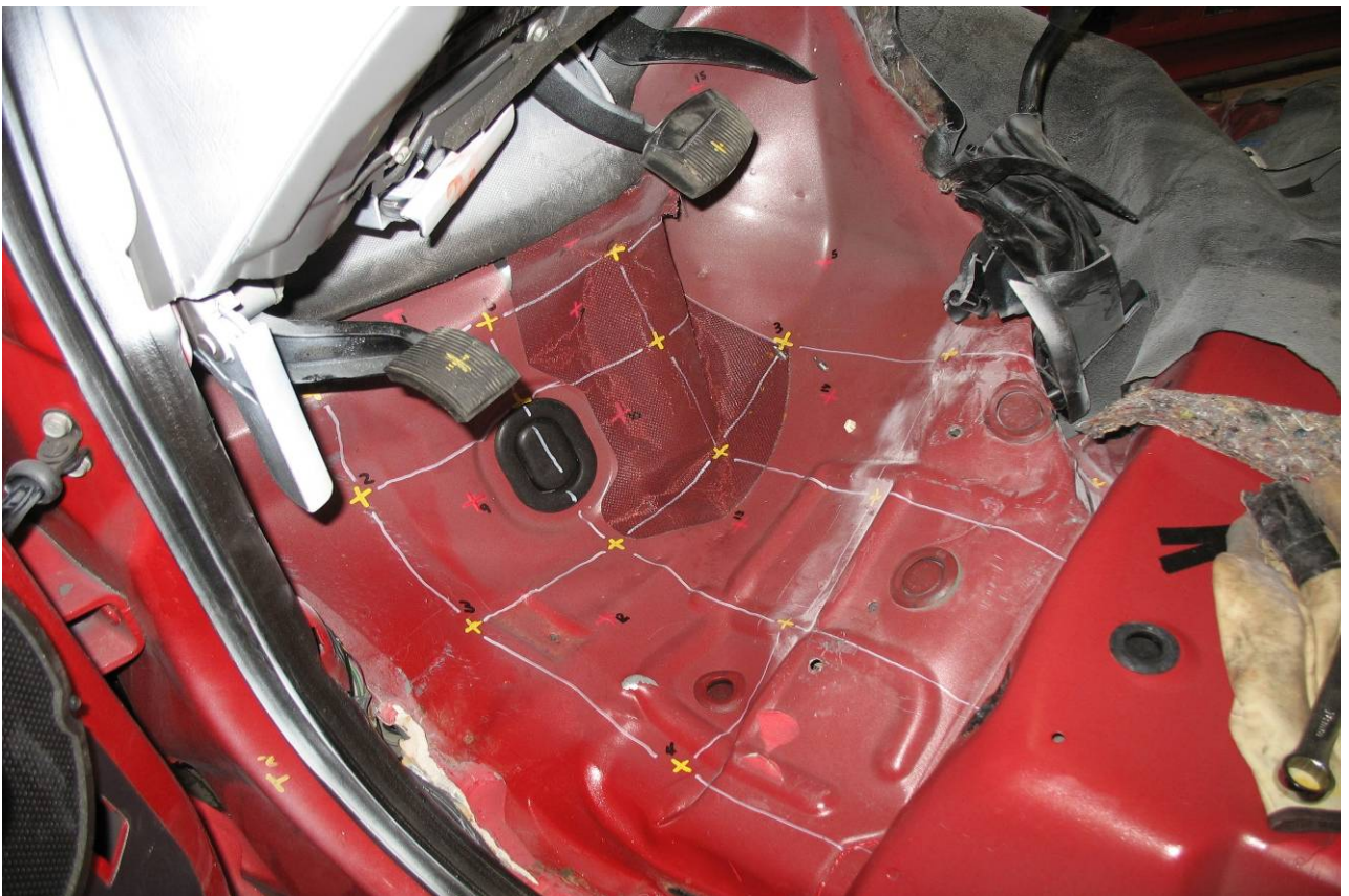
Figure A-110 Post-Test Driver Floorpan – View 6
