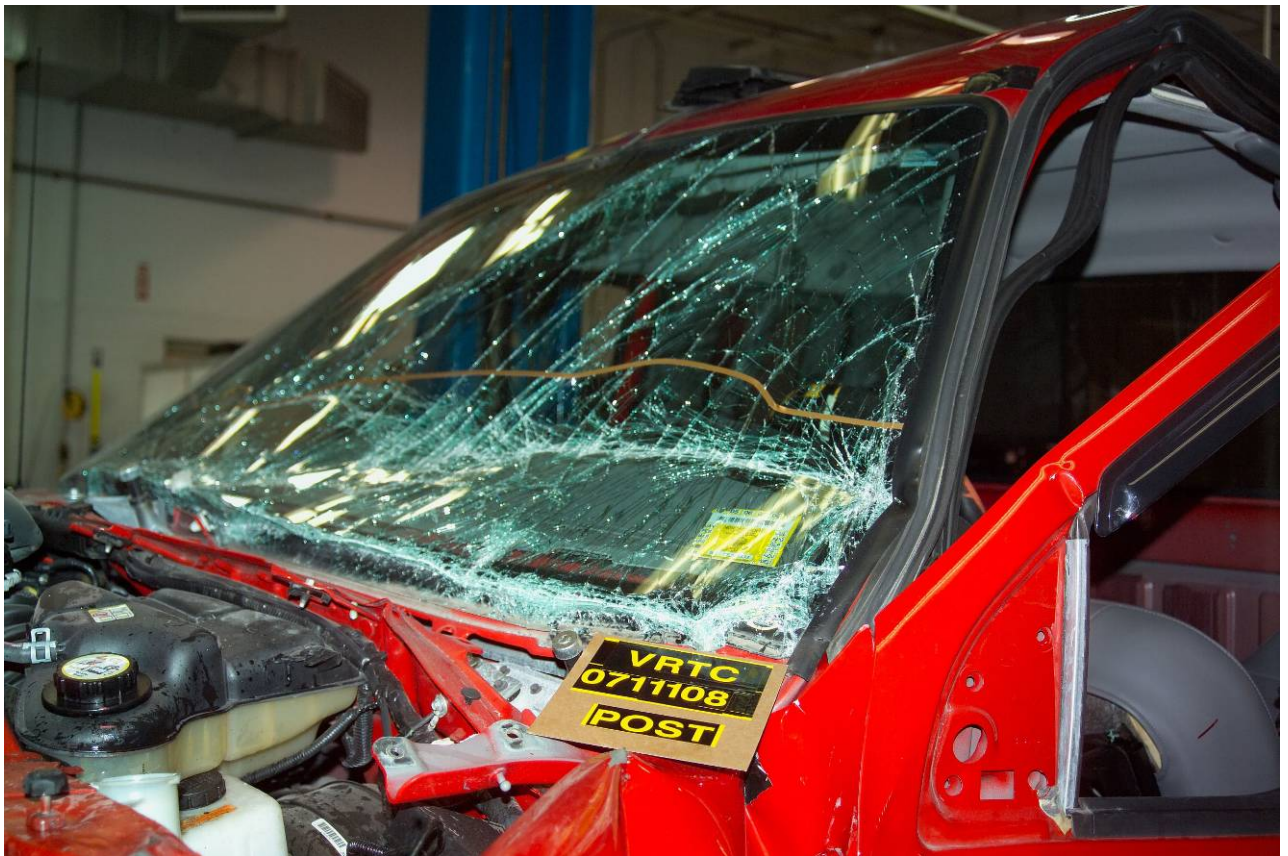
Figure A-45 Post-Test Windshield without Cowl – Left View
