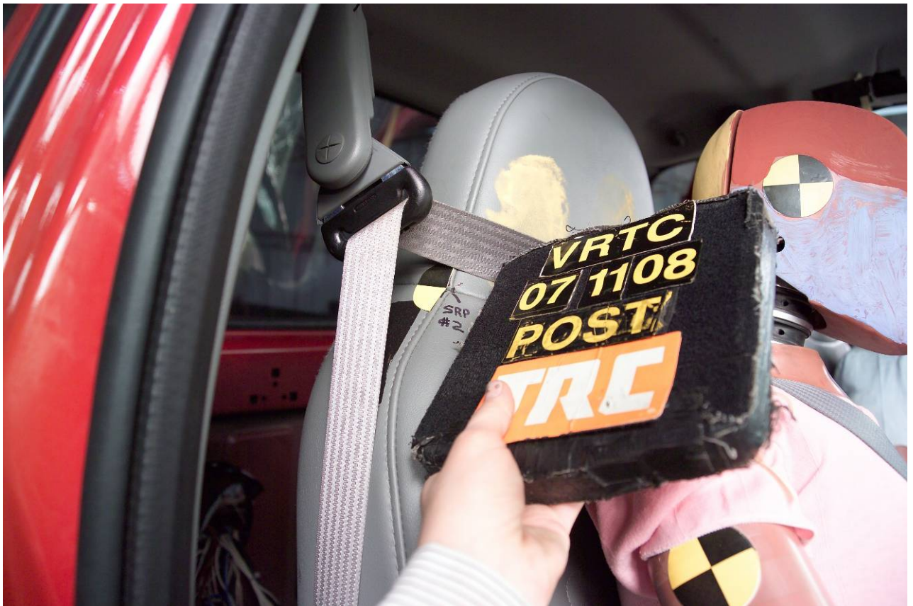
Figure A-82 Post-Test Passenger Dummy Head Contact – View 2
