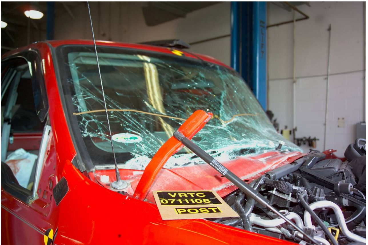
Figure A-47 Post-Test Windshield without Cowl – Right View
