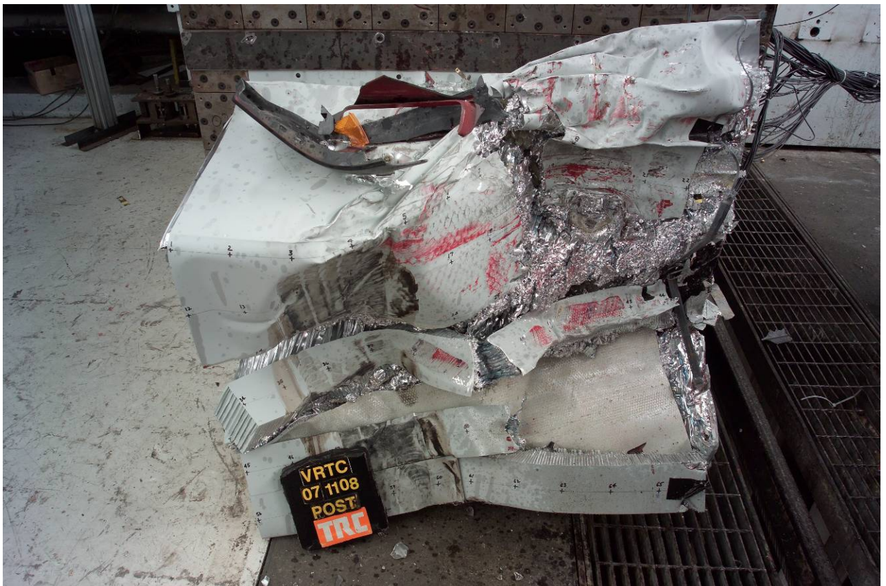
Figure A-88 Post-Test Barrier Front View
