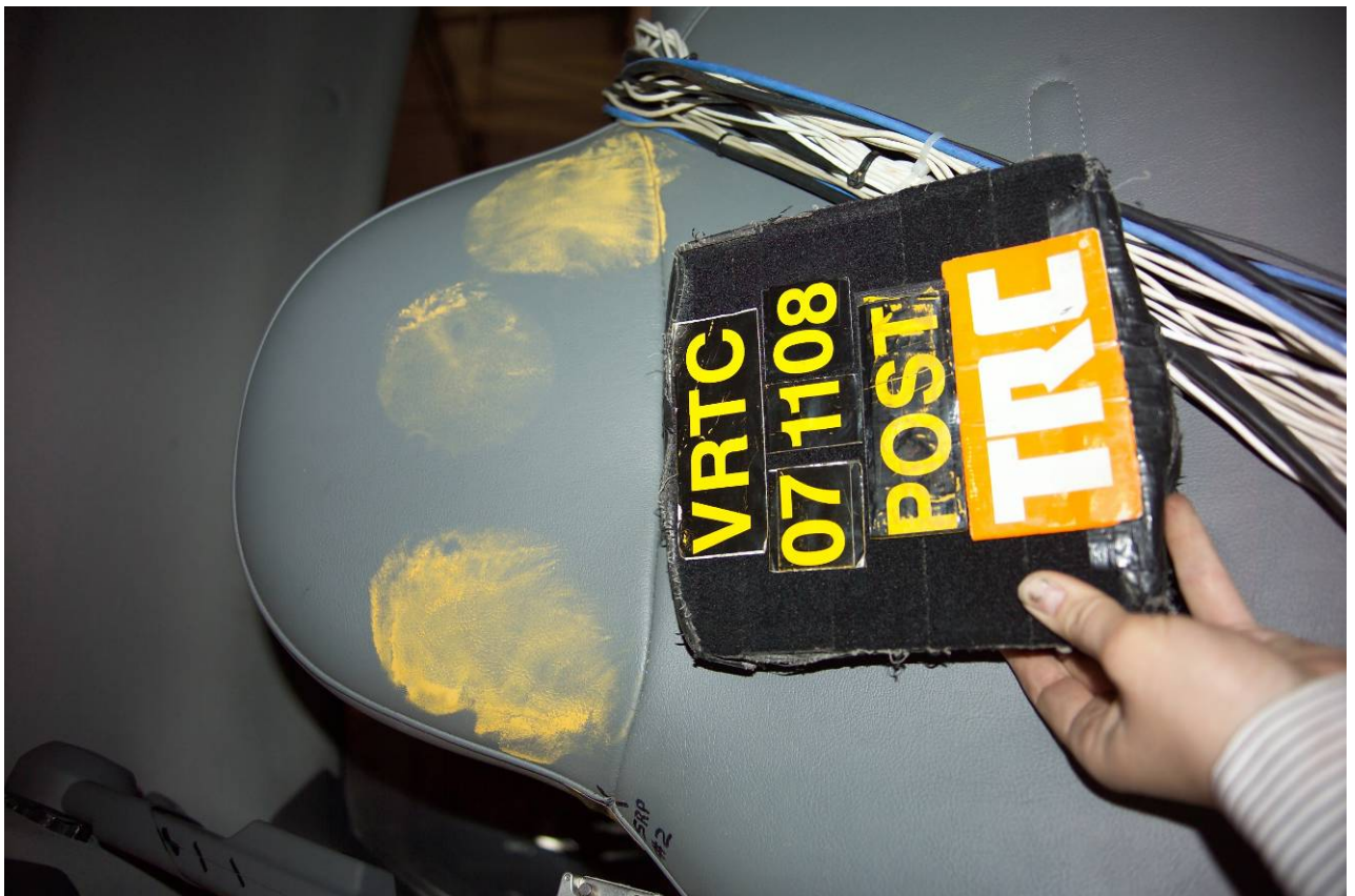
Figure A-83 Post-Test Passenger Dummy Head Contact – View 3
