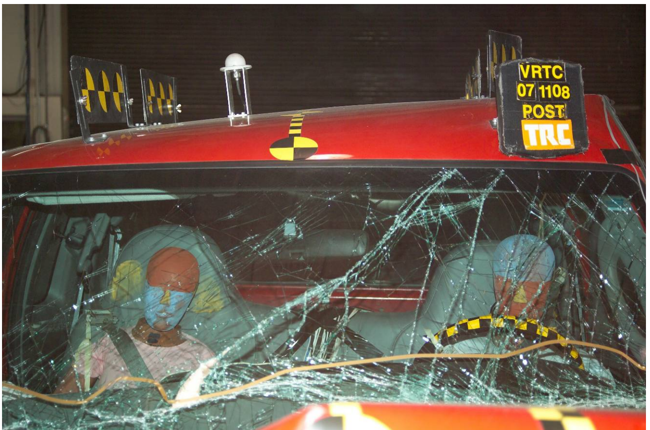
Figure A-49 Post-Test Driver and Passenger Dummies through Windshield View
