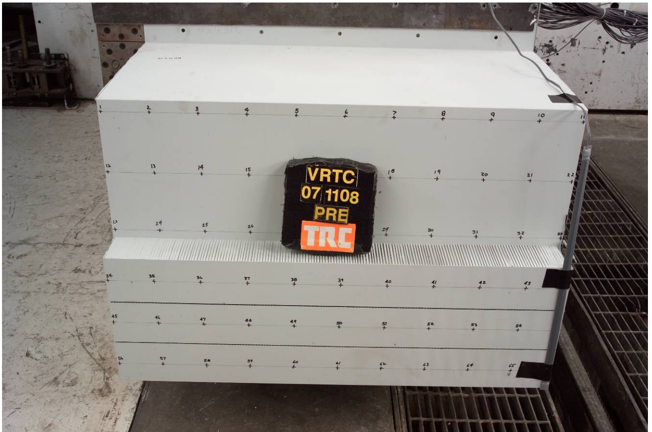
Figure A-87 Pre-Test Barrier Front View
