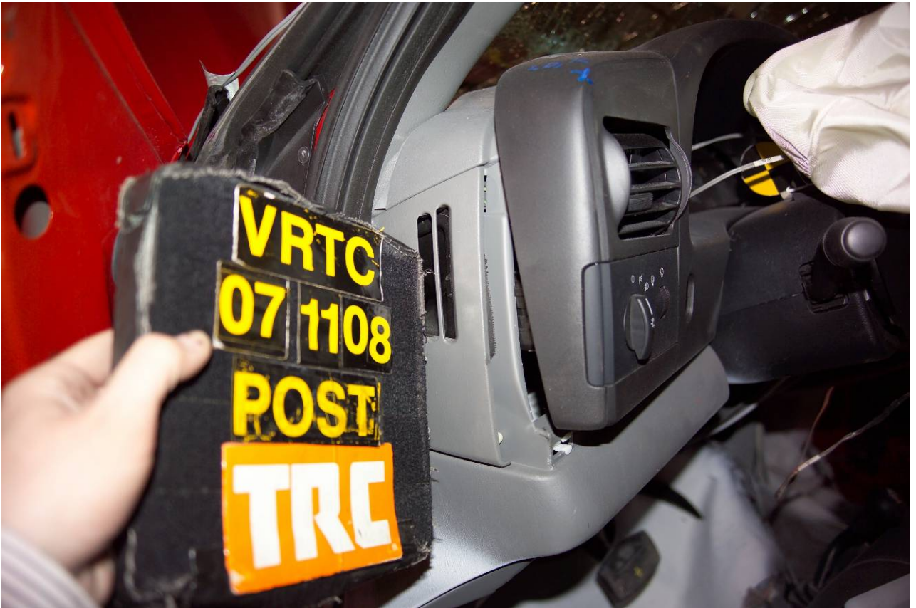
Figure A-68 Post-Test Driver Instrument Panel Damage View
