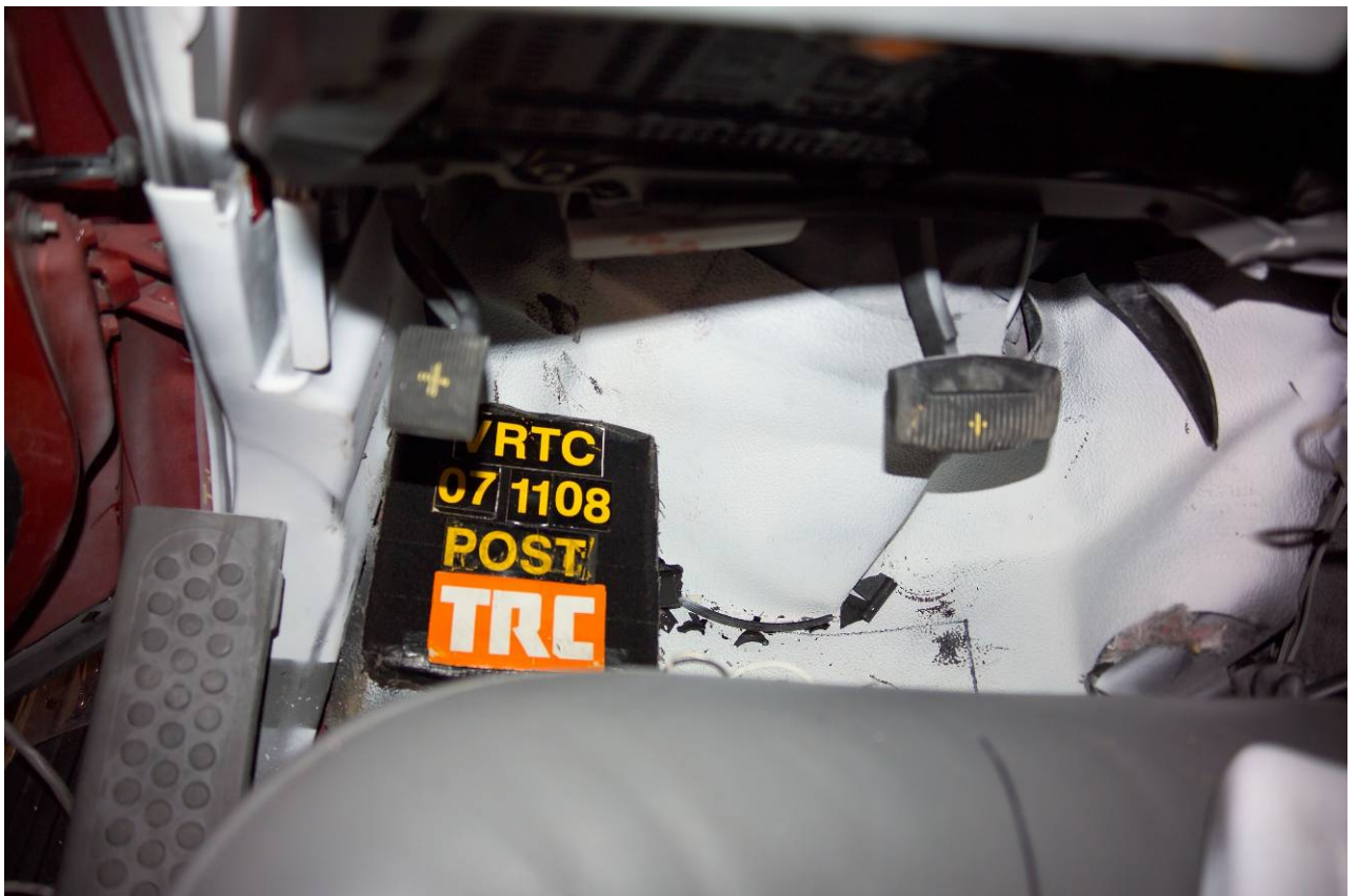
Figure A-63 Post-Test Driver Toeboard Deformation View
