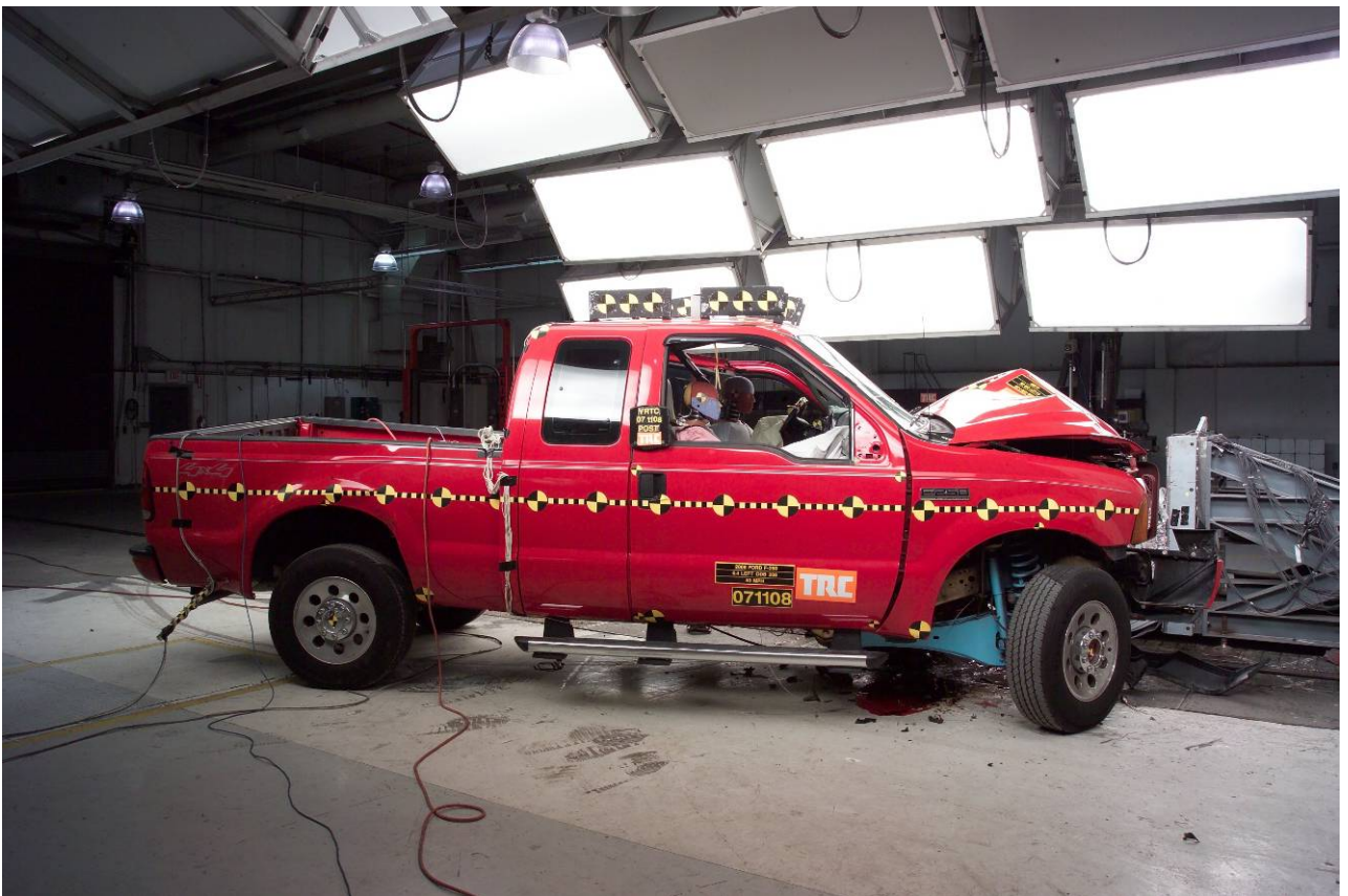
Figure A-14 Post-Test Right Side View
