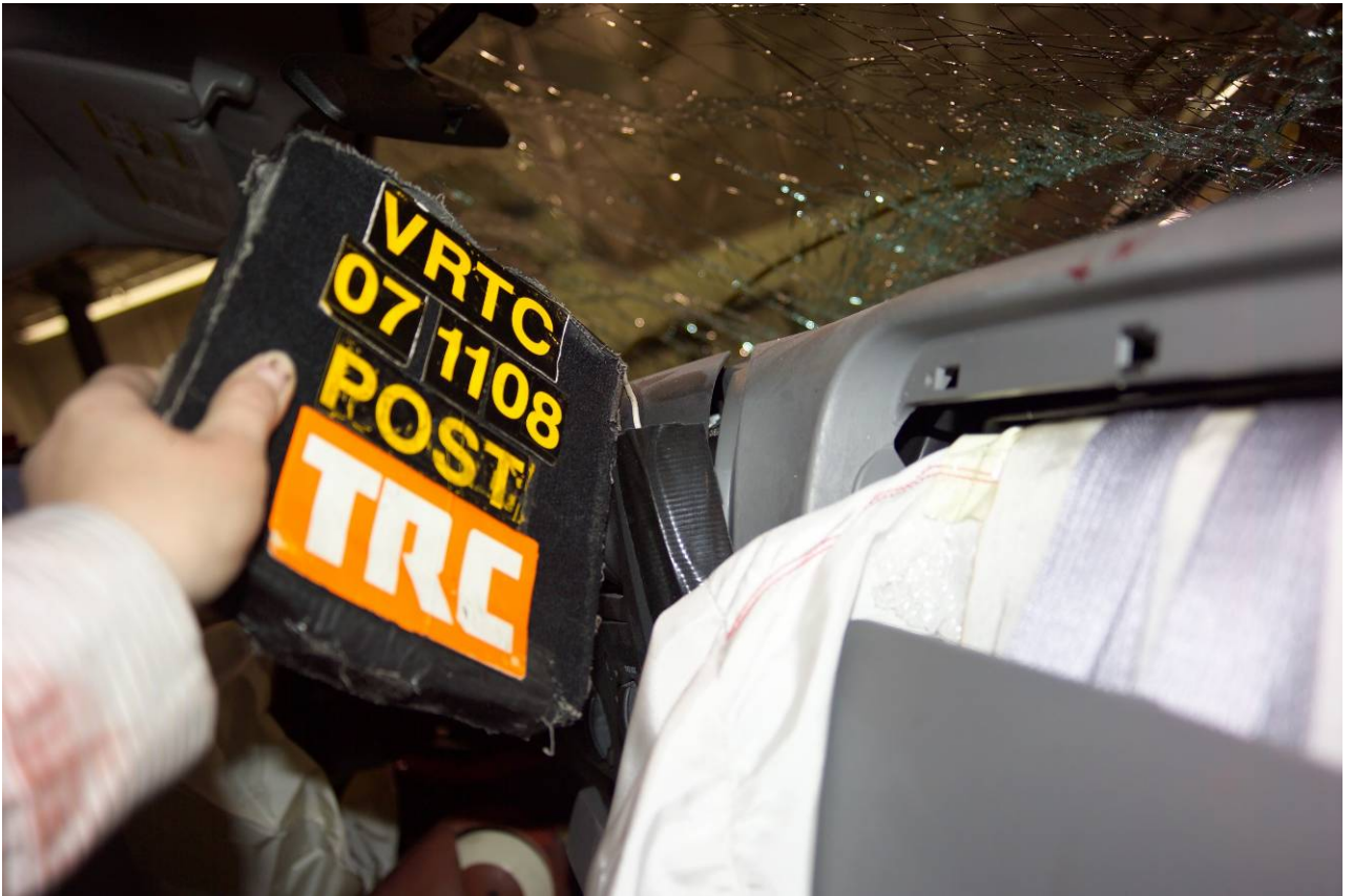
Figure A-86 Post-Test Passenger Dash Damage View
