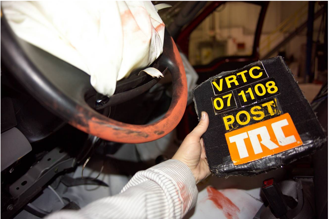
Figure A-66 Post-Test Driver Dummy Chest Contact View
