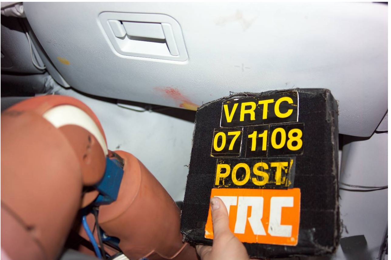
Figure A-85 Post-Test Passenger Dummy Knee Contact View
