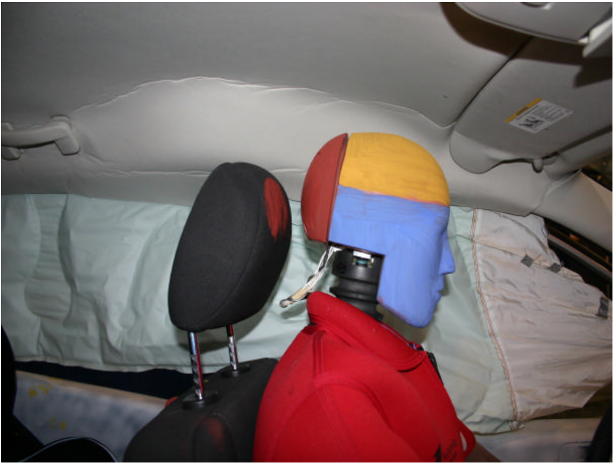
Post-Test Driver Dummy Head Contact
