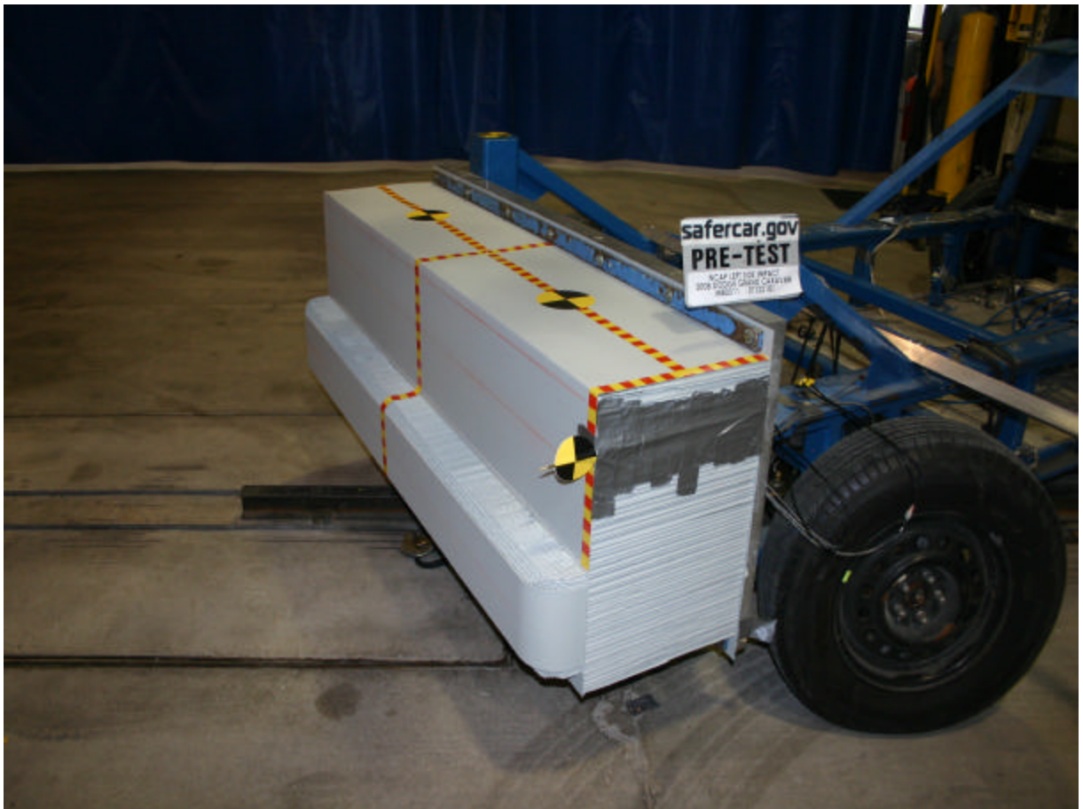
Pre-Test Left Side View of Deformable Barrier
