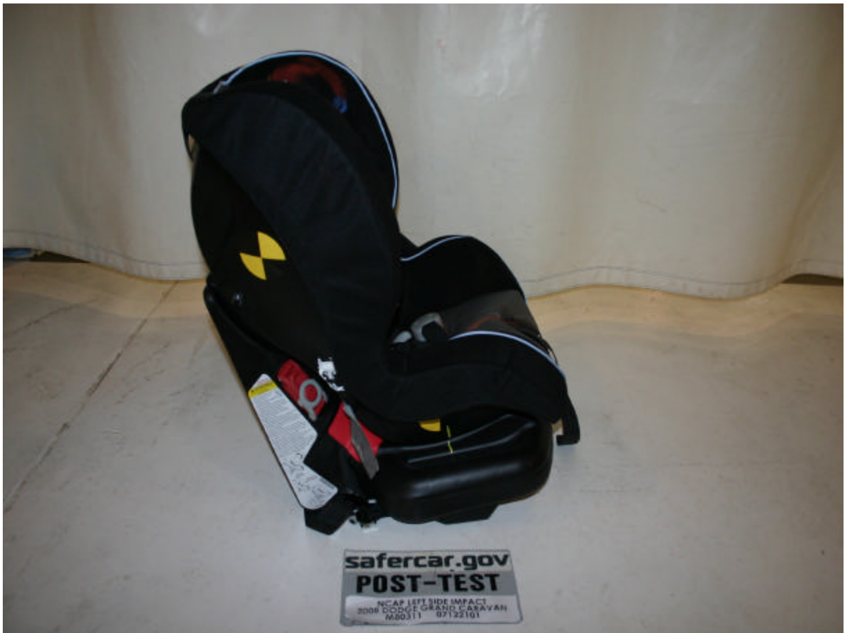
Post-Test Right Side View of Position 4 CRS
