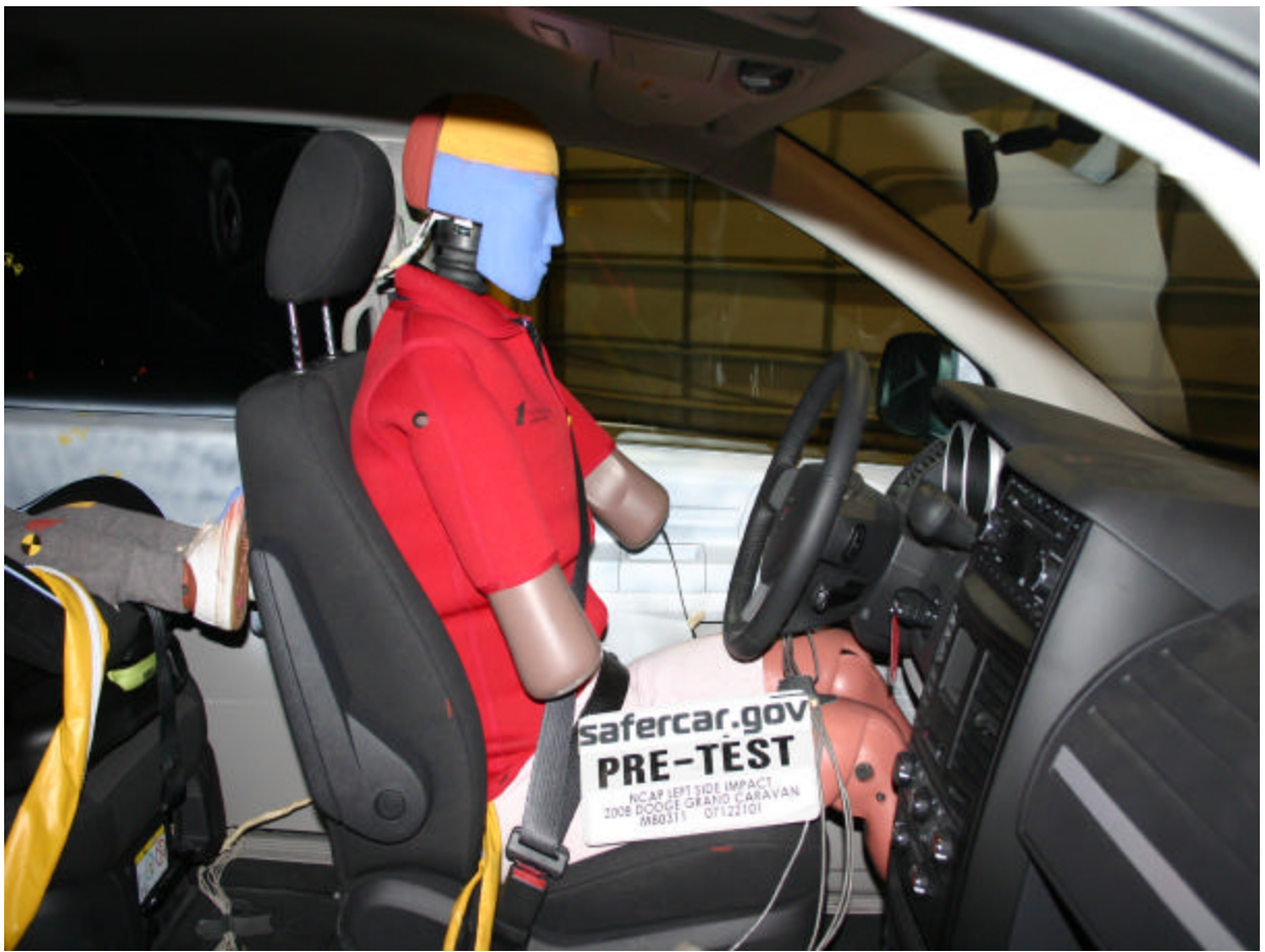
Pre-Test Driver Dummy Right Side View
