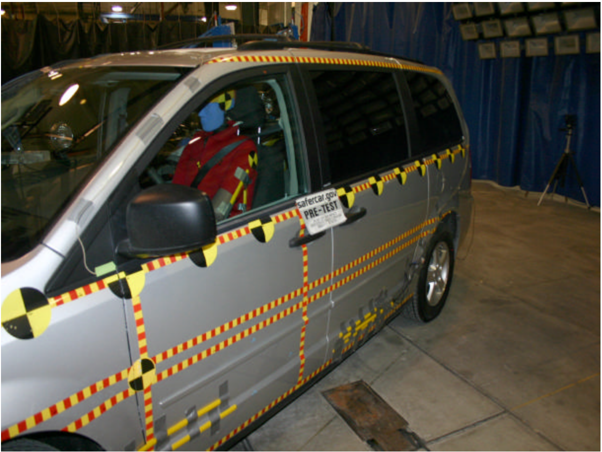
Pre-Test Front 3/4 View of Left Side Doors
