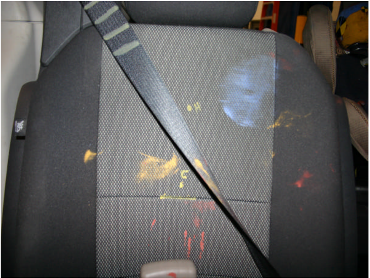
Post-Test Position 3 Head and Feet Contact
