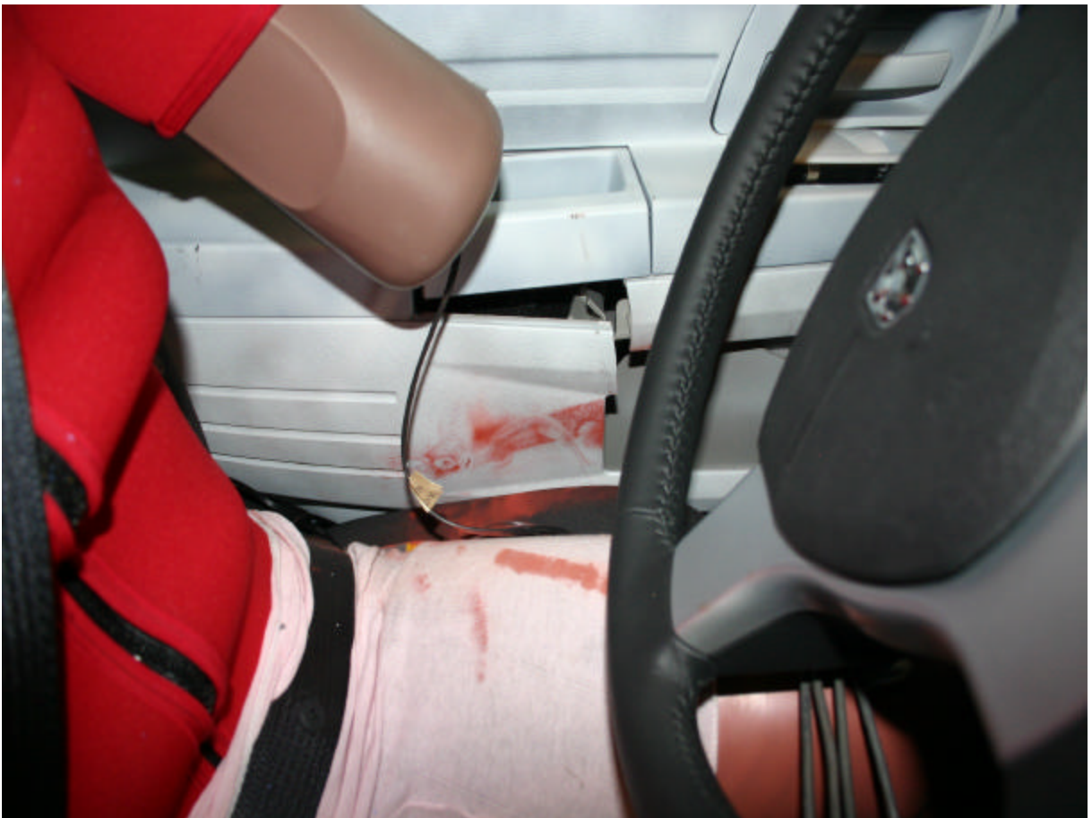
Post-Test Driver Dummy Torso Contact
