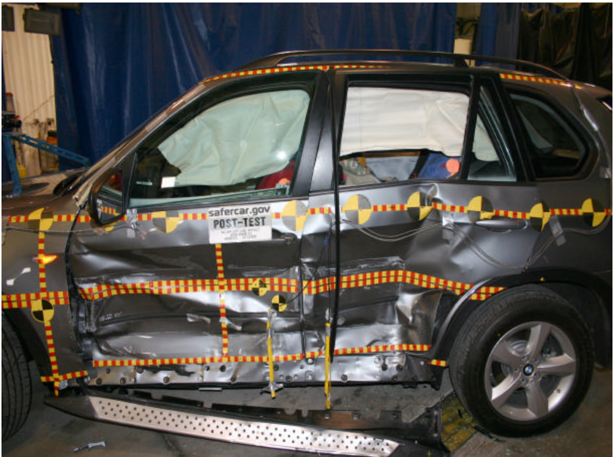
Post-Test Left Side Impact Close-up
