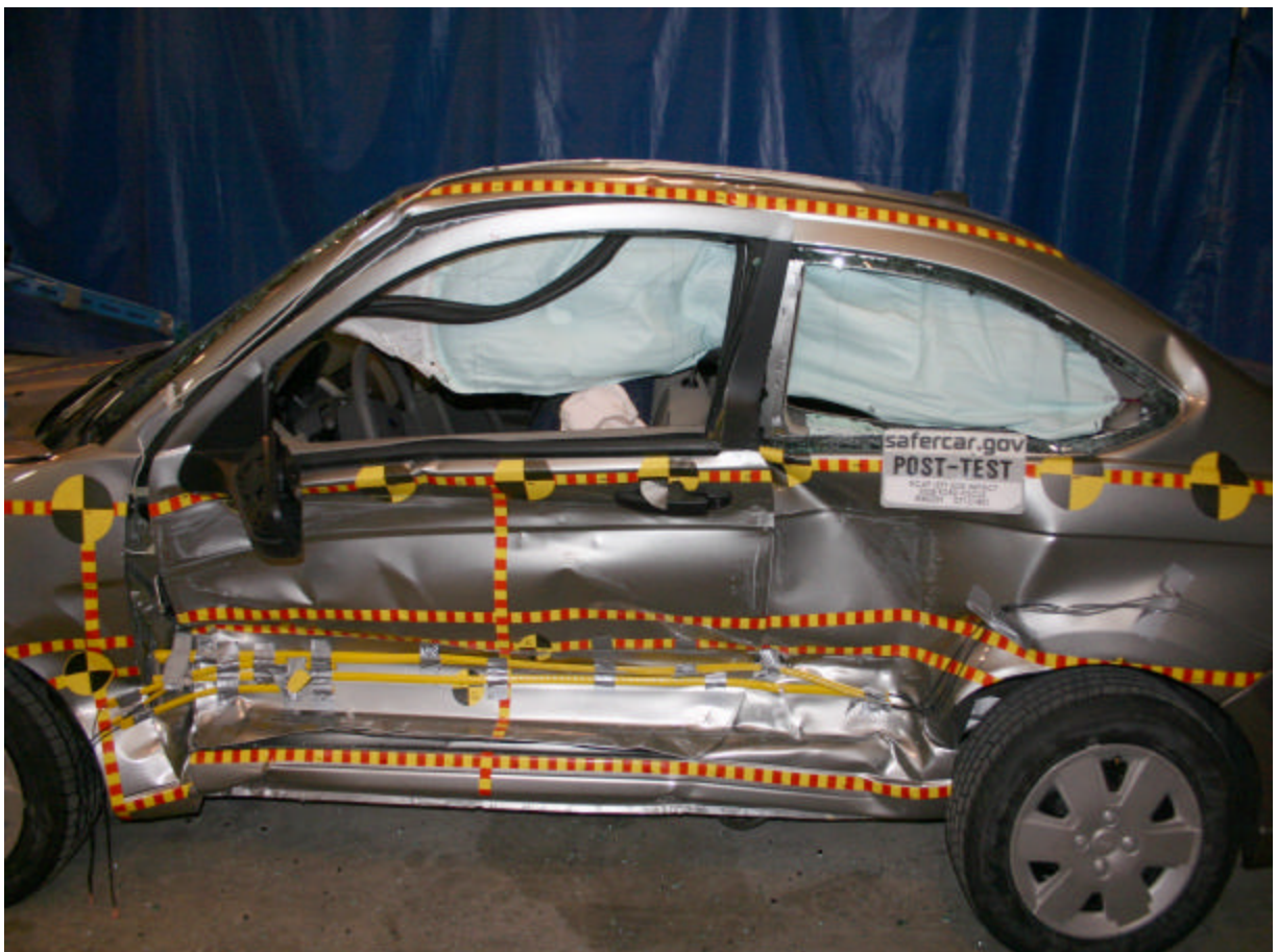
Post-Test Left Side Impact Close-up
