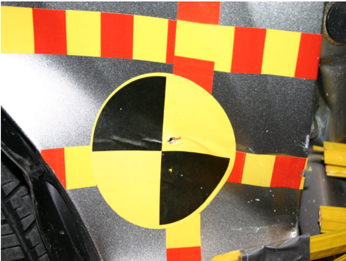
Post-Test Left Impact Point
