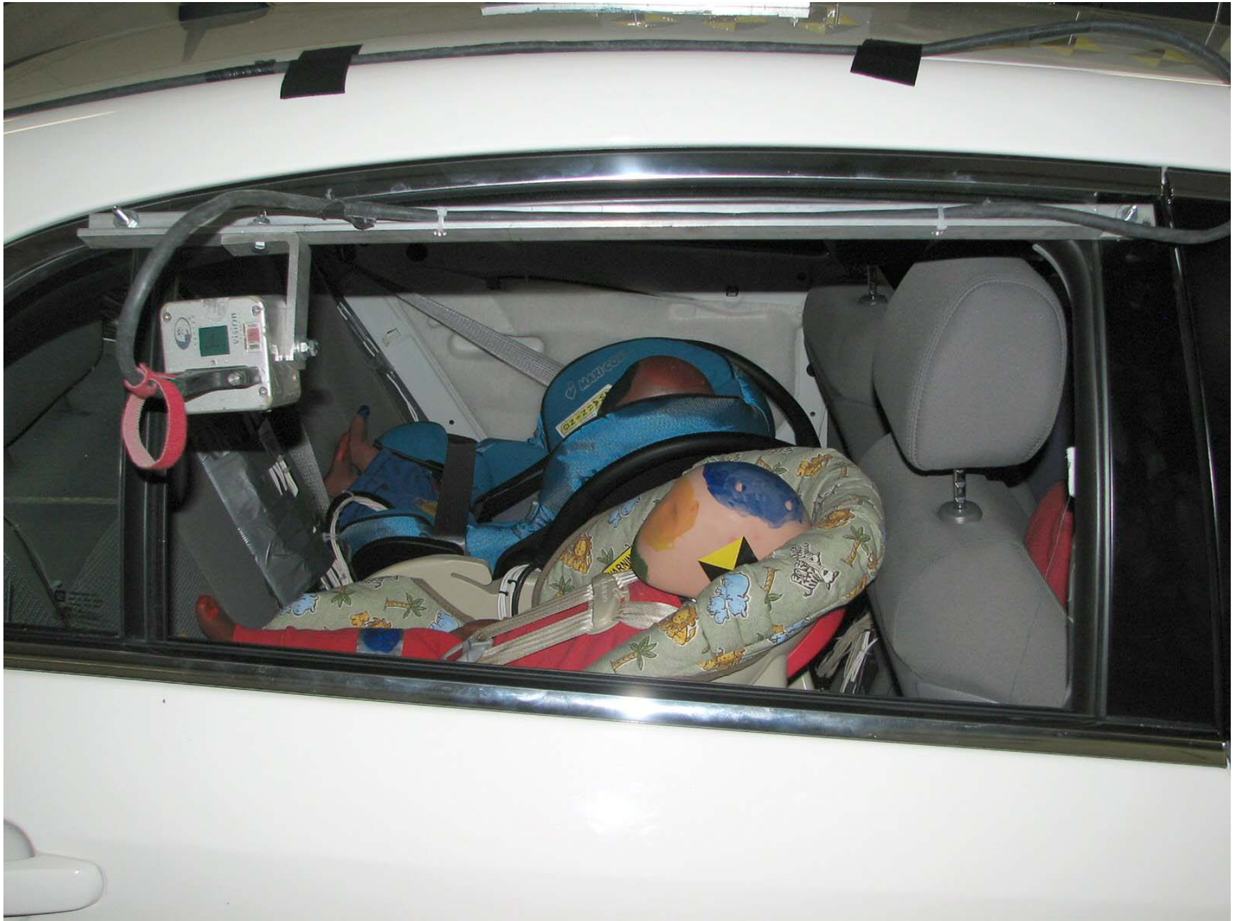
Figure D2-16: Pre-Test Position 3 Right Side View (Through Window)
