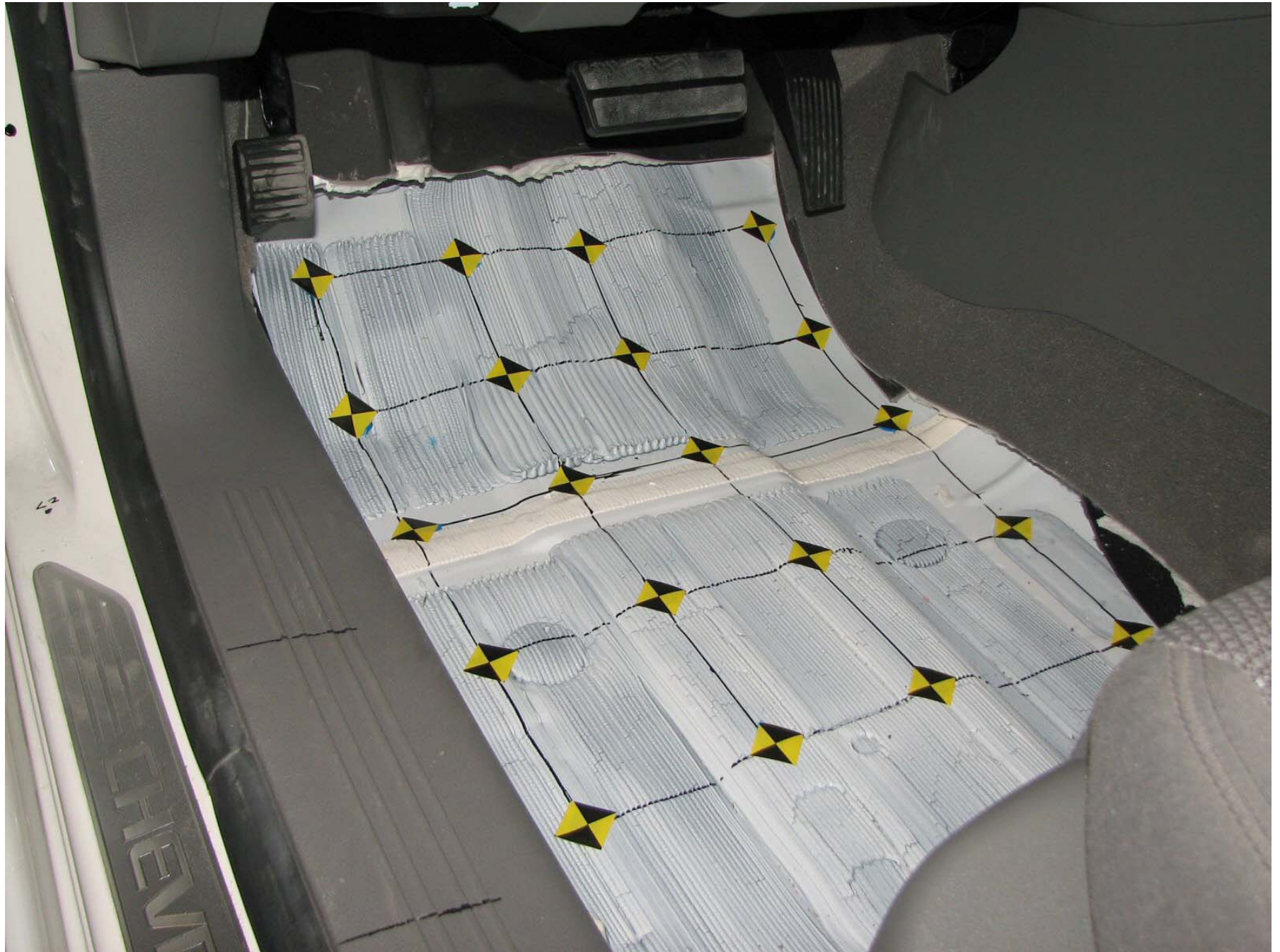
Figure A-40: Pre-Test Driver Side Floor Pan
