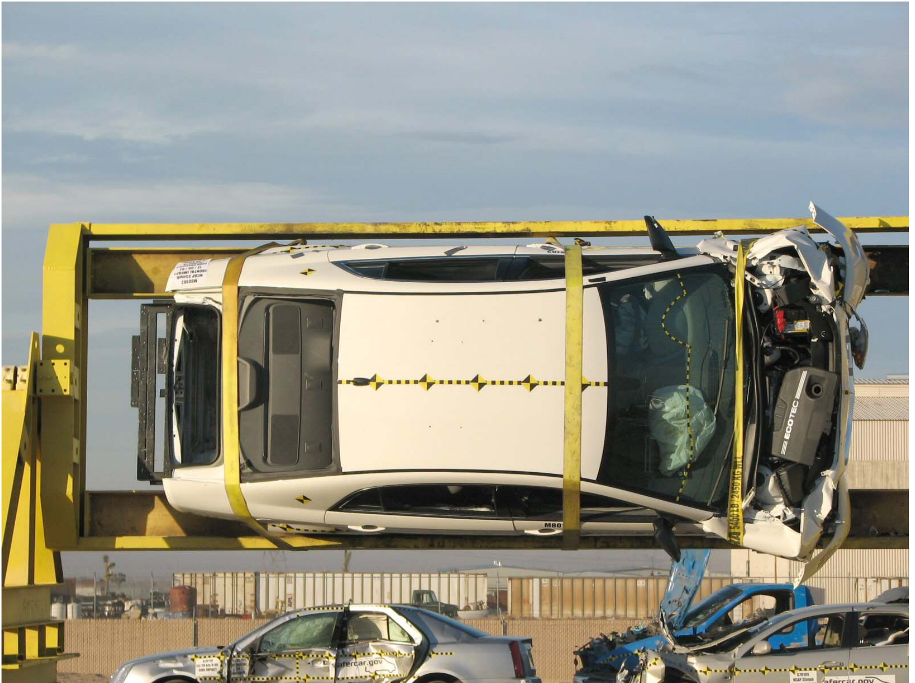
Figure A-59: Vehicle on Rollover Device (90°)
