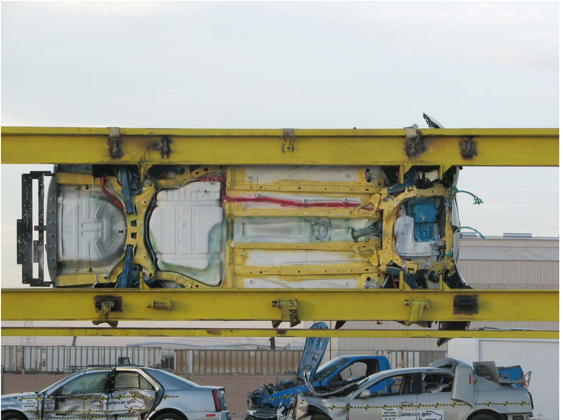
Figure A-61: Vehicle on Rollover Device (270°)
