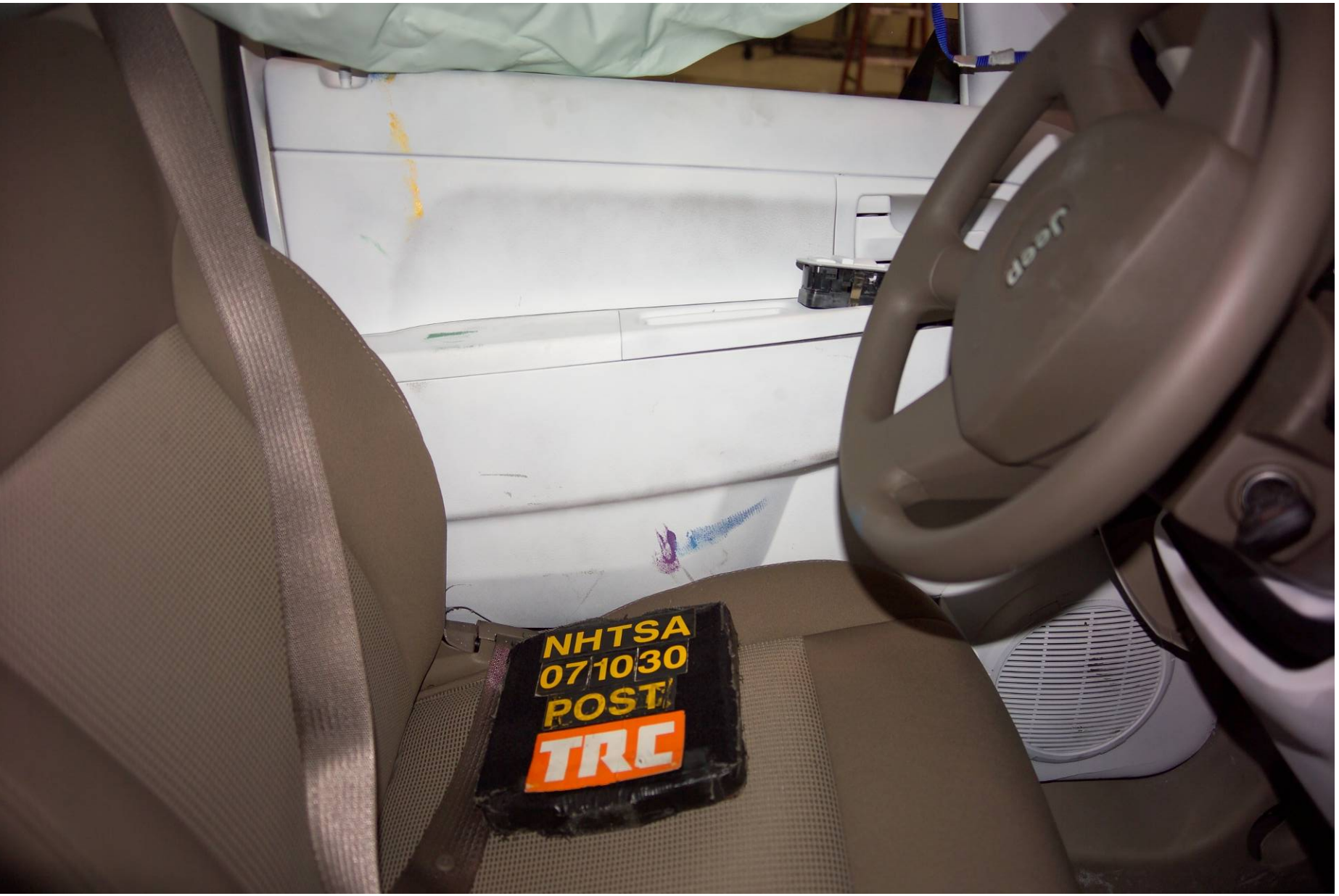
Figure A-61 Post-Test Interior of Front Door Showing SID Impact Locations
