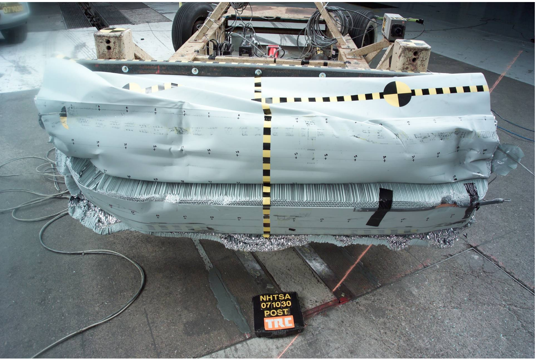
Figure A-43 Post-Test View of MDB Showing Contact Switches in Place
