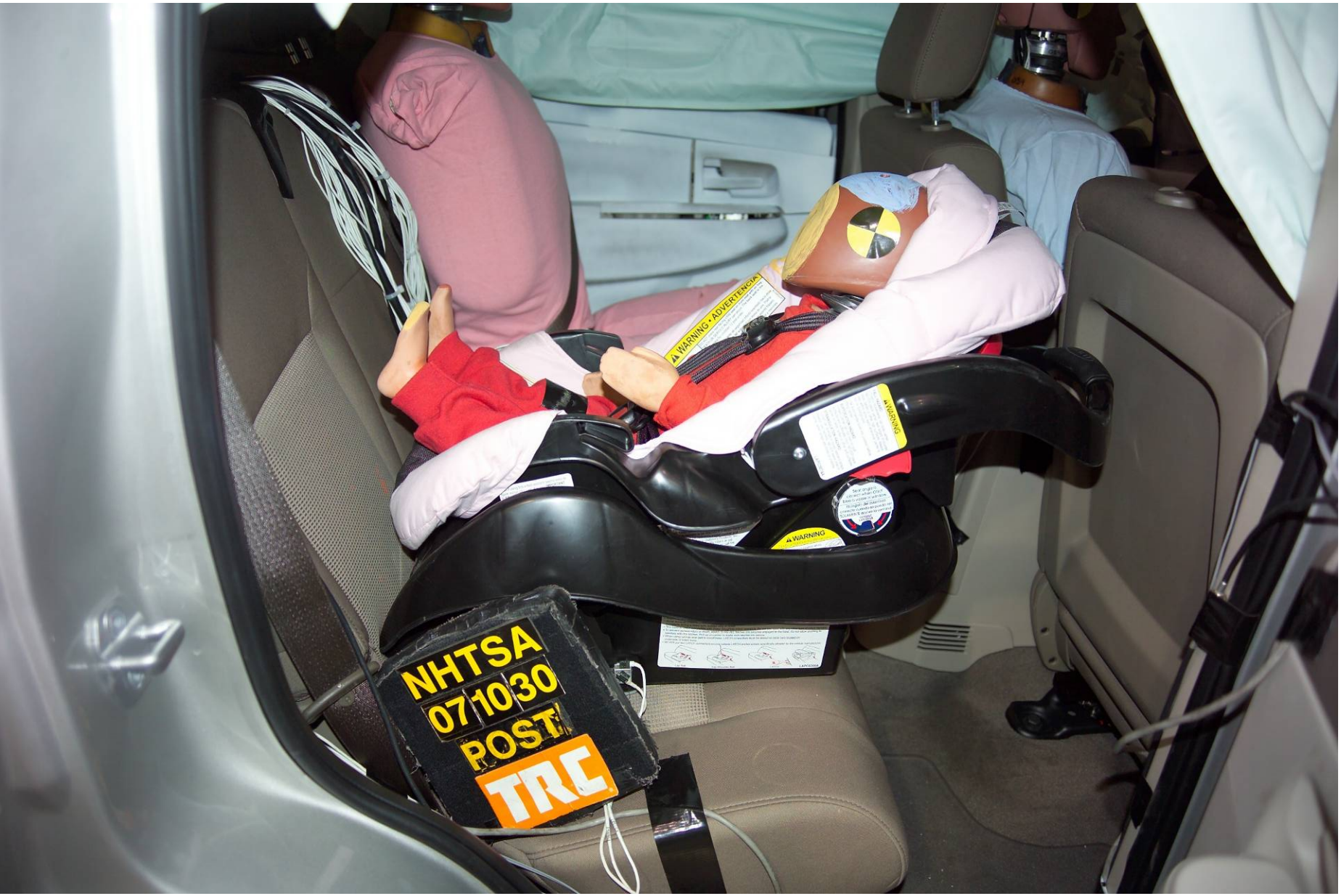
Figure D2-13 Post-Test Right Side View of Right Rear Dummy
