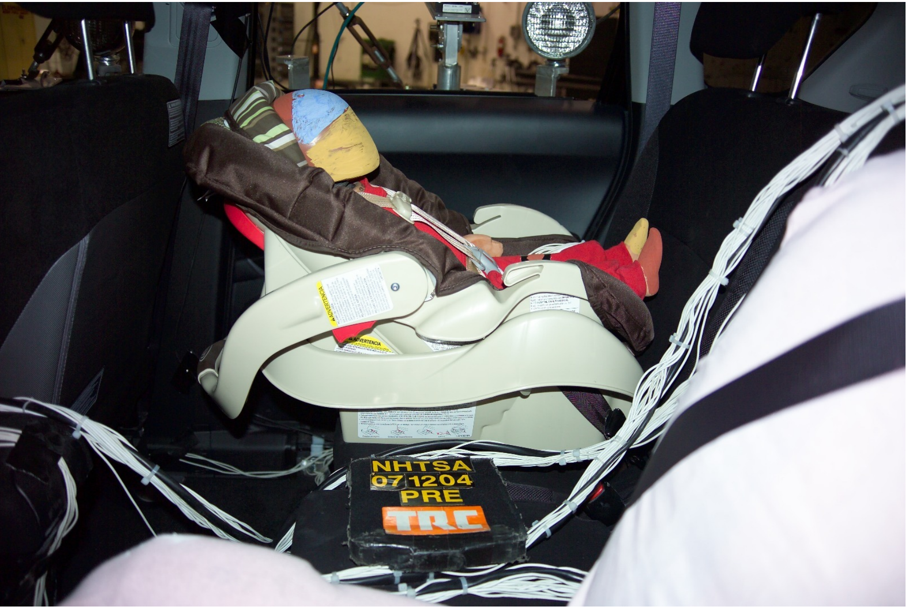
Figure D-10 Pre-Test Left Side View of Right Rear Dummy
