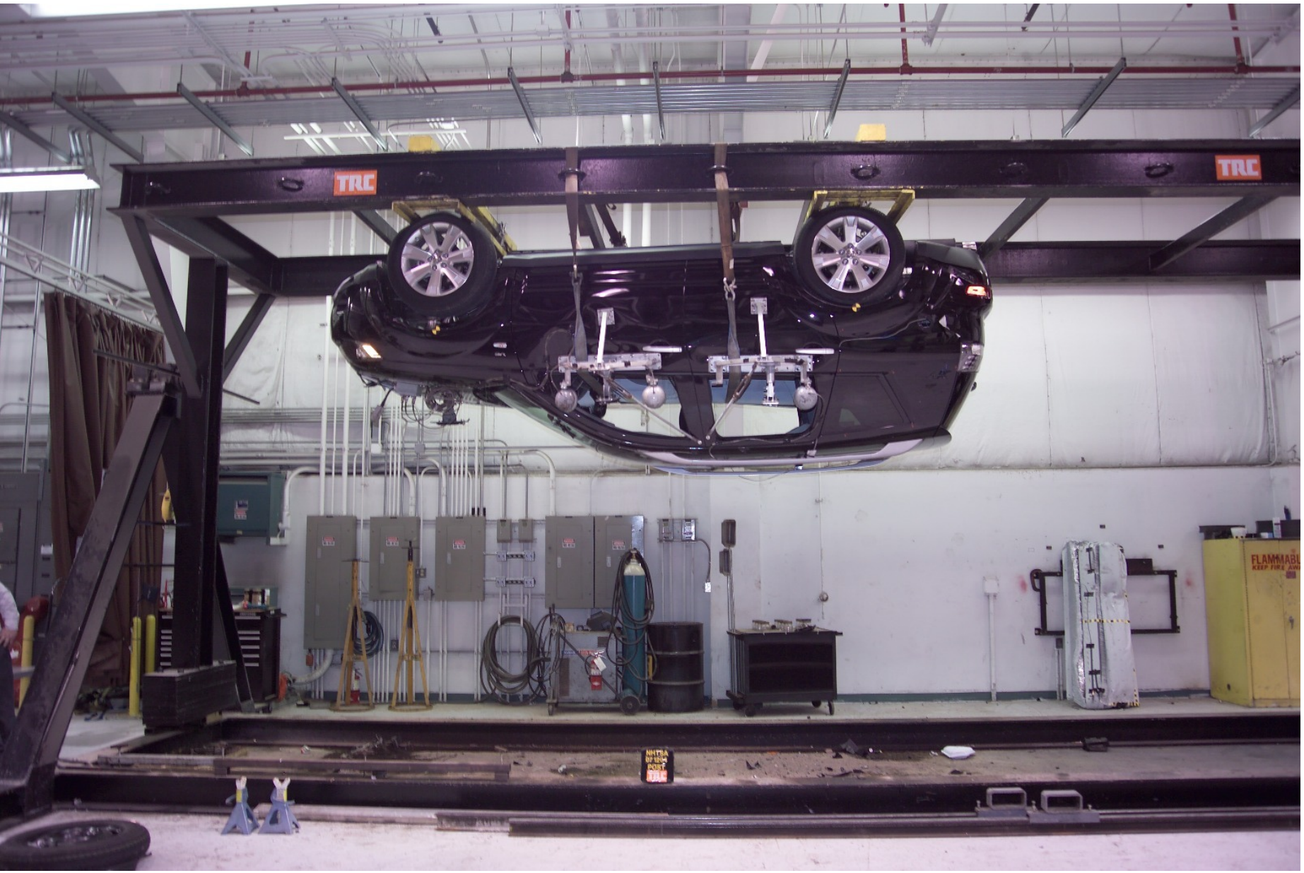
Figure A-84 FMVSS 301 Rollover View at 180°
