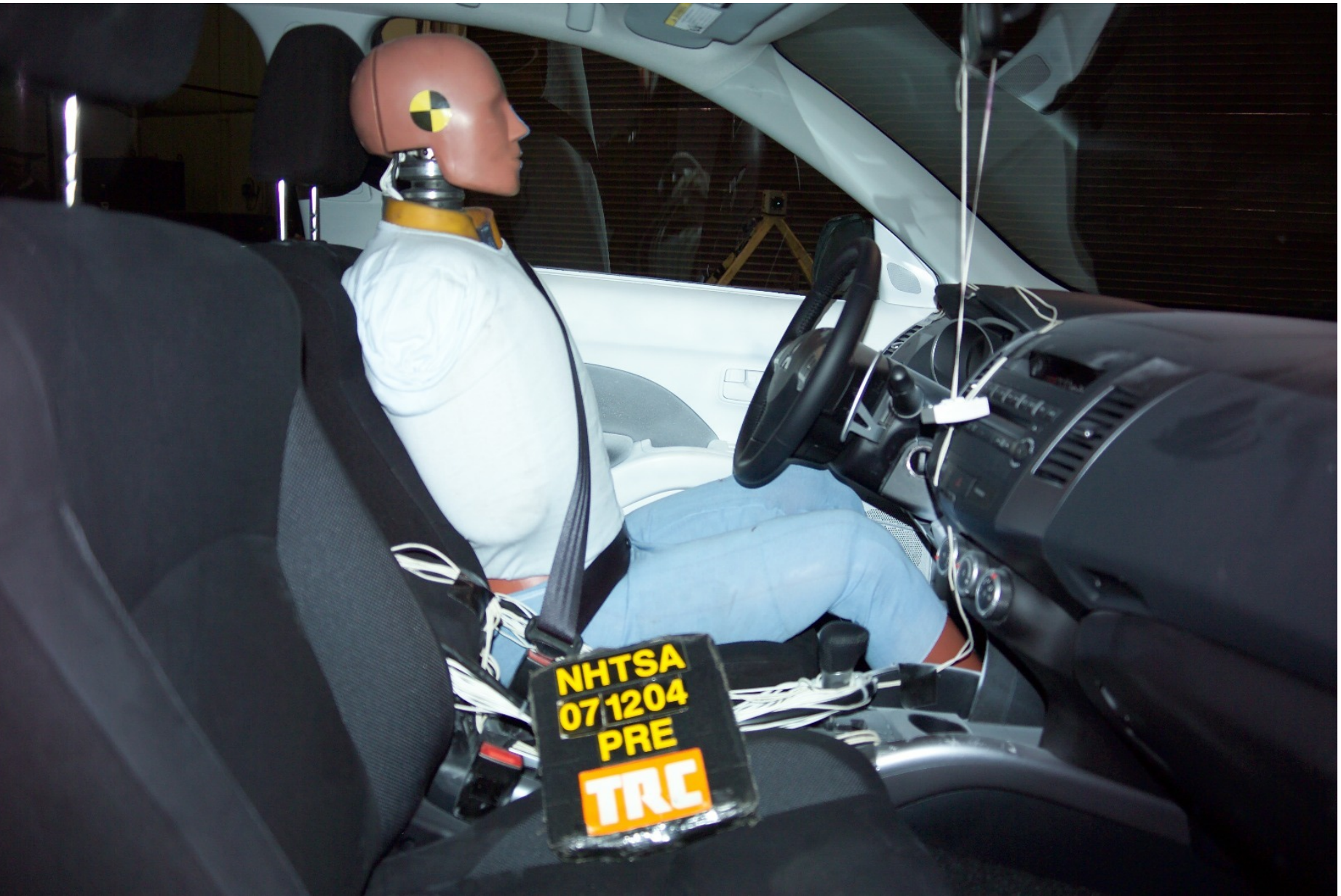
Figure A-45 Pre-Test Right Occupant Compartment View of Front SID
