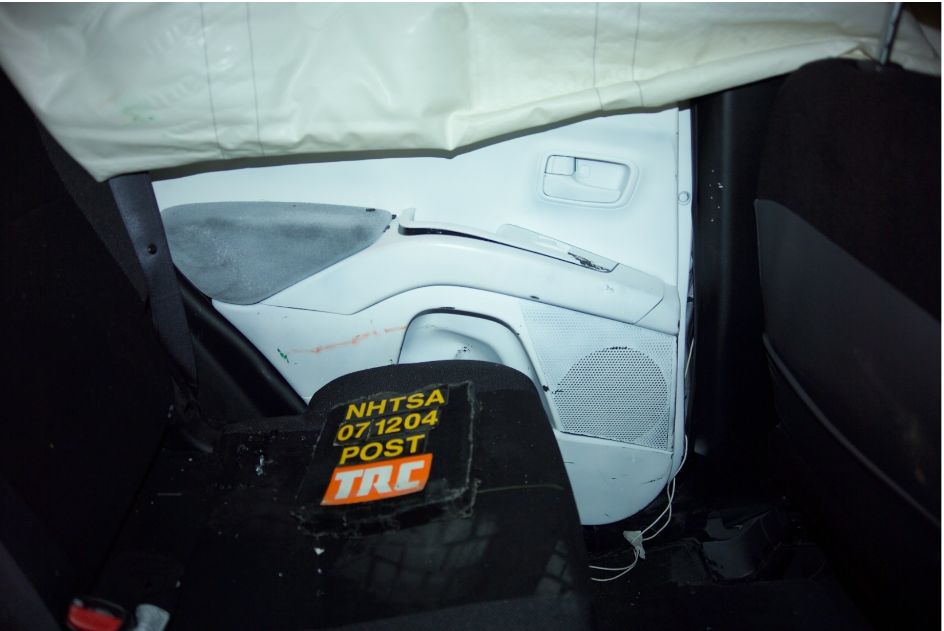
Figure A-64 Post-Test Interior of Rear Door Showing SID Impact Locations
