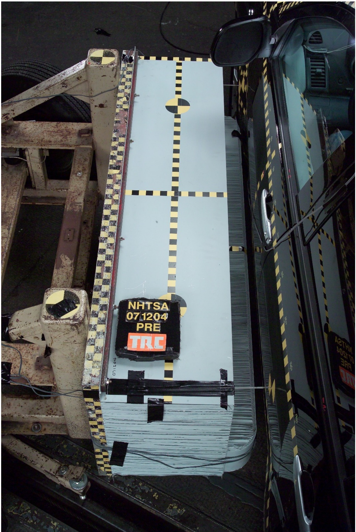
Figure A-43 Pre-Test Overhead View of MDB Aligned with Vehicle
