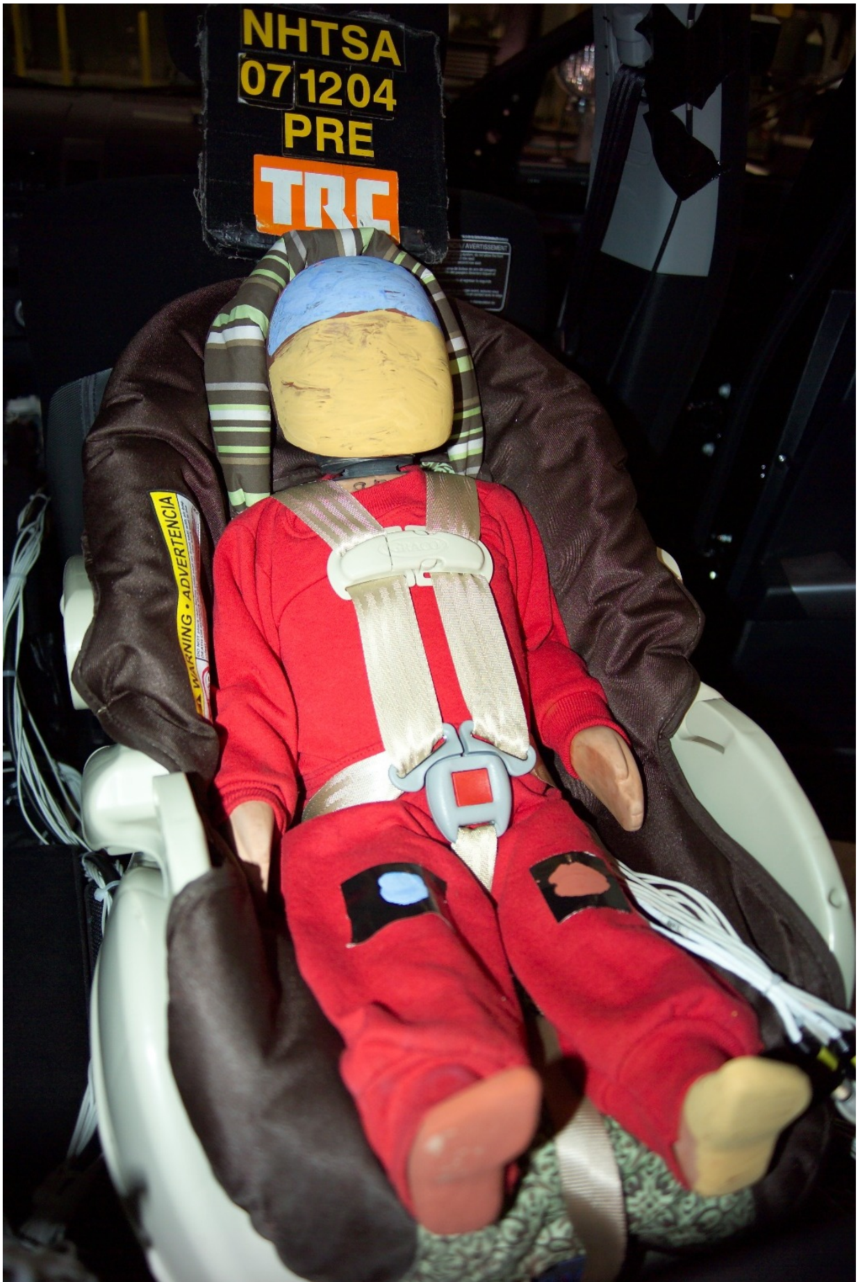
Figure D-8 Pre-Test Front View of Right Rear Dummy
