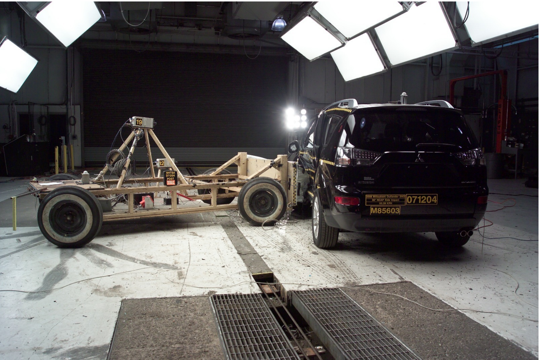
Figure A-72 Post-Test Right Side View of MDB with Impactor Face in Position
