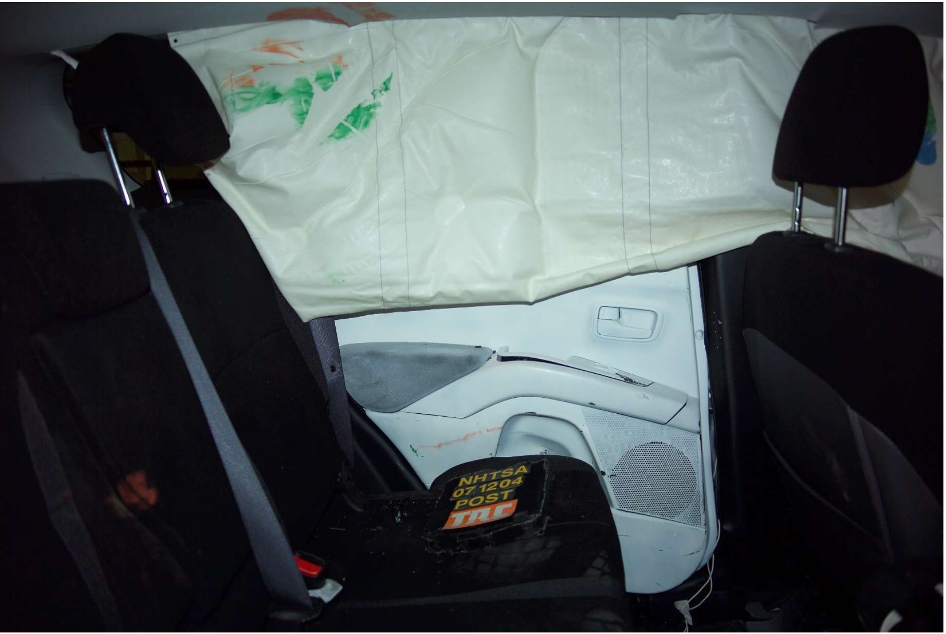
Figure A-66 Post-Test Rear SID Contact - View 2
