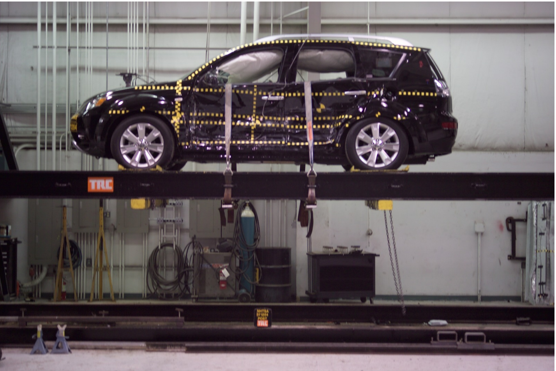
Figure A-86 FMVSS 301 Rollover View at 360°
