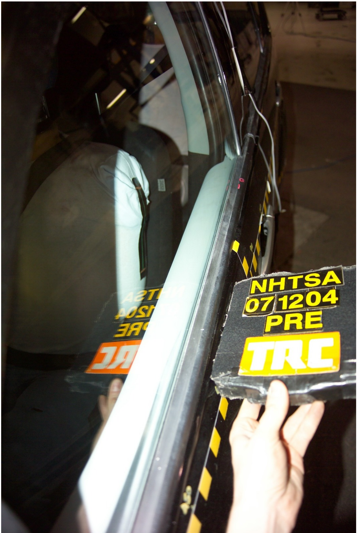
Figure A-52 Pre-Test Left View of Front SID and Door Clearance
