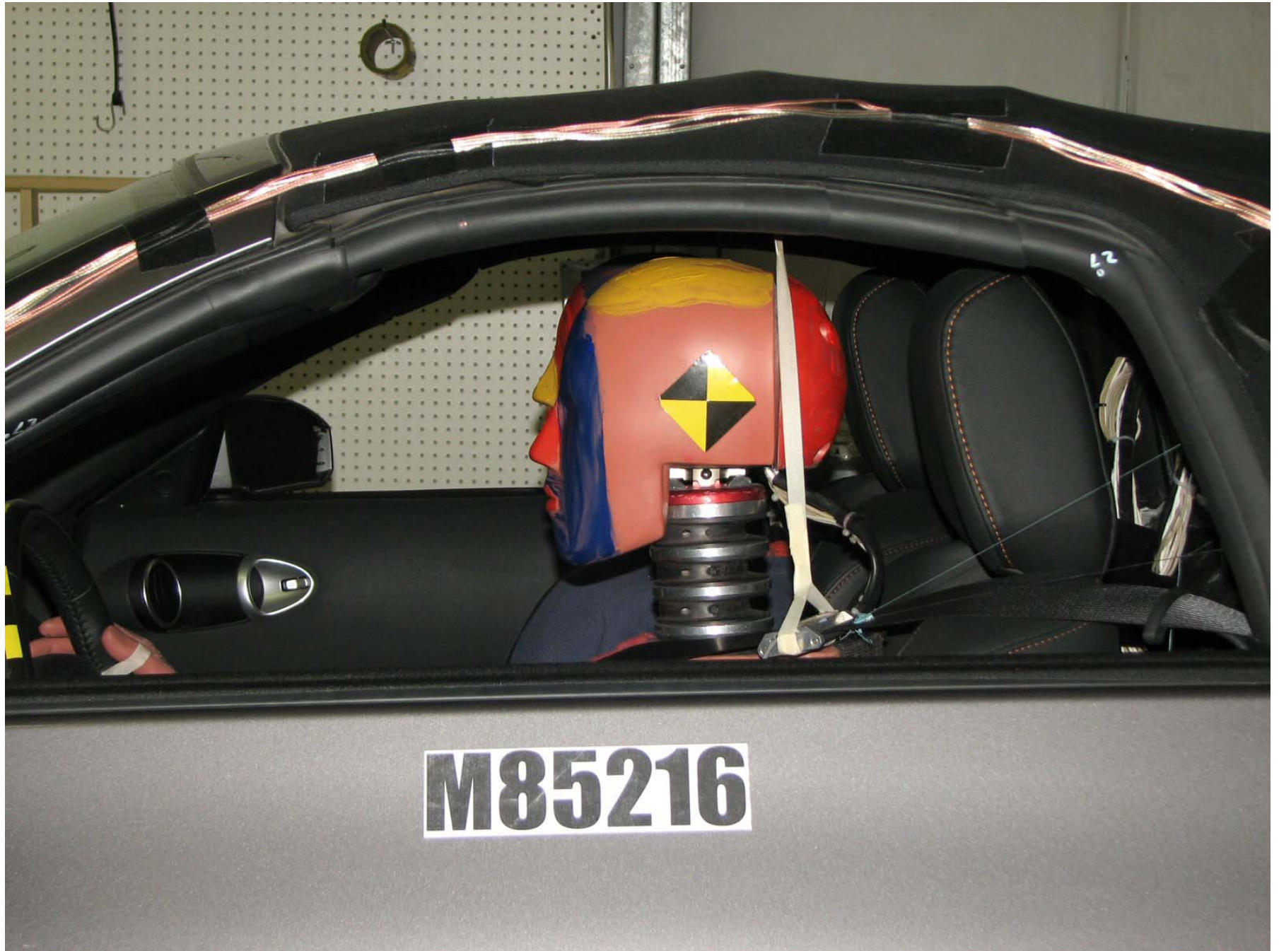
Figure A-32: Pre-Test Driver Dummy (Through Window)
