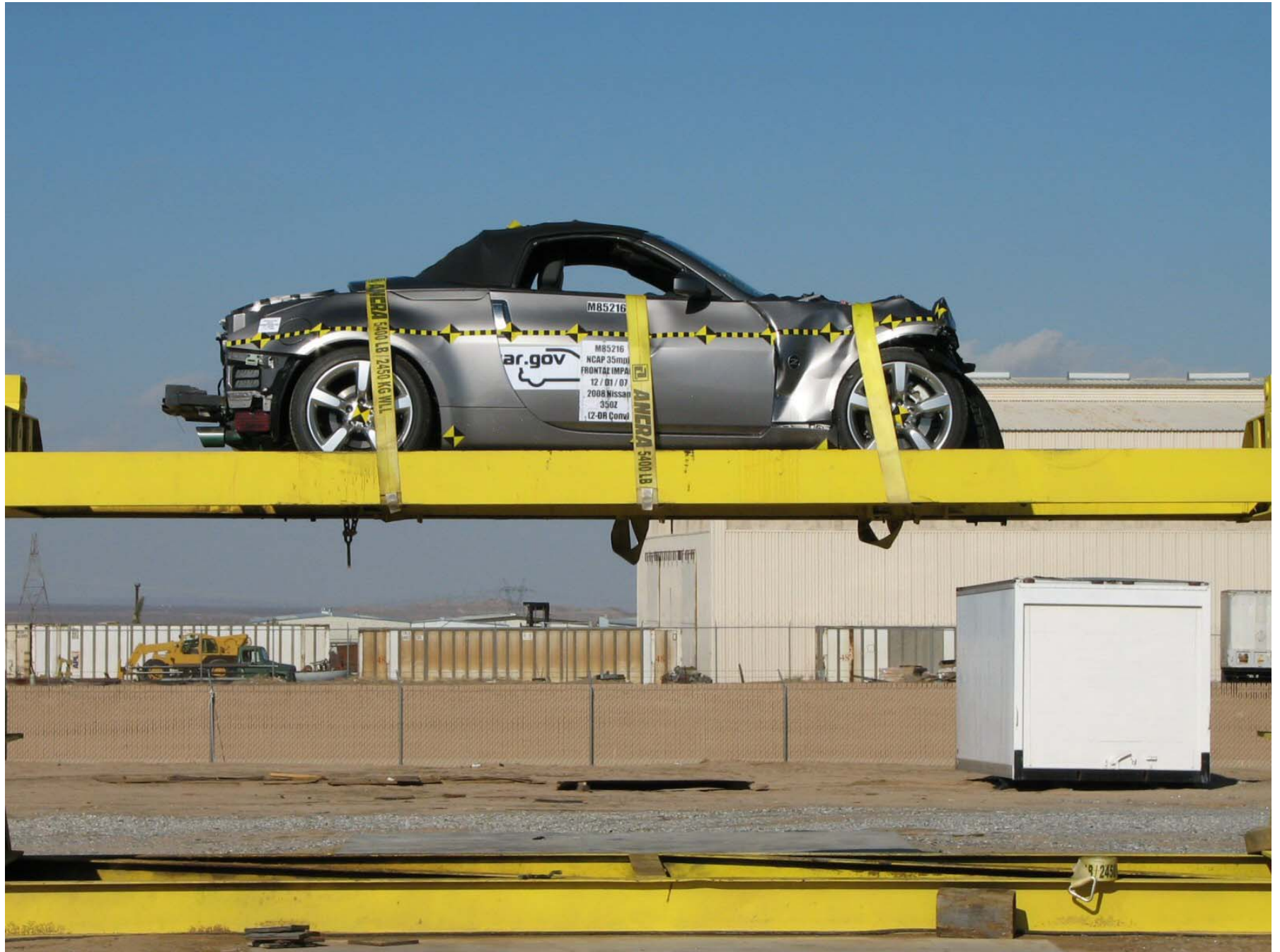
Figure A-58: Vehicle on Rollover Device (0°)
