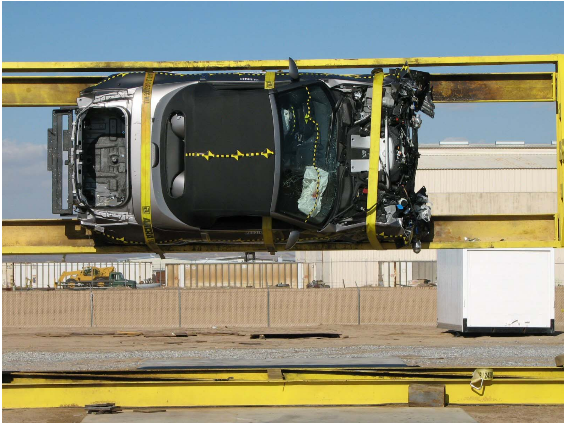
Figure A-59: Vehicle on Rollover Device (90°)
