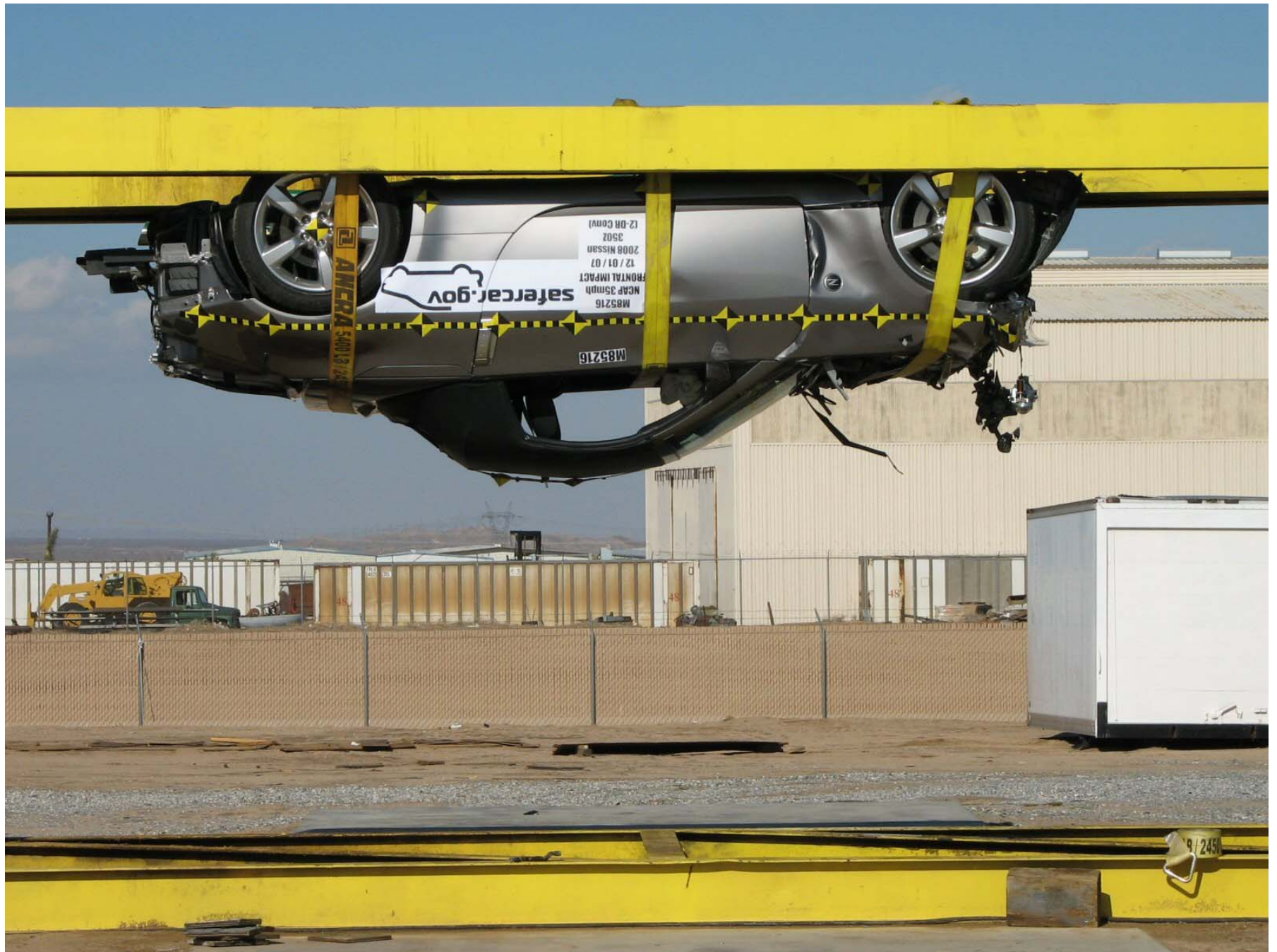
Figure A-60: Vehicle on Rollover Device (180°)
