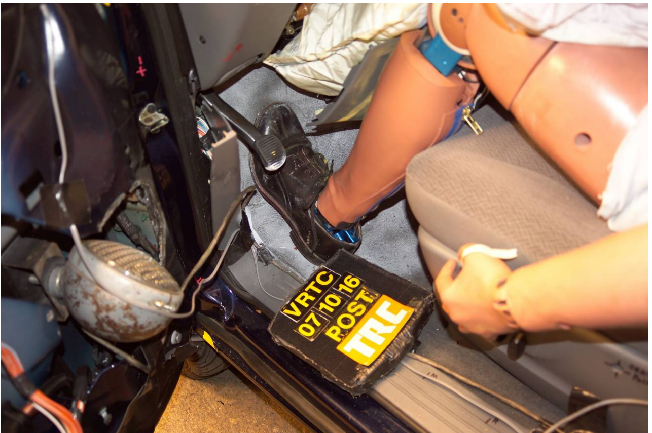
Figure A-50 Post-Test Driver Dummy Foot Position View
