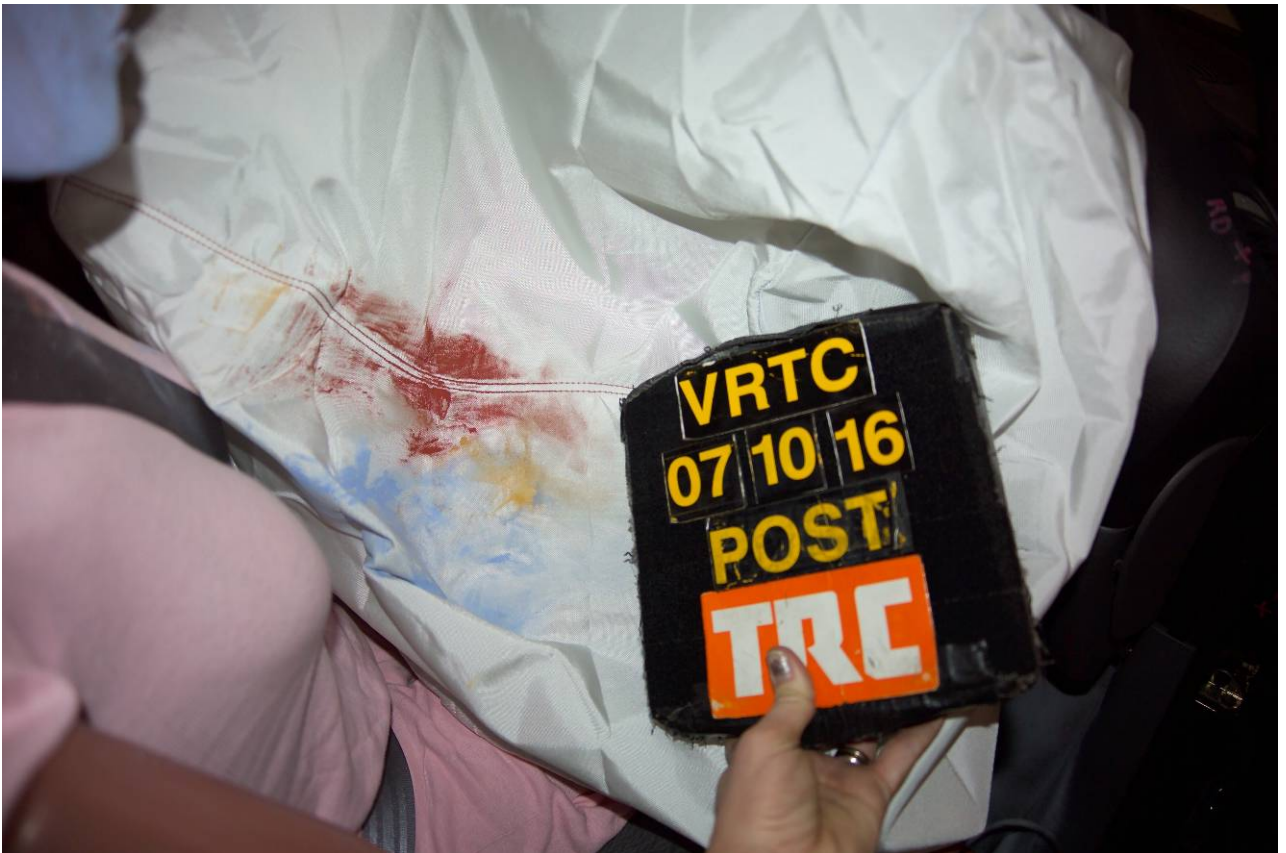
Figure A-72 Post-Test Passenger Dummy Head Contact – View 1
