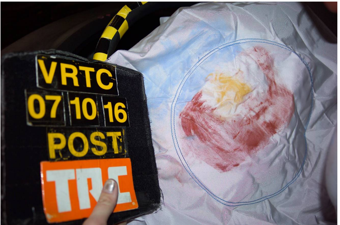
Figure A-58 Post-Test Driver Dummy Head Contact - View 1
