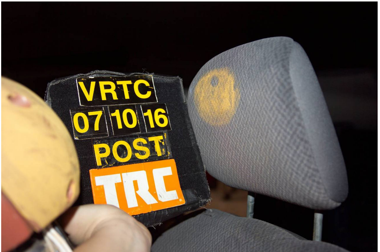
Figure A-59 Post-Test Driver Dummy Head Contact - View 2
