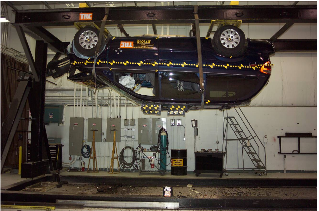
Figure A-89 Vehicle on Rollover Fixture – 180°
