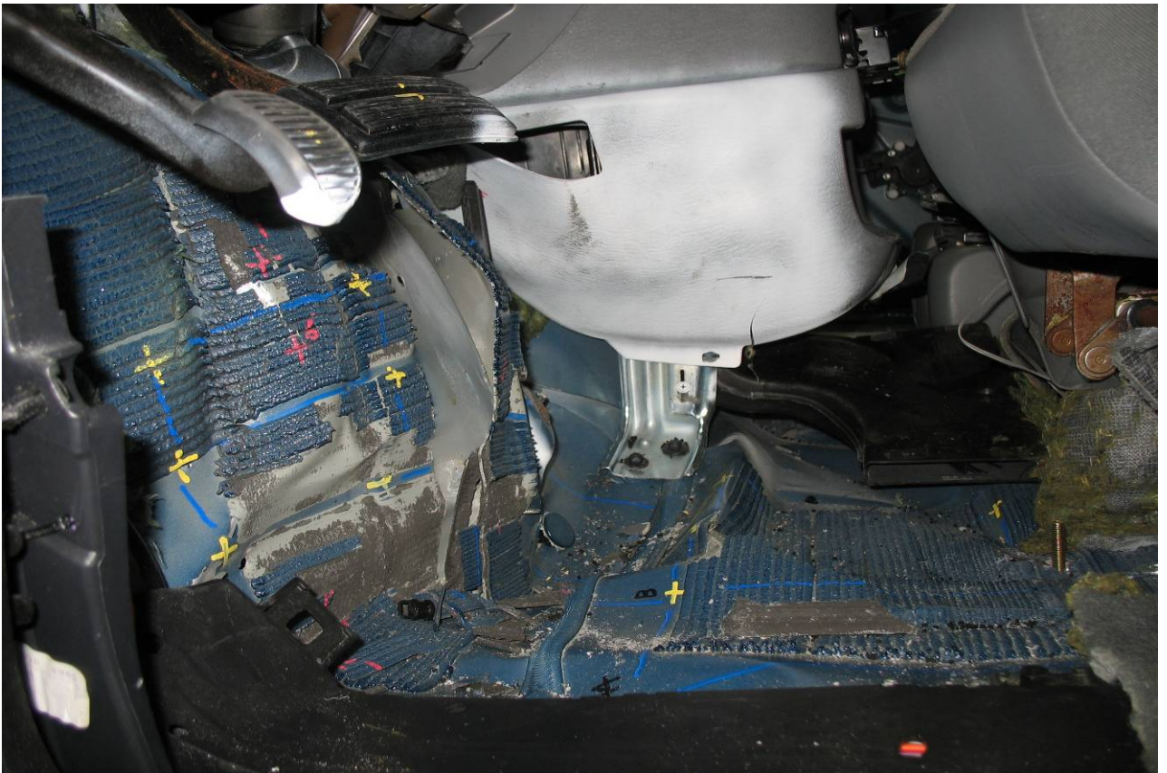
Figure A-95 Post-Test Driver Floorpan – View 2
