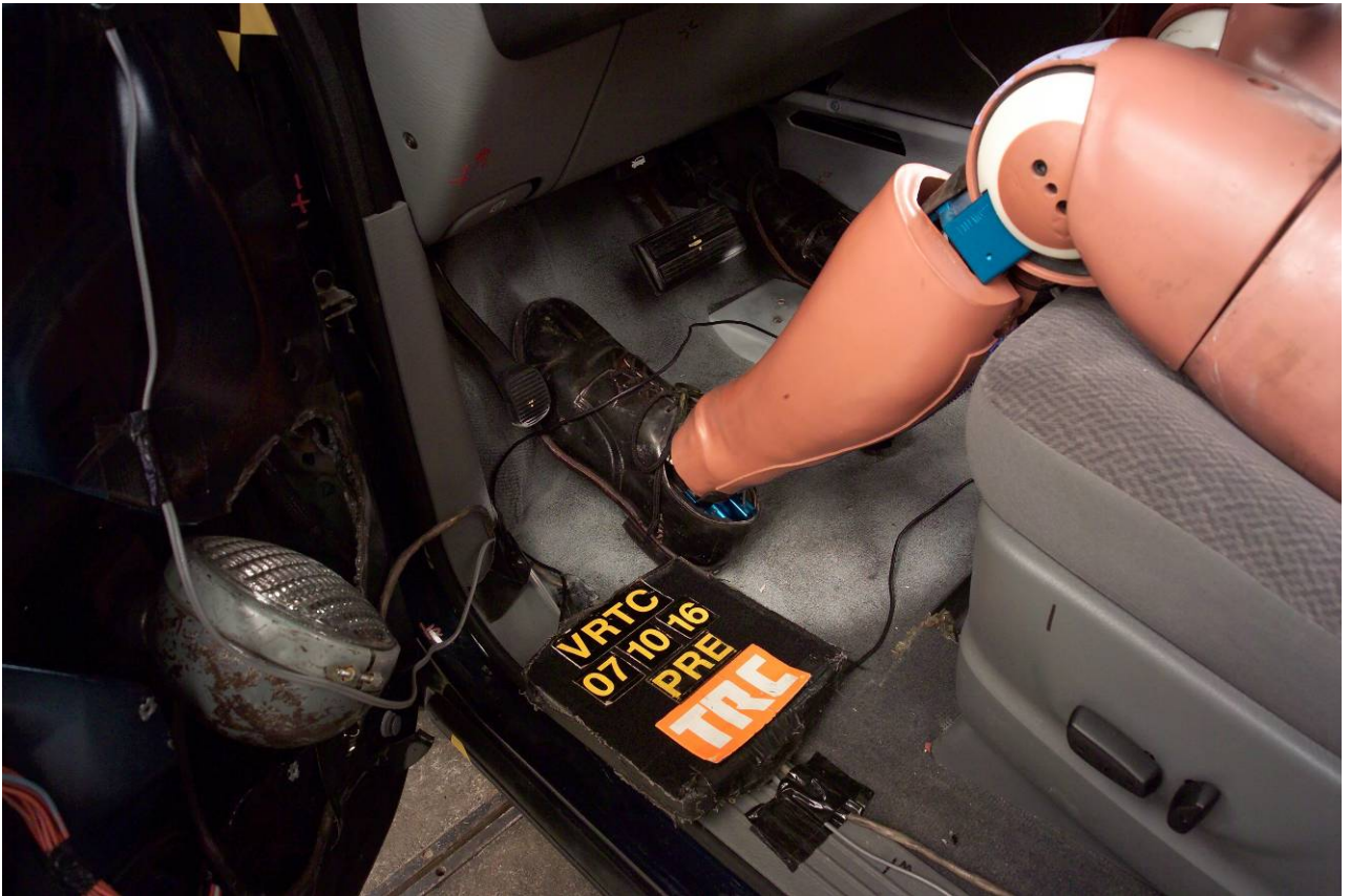
Figure A-49 Pre-Test Driver Dummy Foot Position View
