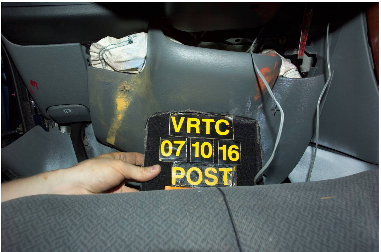
Figure A-60 Post-Test Driver Dummy Knee Contact View
