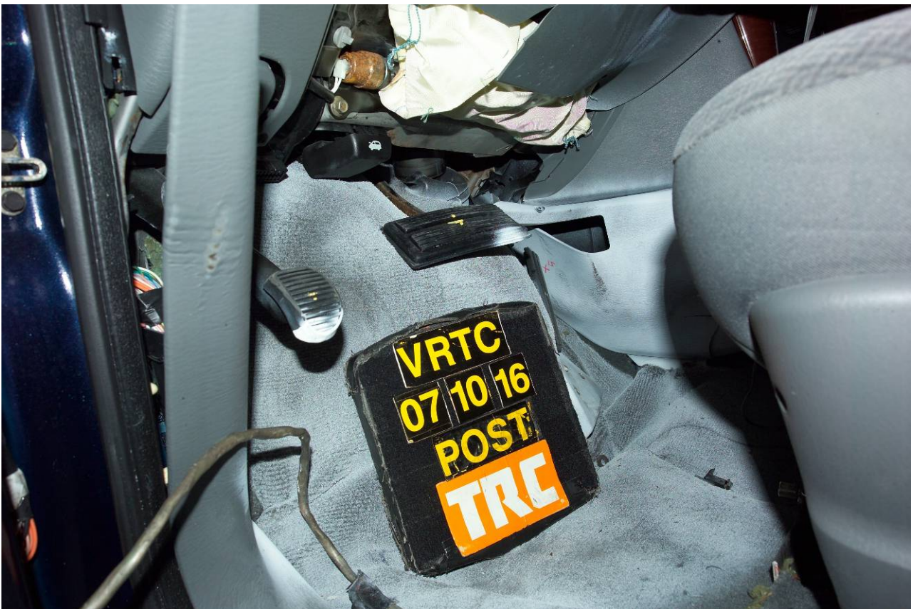
Figure A-54 Post-Test Driver Floorpan Deformation View
