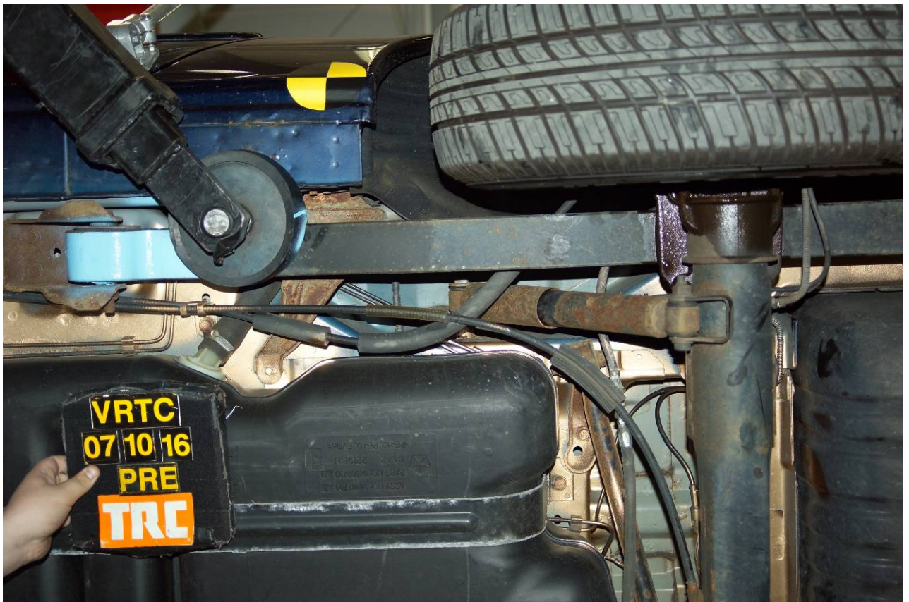
Figure A-31 Pre-Test Fuel Filler Neck View
